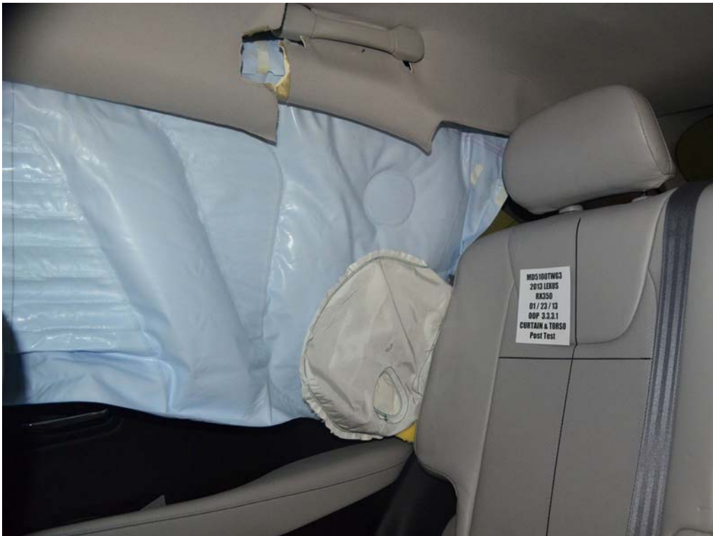
FIGURE 14. Post-Test Airbags, Left Front ¾ View
