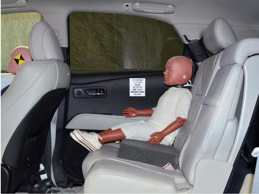
FIGURE 7. Pre-Test Dummy Position, Left Side View
