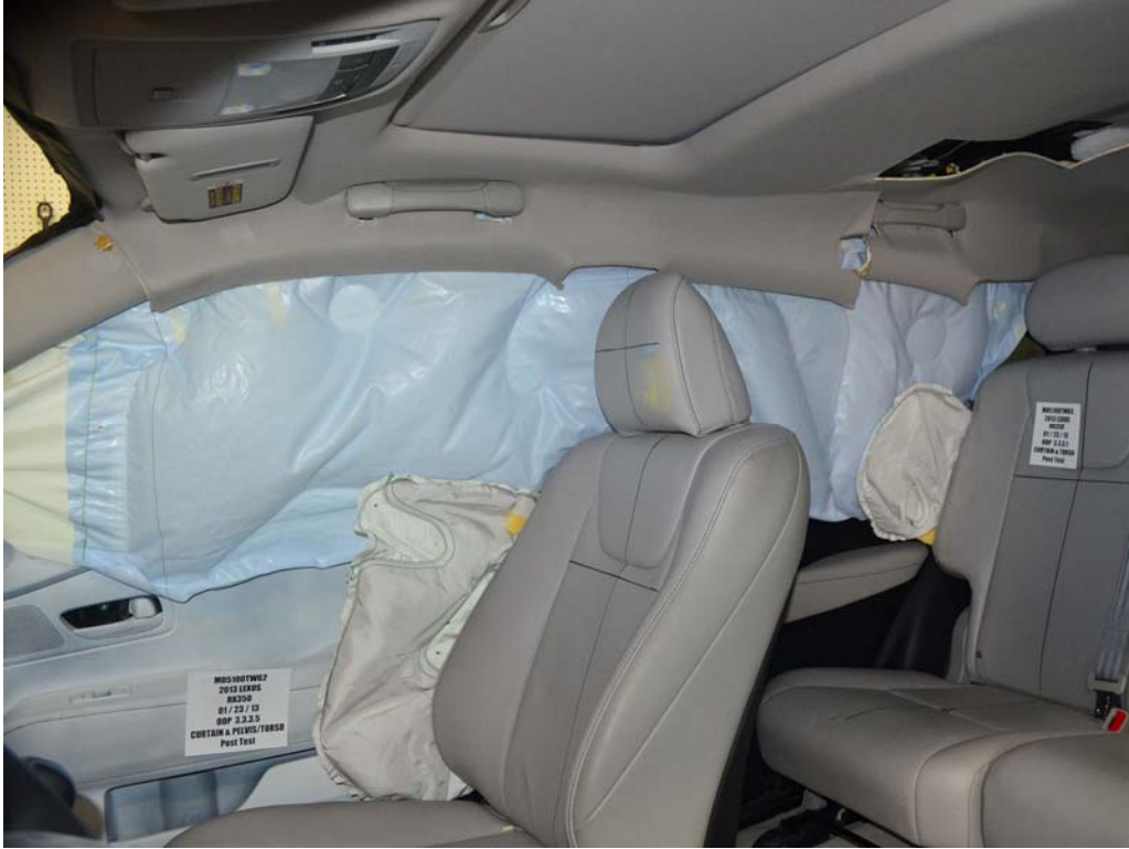
FIGURE 13. Post-Test Airbags, Left Side View
