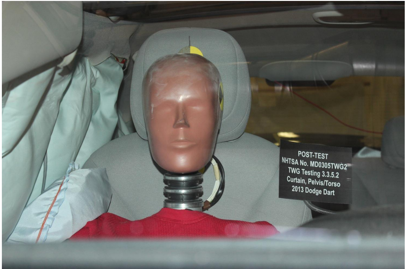
Figure A-21: Post-Test Curtain Airbag Front View
