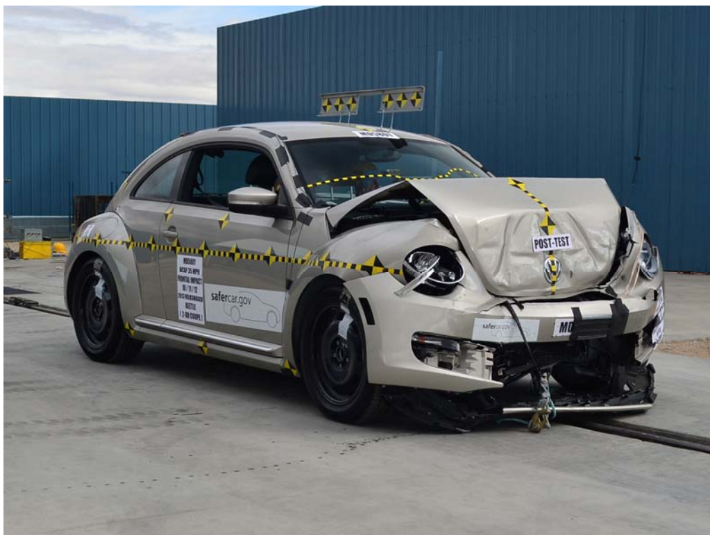
FIGURE 4. Post-Test Right Front 3/4 View of NCAP Frontal Impact Test
