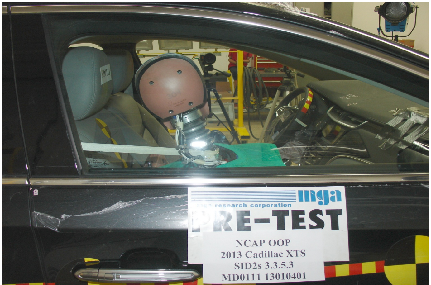
Pre-Test SID-IIs Dummy Right Side View
