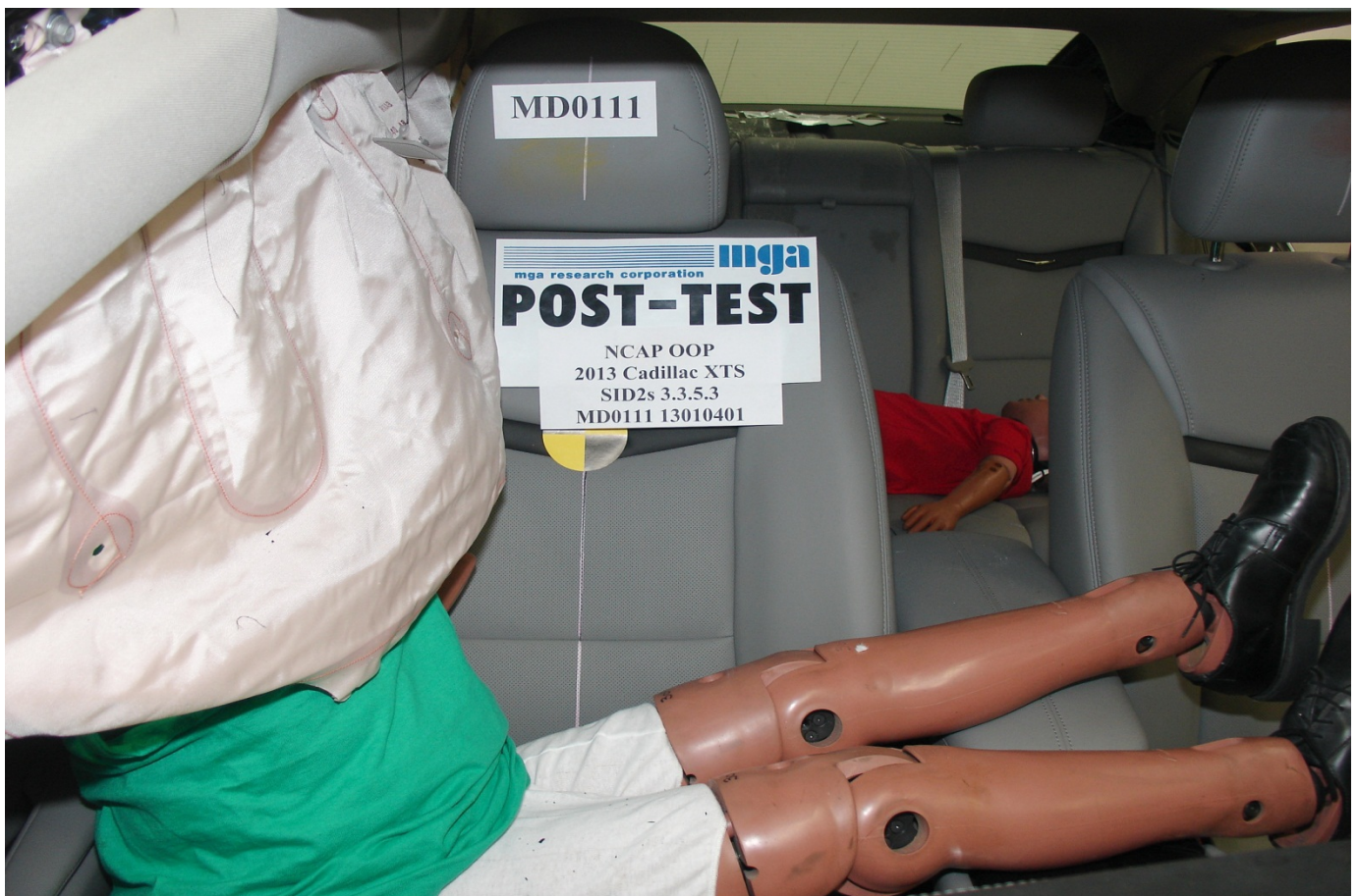
Post-Test SID-IIs Dummy Front View
