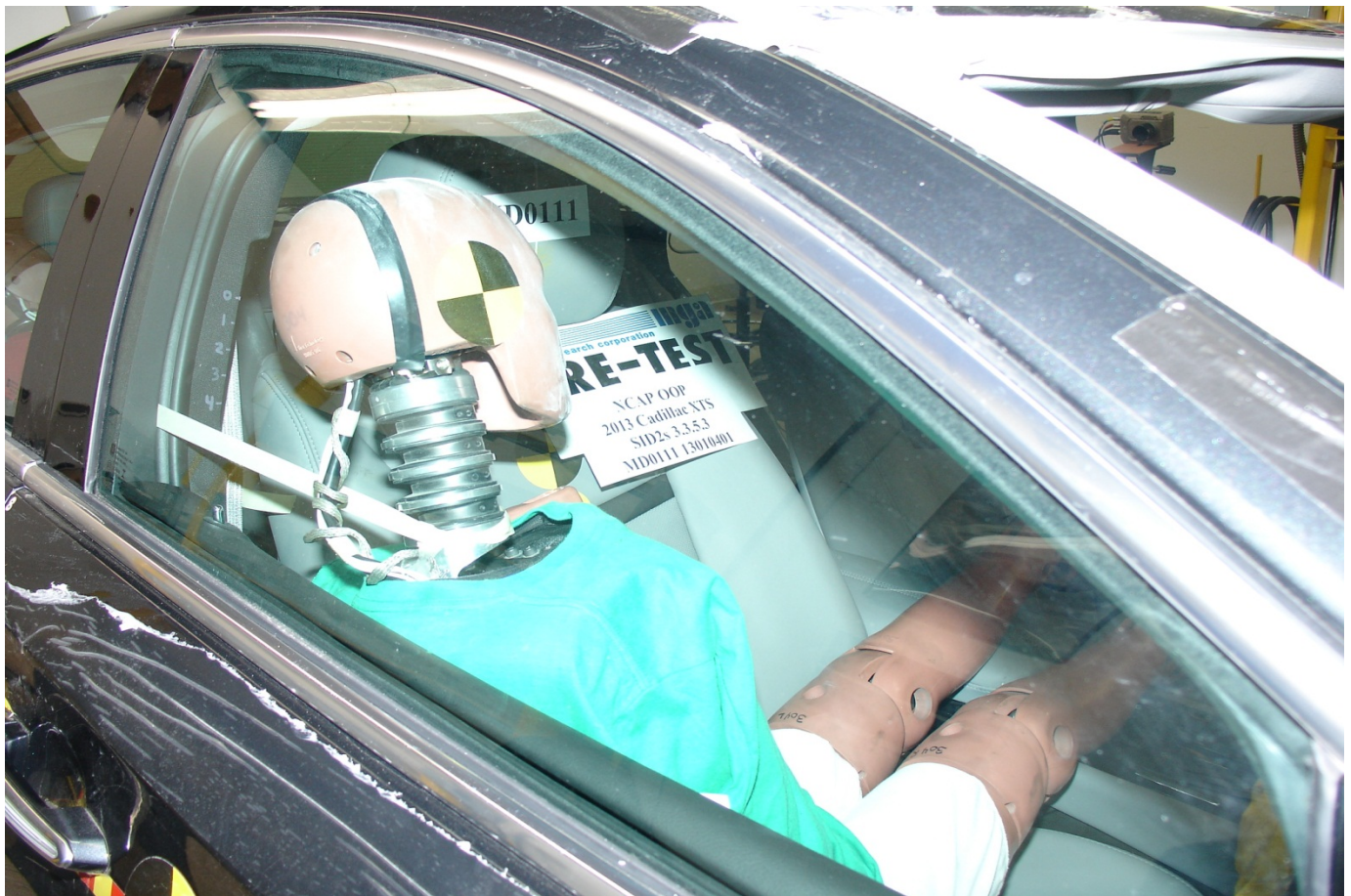
Pre-Test SID-IIs Dummy Right \frac{3}{4} Front View
