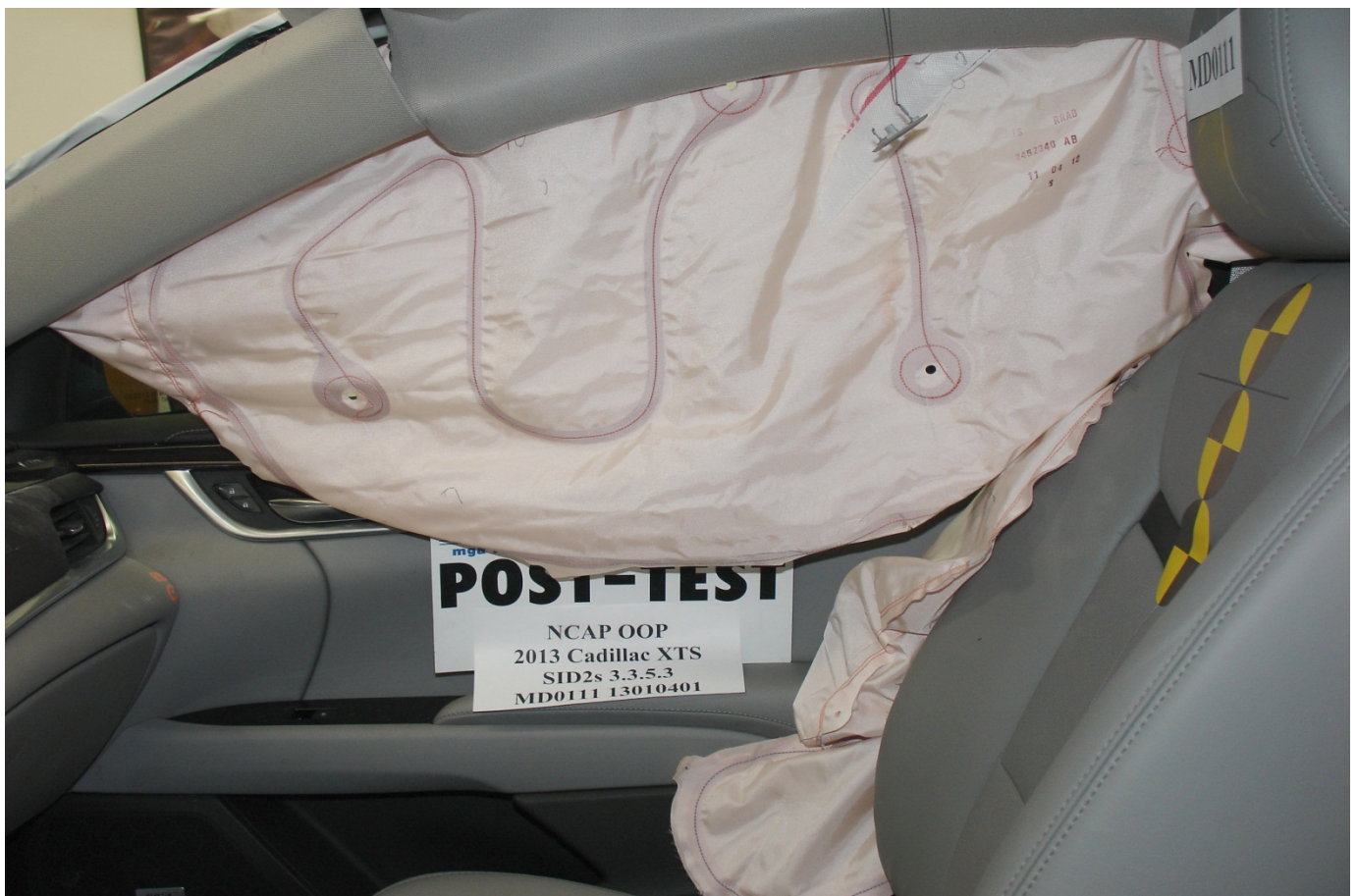
Post-Test Curtain Airbag Left Side View
