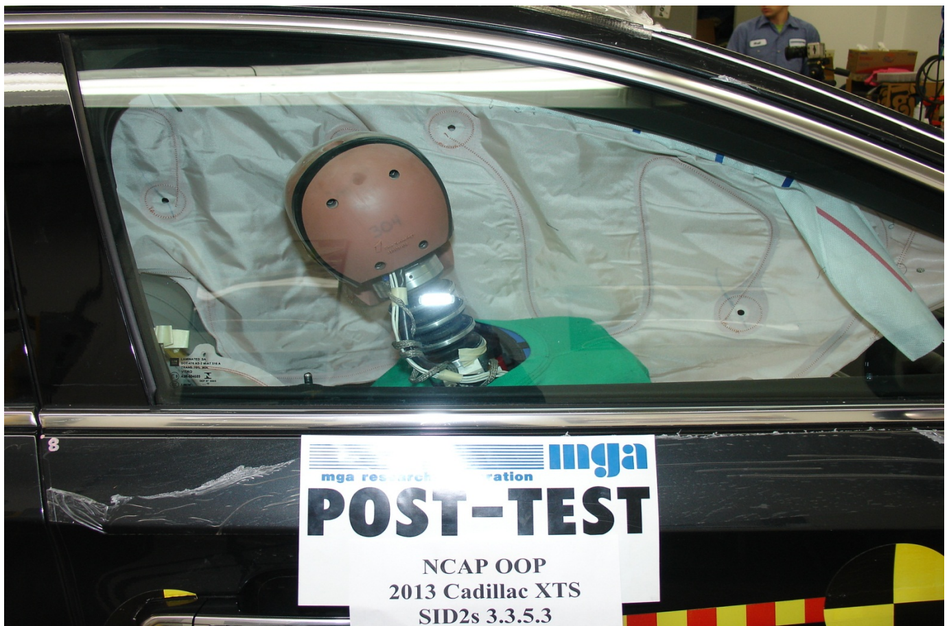
Post-Test SID-IIs Dummy Right Side View
