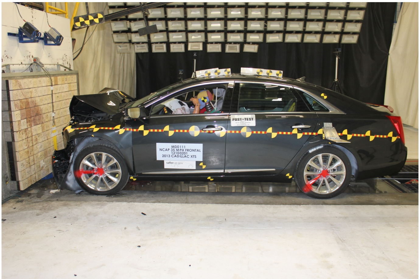
Post-Test Vehicle Left Side View
