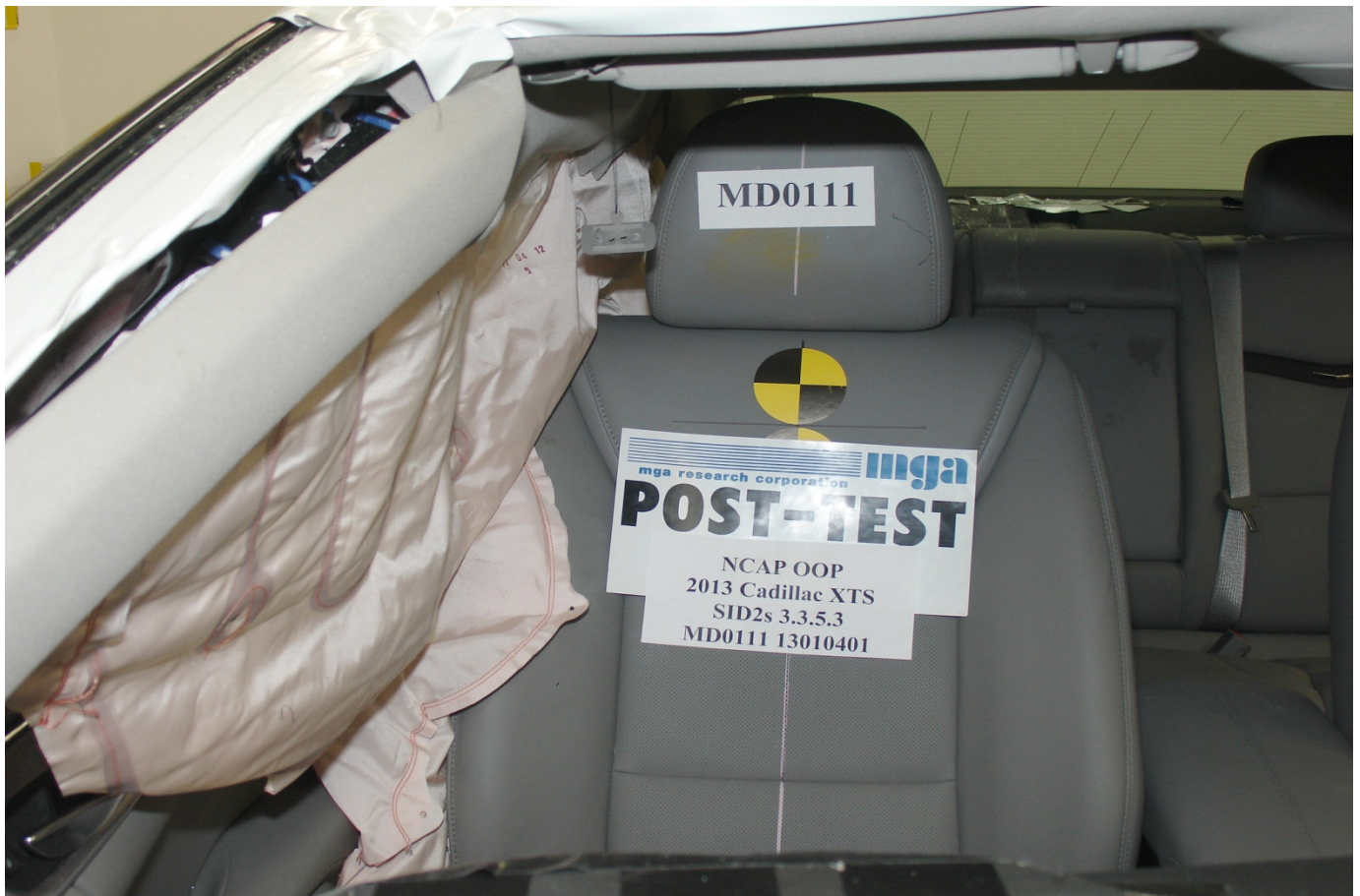
Post-Test Curtain Airbag Front View
