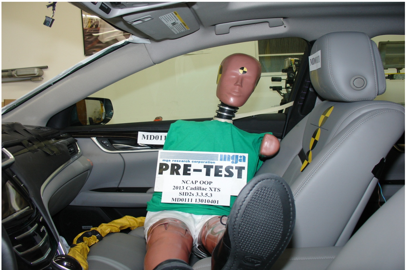
Pre-Test SID-IIs Dummy Left Side View
