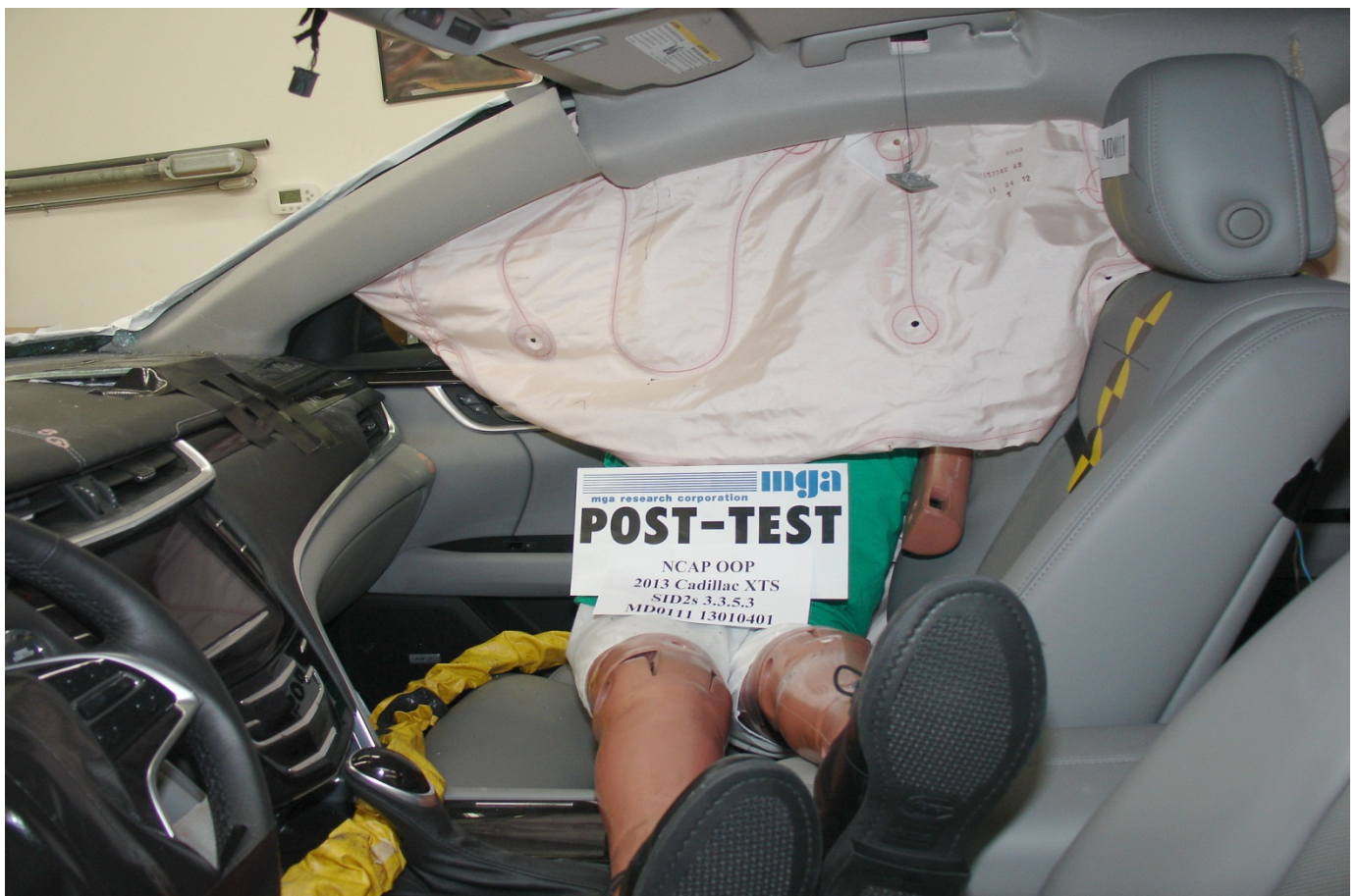
Post-Test SID-IIs Dummy Left Side View
