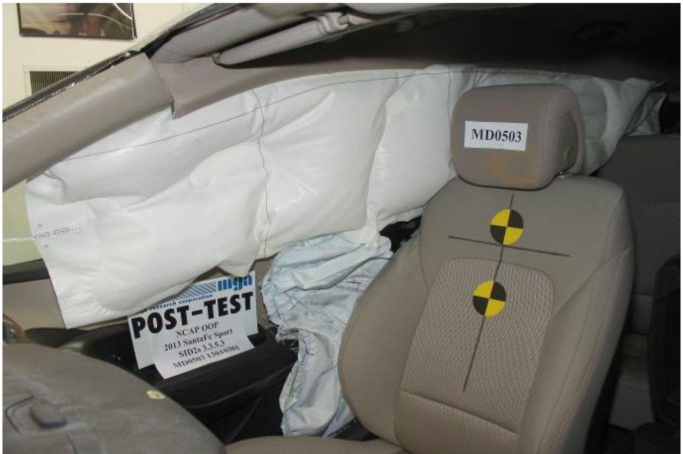
Post-Test Curtain Airbag Left ¾ Front View
