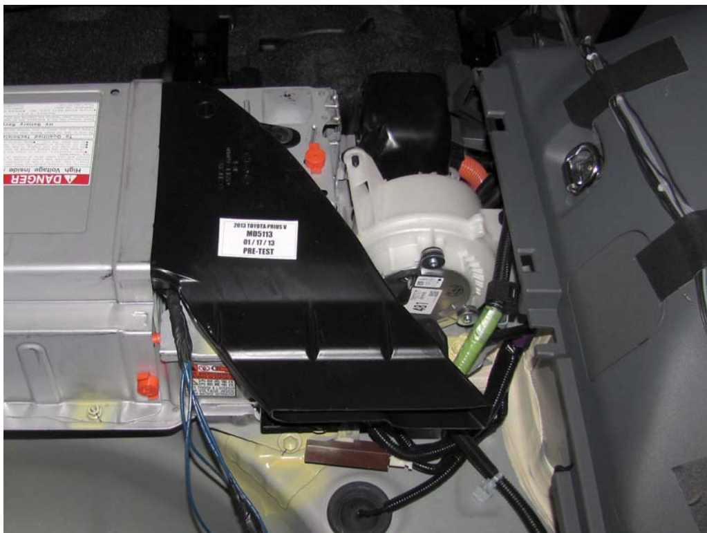
FIGURE 19. Pre-Impact View of Propulsion Battery Venting System(s)
