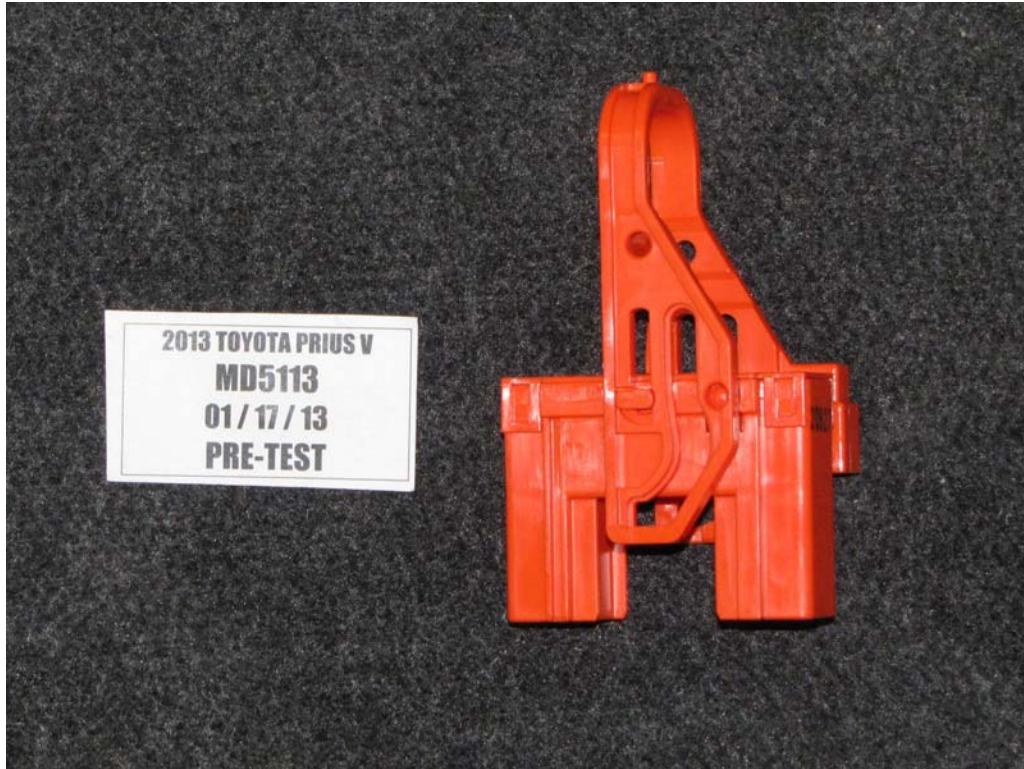
FIGURE 7. Manual High Voltage Service Disconnect Removed
