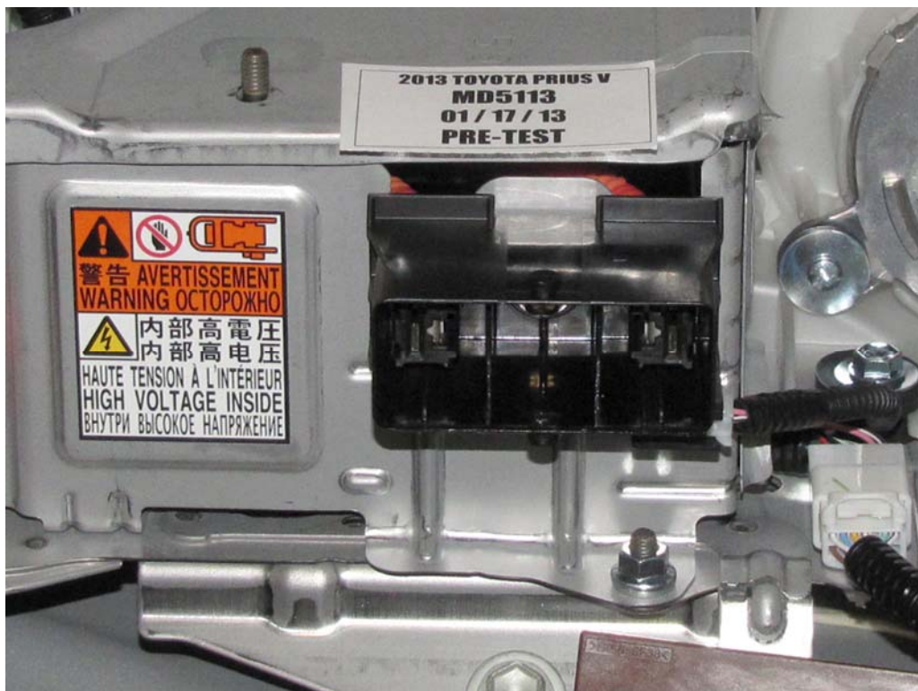
FIGURE 8. Manual High Voltage Service Disconnect Removed
