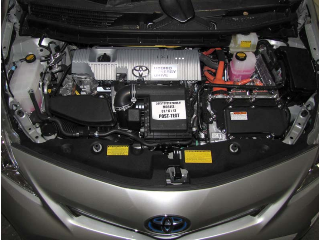
FIGURE 17. Post-Impact View of Electric Propulsion Drive
