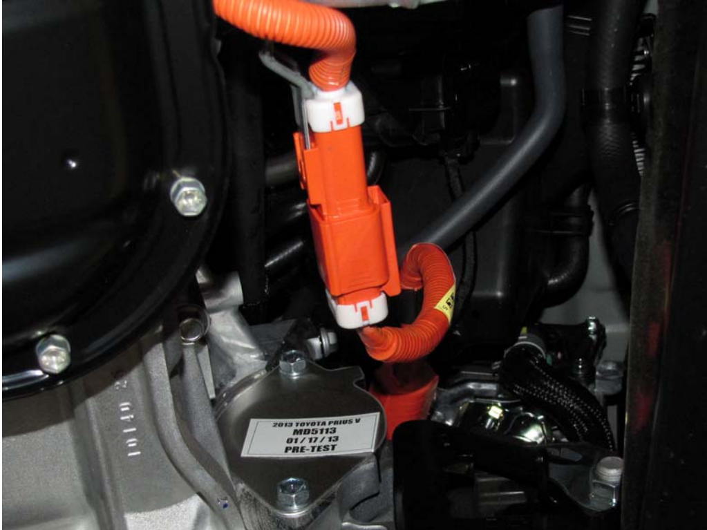
FIGURE 18. Pre-Impact View of High Voltage Interconnect(s)
