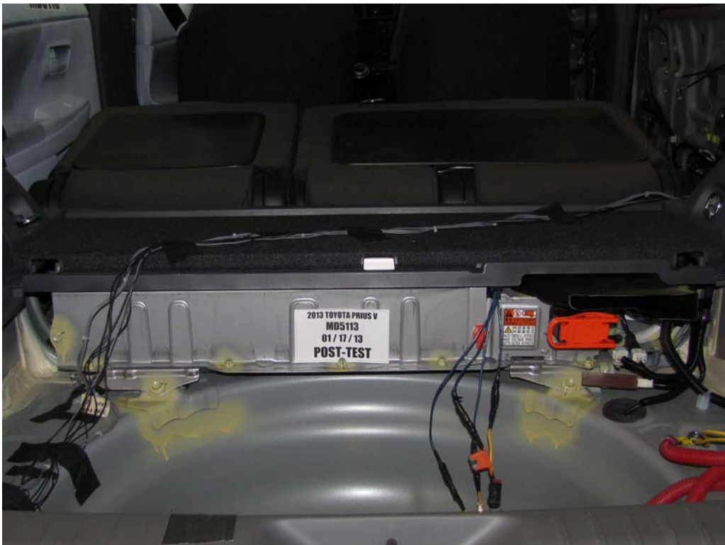
FIGURE 11. Post-Impact Rear View of Propulsion Battery
