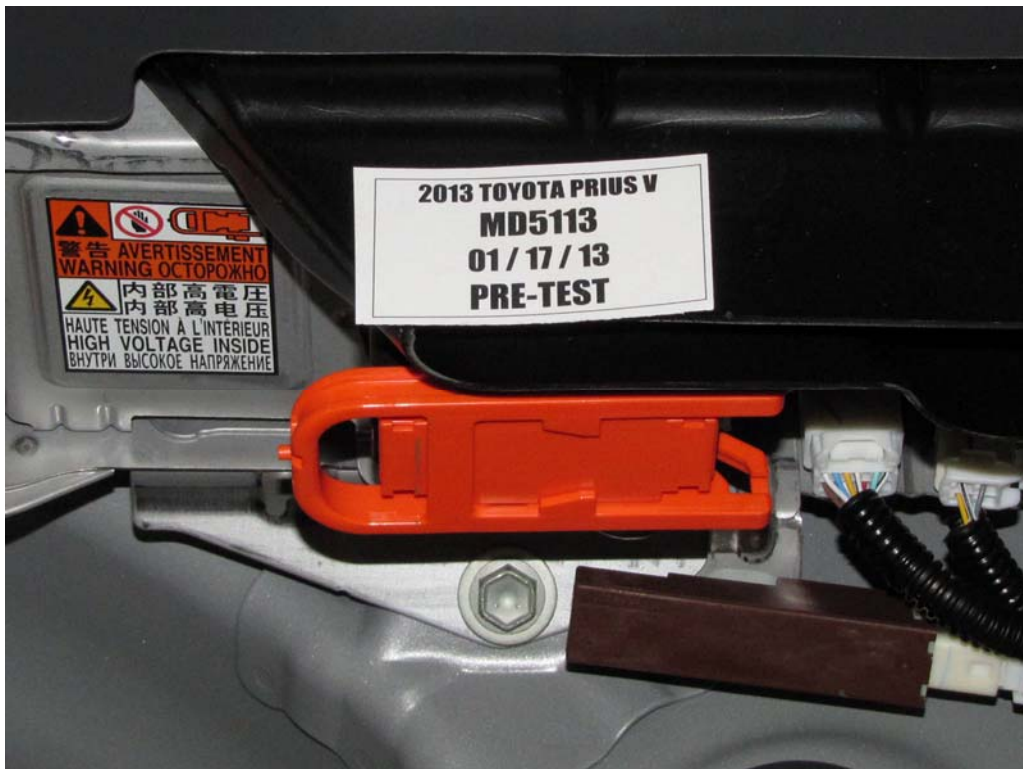
FIGURE 6. Manual High Voltage Service Disconnect In Place
