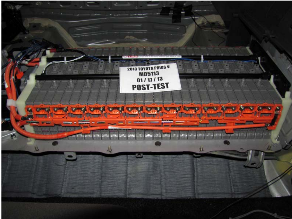
FIGURE 15. Post-Impact View of Propulsion Battery Modules
