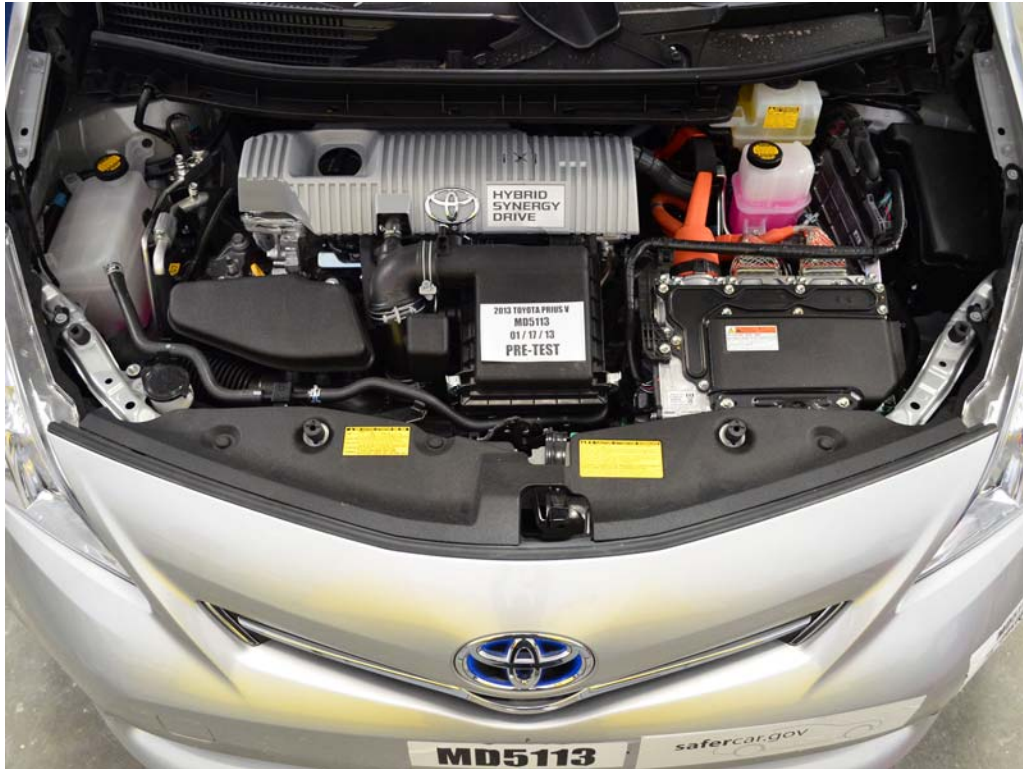
FIGURE 16. Pre-Impact View of Electric Propulsion Drive
