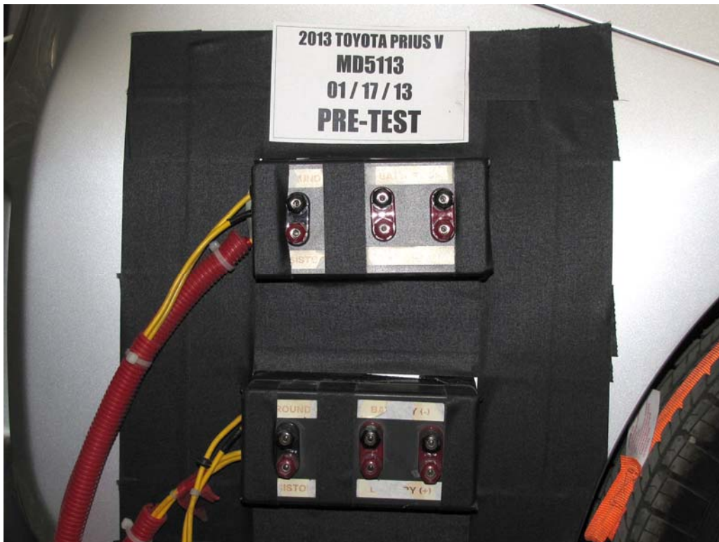
FIGURE 24. Pre-Impact View of Installed Test Interface Port
