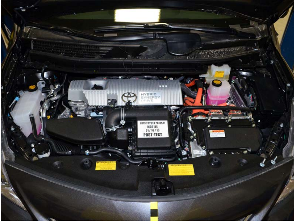
FIGURE 17. Post-Impact View of Electric Propulsion Drive
