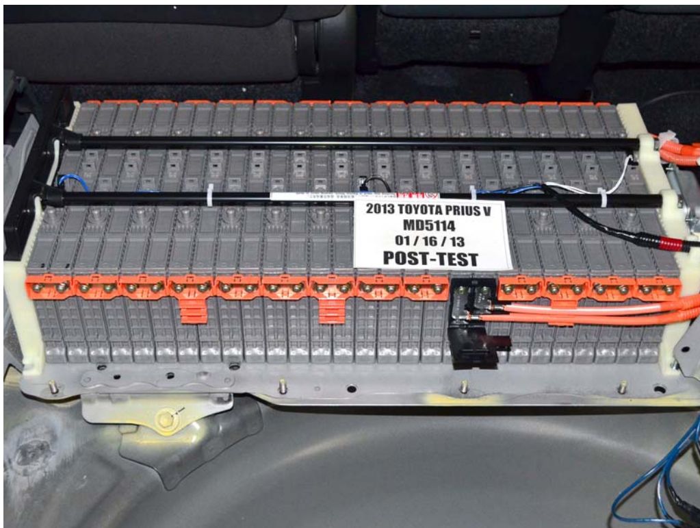
FIGURE 15a. Post-Impact View of Propulsion Battery Modules
