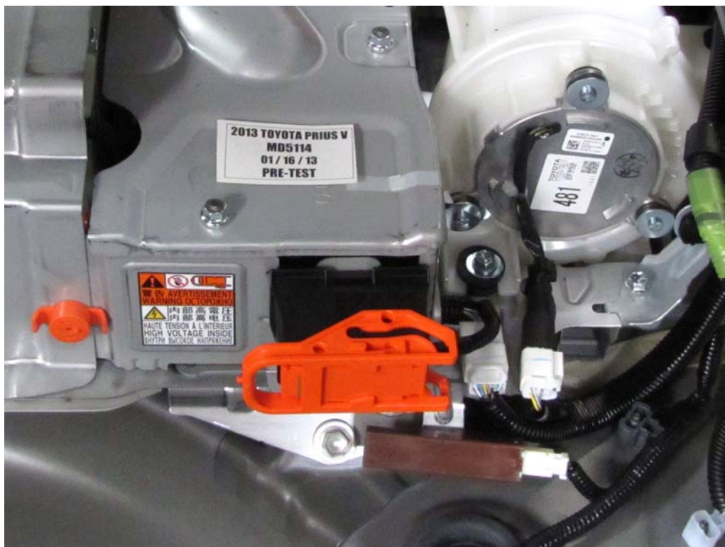
FIGURE 6. Manual High Voltage Service Disconnect In Place
