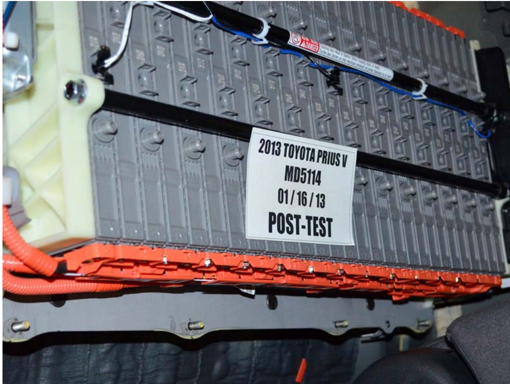
FIGURE 15. Post-Impact View of Propulsion Battery Modules
