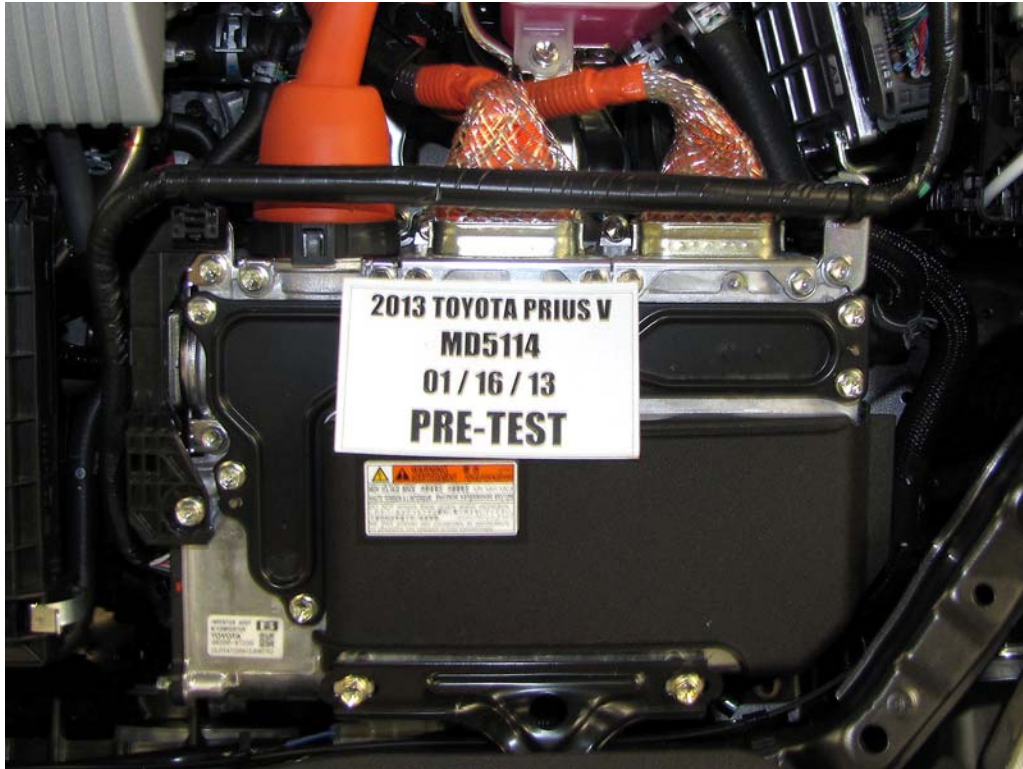
FIGURE 18b. Pre-Impact View of High Voltage Interconnect(s)
