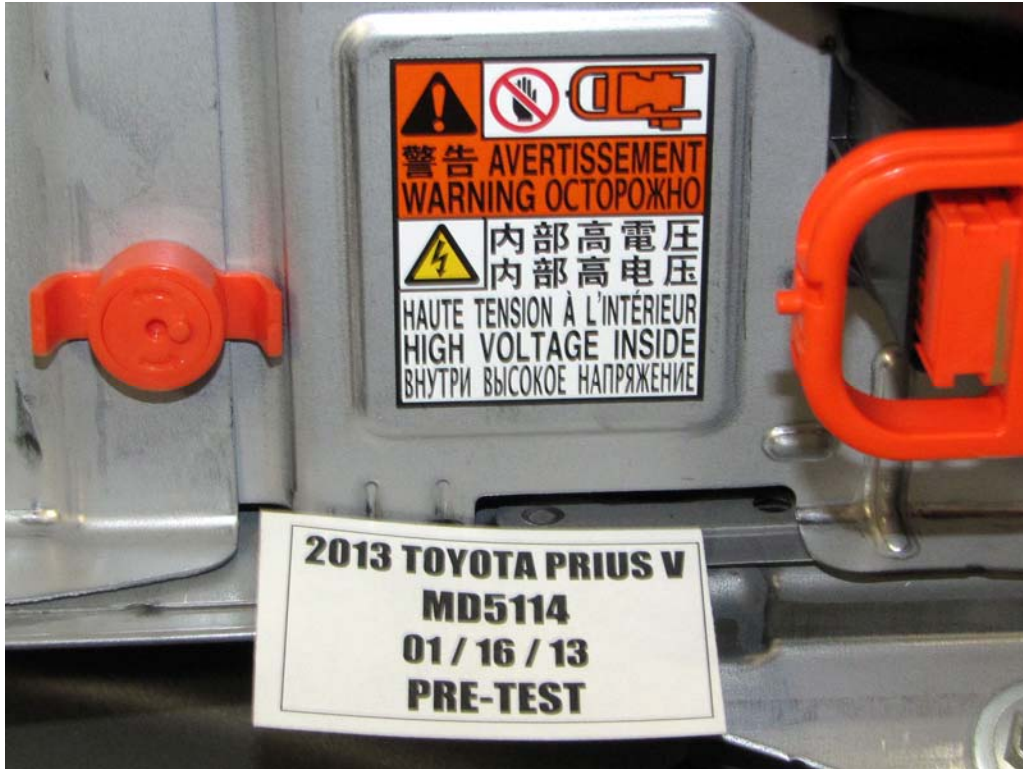
FIGURE 1b. Auxiliary Power Module Warning Label
