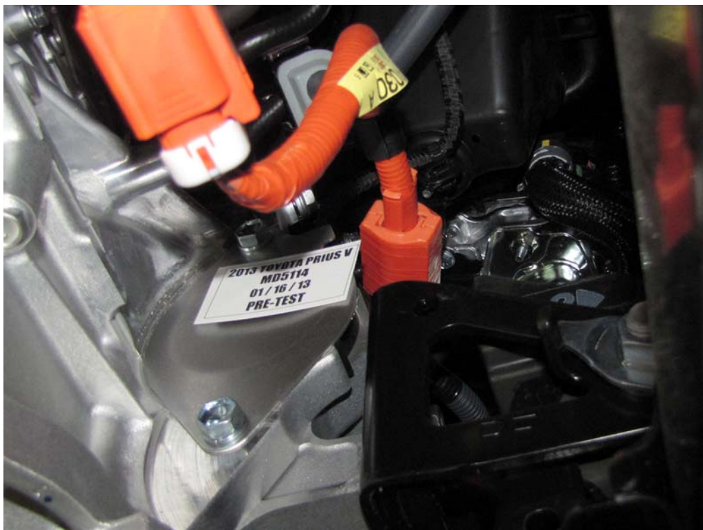
FIGURE 18a. Pre-Impact View of High Voltage Interconnect(s)
