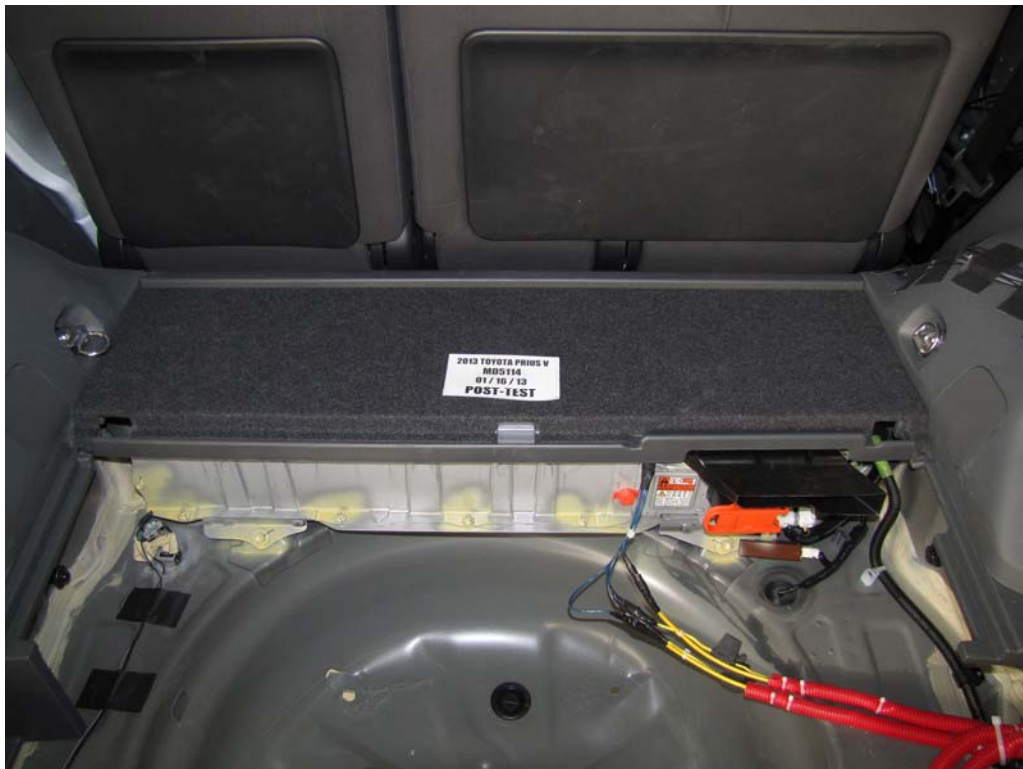
FIGURE 11. Post-Impact Rear View of Propulsion Battery
