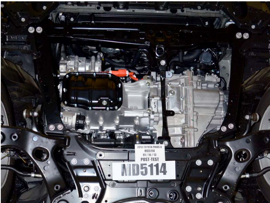
FIGURE 17a. Post-Impact View of Electric Propulsion Drive
