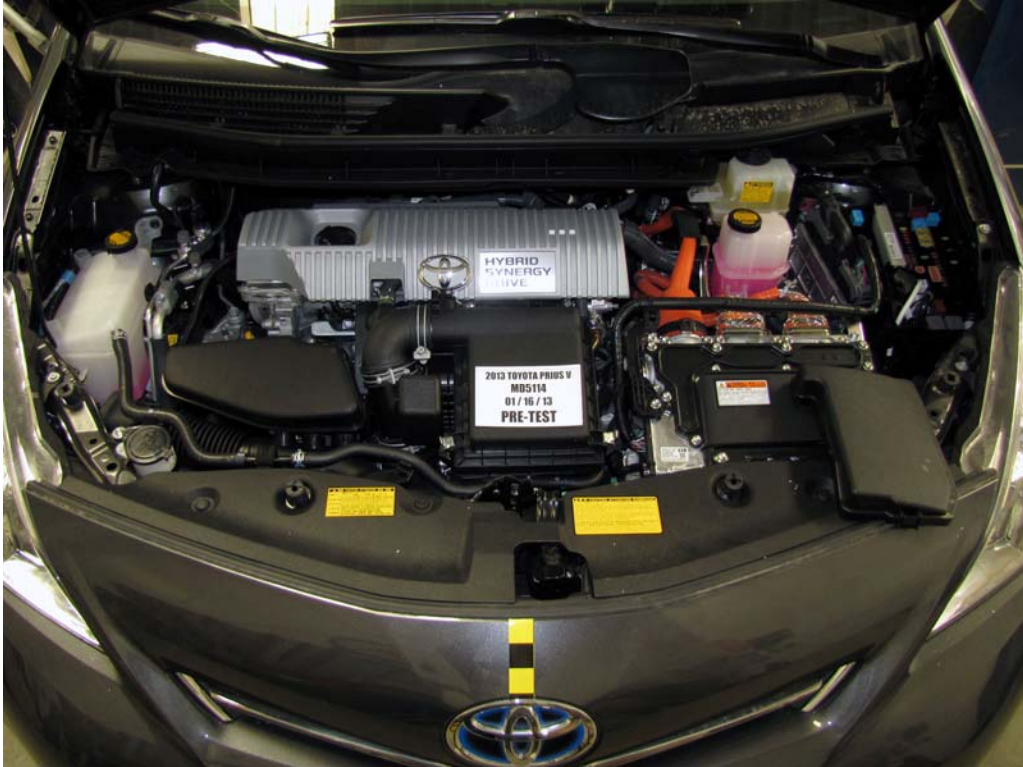
FIGURE 16. Pre-Impact View of Electric Propulsion Drive
