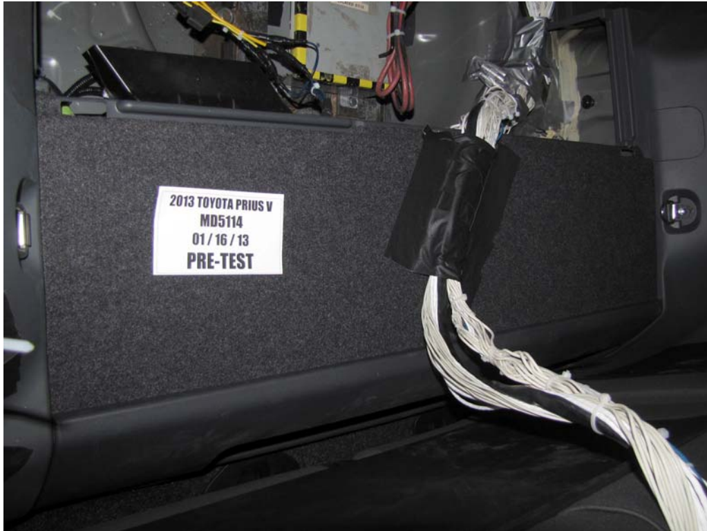
FIGURE 9. Pre-Impact View of Propulsion Battery
