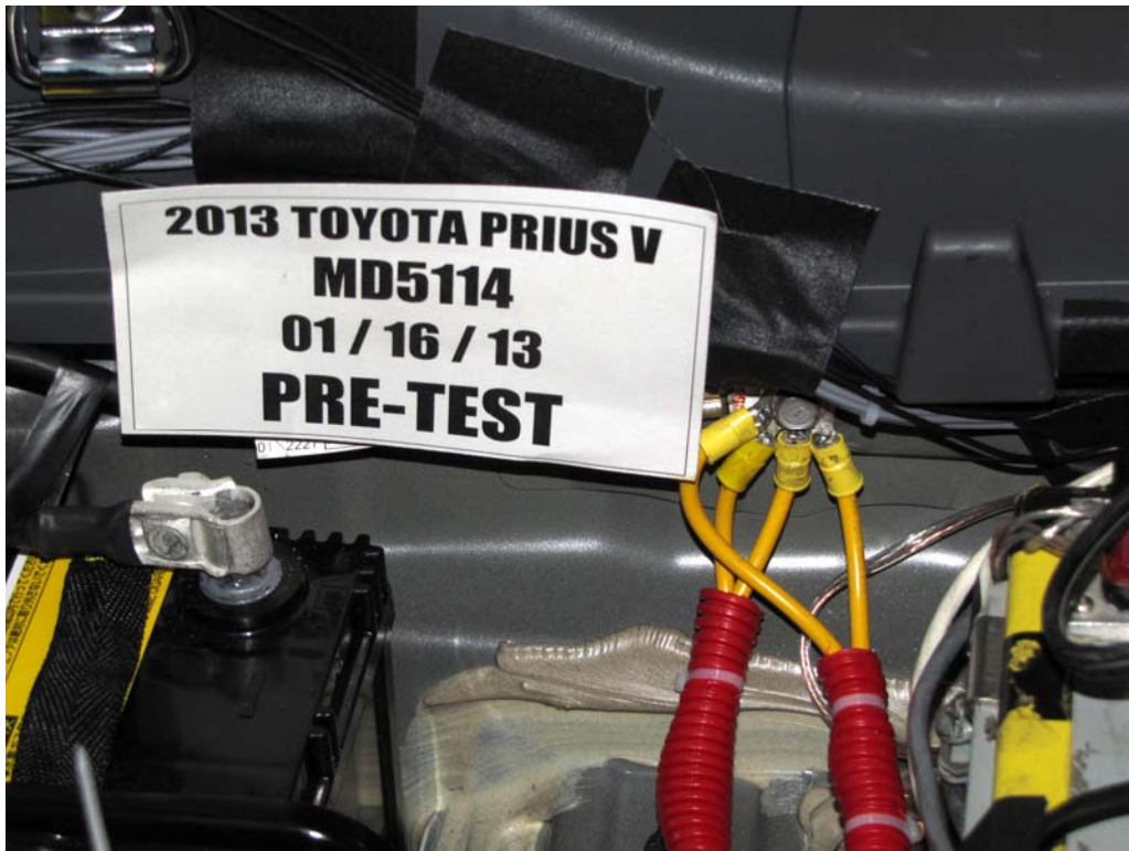
FIGURE 21. Pre-Impact View of Ground Lead Attached
