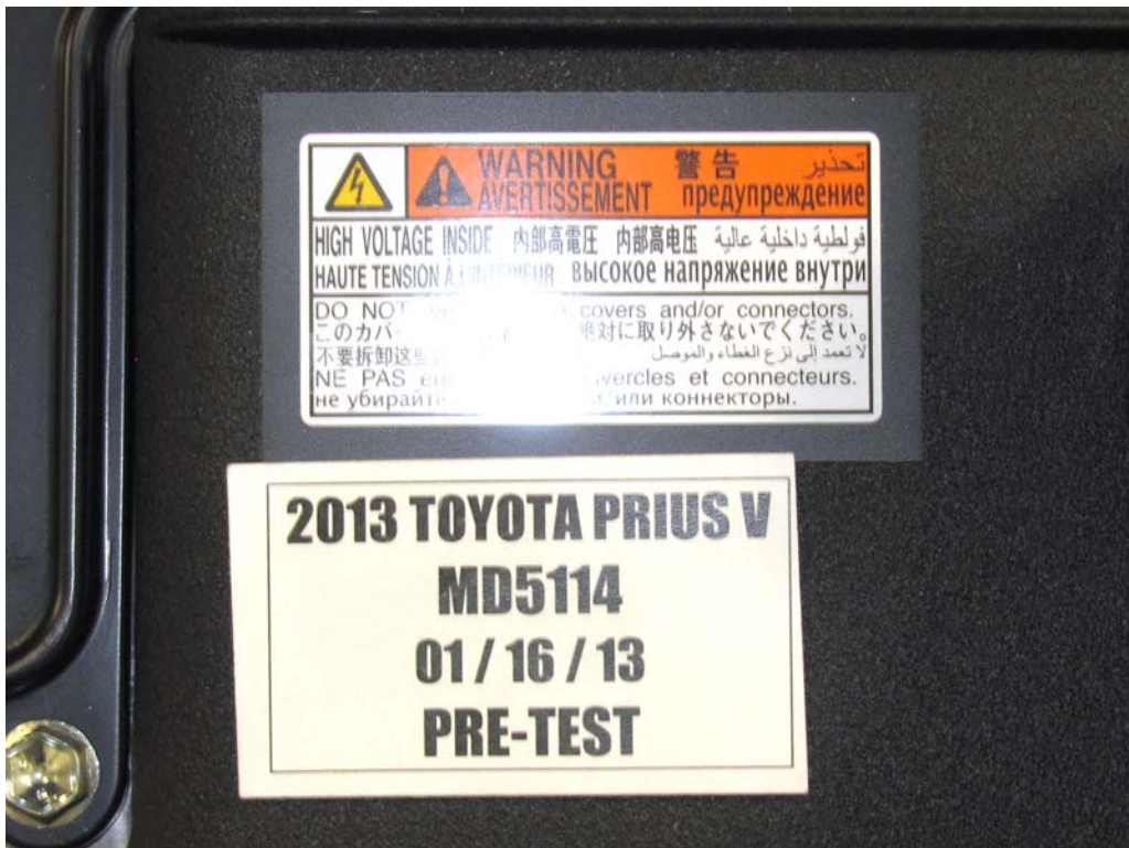
FIGURE 2. Power Inverter Warning Label
