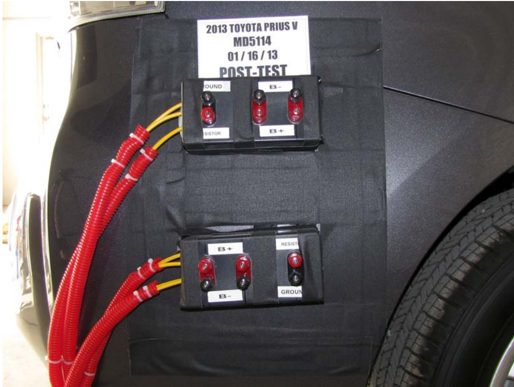
FIGURE 25. Post-Impact View of Installed Test Interface Port
