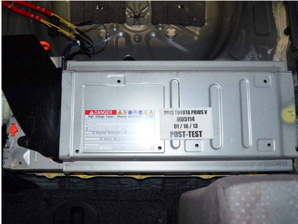
FIGURE 10. Post-Impact Front View of Propulsion Battery
