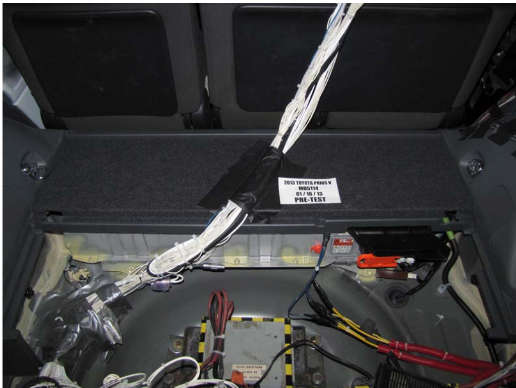
FIGURE 9a. Pre-Impact View of Propulsion Battery
