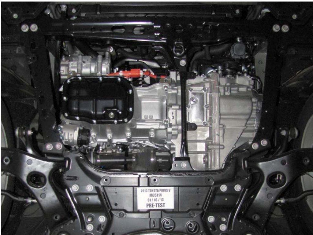
FIGURE 16a. Pre-Impact View of Electric Propulsion Drive
