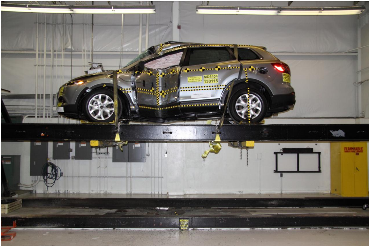
067 FMVSS No. 301 Static Rollover 360 Degrees
