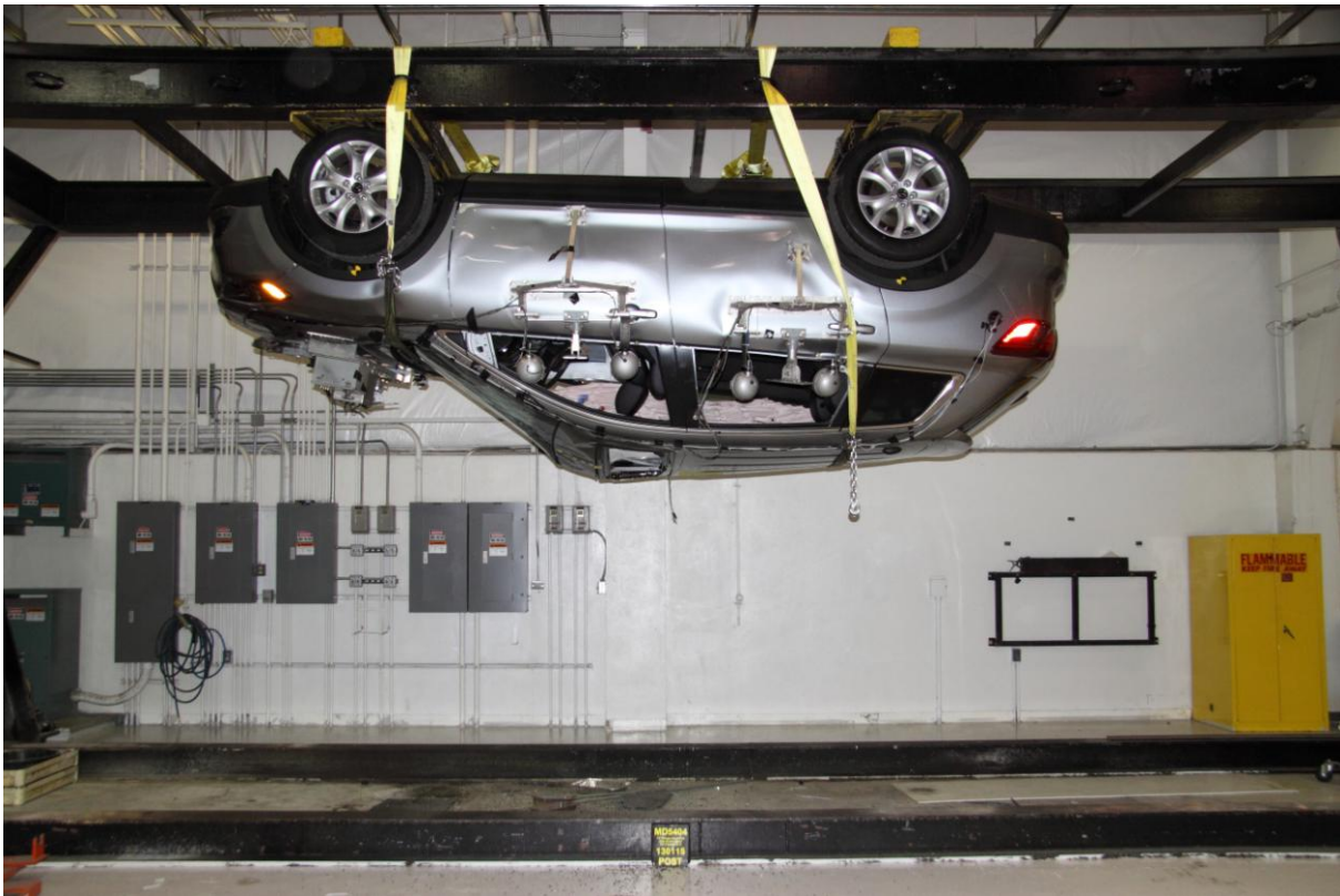
065 FMVSS No. 301 Static Rollover 180 Degrees
