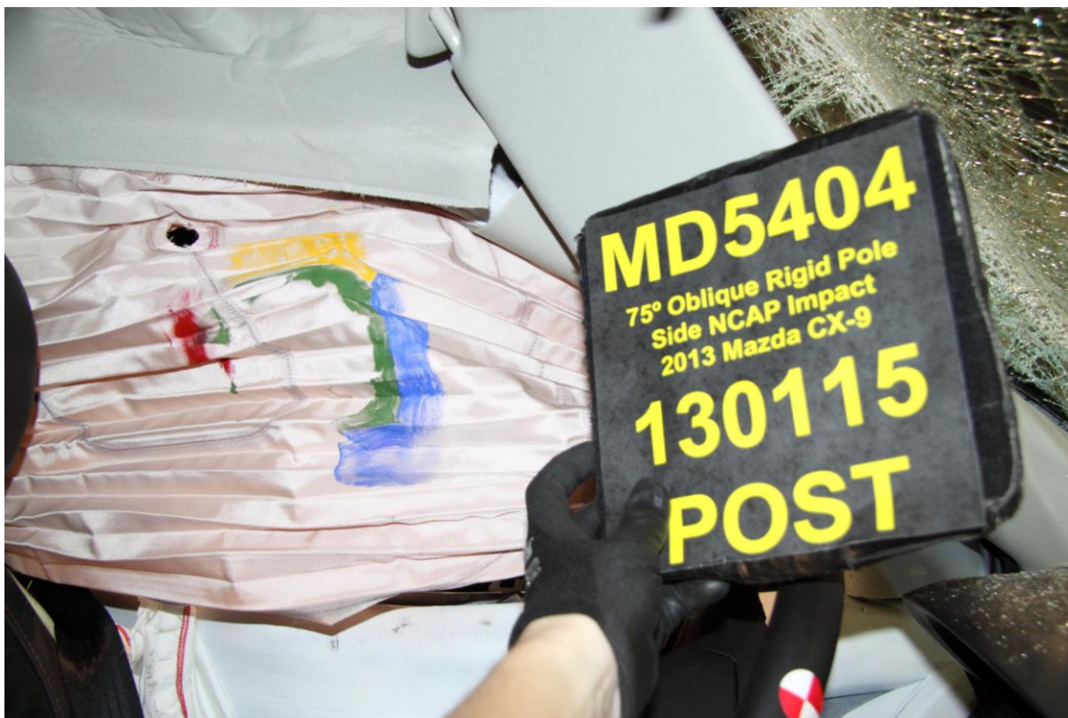
047 Post-Test Dummy Close-Up Head Contact with Side Airbag View
