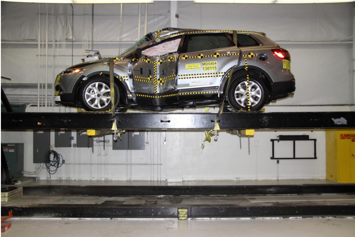
063 FMVSS No. 301 Static Rollover 0 Degrees
