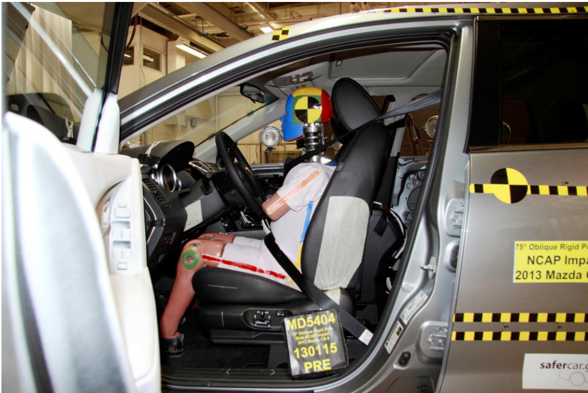
023 Pre-Test Left Side View of Dummy Showing Belt and Chalking
