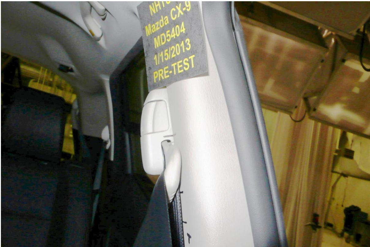
033 Pre-Test View of Belt Anchorage for Dummy
