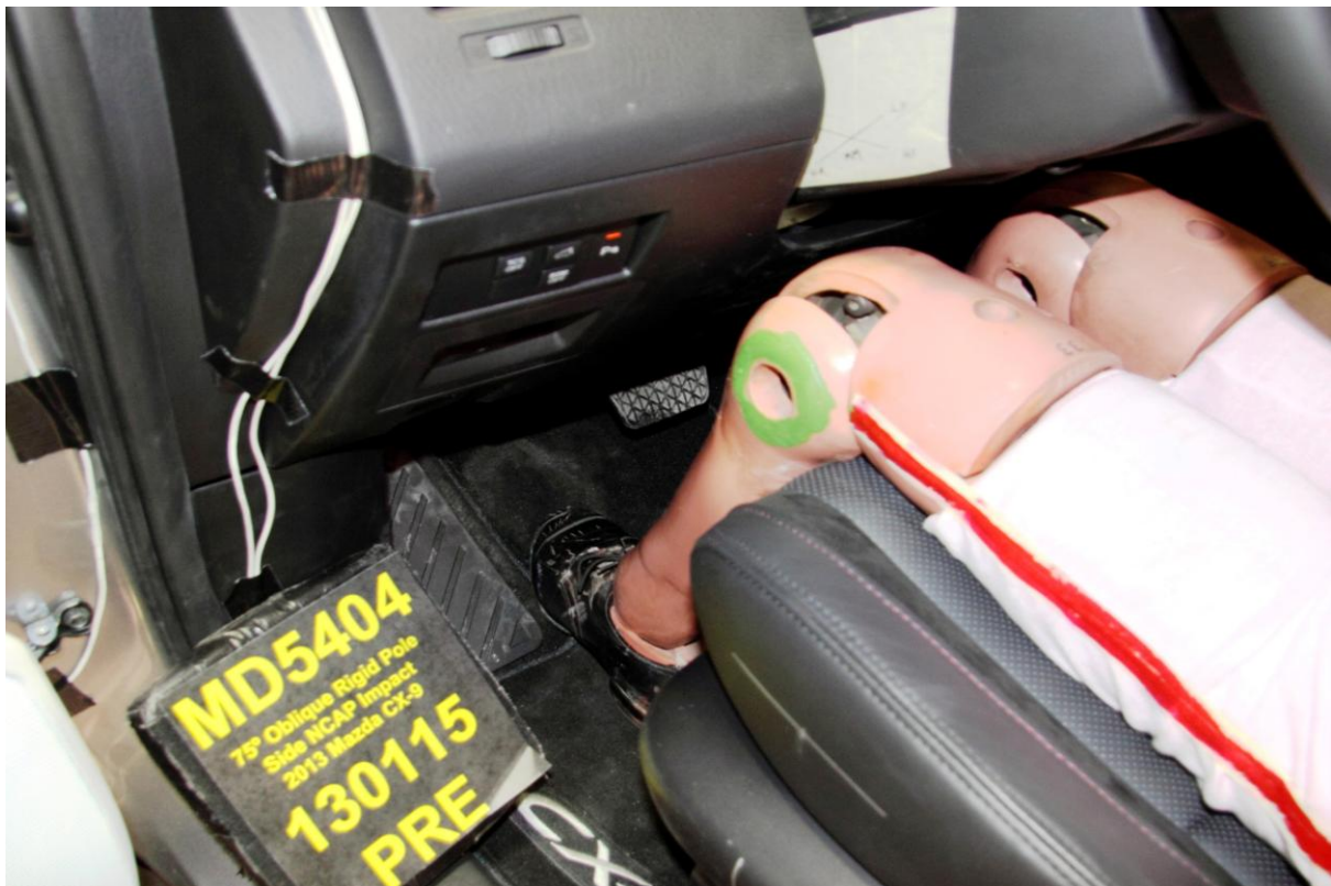
032 Pre-Test Placement of Dummy Feet
