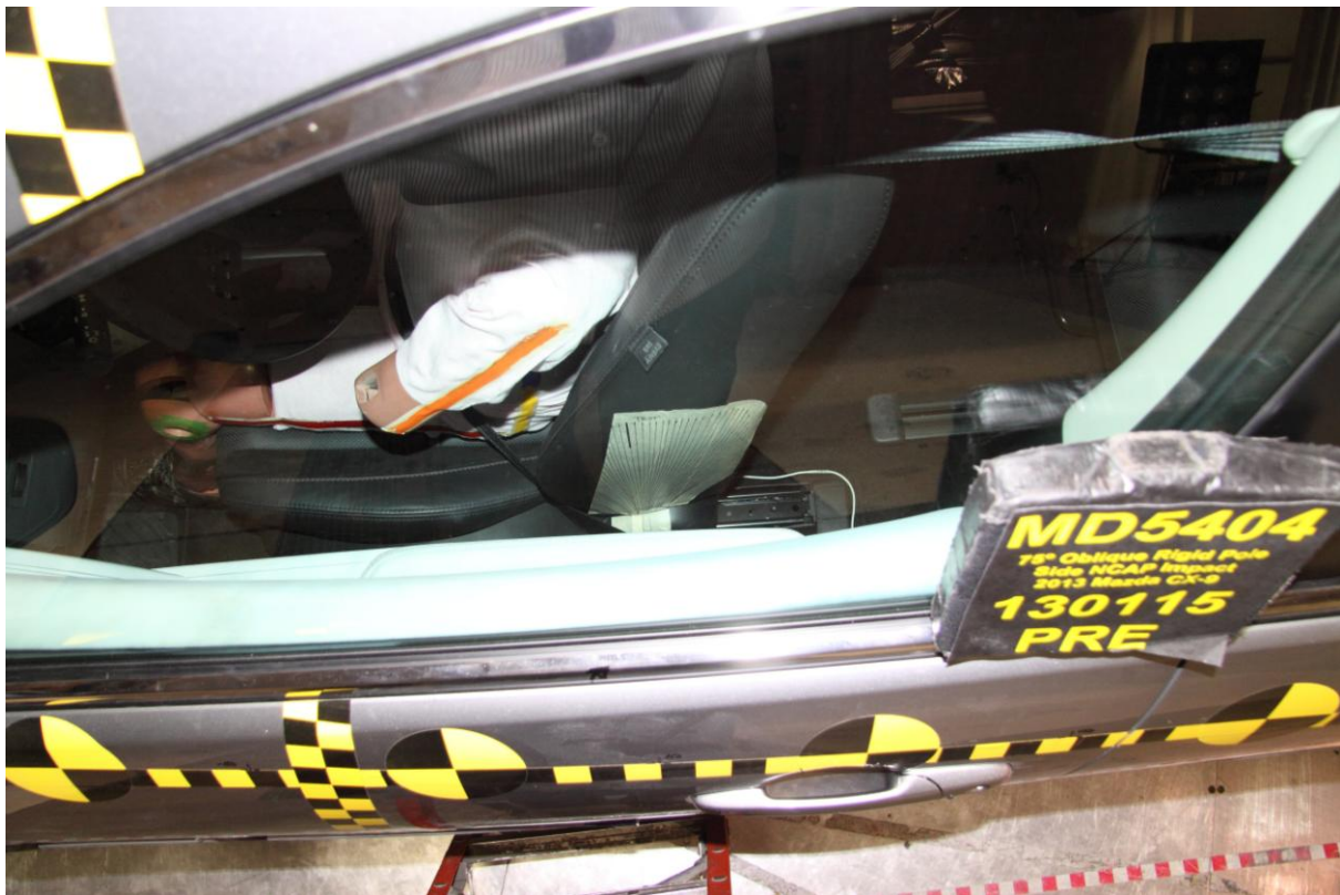
040 Pre-Test Dummy and Door Clearance View
