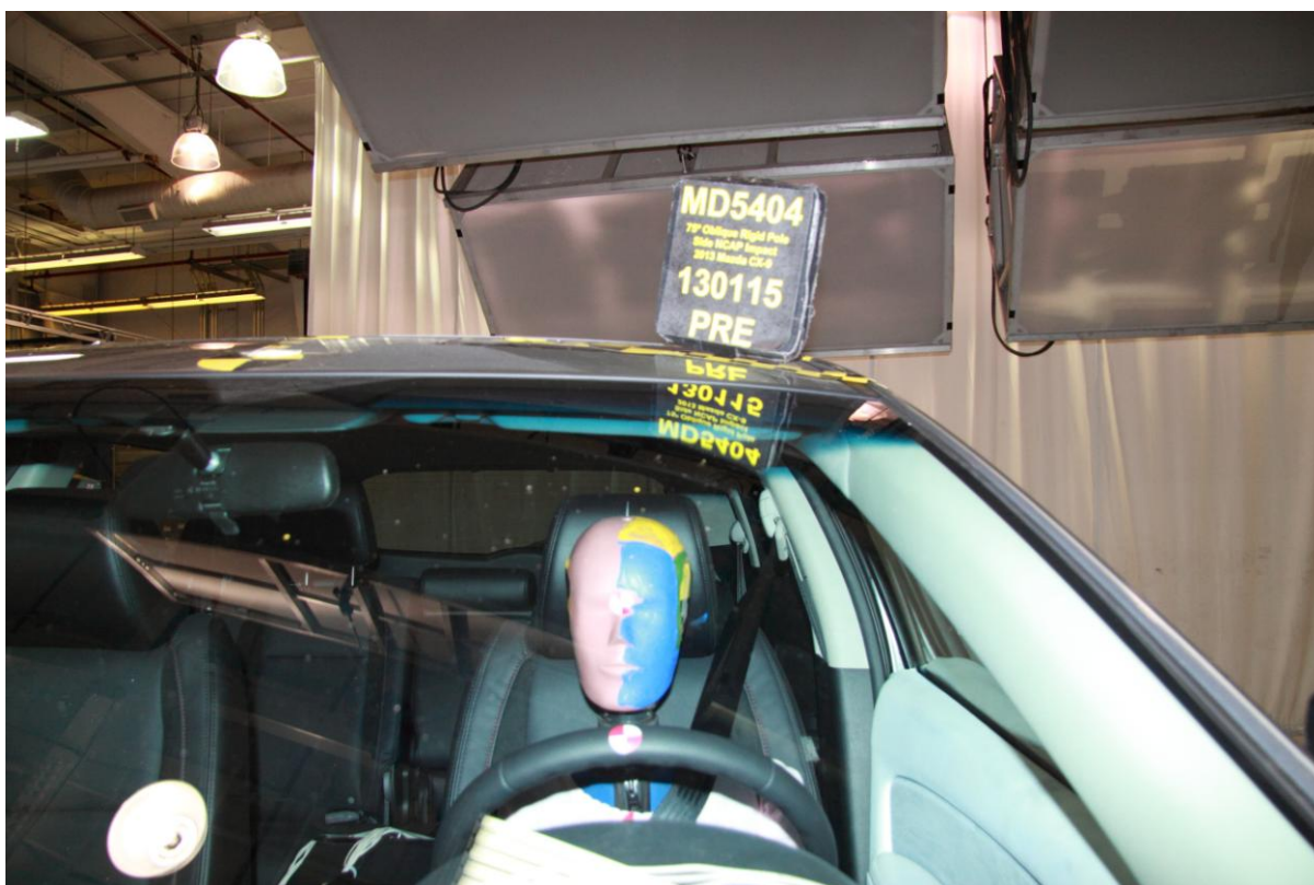
021 Pre-Test Front Close-Up View of Dummy Head and Chest
