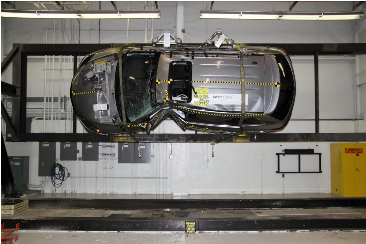
064 FMVSS No. 301 Static Rollover 90 Degrees
