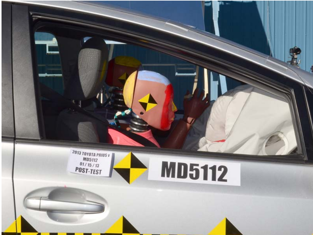
FIGURE 53. Post-Test Passenger Dummy Window View
