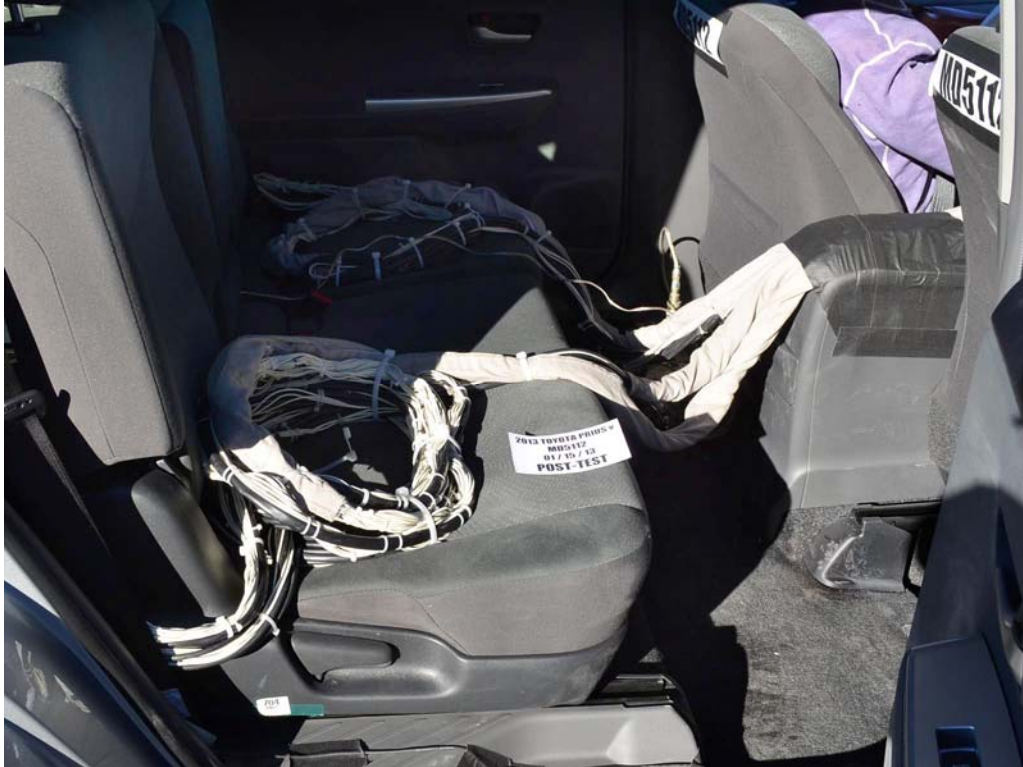
FIGURE 28. Post-Test Dummy Cable Routing
