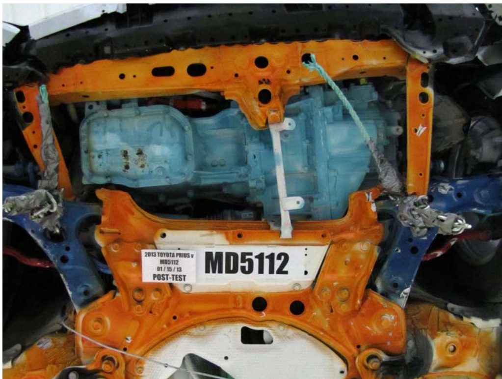
FIGURE 17a. Post-Impact View of Electric Propulsion Drive
