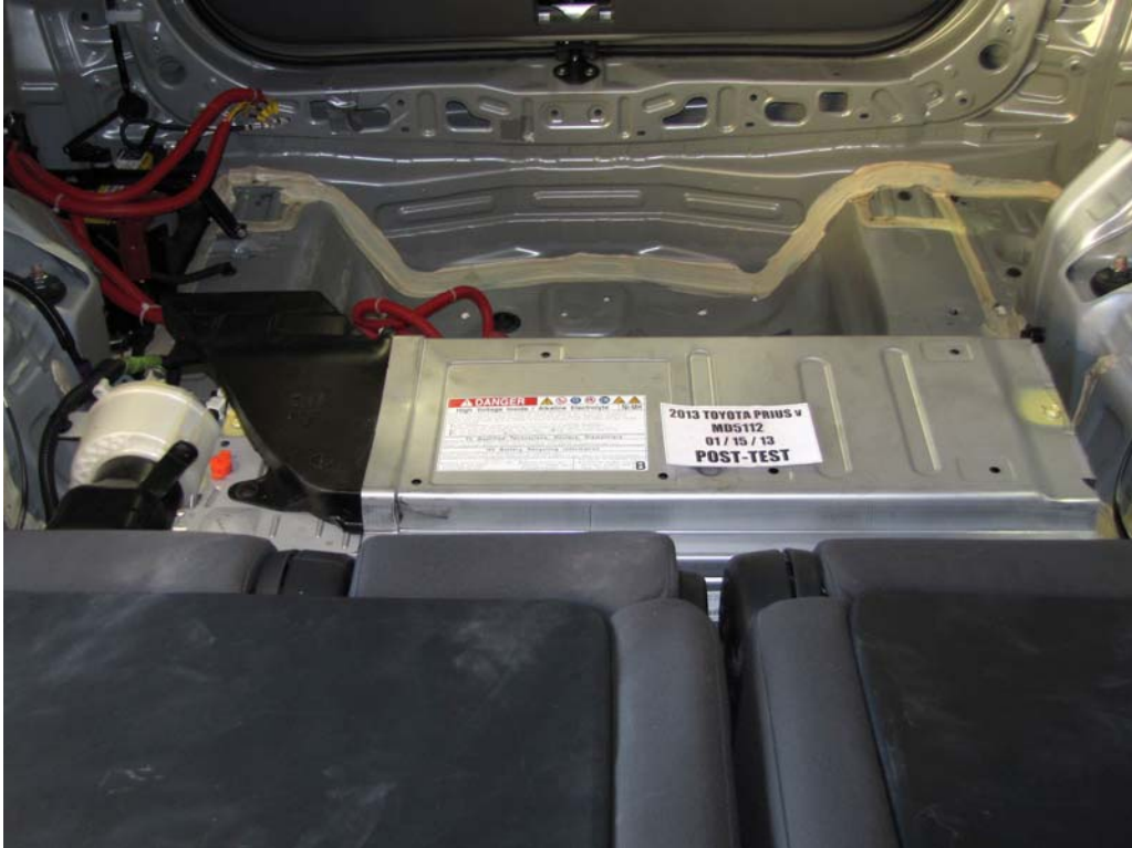
FIGURE 10. Post-Impact Front View of Propulsion Battery
