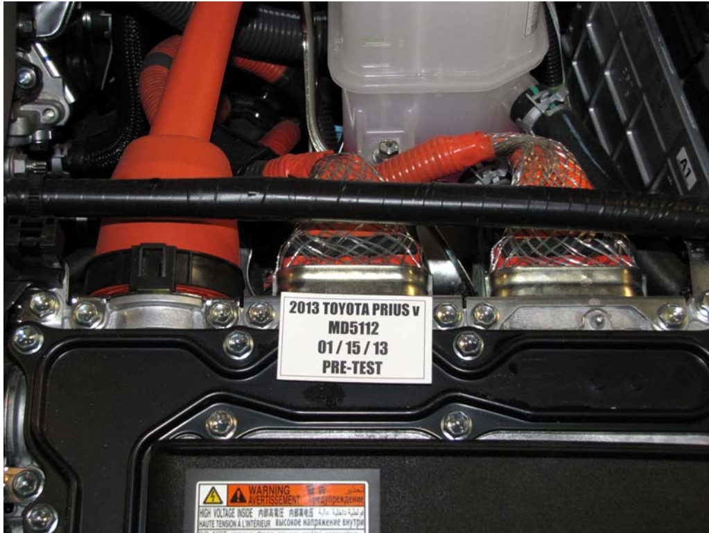
FIGURE 18b. Pre-Impact View of High Voltage Interconnect(s)
