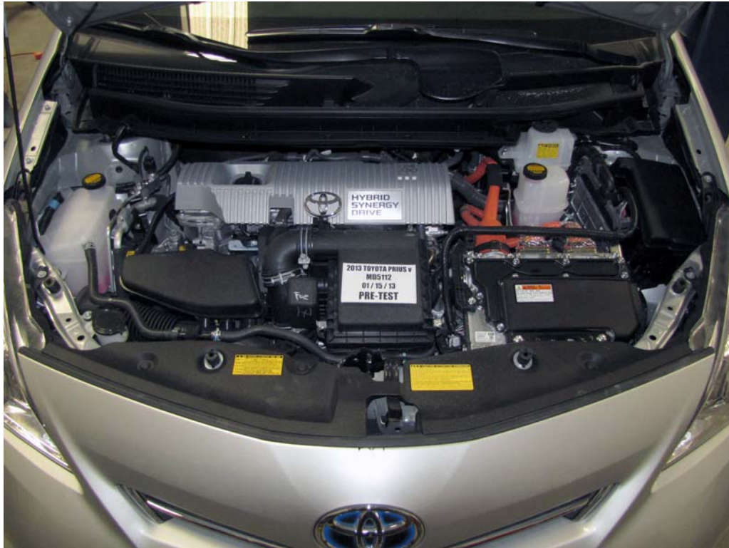
FIGURE 16. Pre-Impact View of Electric Propulsion Drive
