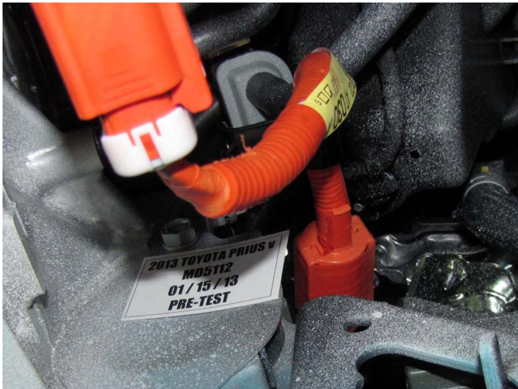
FIGURE 18a. Pre-Impact View of High Voltage Interconnect(s)
