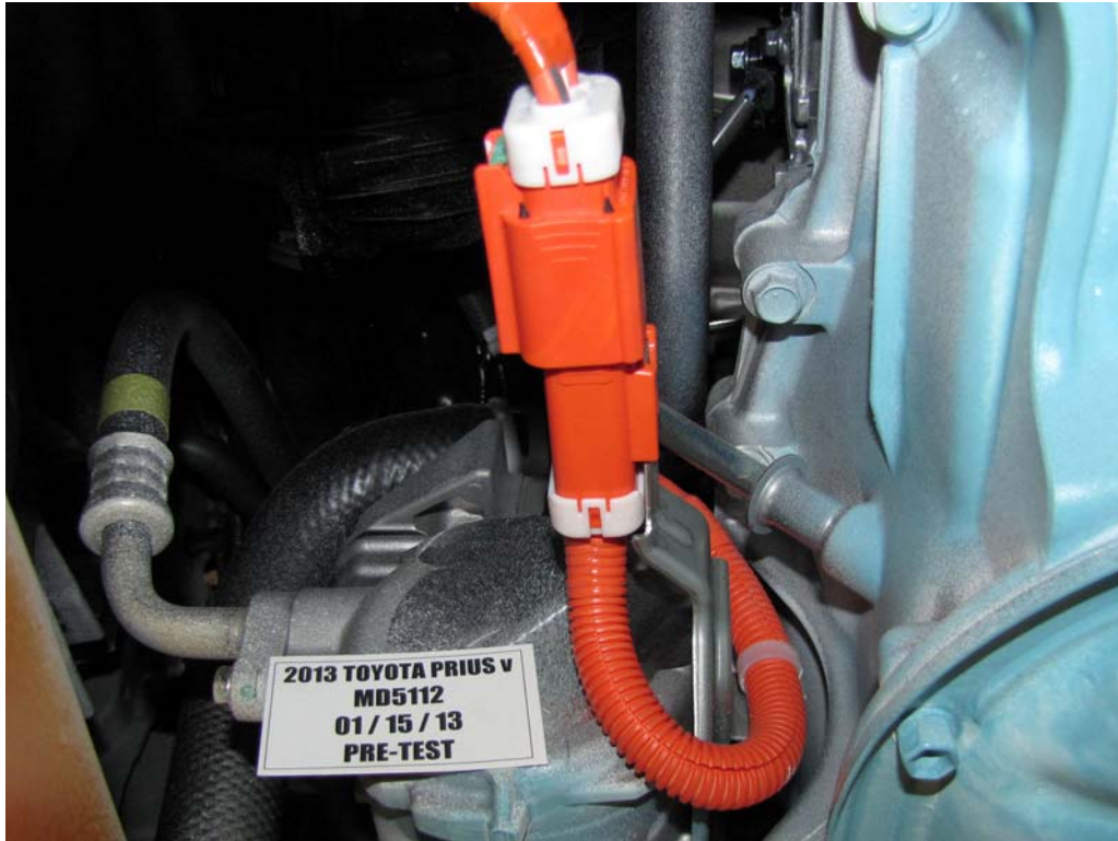
FIGURE 18. Pre-Impact View of High Voltage Interconnect(s)
