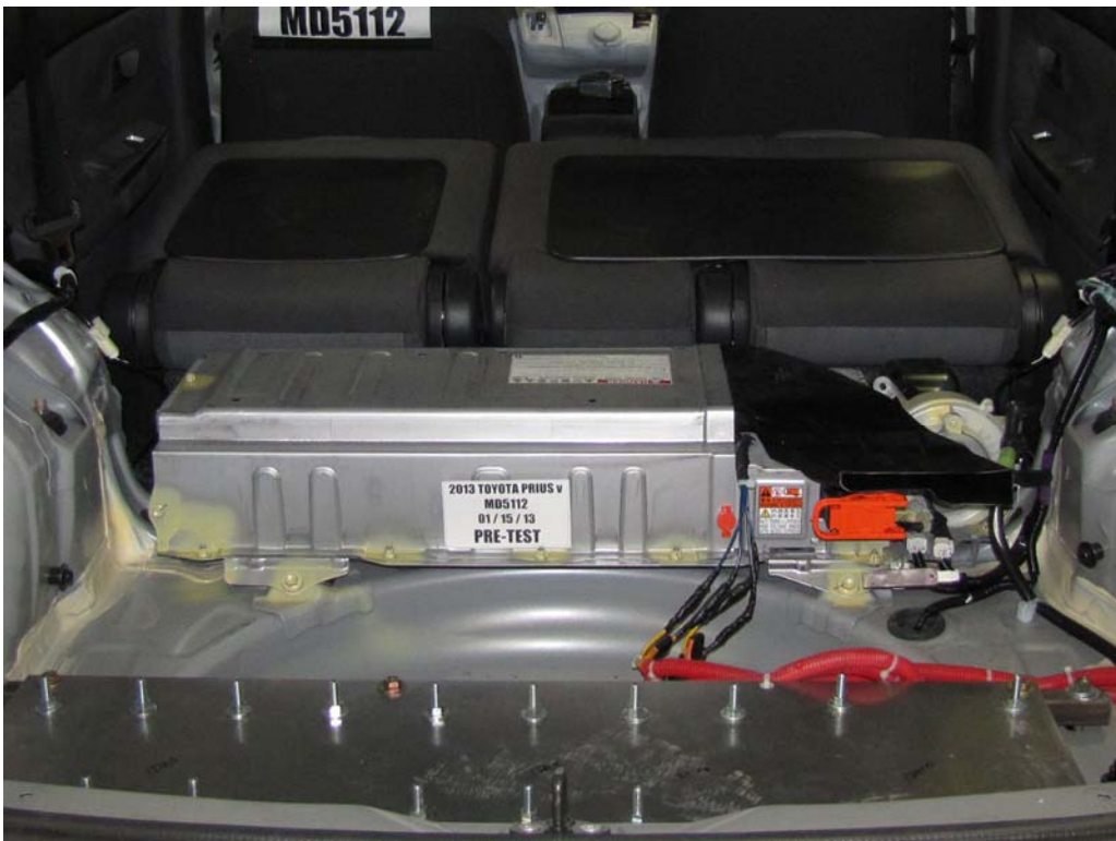
FIGURE 9a. Pre-Impact View of Propulsion Battery
