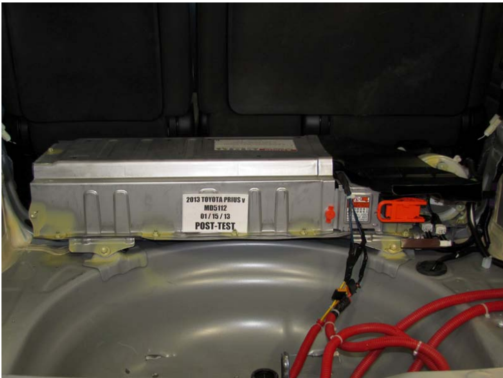
FIGURE 11. Post-Impact Rear View of Propulsion Battery
