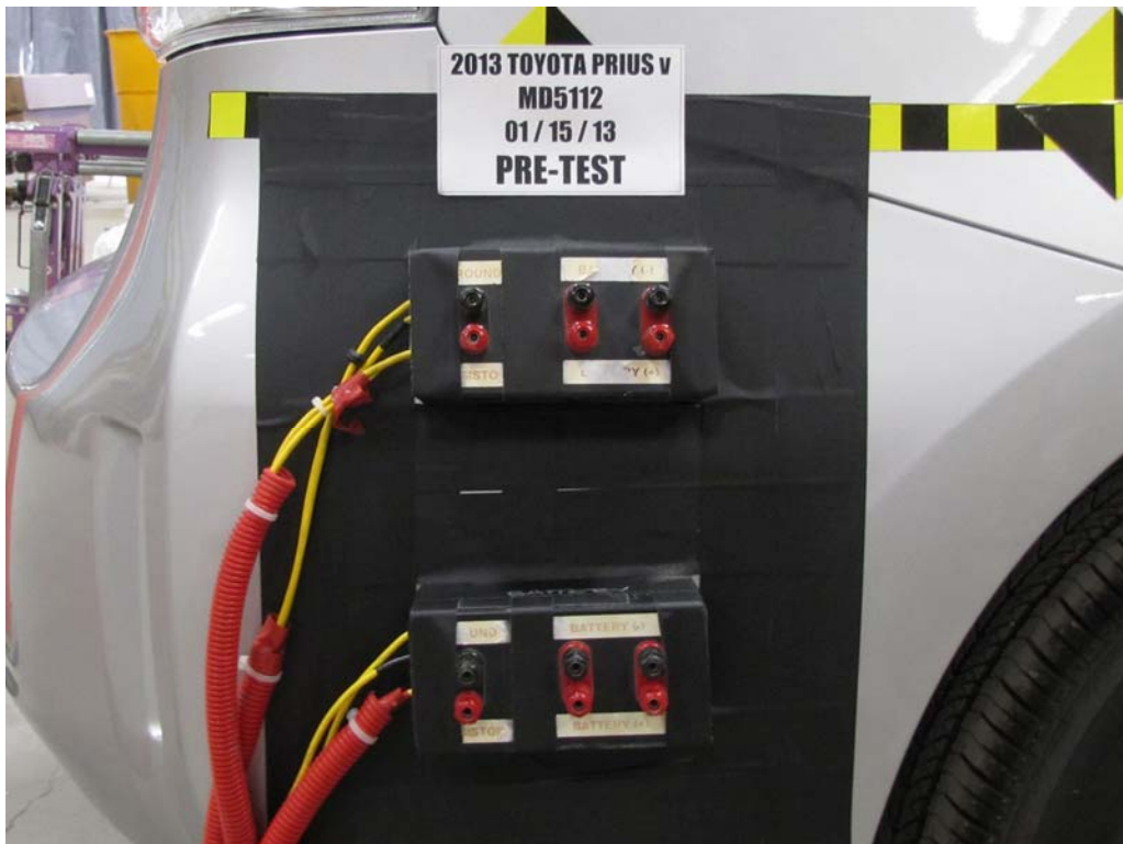
FIGURE 24. Pre-Impact View of Installed Test Interface Port
