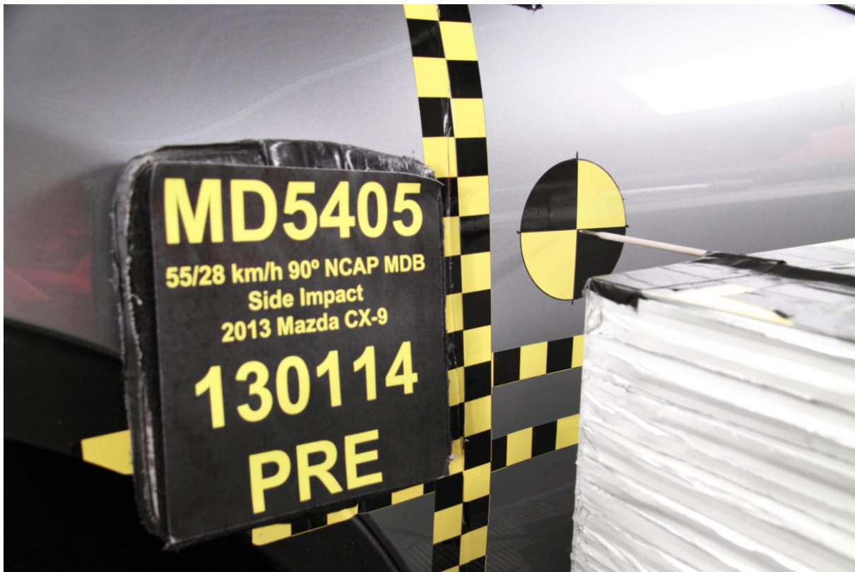
019 Pre-Test Close-up View of Impact Point Target
