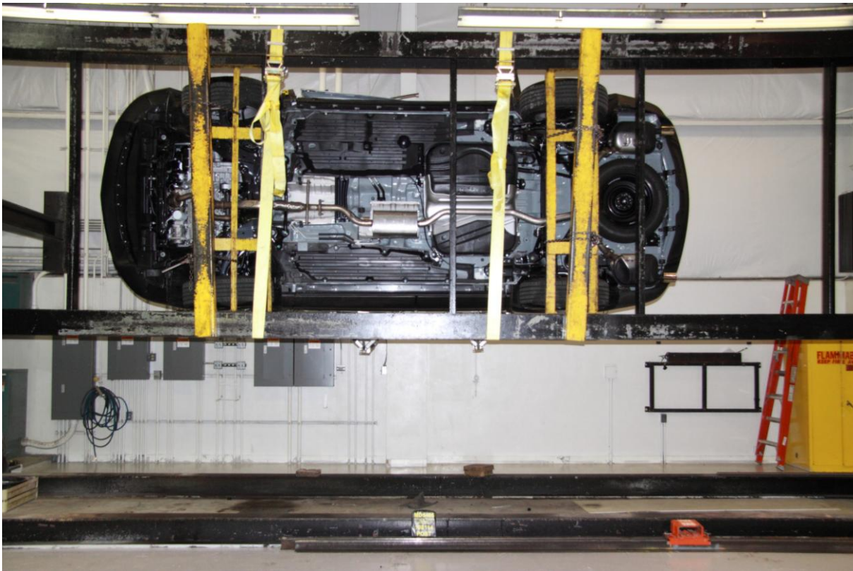
099 FMVSS No. 301 Static Rollover 270 Degrees
