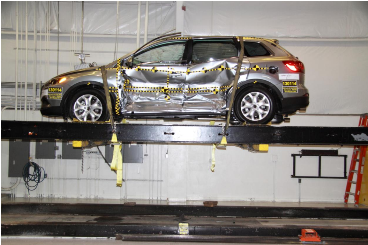
100 FMVSS No. 301 Static Rollover 360 Degrees
