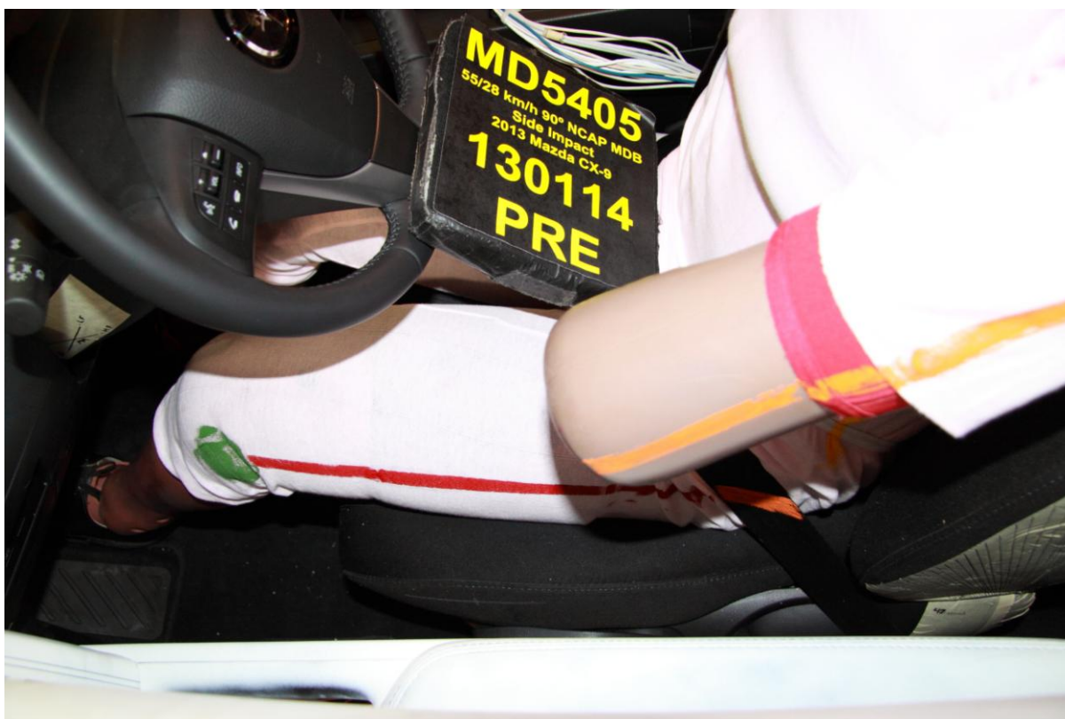
042 Pre-Test Driver Dummy and Door Clearance View
