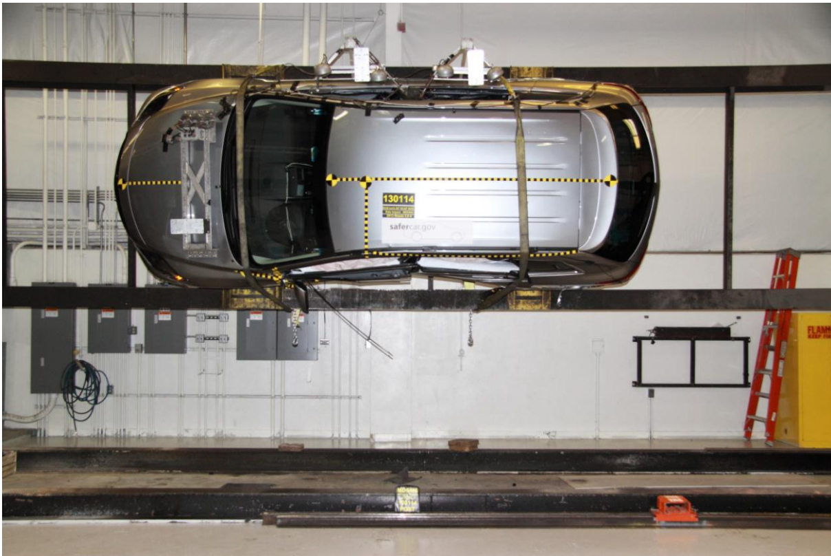
097 FMVSS No. 301 Static Rollover 90 Degrees
