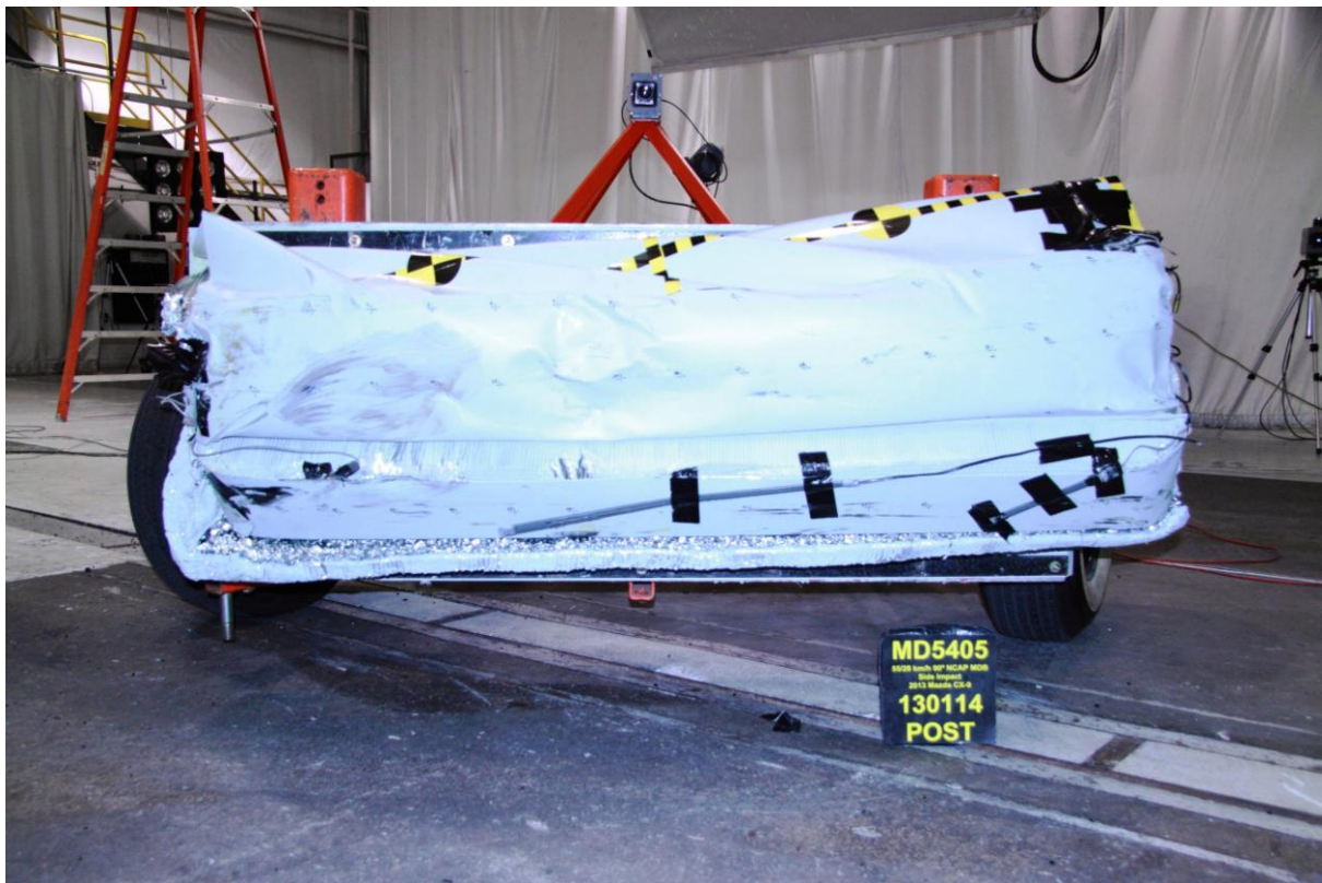
085 Post-Test Front View of MDB Impactor Face
