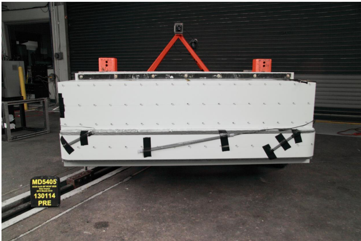
084 Pre-Test Front View of MDB Impactor Face
