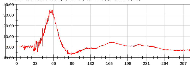
Driver Head Acceleration (Z) Primary vs. Time (g) vs. Time [ms]
