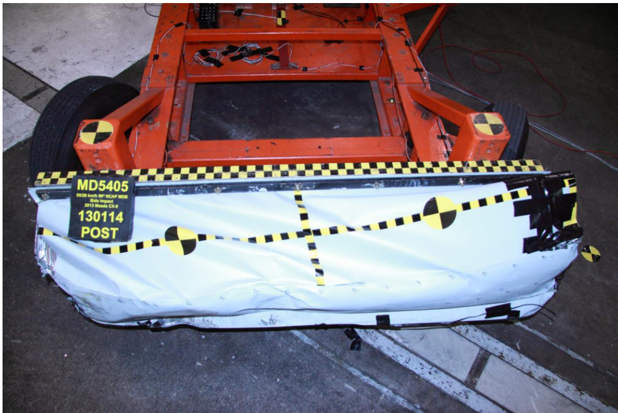
087 Post-Test Top View of MDB Impactor Face
