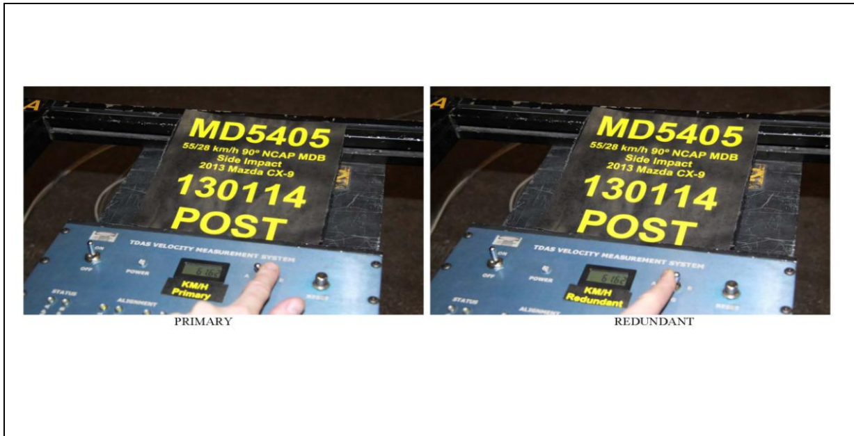
095 Post-Test Primary and Redundant Speed Trap Read-Out
