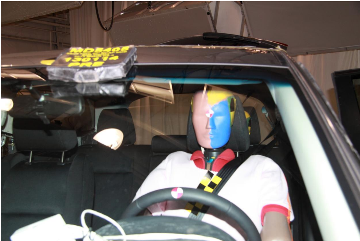
025 Pre-Test Front Close-up View of Driver Dummy
