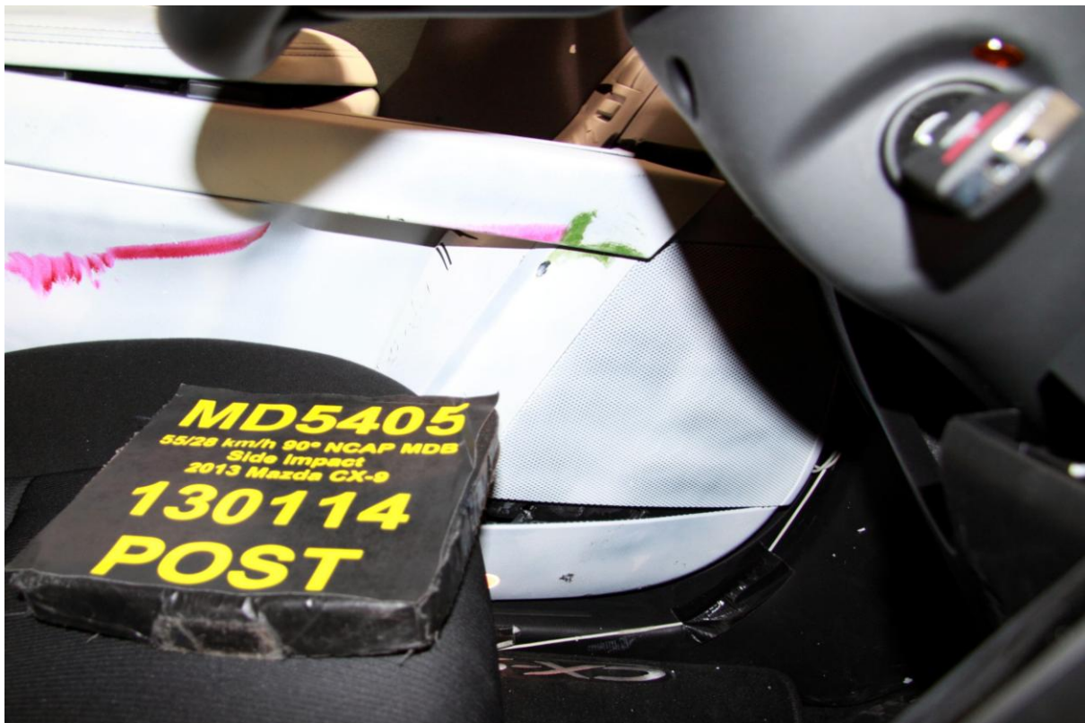
054 Post-Test Driver Dummy Close-Up Knee Contact View
