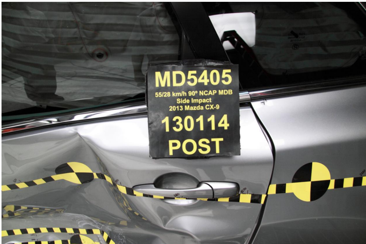
024 Post-Test Left Rear Door Latch Close-up
