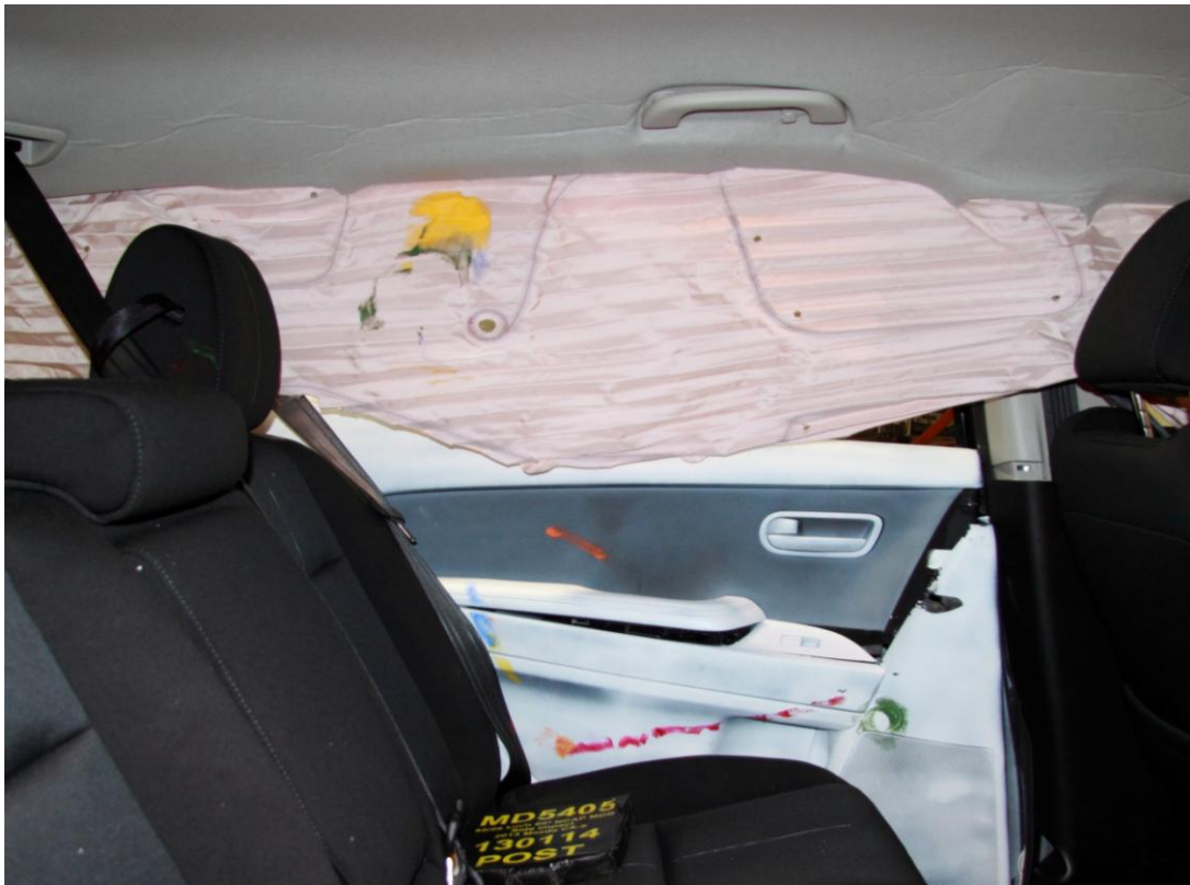
075 Post-Test Rear Passenger Dummy Close-Up Head Contact with Vehicle View
