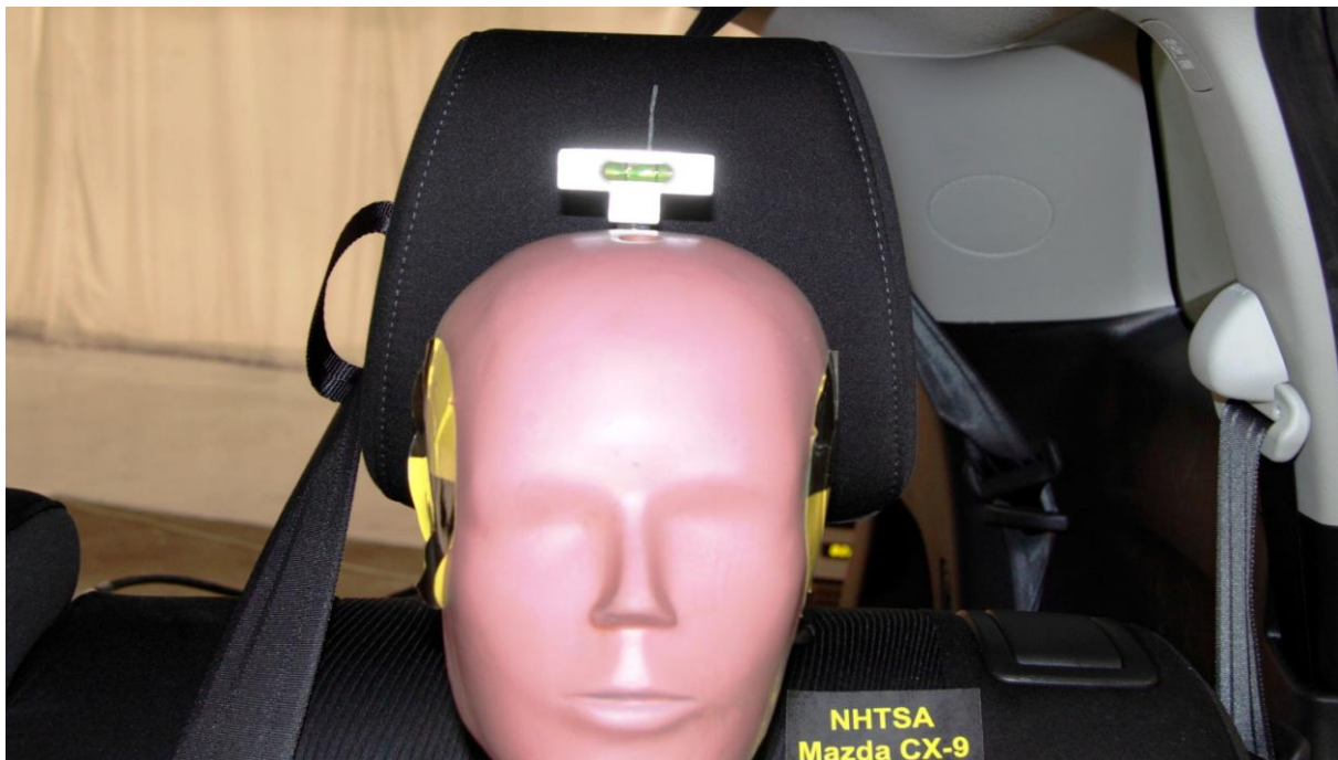
063 Pre-Test View of Rear Passenger Dummy Head Showing Dummy Head is Level
