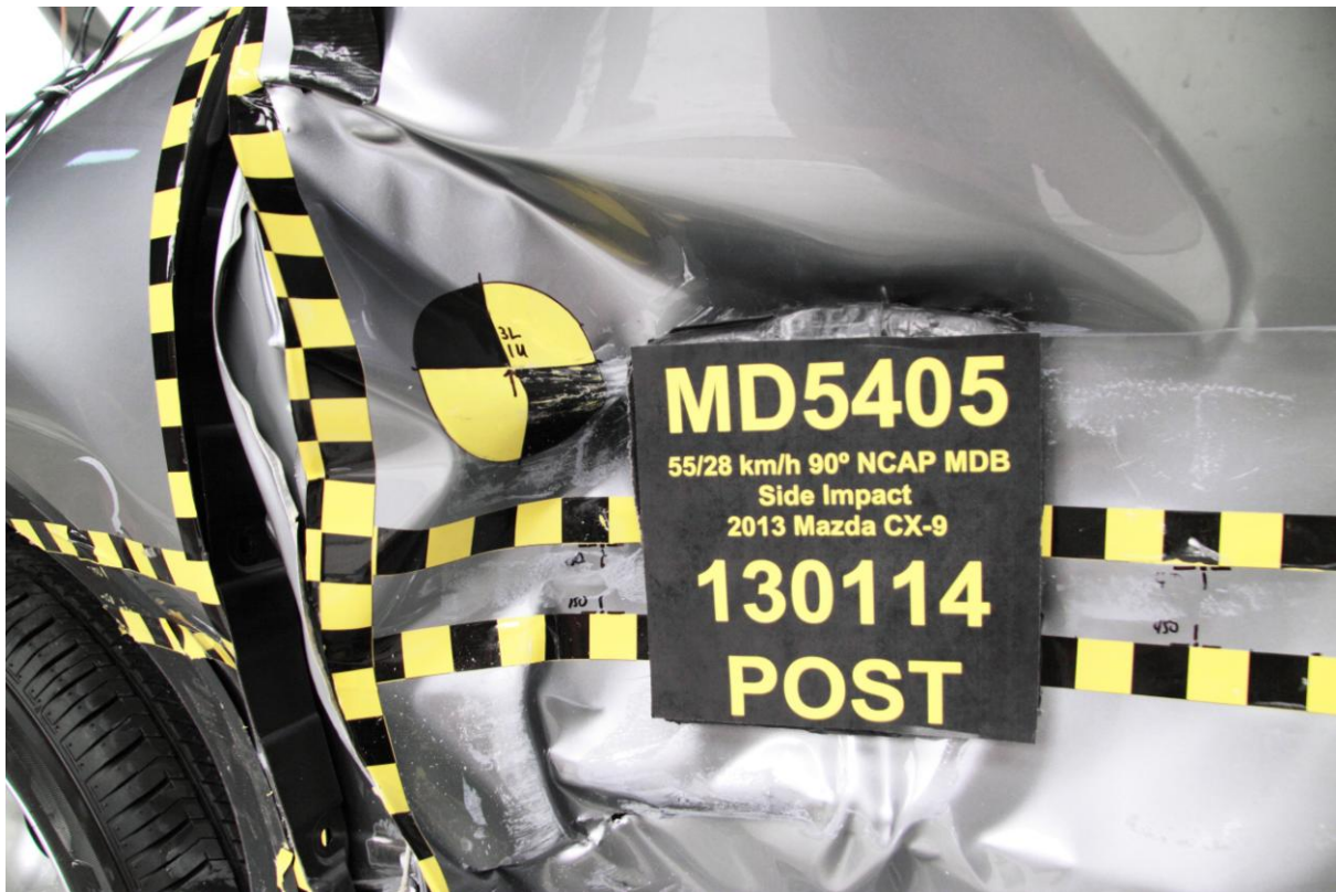
020 Post-Test Close-up View of Impact Point Target
