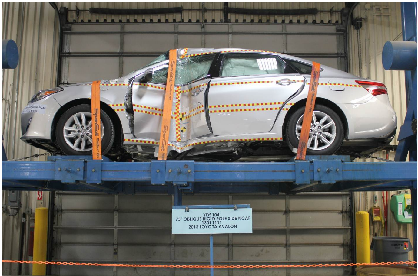
FMVSS No. 301 Static Rollover 0 Degrees
