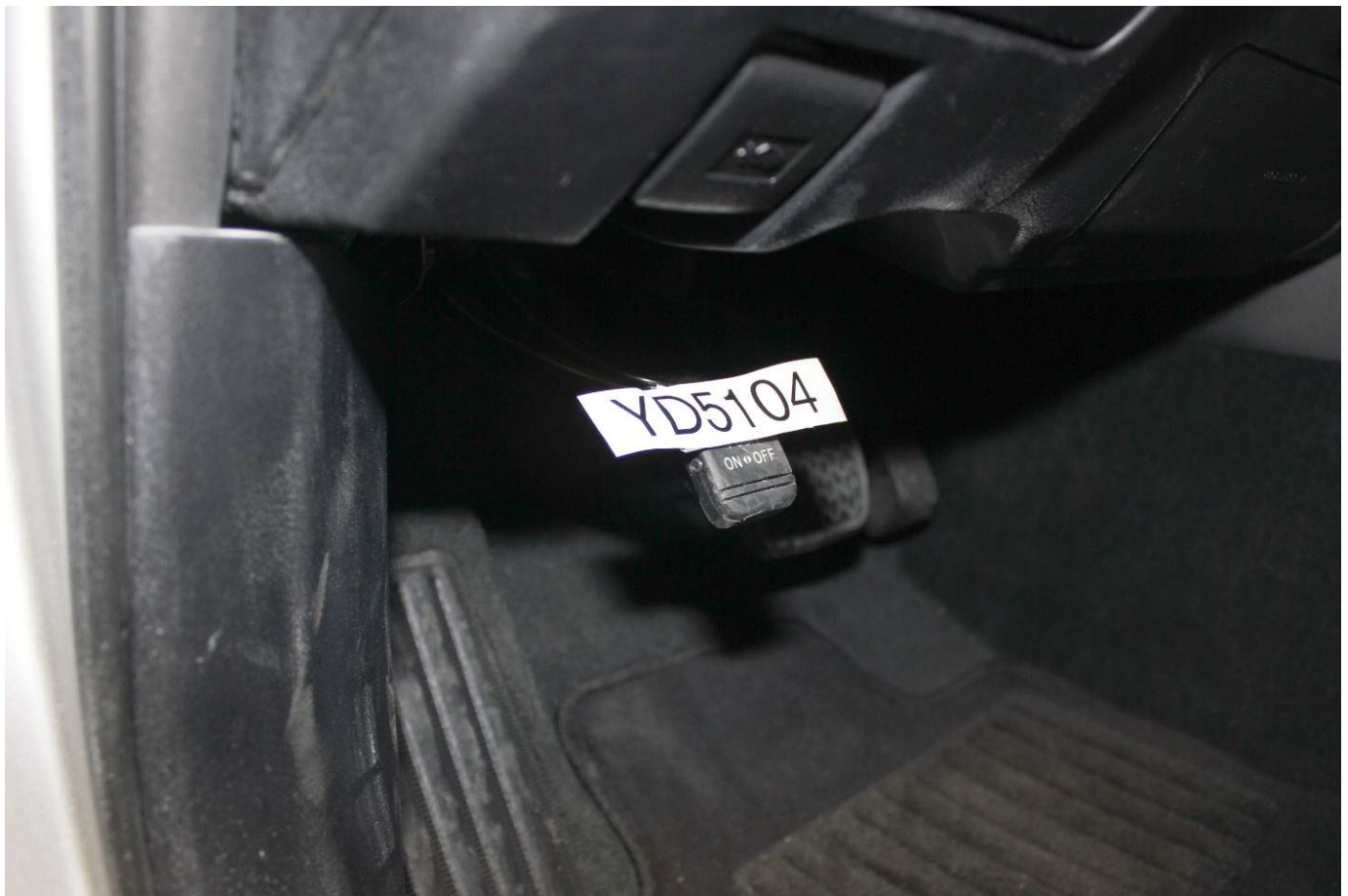
Pre-Test View of Disengaged Parking Brake
