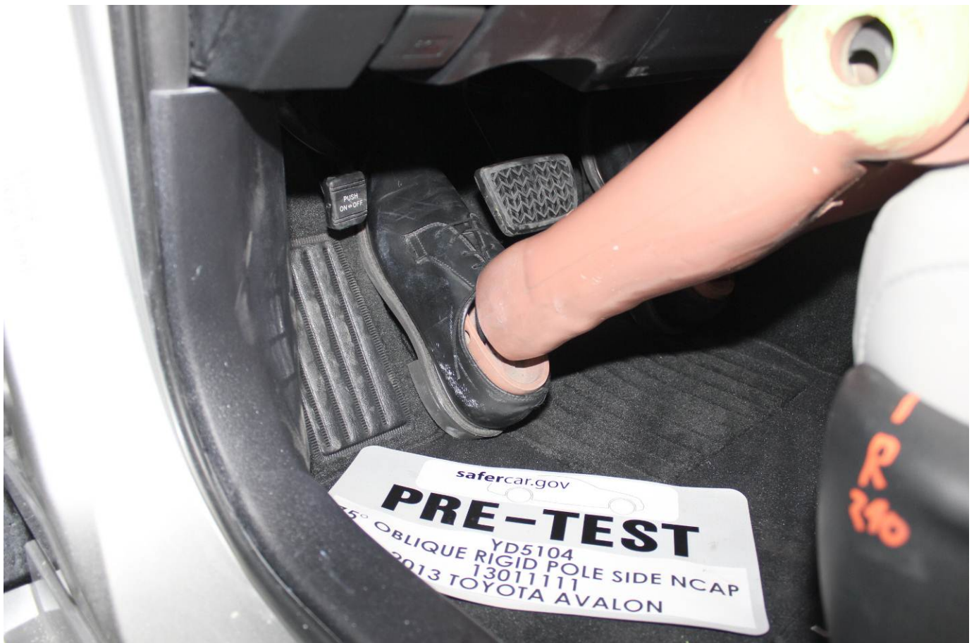
Pre-Test Placement of Dummy's Feet
