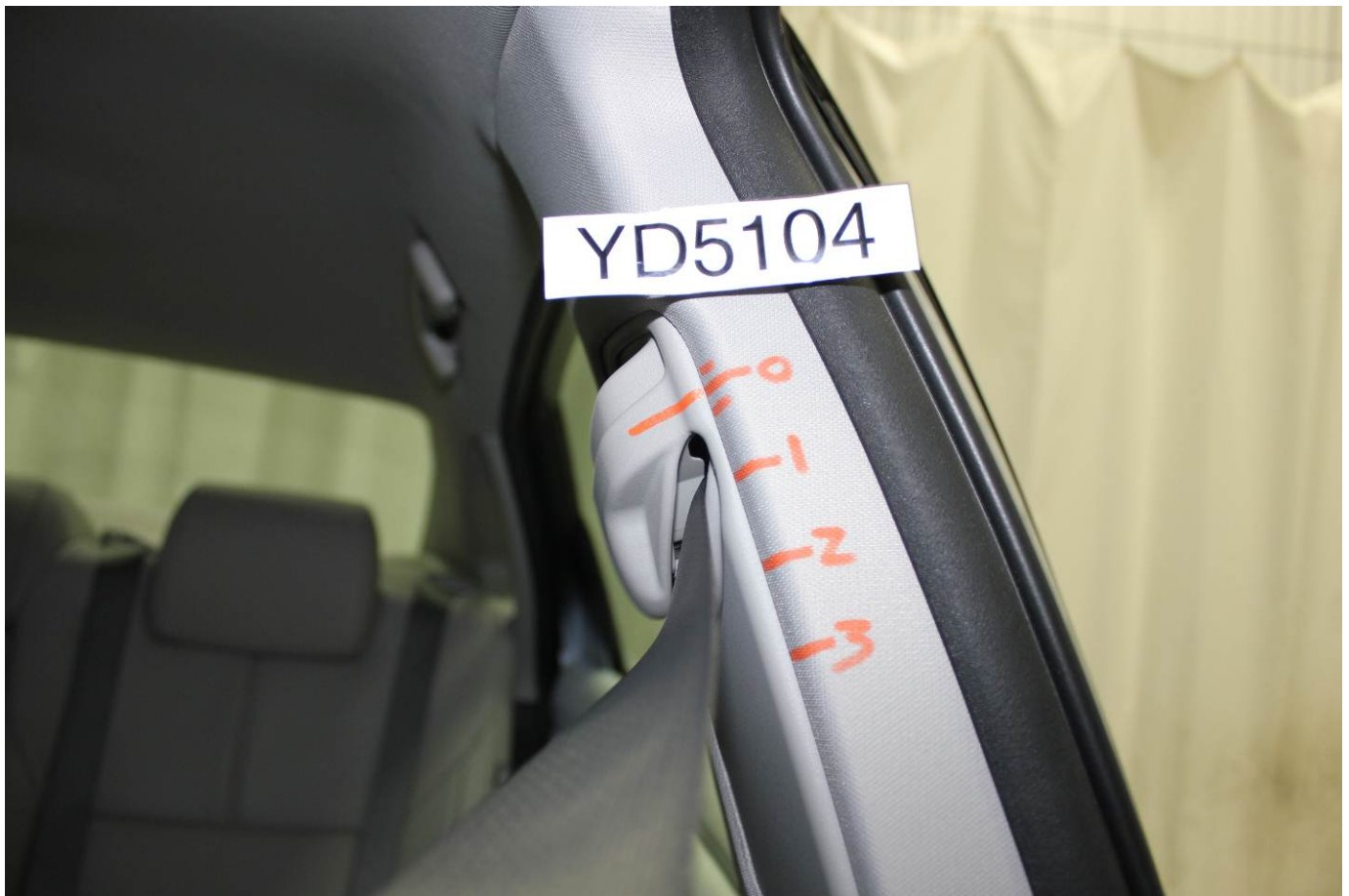
Pre-Test View of Belt Anchorage for Dummy
