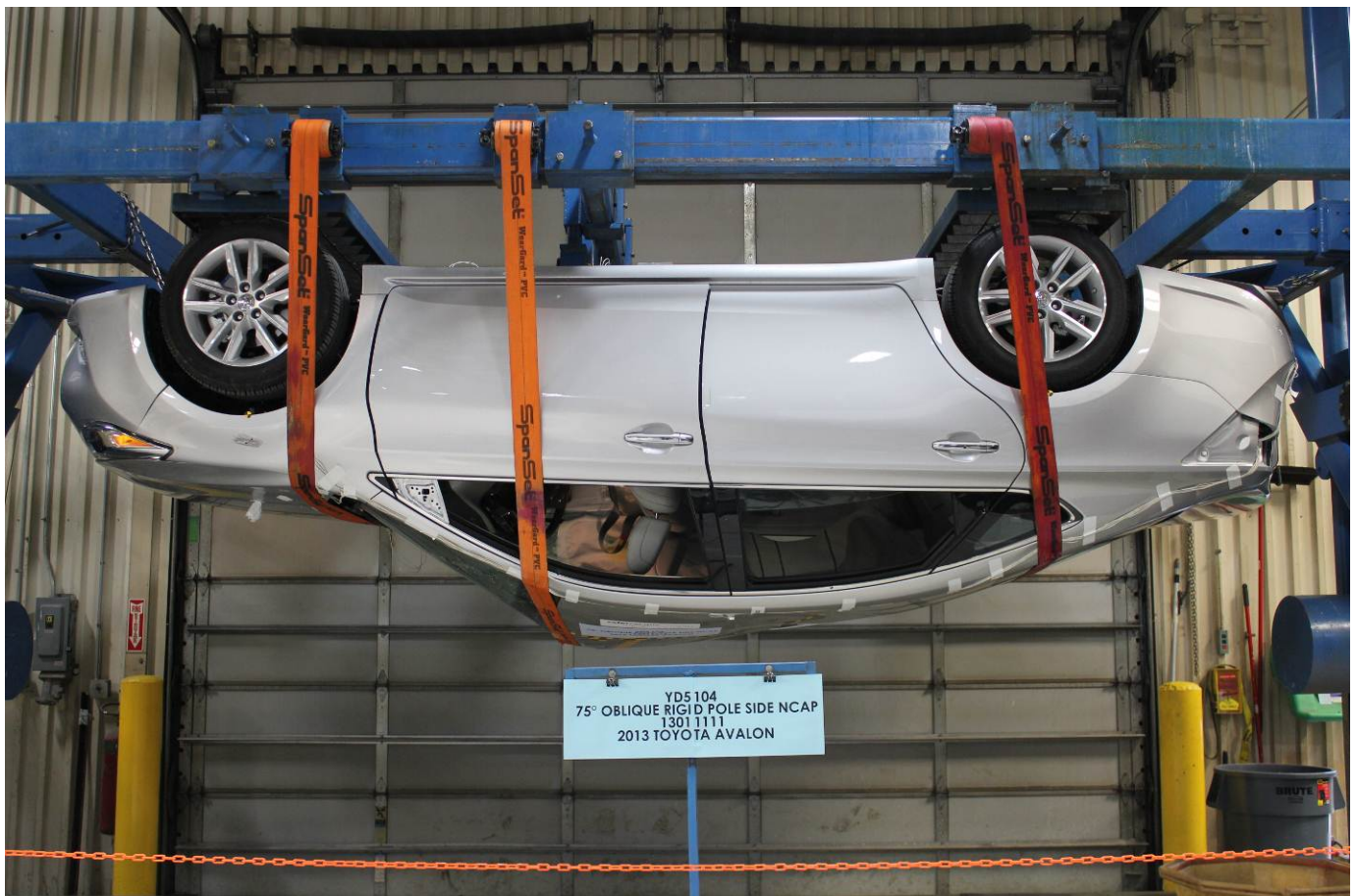
FMVSS No. 301 Static Rollover 180 Degrees
