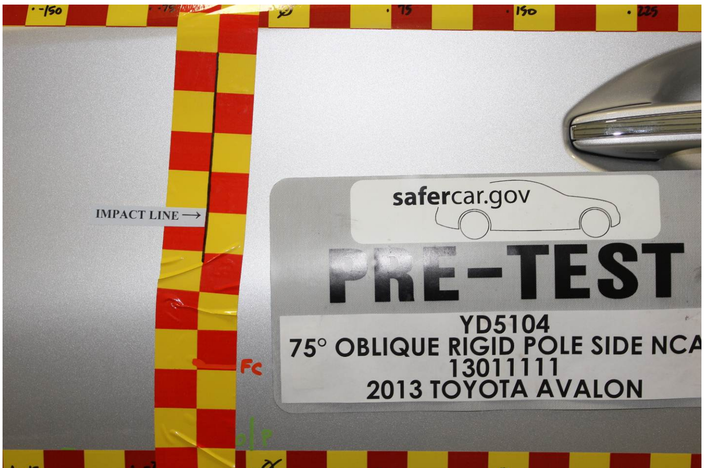
Pre-Test Close-Up View of Impact Point Target
