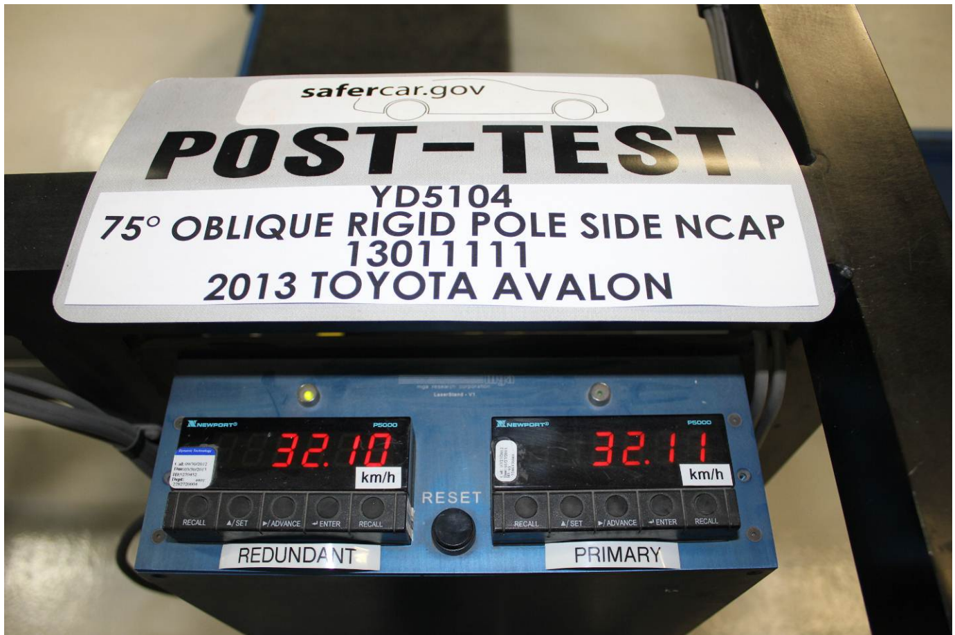
Post-Test Primary and Redundant Speed Trap Read-Out
