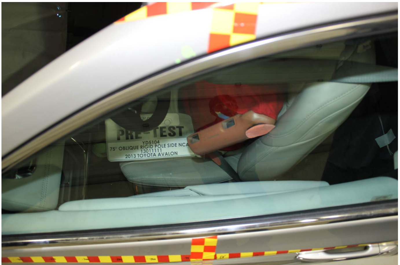
Pre-Test Dummy and Door Clearance View
