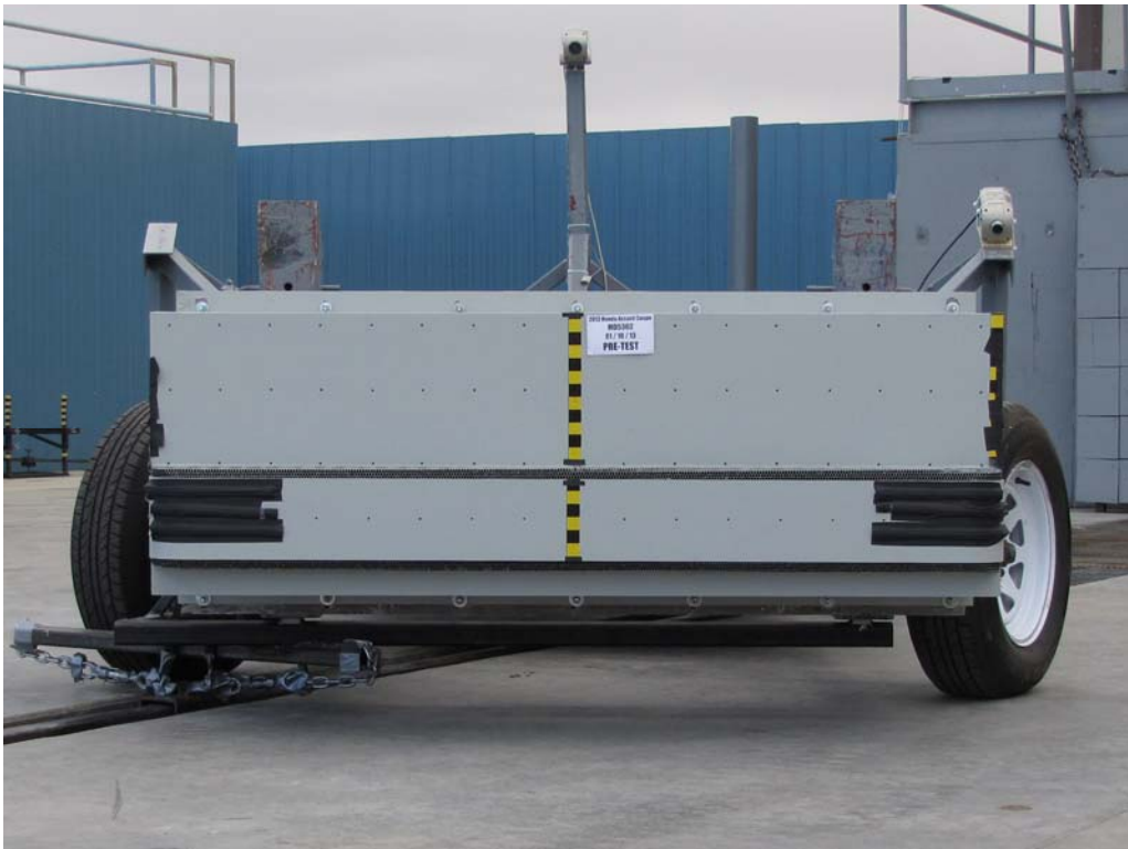
FIGURE 84. Pre-Test Front View of MDB Impactor Face
