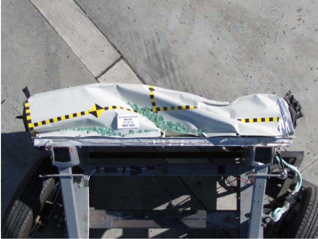
FIGURE 87. Post-Test Top View of MDB Impactor Face
