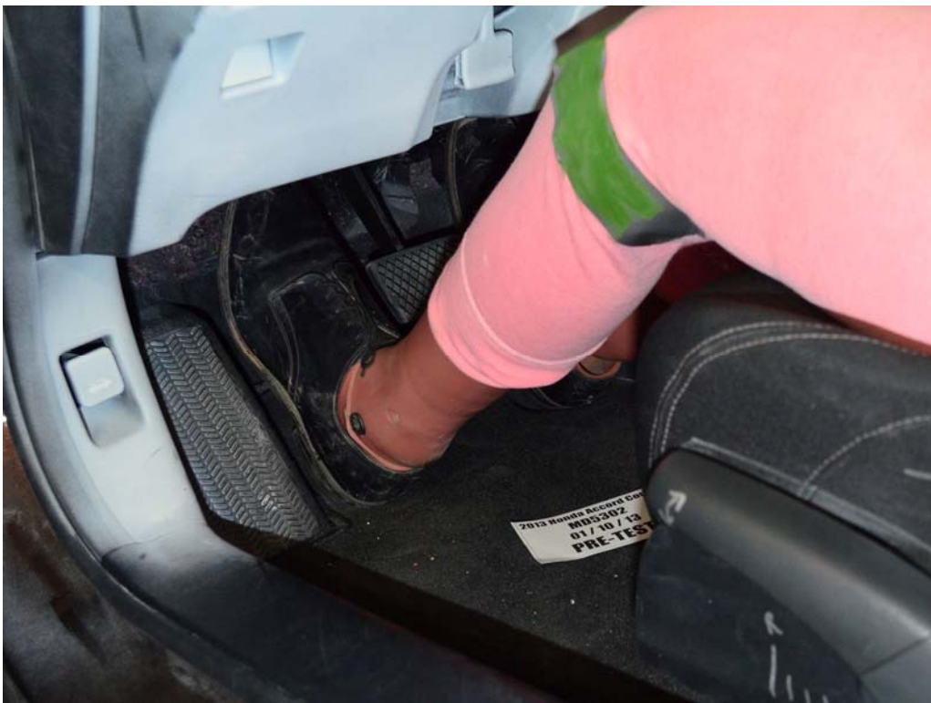
FIGURE 34. Pre-Test Placement of Driver Dummy's Feet
