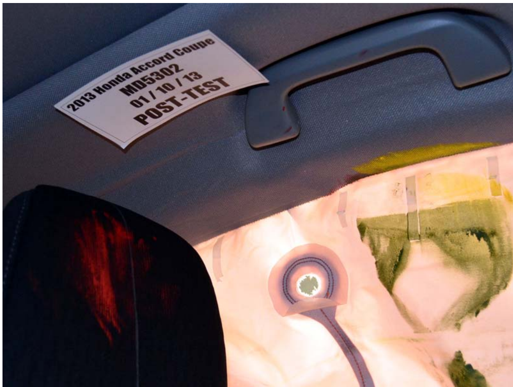
FIGURE 48. Post-Test Driver Dummy Close-Up Head Contact with Vehicle View
