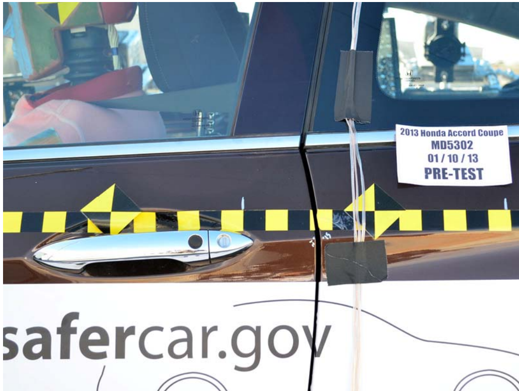
FIGURE 21. Pre-Test Left Front Door Latch Close-Up
