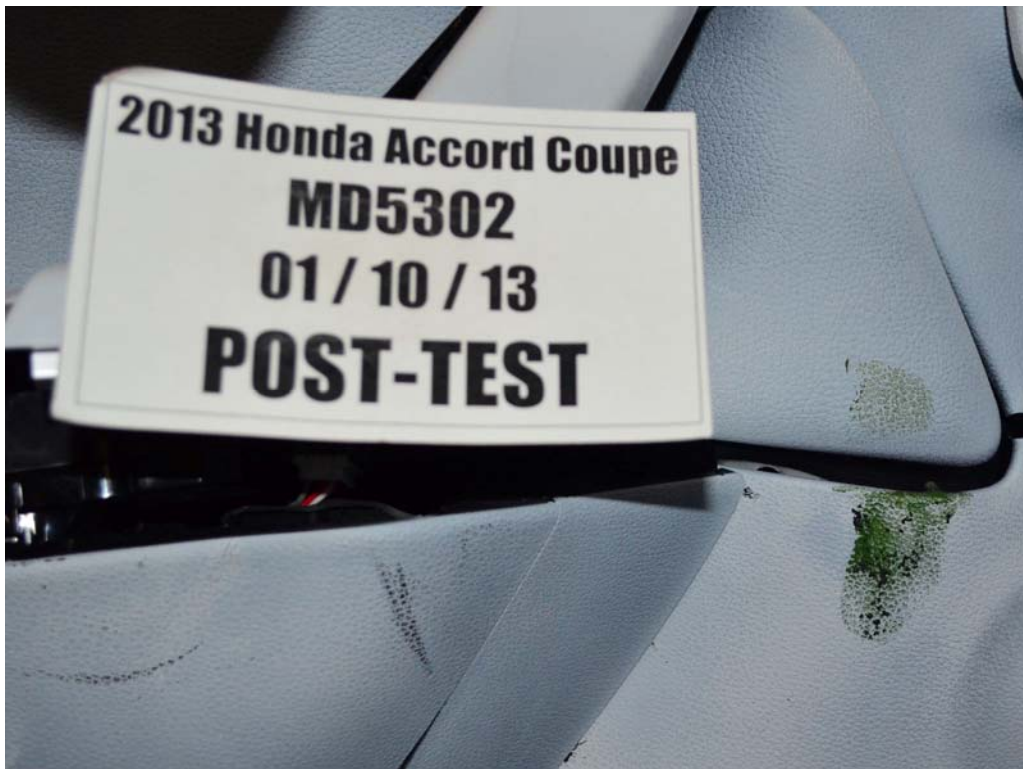
FIGURE 54. Post-Test Driver Dummy Close-Up Knee Contact View
