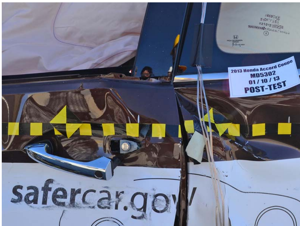
FIGURE 22. Post-Test Left Front Door Latch Close-Up
