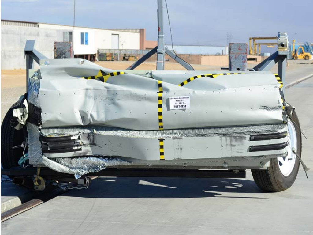
FIGURE 85. Post-Test Front View of MDB Impactor Face
