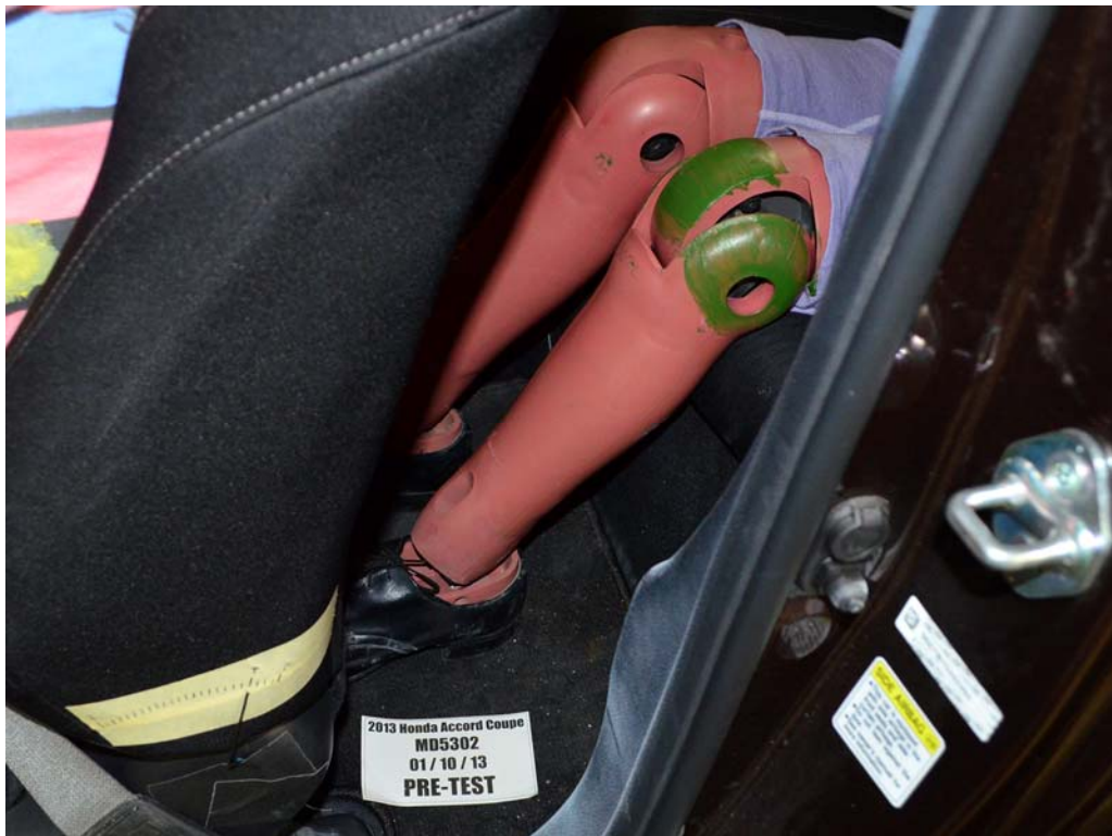
FIGURE 64. Pre-Test Placement of Rear Passenger Dummy's Feet
