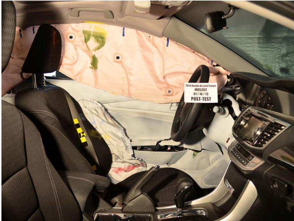
FIGURE 47. Post-Test Driver Inner Door Panel View
