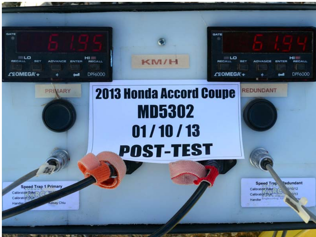
FIGURE 95. Post-Test Primary and Redundant Speed Trap Read-Out
