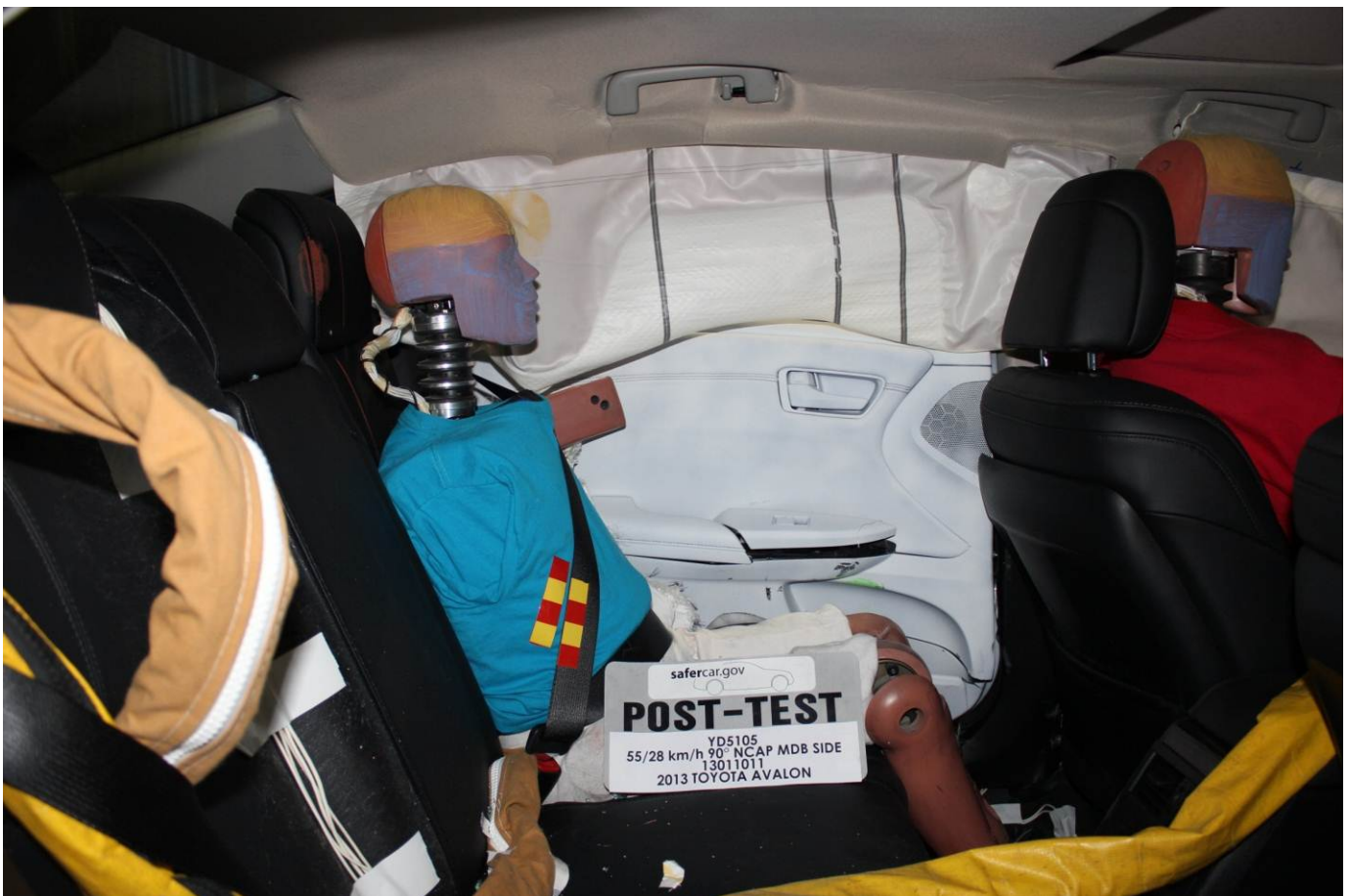
Post-Test Right Side View of Rear Passenger Dummy and Rear Seat Occupant Compartment
