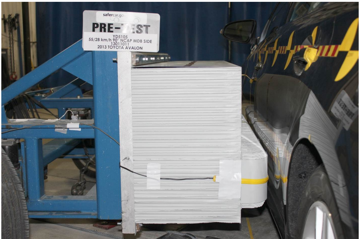
Pre-Test Right Side View of MDB Positioned Against Side of Test Vehicle
