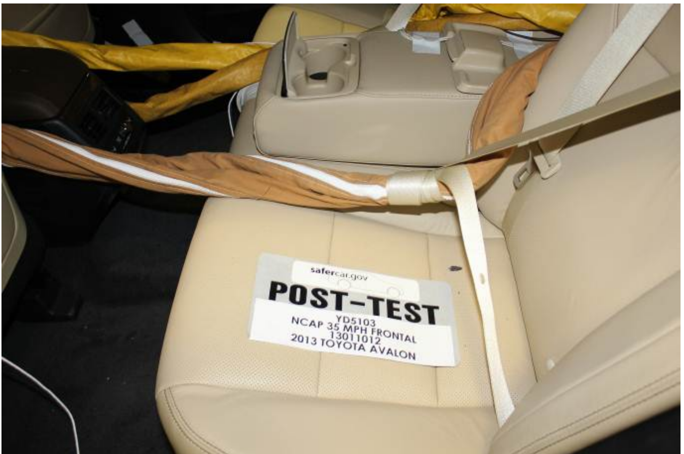
Post-Test Dummy Cable Routing
