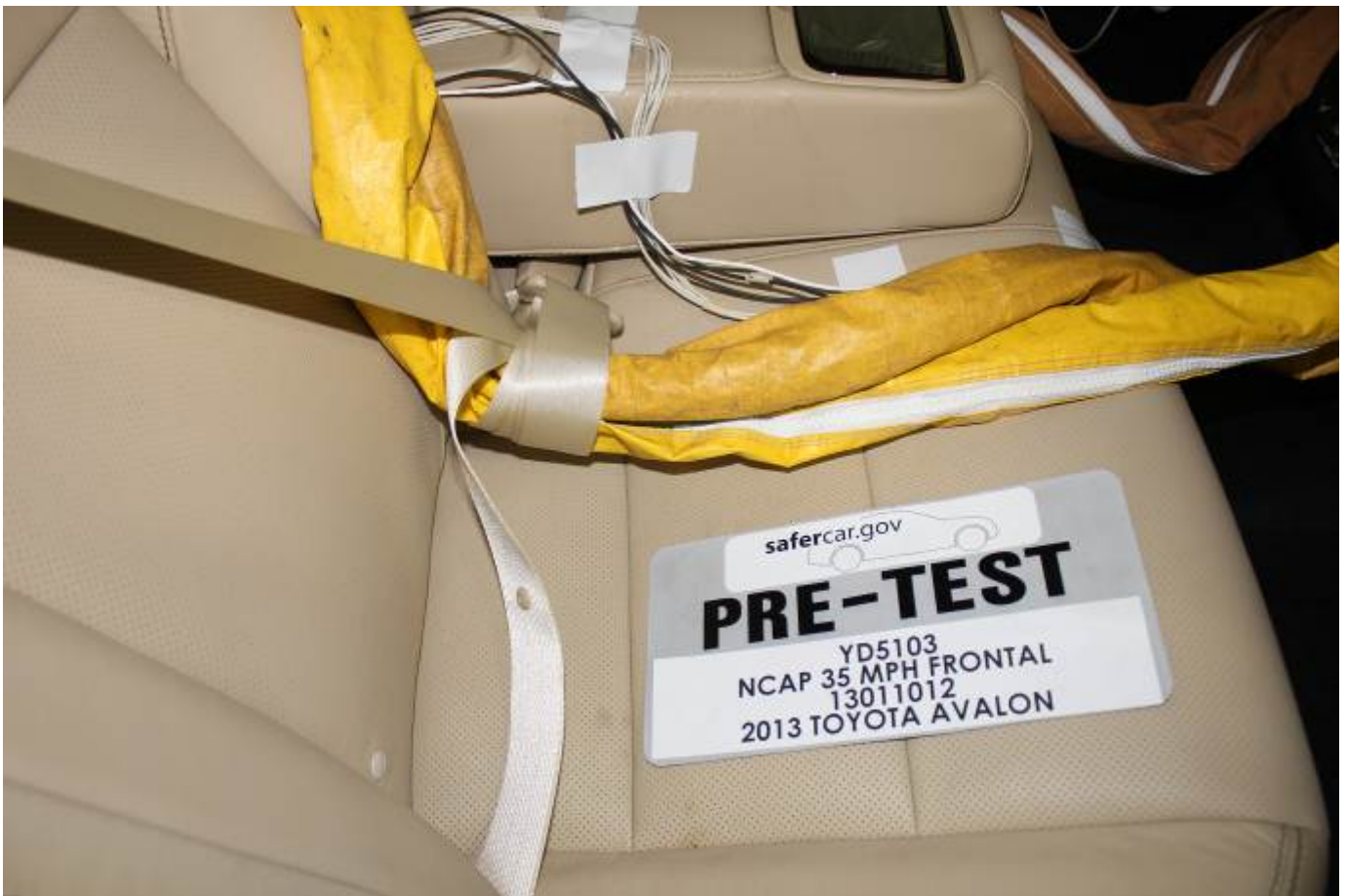
Pre-Test Dummy Cable Routing
