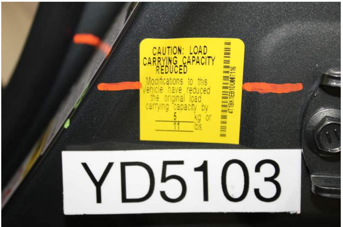
Reduced Load Carrying Capacity
