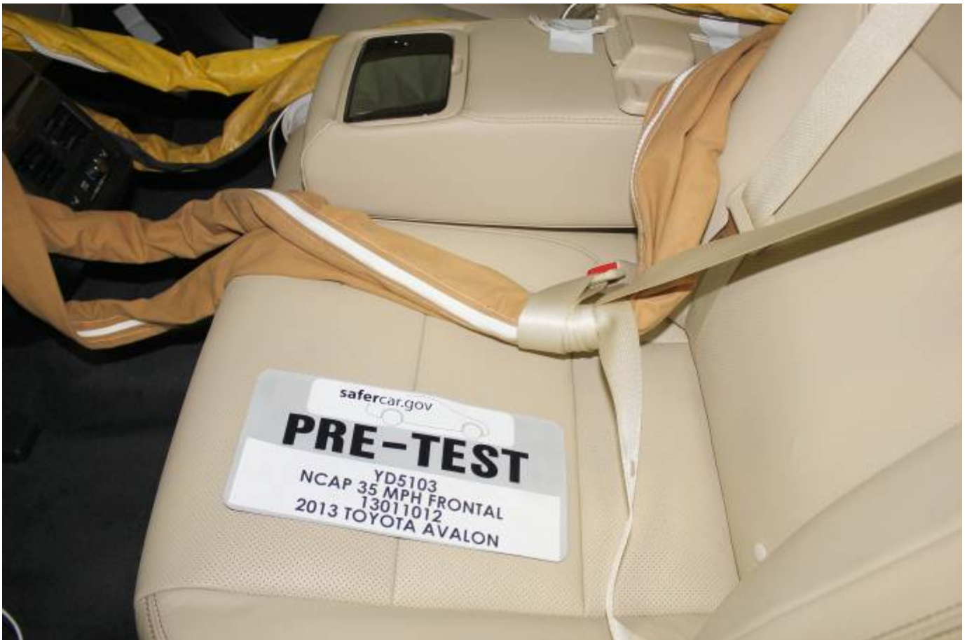
Pre-Test Dummy Cable Routing
