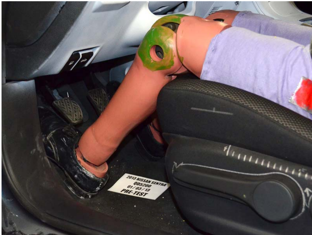
FIGURE 32. Pre-Test Placement of Dummy's Feet
