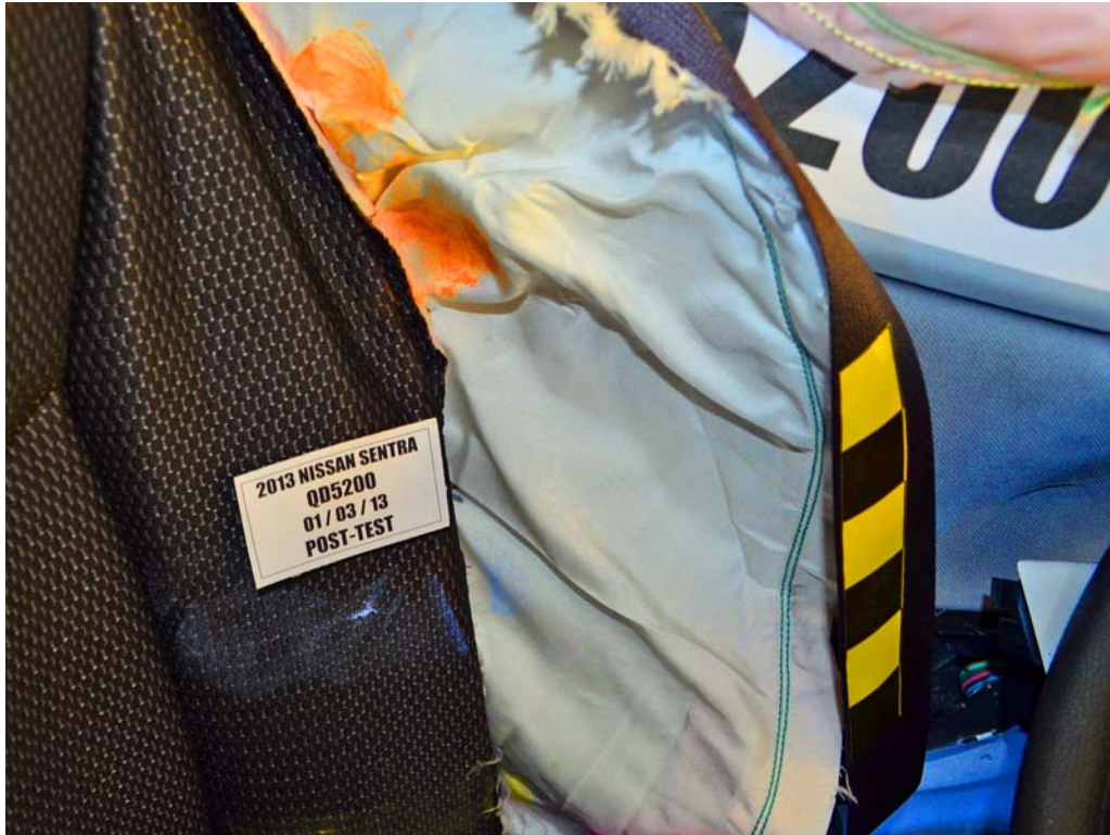
FIGURE 49. Post-Test Dummy Close-Up Torso Contact with Side Airbag View
