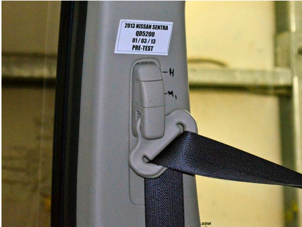
FIGURE 33. Pre-Test View of Belt Anchorage for Dummy
