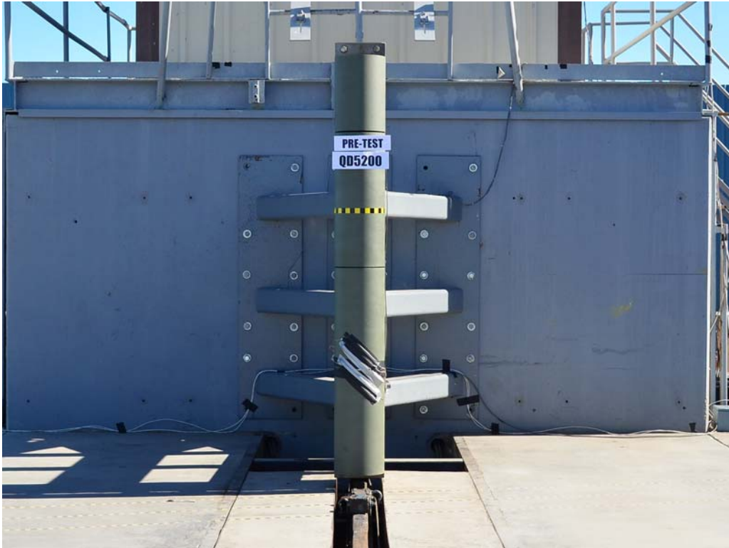
FIGURE 57. Pre-Test Pole Barrier Front View
