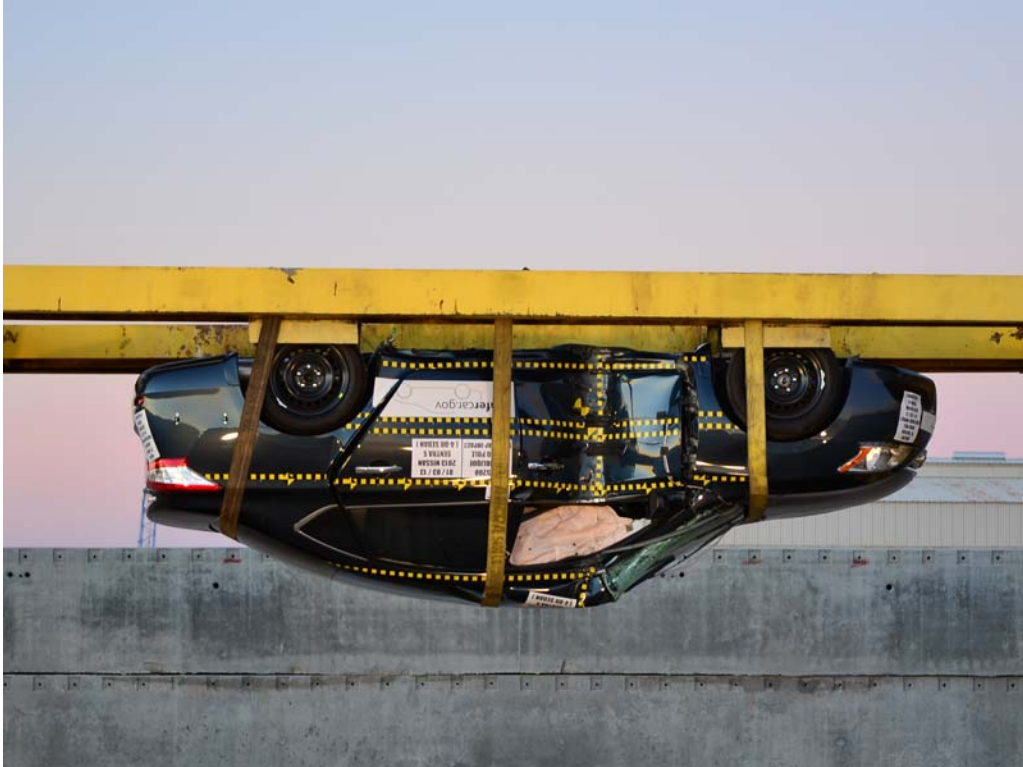
FIGURE 65. FMVSS No. 301 Static Rollover 180 Degrees
