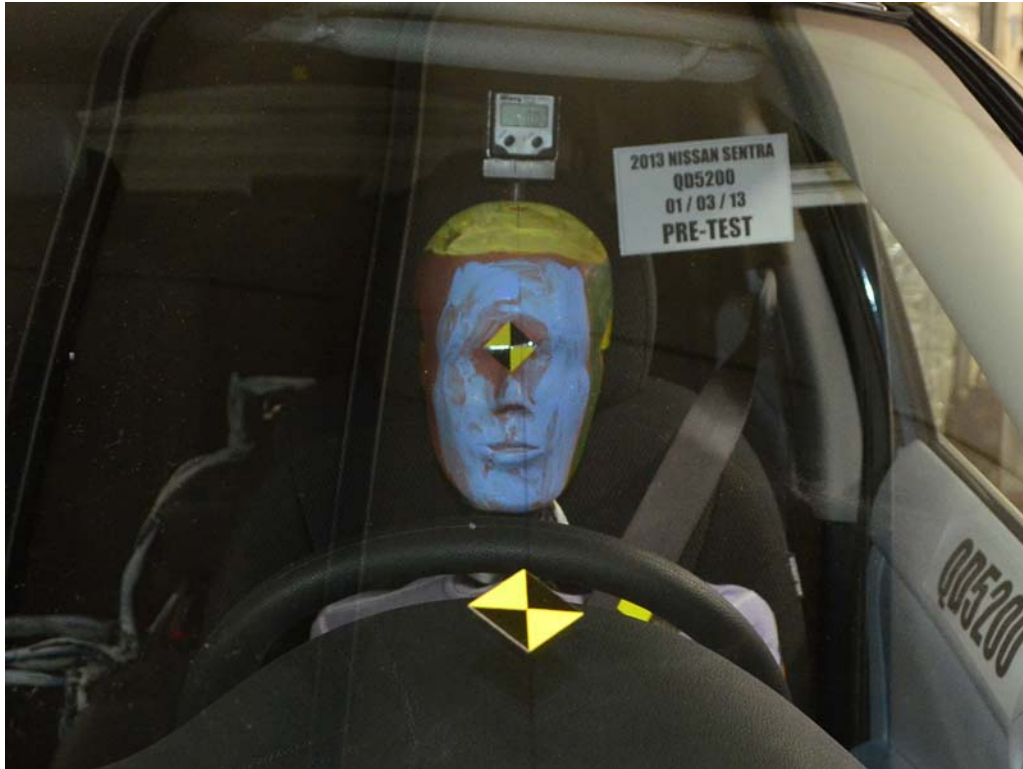
FIGURE 27. Pre-Test Frontal Close-Up View of Dummy Head and Shoulders in Relation to Head Restraint
