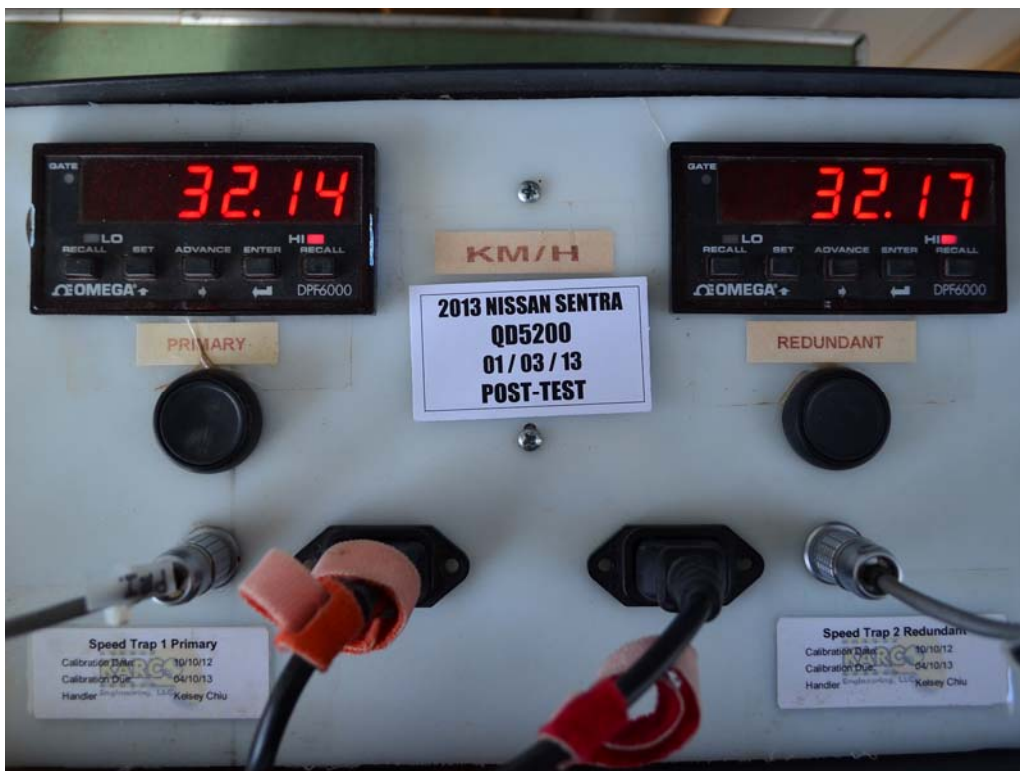
FIGURE 62. Post-Test Primary and Redundant Speed Trap Read-Out
