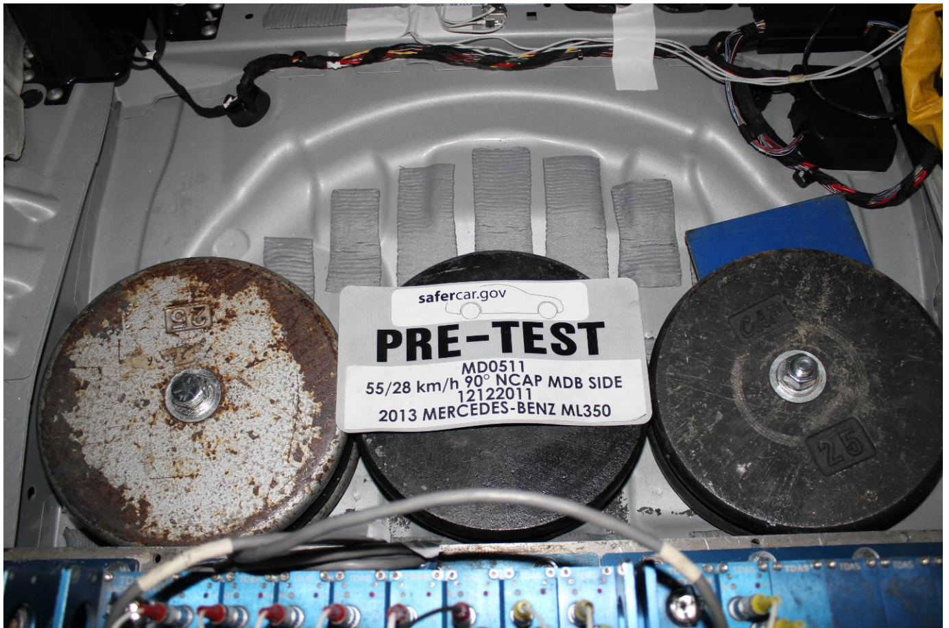
Pre-Test Ballast View
