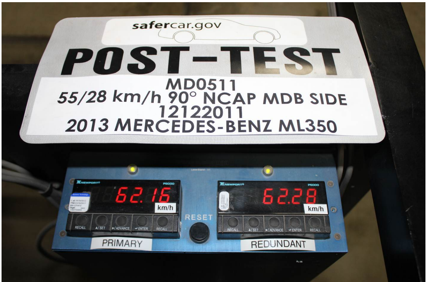
Post-Test Primary and Redundant Speed Trap Read-Out
