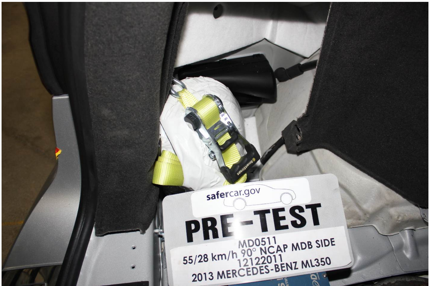
Pre-Test Ballast View
