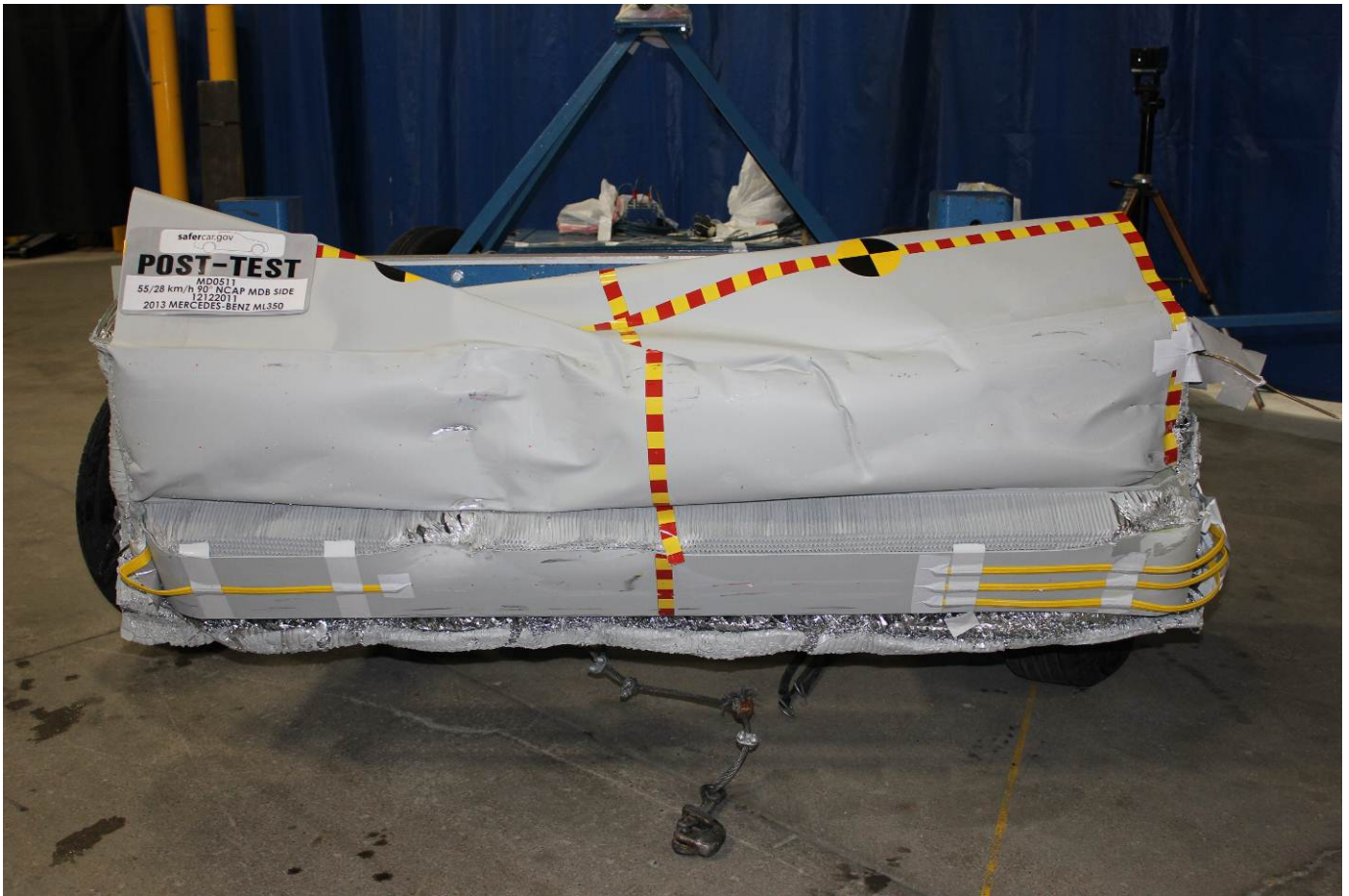
Post-Test Front View of MDB Impactor Face
