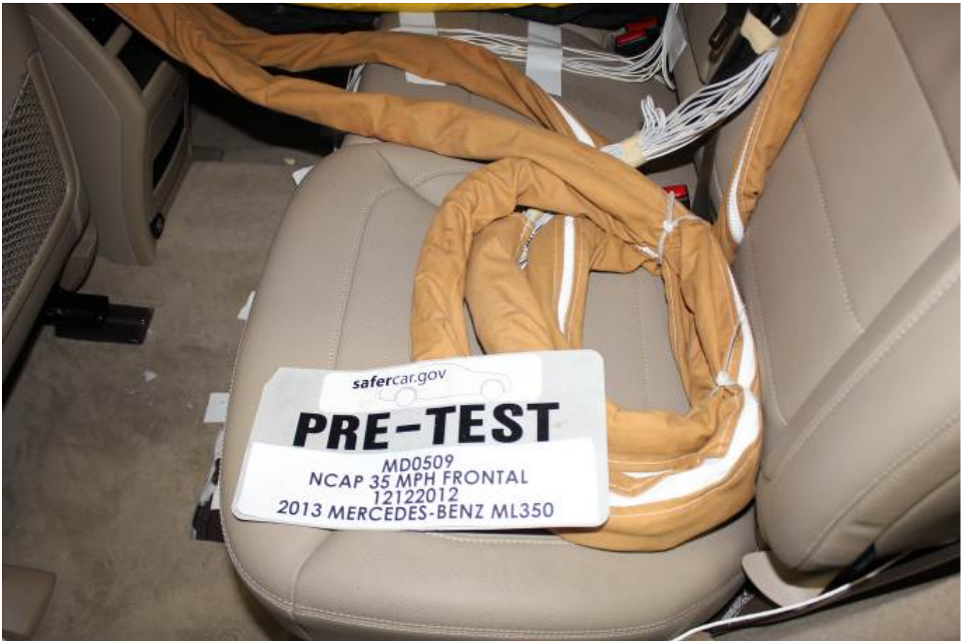
Pre-Test Dummy Cable Routing
