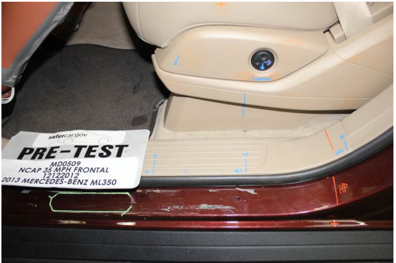
Pre-Test Driver's Seat Fore-Aft Markings
