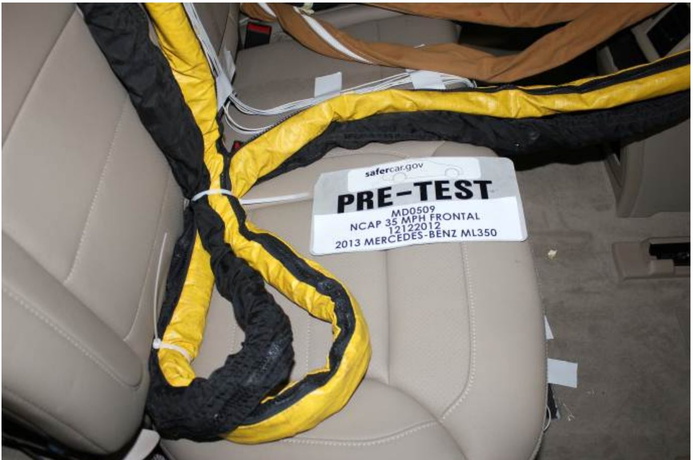
Pre-Test Dummy Cable Routing
