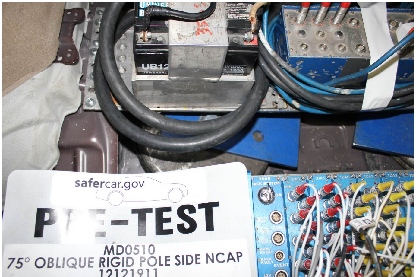
Pre-Test Ballast View
