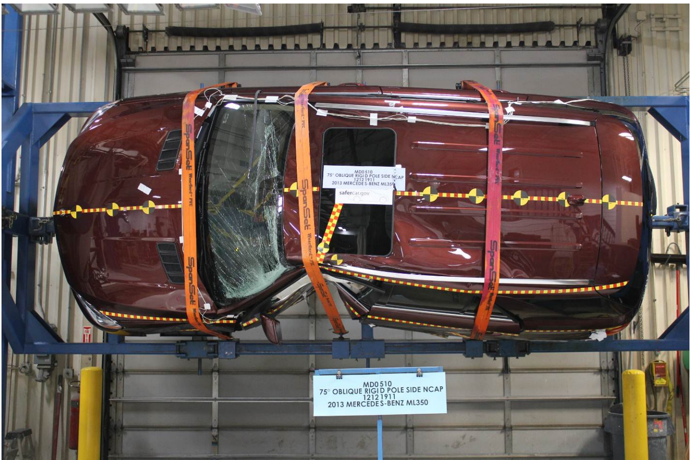
FMVSS No. 301 Static Rollover 270 Degrees
