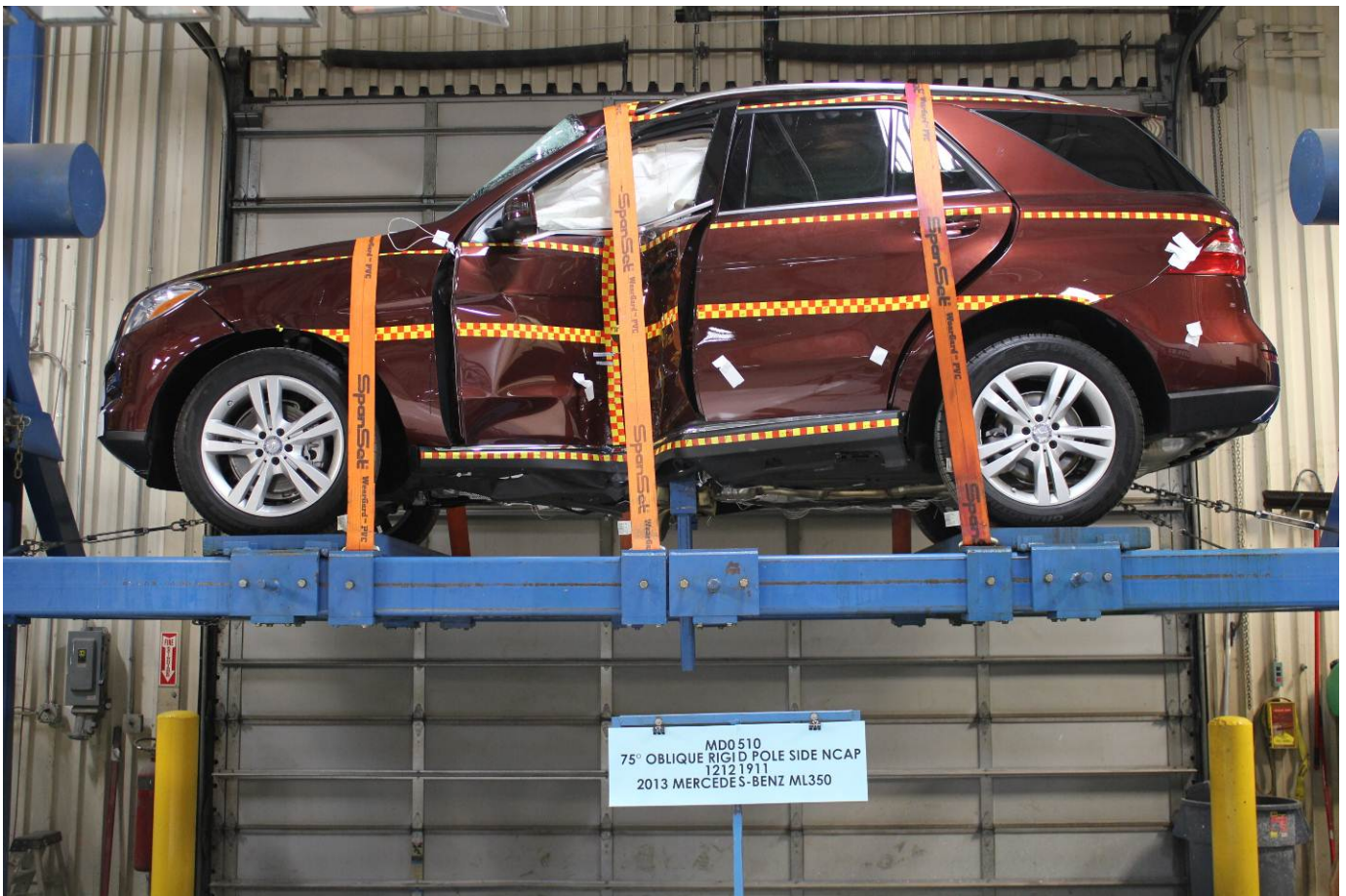
FMVSS No. 301 Static Rollover 360 Degrees
