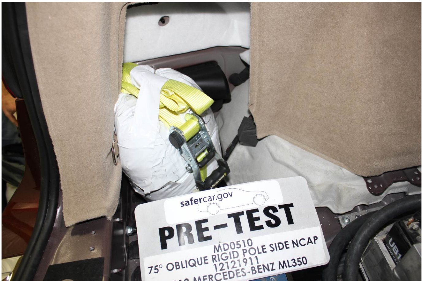
Pre-Test Ballast View
