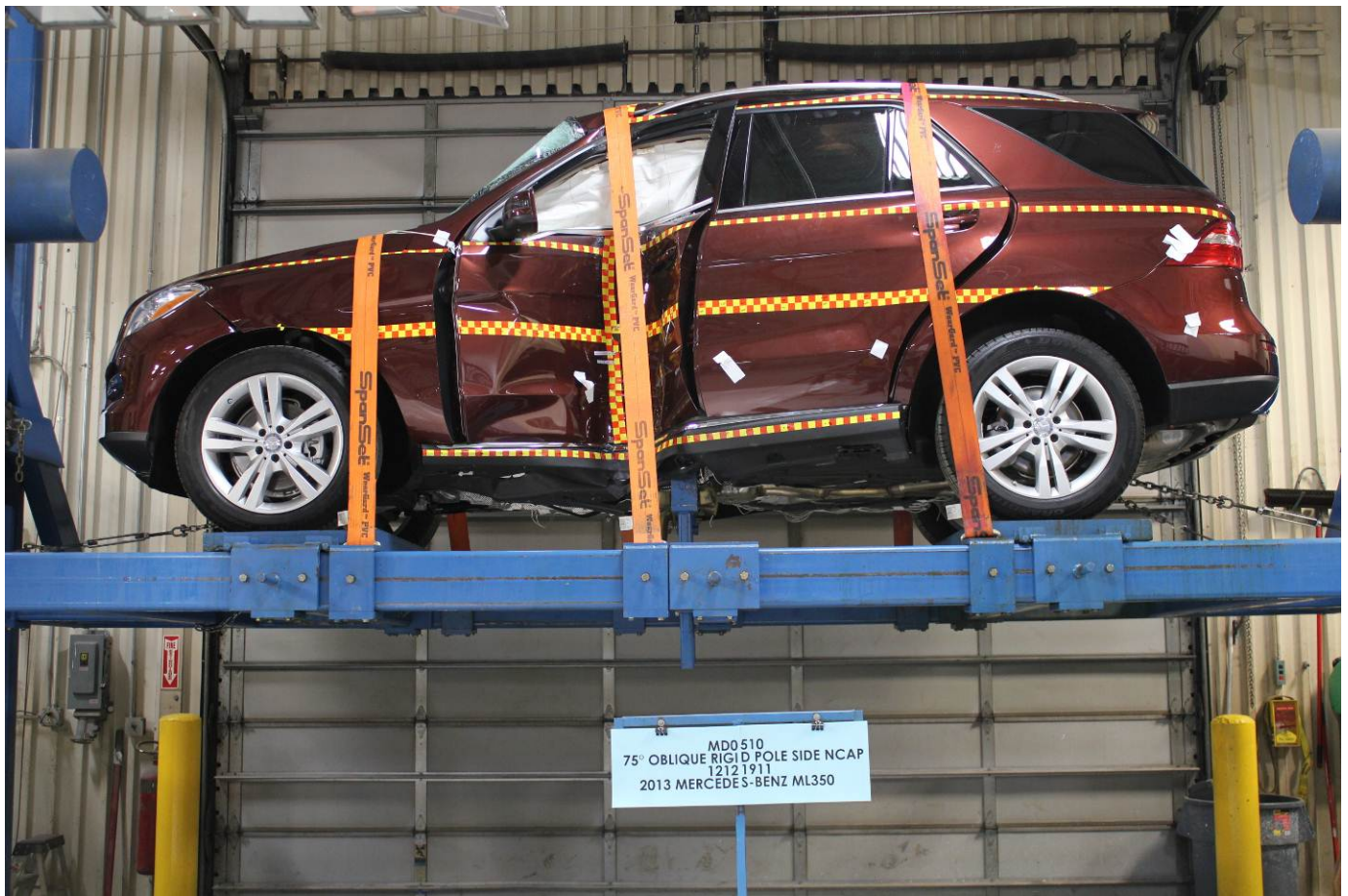
FMVSS No. 301 Static Rollover 0 Degrees
