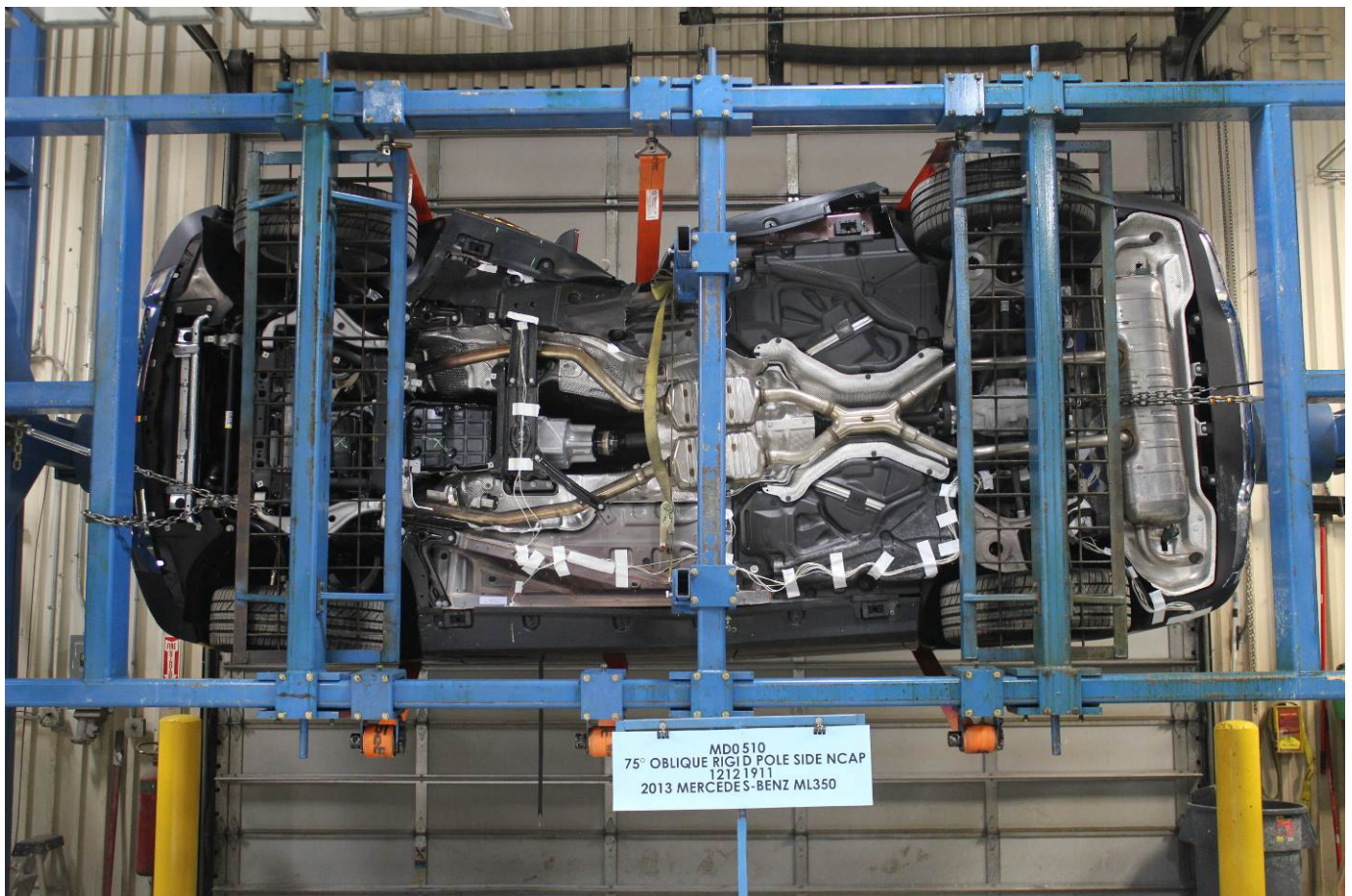
FMVSS No. 301 Static Rollover 90 Degrees
