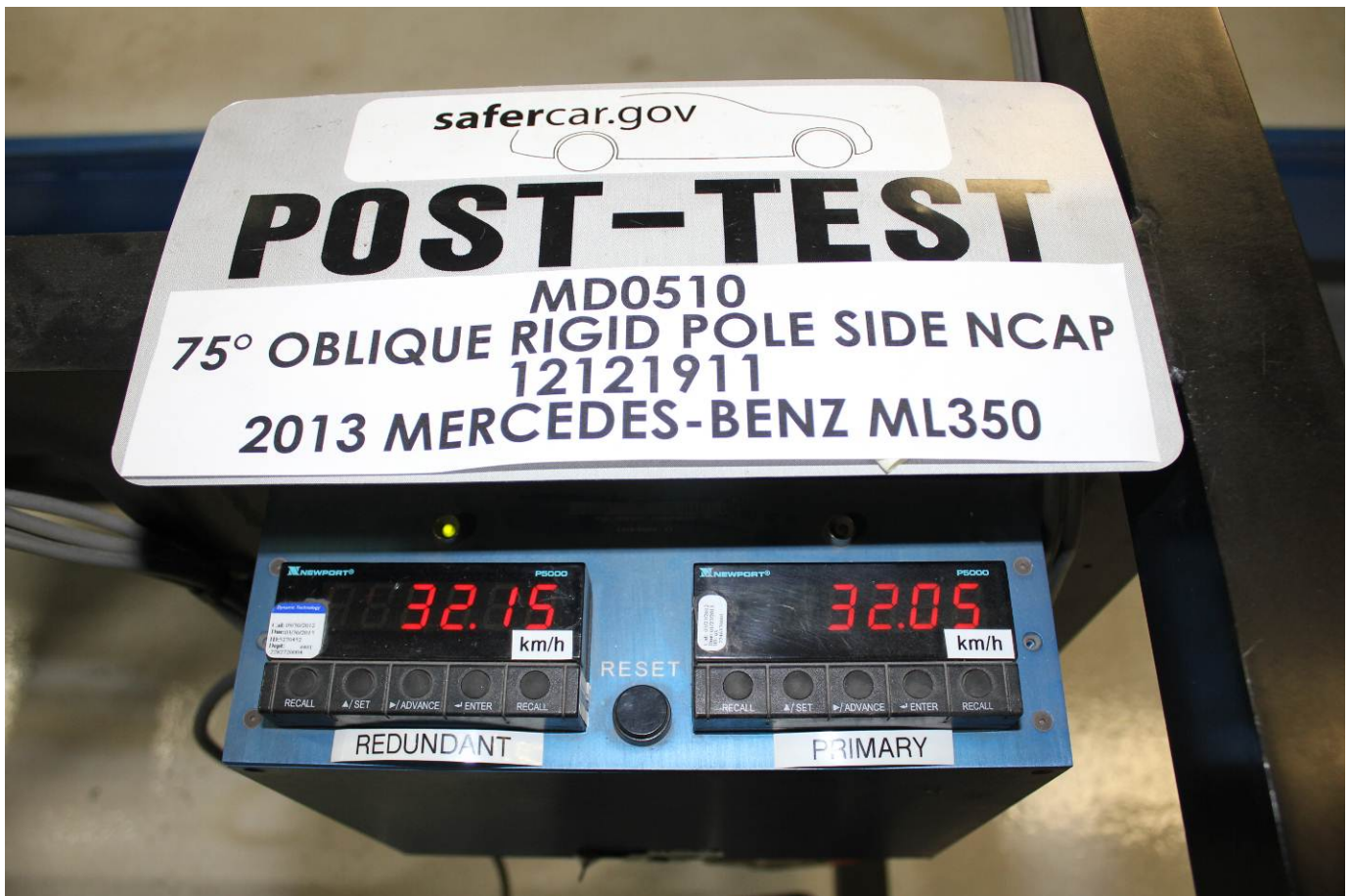
Post-Test Primary and Redundant Speed Trap Read-Out
