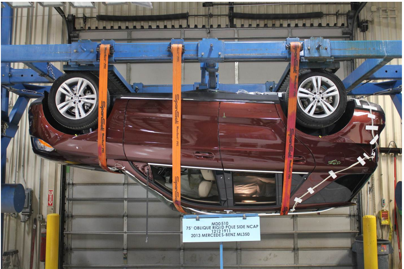
FMVSS No. 301 Static Rollover 180 Degrees
