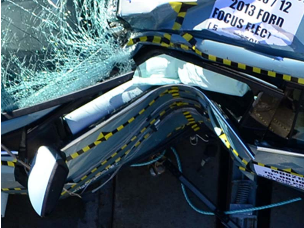
FIGURE 41. Post-Test Dummy and Door Clearance
