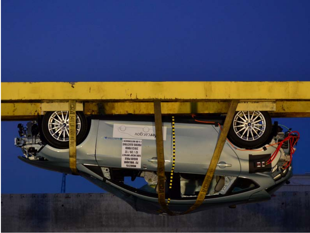
FIGURE 65. FMVSS No. 301 Rollover 180 Degrees
