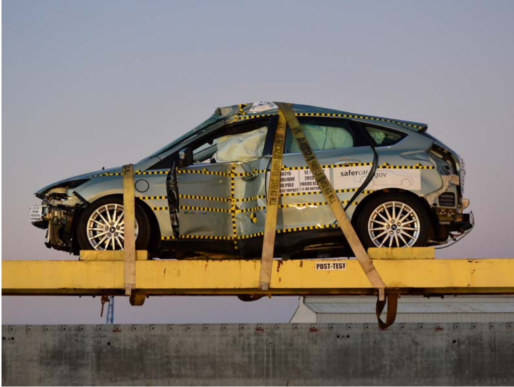
FIGURE 63. FMVSS No. 301 Rollover 0 Degrees
