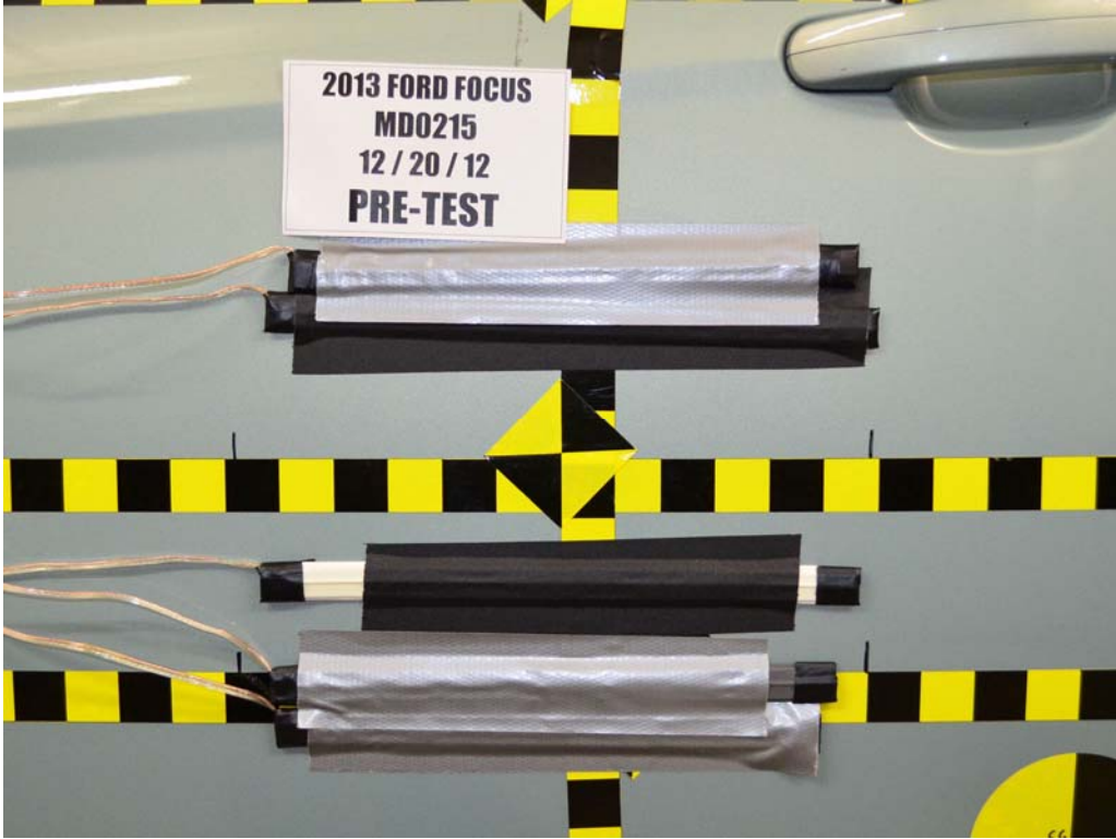
FIGURE 19. Pre-Test Close-Up View of Impact Point Target
