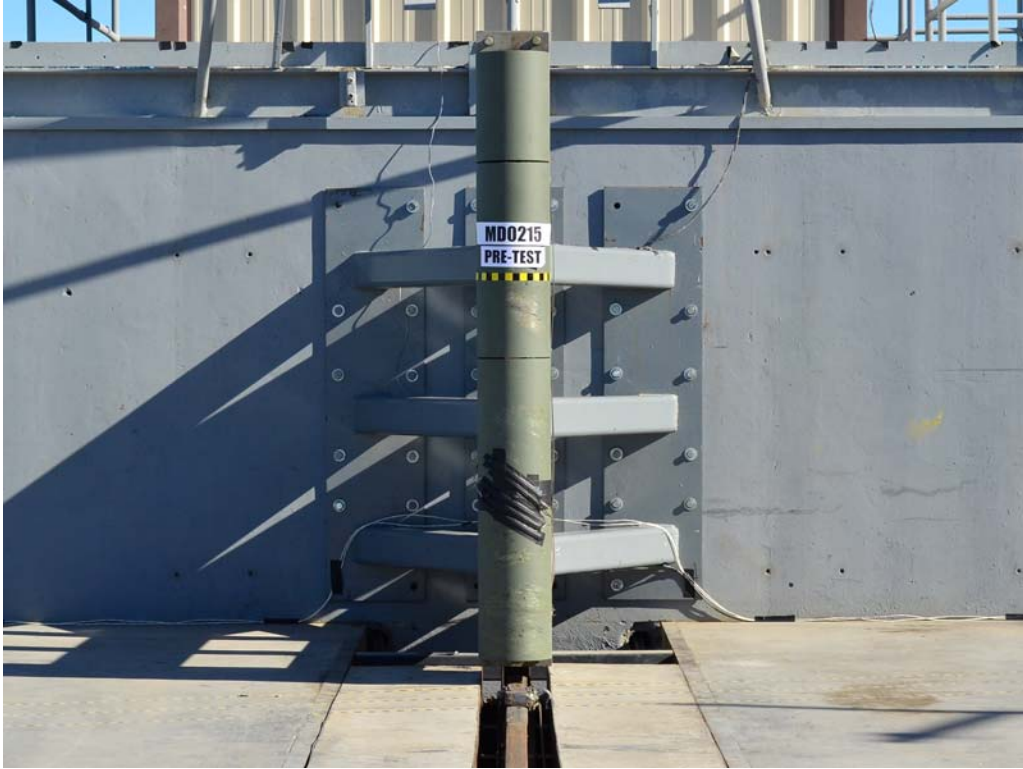
FIGURE 57. Pre-Test Pole Barrier Front View
