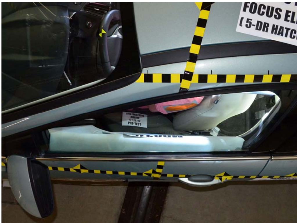
FIGURE 40. Pre-Test Dummy and Door Clearance
