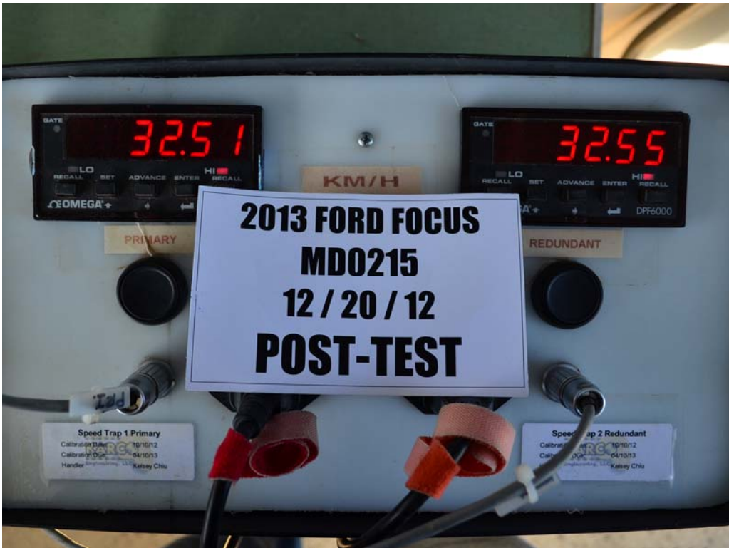
FIGURE 62. Post-Test Primary and Redundant Speed Trap Read-Out
