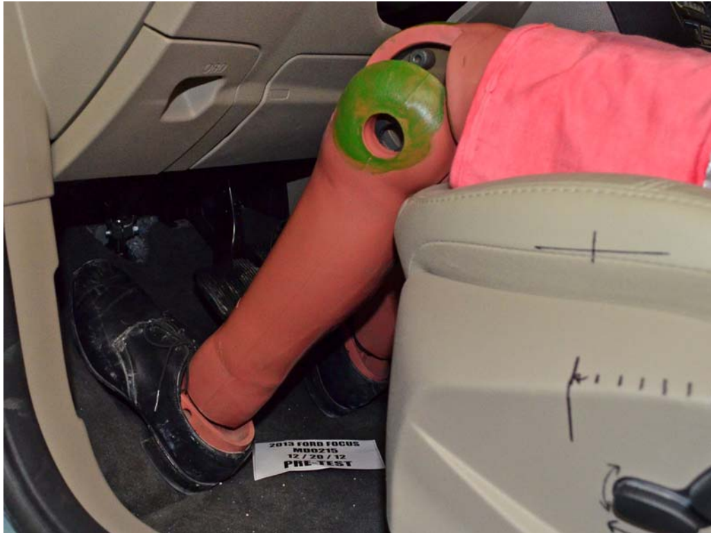
FIGURE 32. Pre-Test Placement of Dummy's Feet
