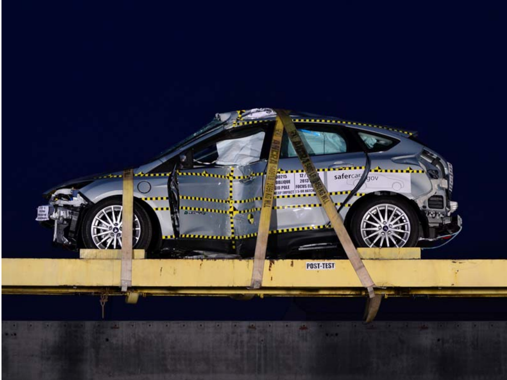
FIGURE 67. FMVSS No. 301 Rollover 360 Degrees
