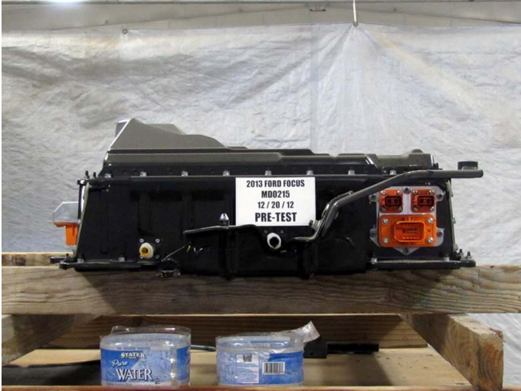
FIGURE 12c. Pre-Impact View of Battery Box or Container Which Hold Individual Battery Modules
