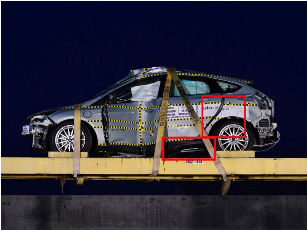
FIGURE 32. FMVSS No. 305 Static Rollover at 360°
