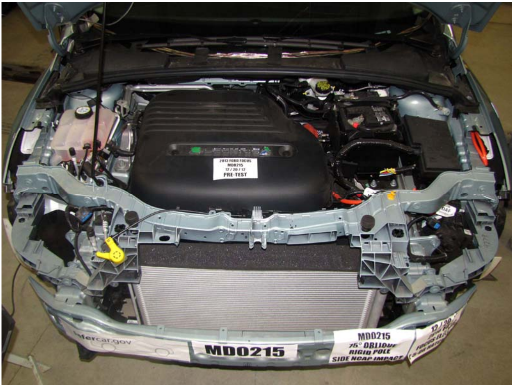
FIGURE 16. Pre-Impact View of Electric Propulsion Drive
