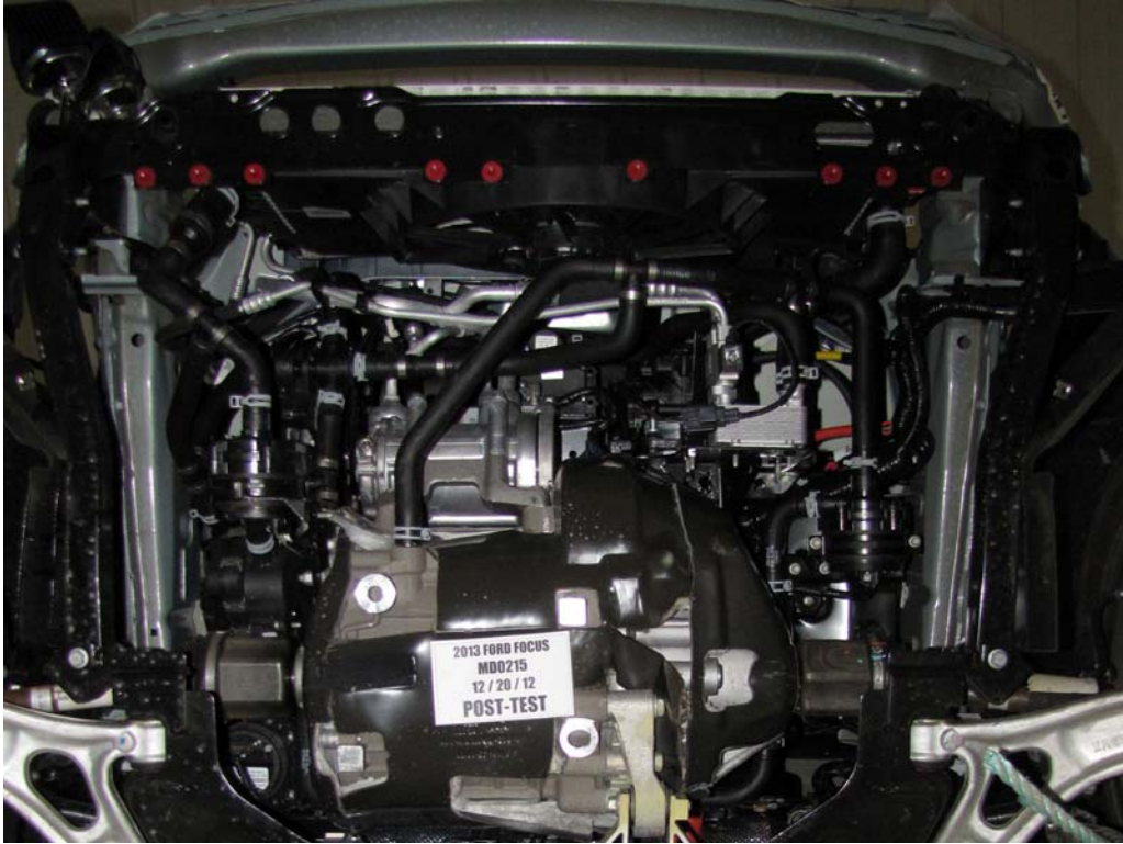
FIGURE 17a. Post-Impact View of Electric Propulsion Drive
