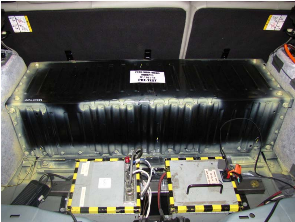
FIGURE 33a. Pre-Impact View of Vehicle Passenger Compartment Adjacent to Propulsion Battery
