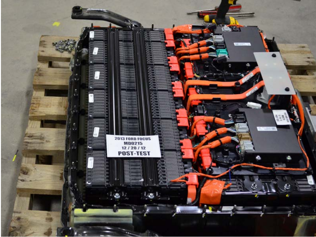
FIGURE 15c. Post-Impact View of Battery Modules
