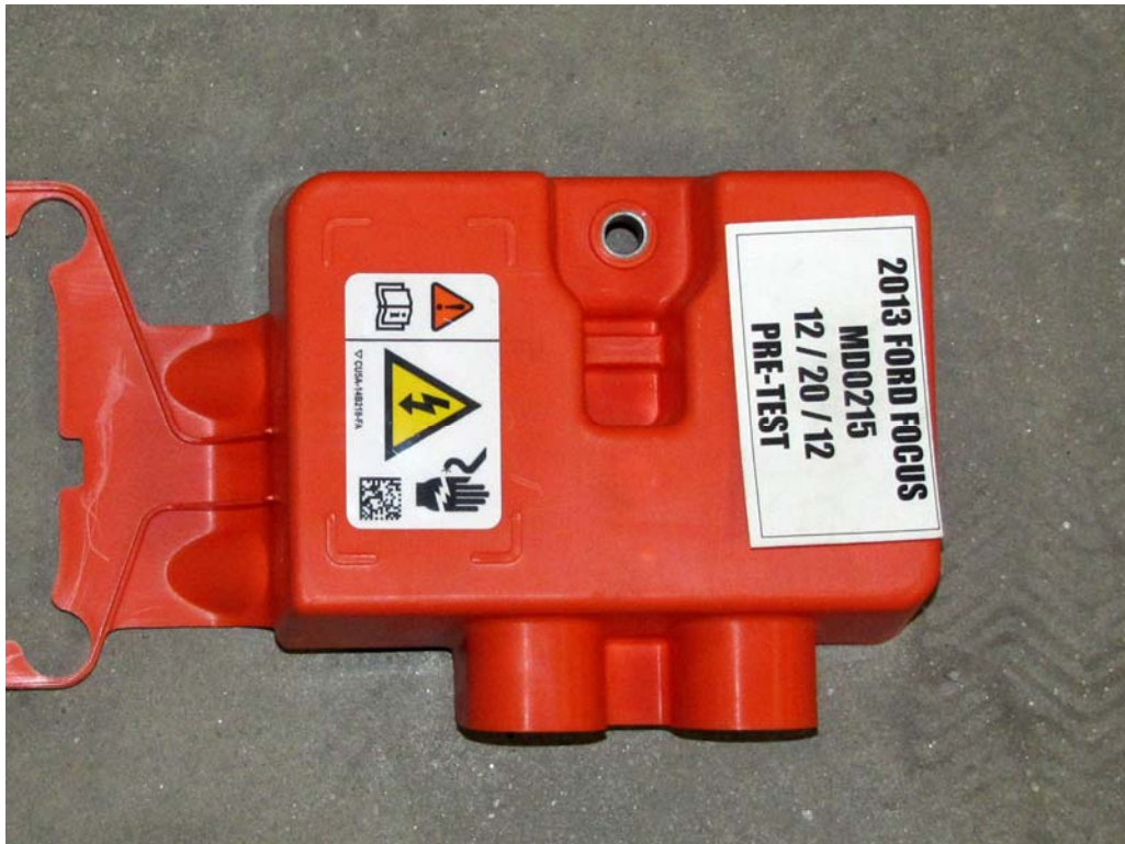
FIGURE 1c. Auxiliary Power Module Warning Label
