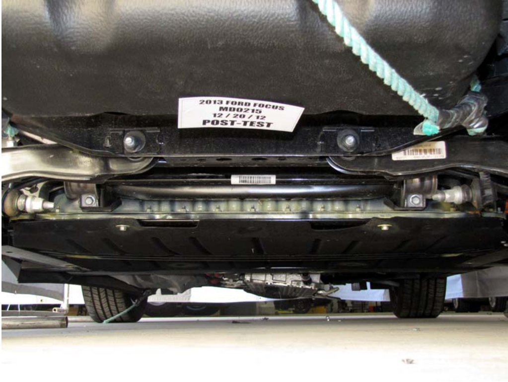
FIGURE 11a. Post-Impact Rear View of Propulsion Battery
