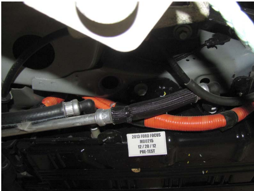
FIGURE 19. Pre-Impact View of Propulsion Battery Venting System(s)
