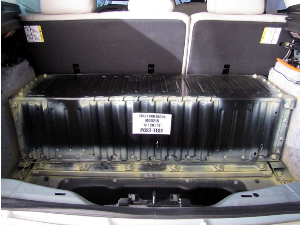
FIGURE 13. Post-Impact View of Battery Box or Container Which Hold Individual Battery Modules
