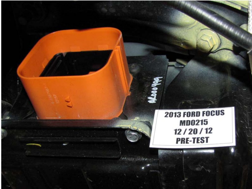
FIGURE 7a. Manual High Voltage Service Disconnect Removed
