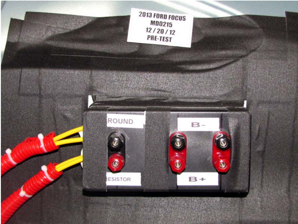
FIGURE 24. Pre-Impact View of Installed Test Interface Port
