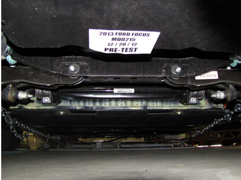
FIGURE 9c. Pre-Impact View of Propulsion Battery
