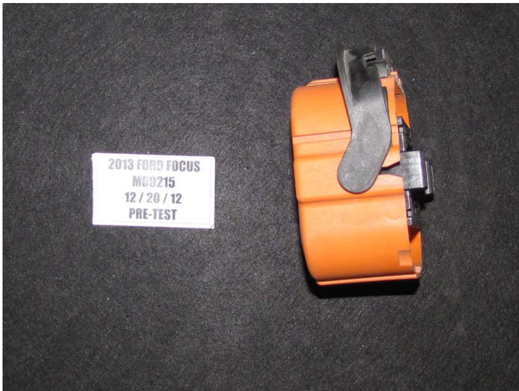
FIGURE 8. Manual High Voltage Service Disconnect Removed
