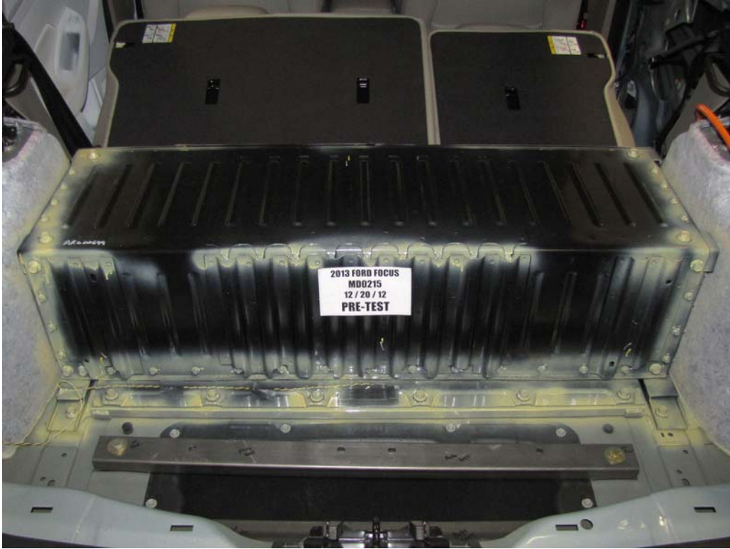
FIGURE 9a. Pre-Impact View of Propulsion Battery
