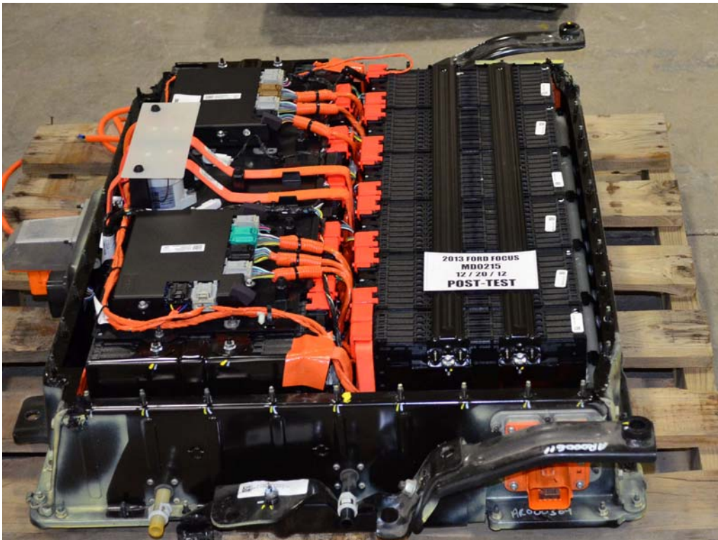
FIGURE 15b. Post-Impact View of Battery Modules
