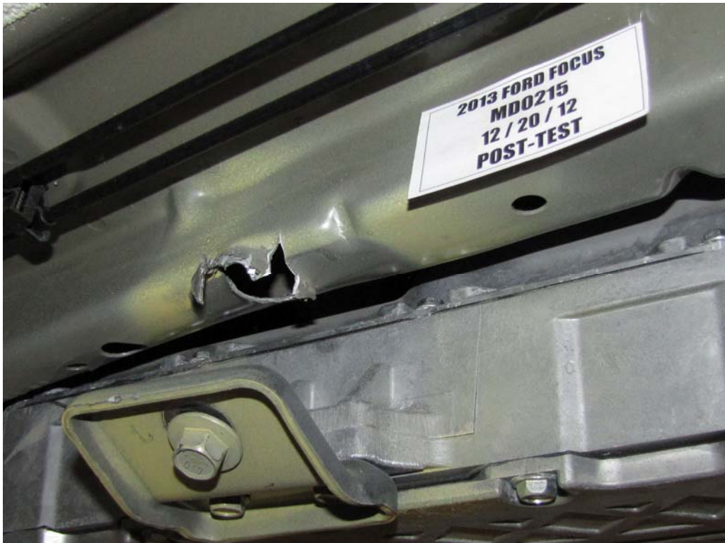
FIGURE 35a. Post-Impact Propulsion Battery System Mounting and/or Intrusion Failure
