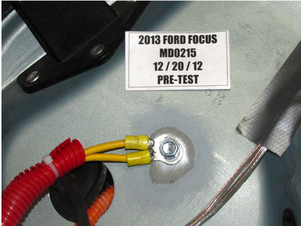
FIGURE 21. Pre-Impact View of Ground Lead Attached
