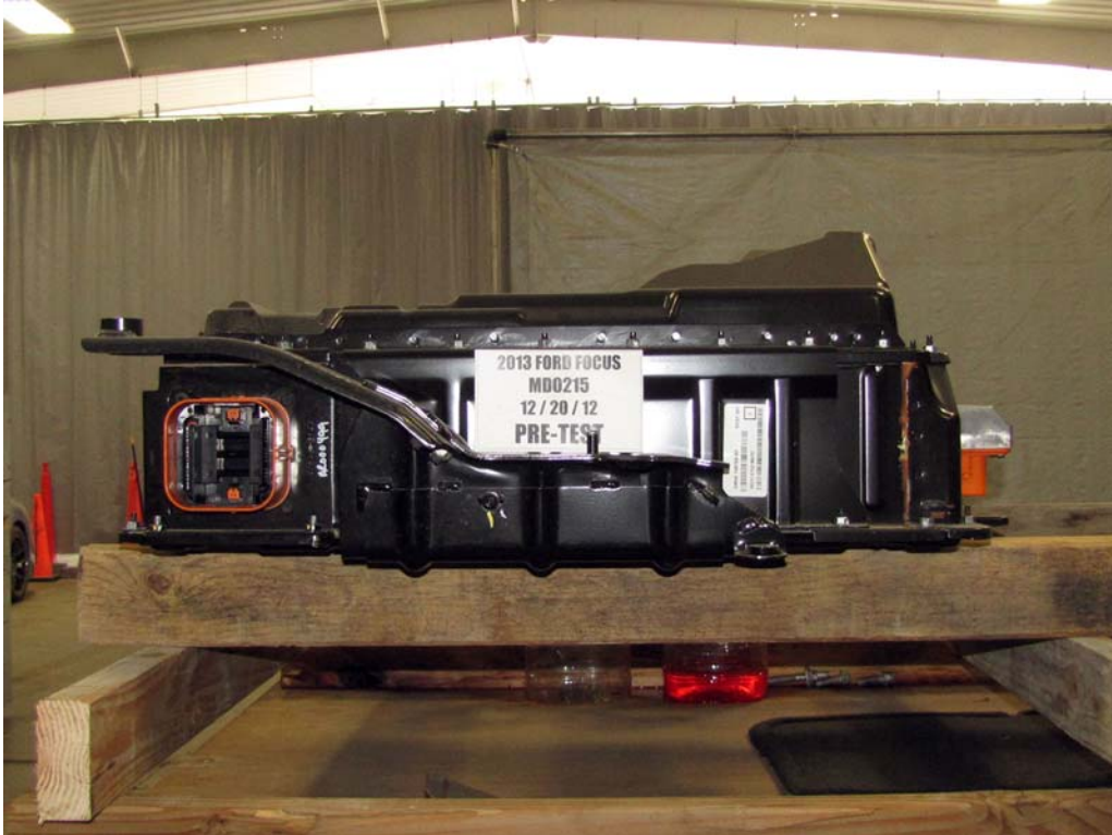
FIGURE 12e. Pre-Impact View of Battery Box or Container Which Hold Individual Battery Modules
