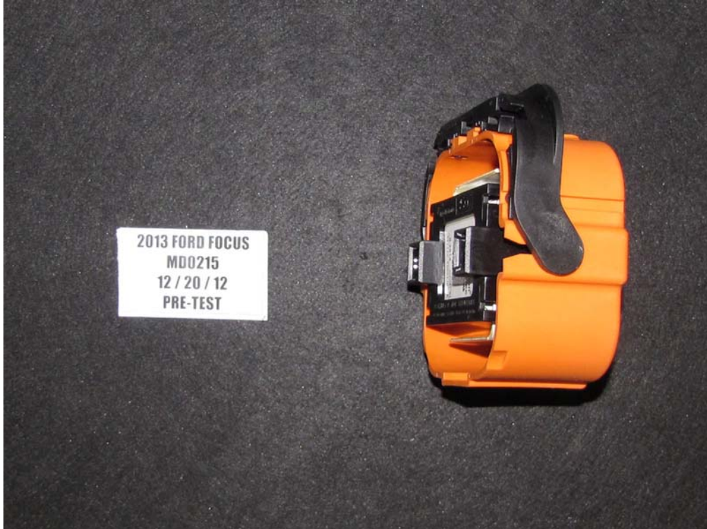
FIGURE 8a. Manual High Voltage Service Disconnect Removed
