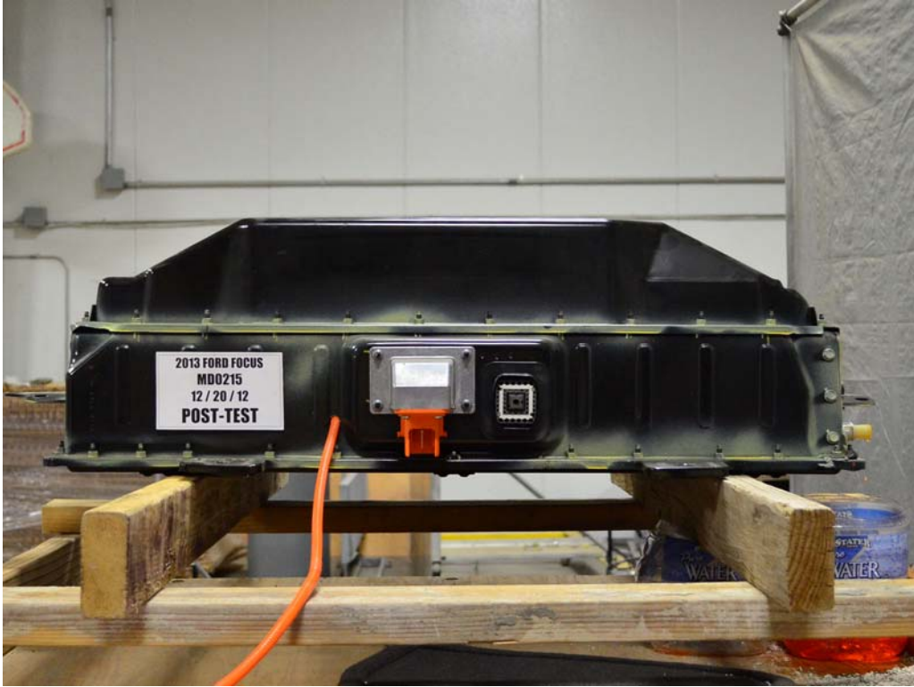
FIGURE 13d. Post-Impact View of Battery Box or Container Which Hold Individual Battery Modules
