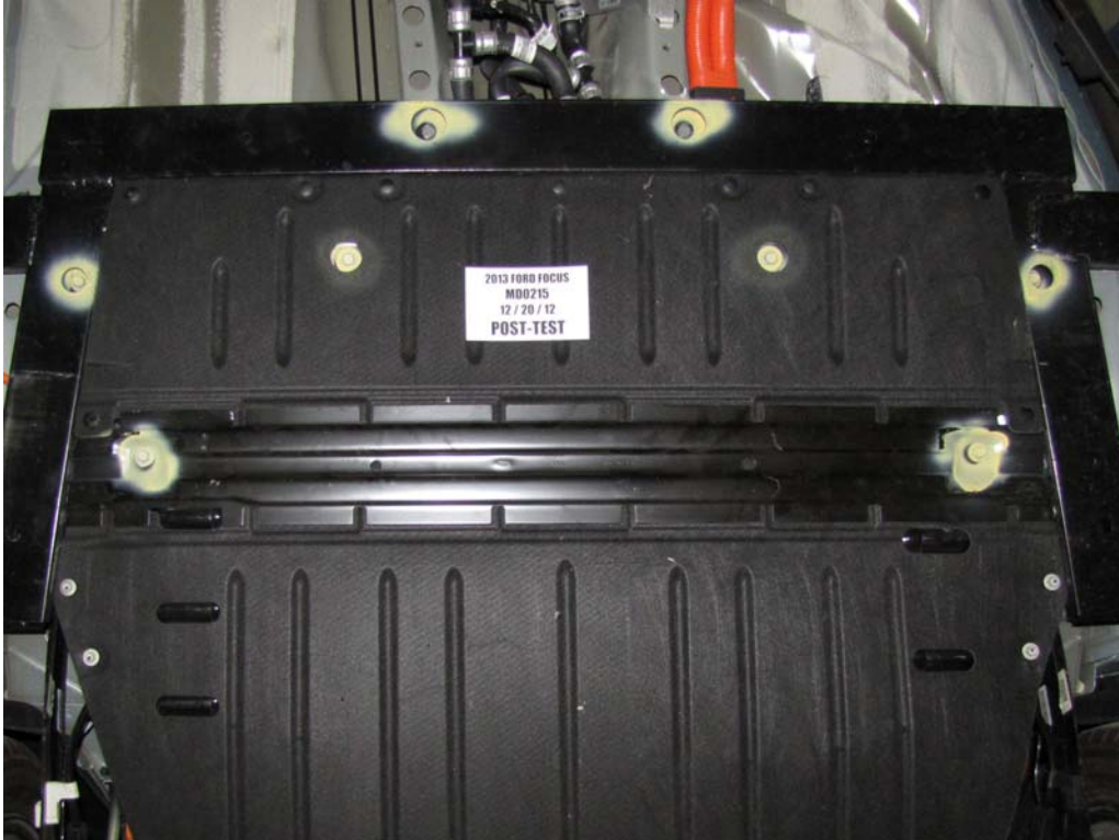
FIGURE 35b. Post-Impact Propulsion Battery System Mounting and/or Intrusion Failure
