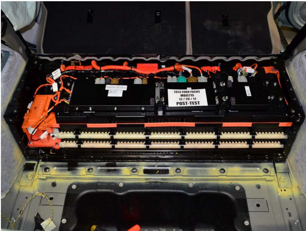
FIGURE 15. Post-Impact View of Battery Modules
