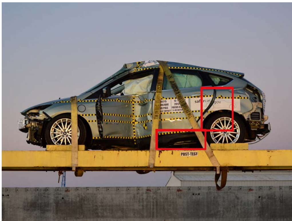
FIGURE 28. FMVSS No. 305 Static Rollover at 0°
