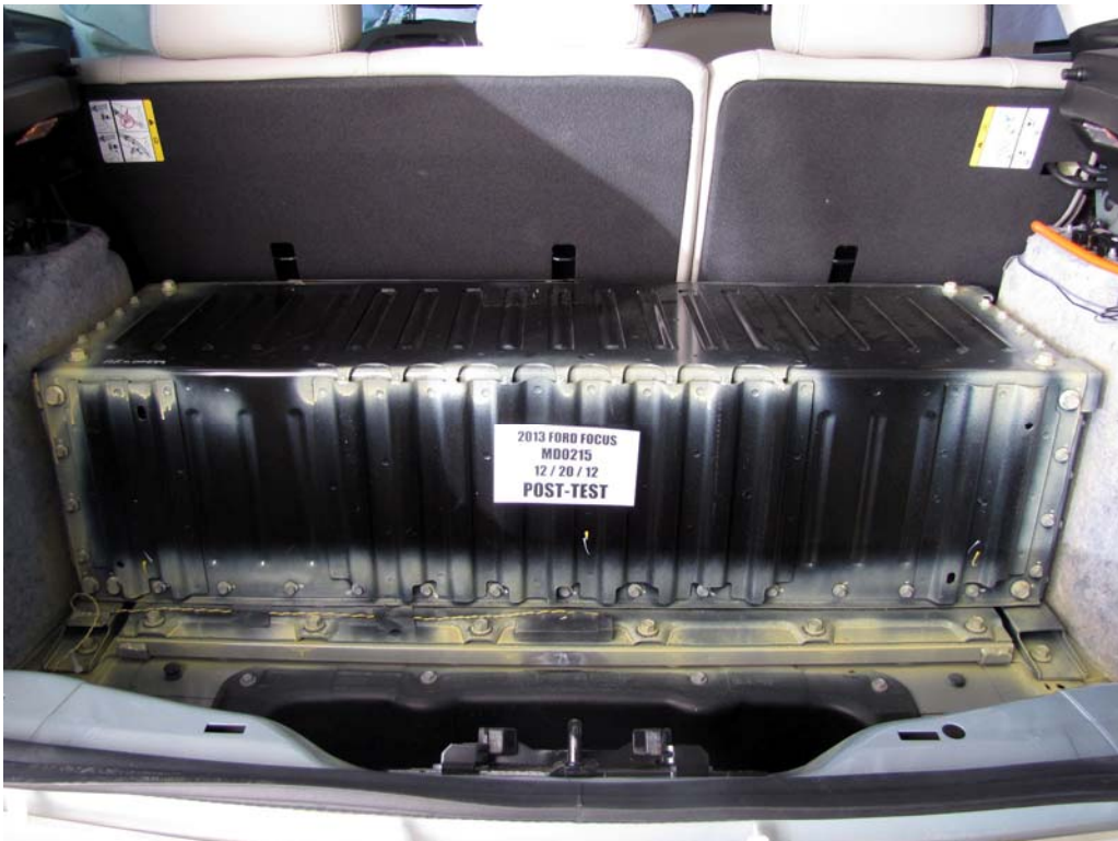
FIGURE 34a. Post-Impact View of Vehicle Passenger Compartment Adjacent to Propulsion Battery
