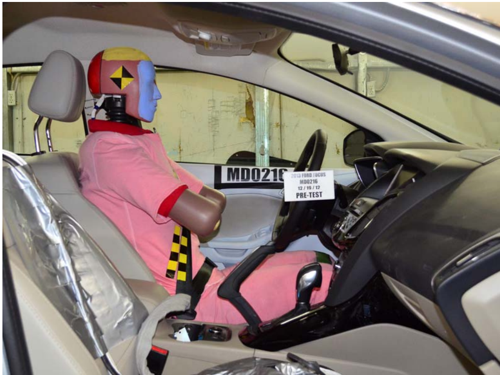
FIGURE 44. Pre-Test Right Side View of Driver Dummy and Front Seat Occupant Compartment
