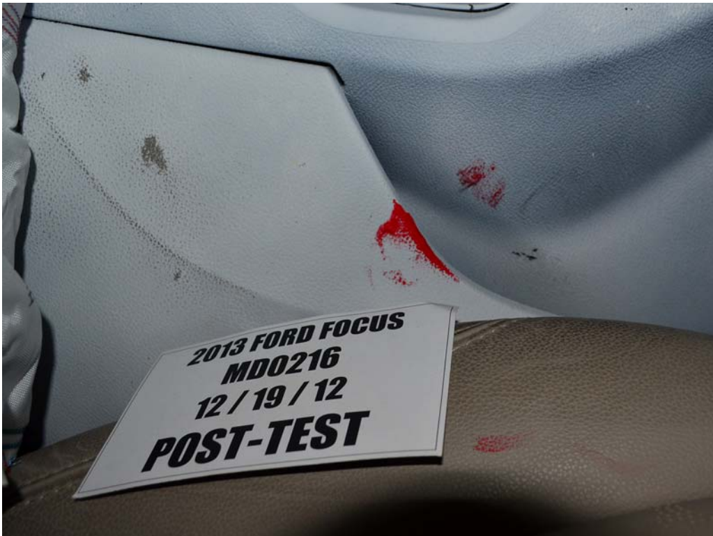
FIGURE 52. Post-Test Driver Dummy Close-Up Pelvis Contact View
