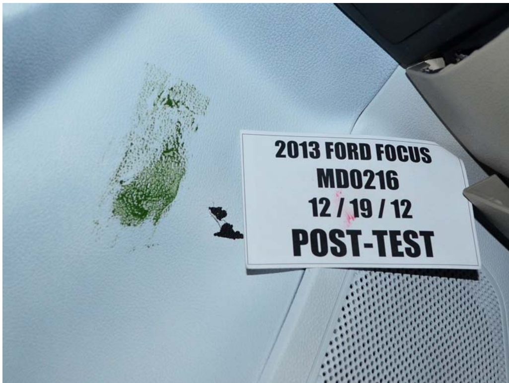
FIGURE 54. Post-Test Driver Dummy Close-Up Knee Contact View
