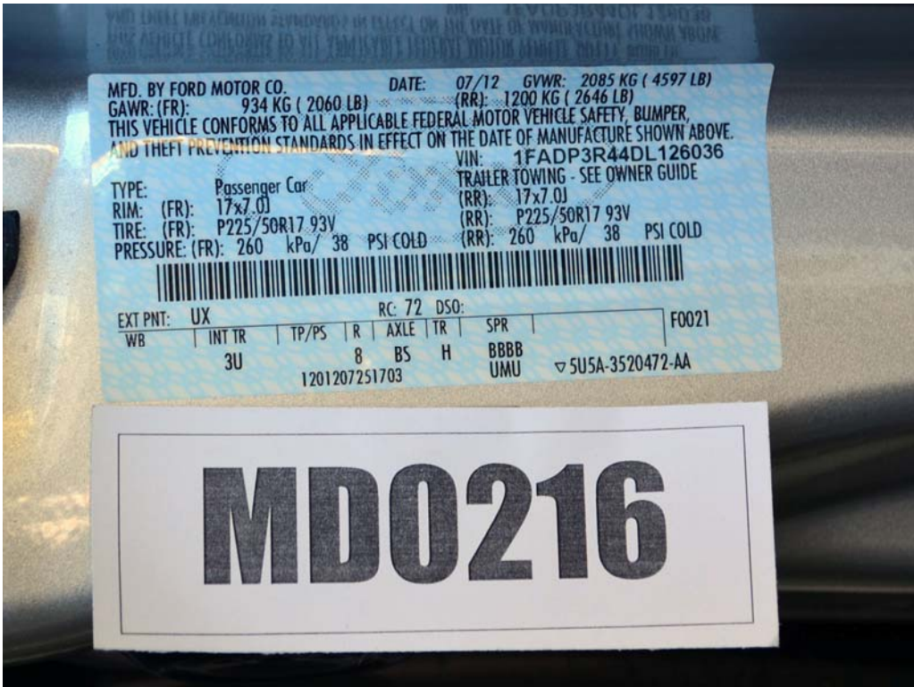
FIGURE 92. Close-Up View of Vehicle's Certification Label
