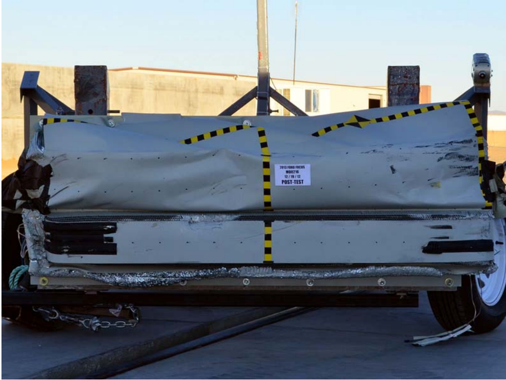
FIGURE 85. Post-Test Front View of MDB Impactor Face
