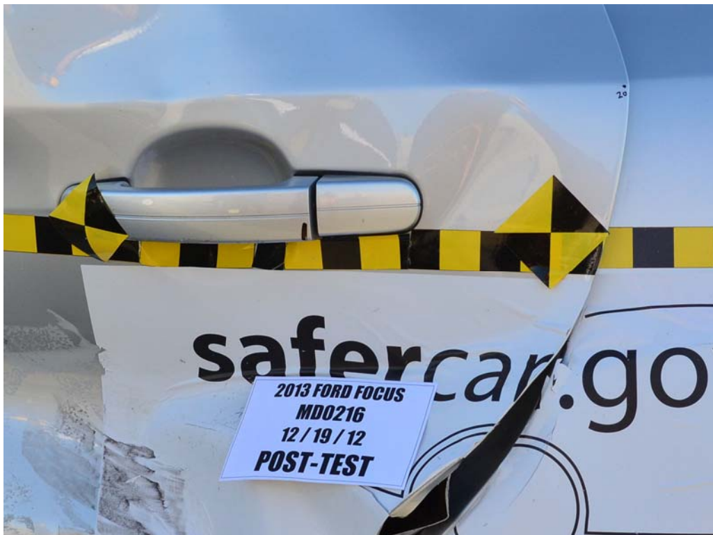
FIGURE 24. Post-Test Left Rear Door Latch Close-Up
