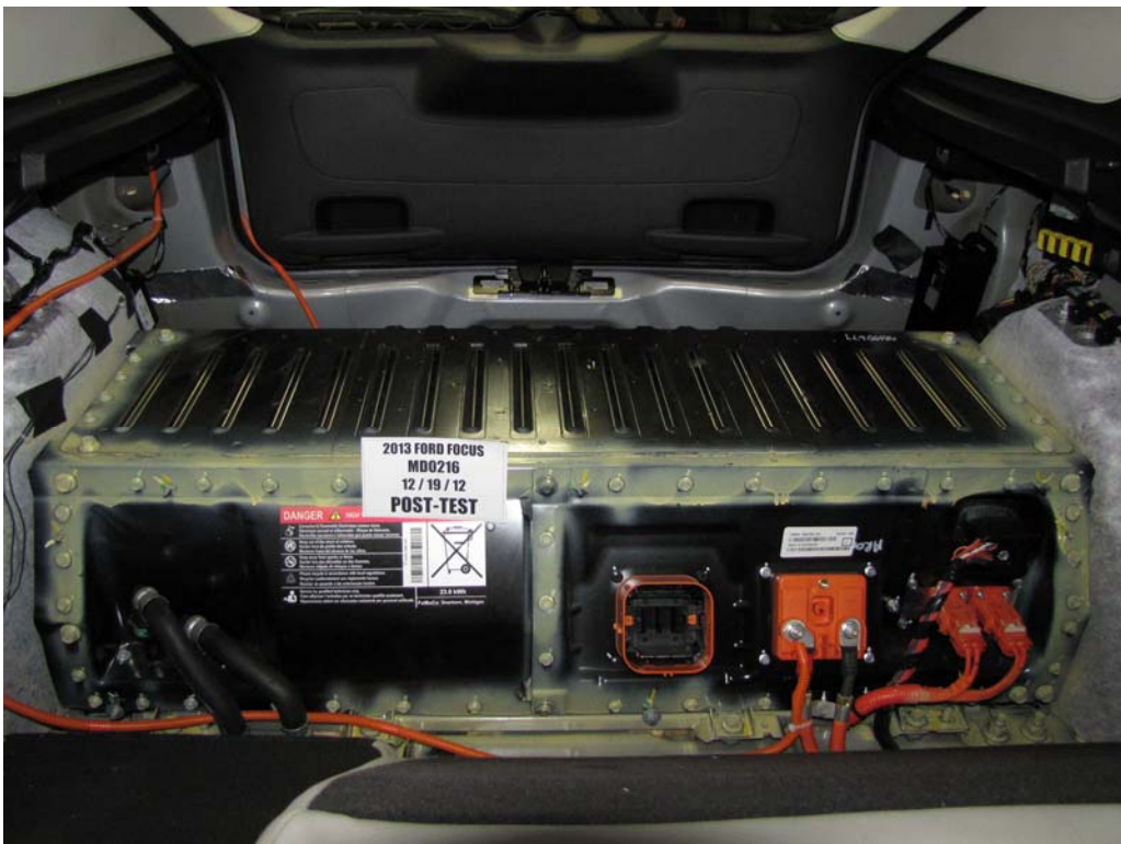
FIGURE 10. Post-Impact Front View of Propulsion Battery
