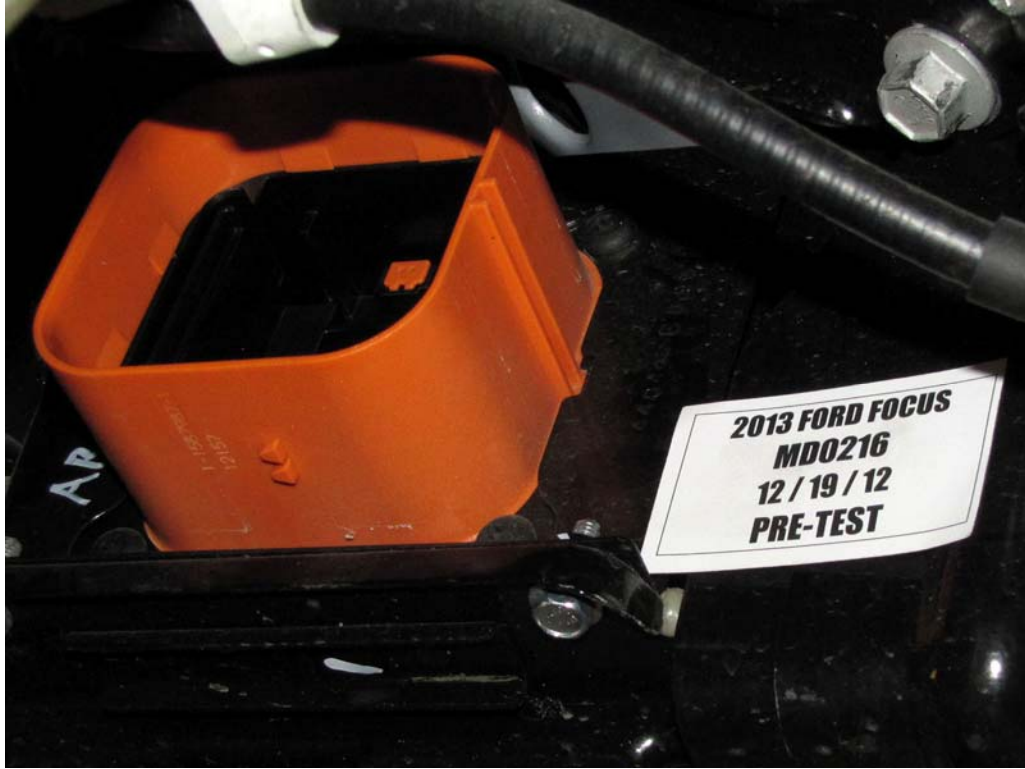
FIGURE 7a. Manual High Voltage Disconnect Removed
