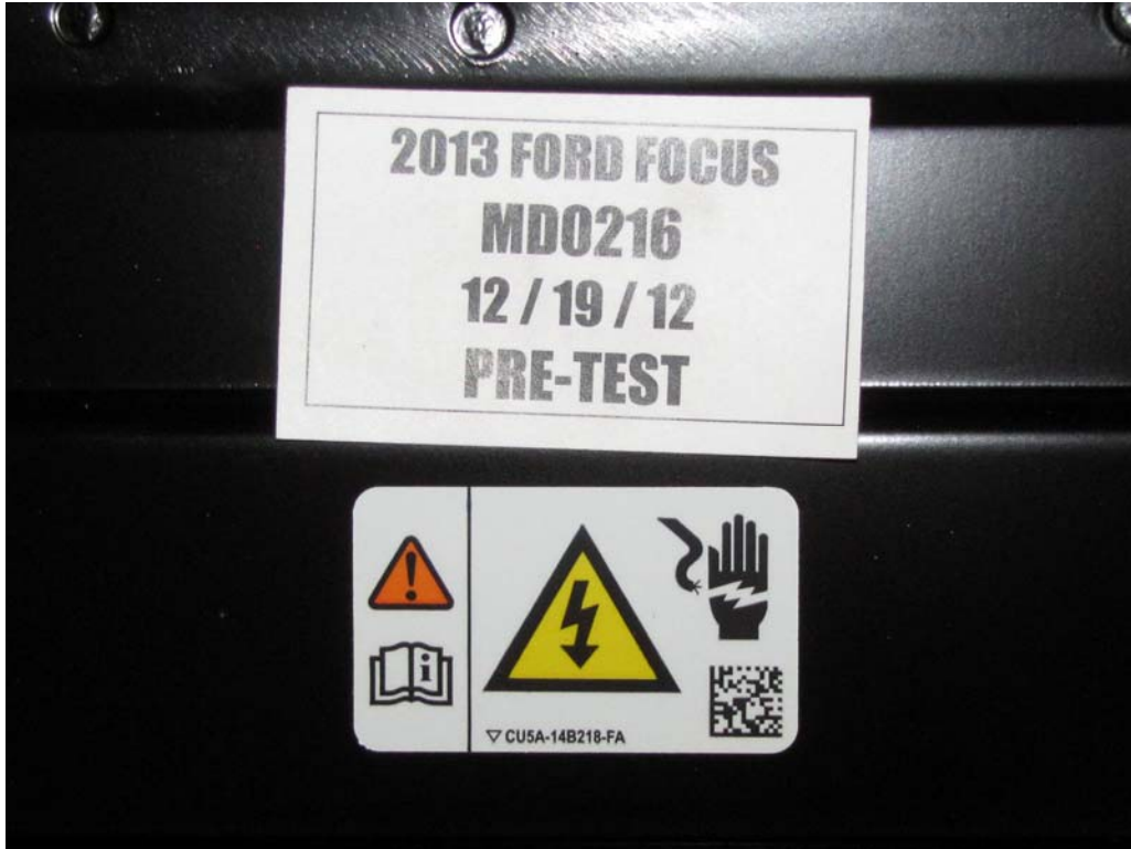
FIGURE 1. Auxiliary Power Module Warning Label
