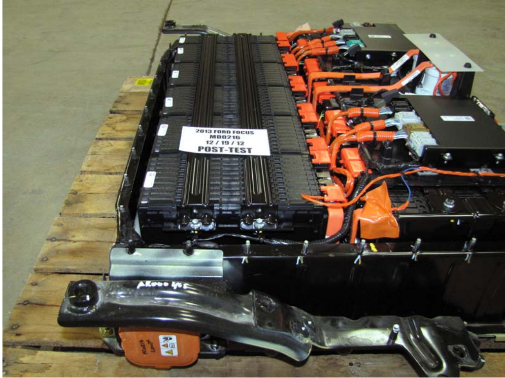
FIGURE 15c. Post-Impact View of Battery Modules
