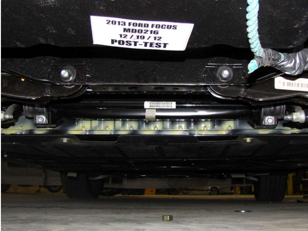
FIGURE 11a. Post-Impact Rear View of Propulsion Battery
