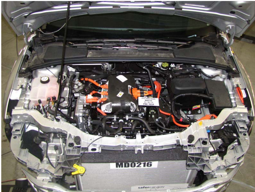
FIGURE 16. Pre-Impact View of Electric Propulsion Drive
