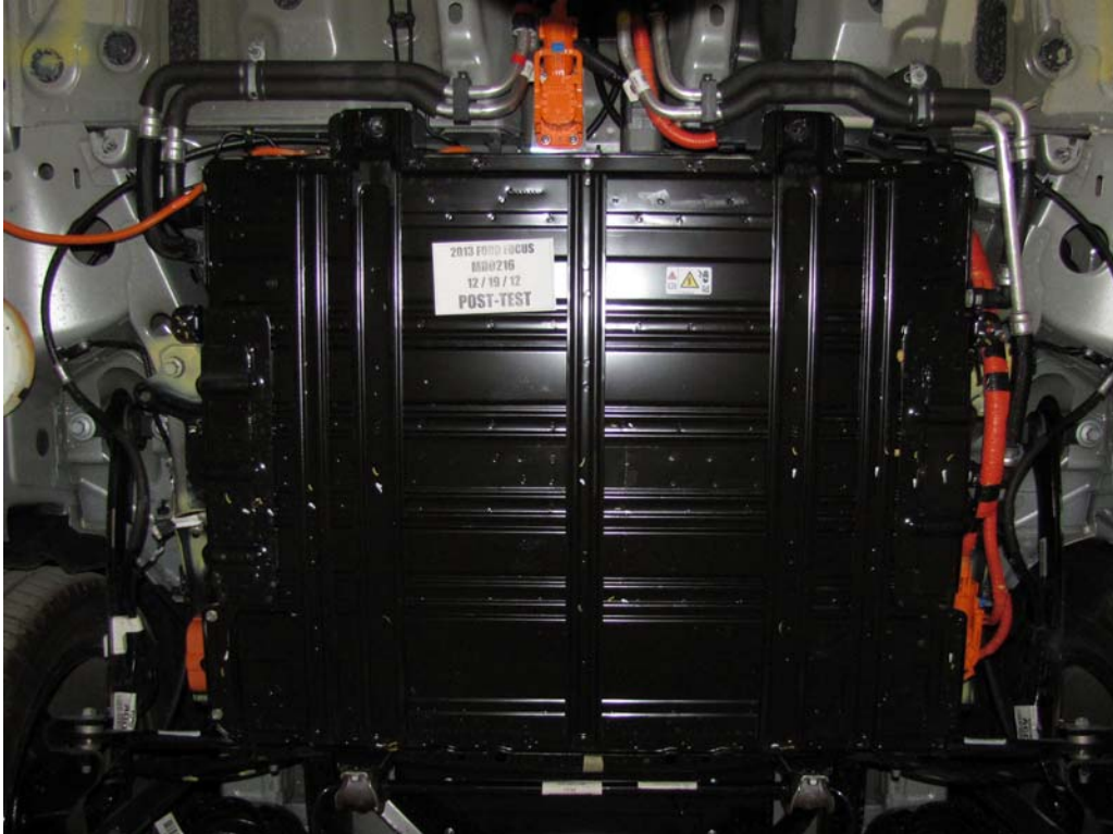
FIGURE 10a. Post-Impact Front View of Propulsion Battery
