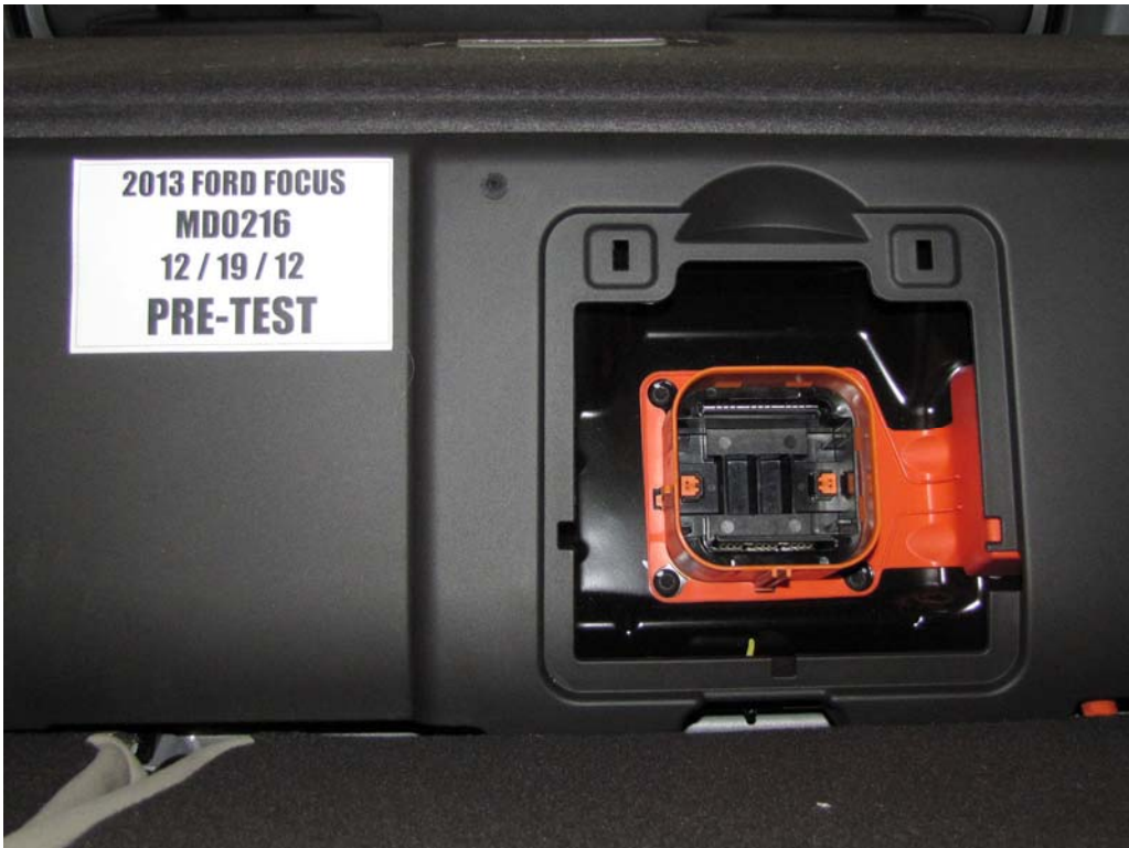
FIGURE 7. Manual High Voltage Disconnect Removed
