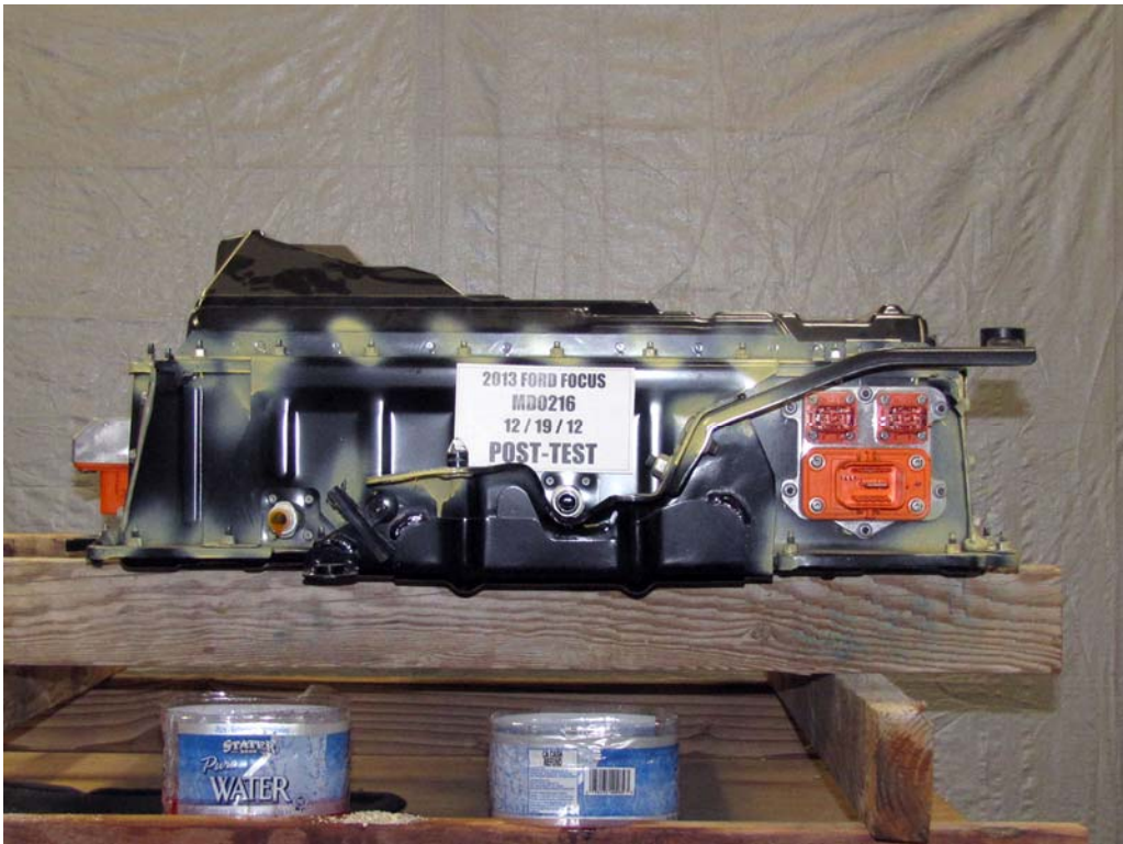
FIGURE 13c. Post-Impact View of Battery Box or Container Which hold Individual Battery Modules
