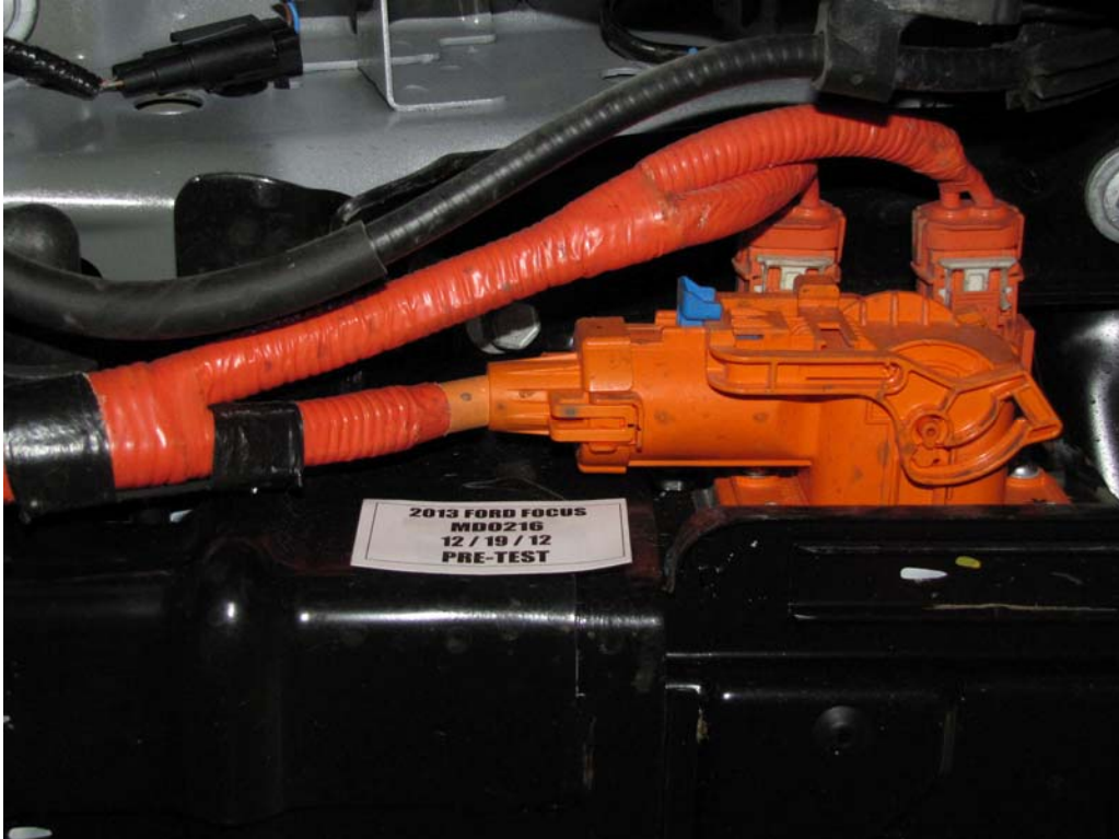
FIGURE 18c. Pre-Impact View of High Voltage Interconnect(s)
