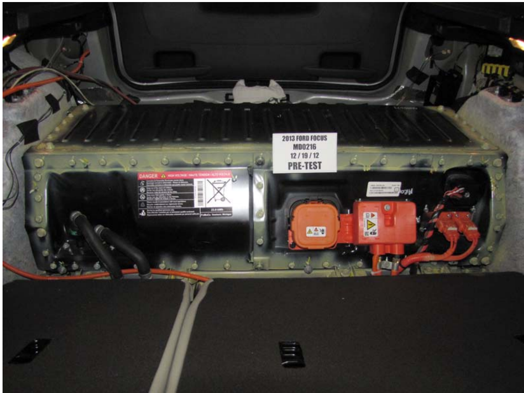
FIGURE 9. Pre-Impact View of Propulsion Battery
