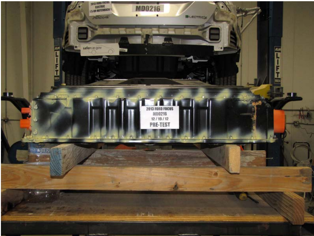
FIGURE 12f. Pre-Impact View of Battery Box or Container Which hold Individual Battery Modules
