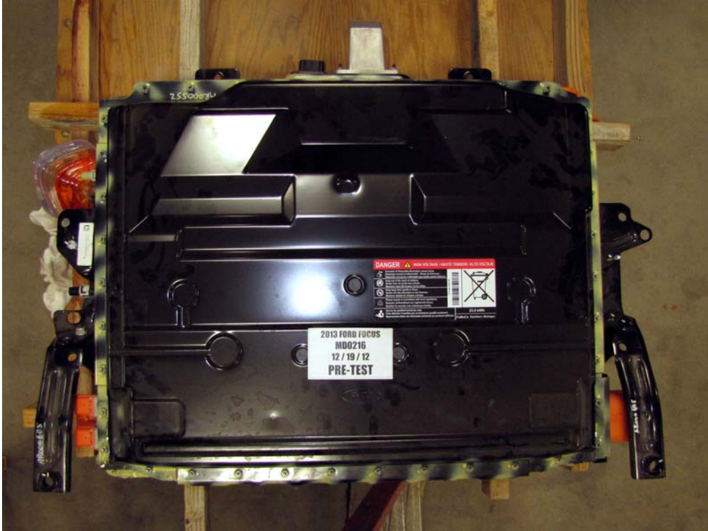
FIGURE 12a. Pre-Impact View of Battery Box or Container Which hold Individual Battery Modules
