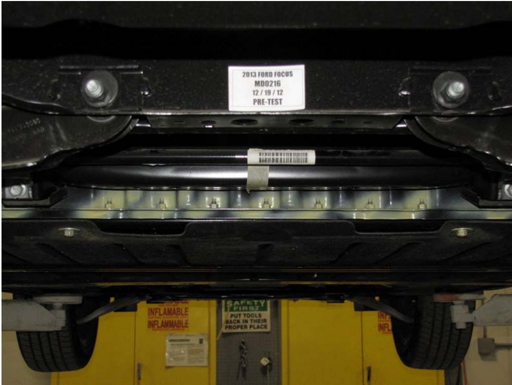
FIGURE 9c. Pre-Impact View of Propulsion Battery
