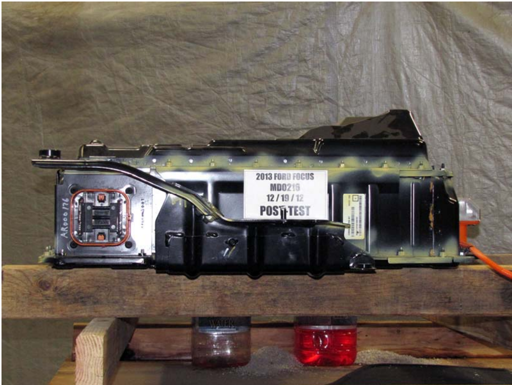
FIGURE 13e. Post-Impact View of Battery Box or Container Which hold Individual Battery Modules
