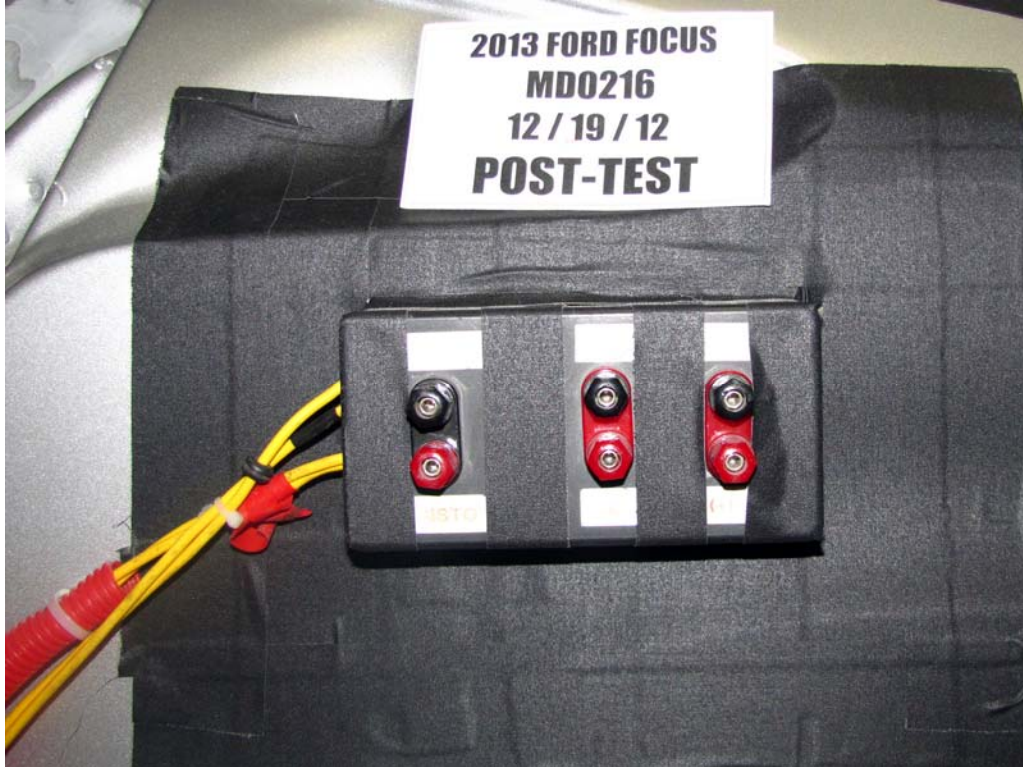
FIGURE 25. Post-Impact View of Installed Test Interface Port
