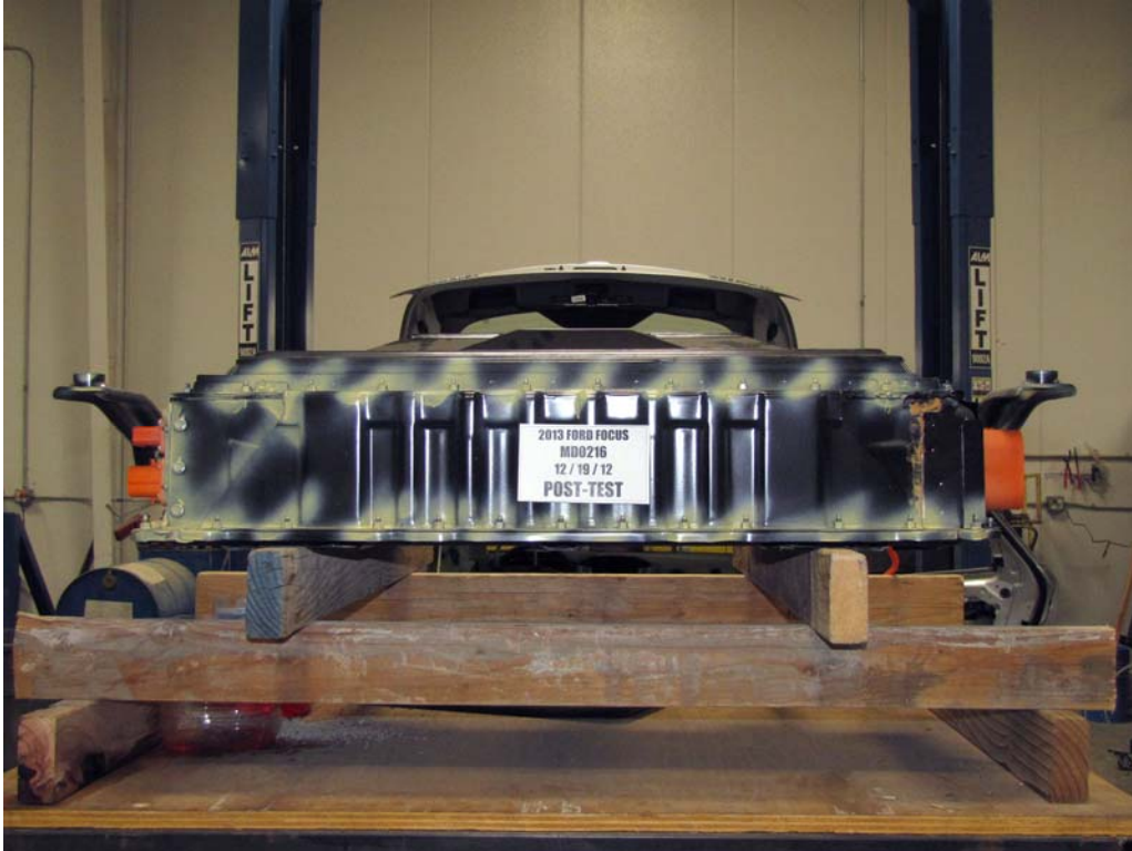
FIGURE 13f. Post-Impact View of Battery Box or Container Which hold Individual Battery Modules
