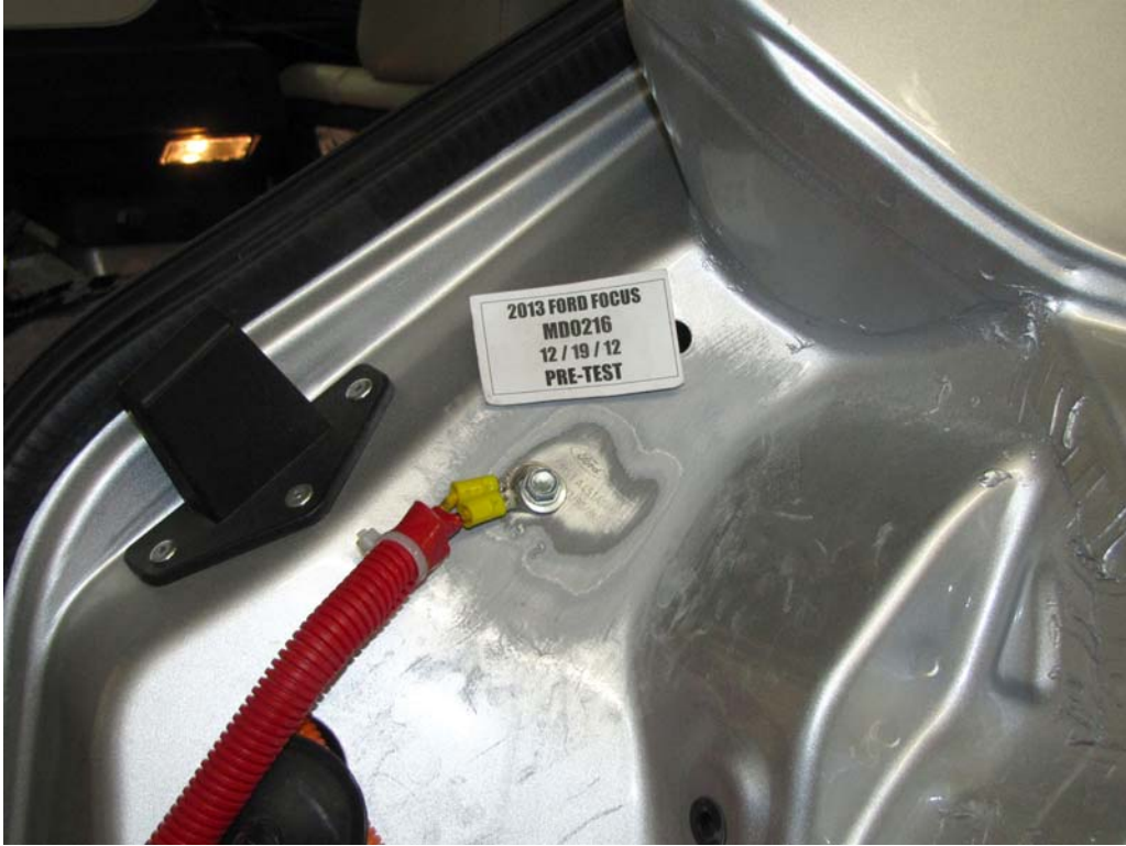
FIGURE 21. Pre-Impact View of Ground Lead Attached
