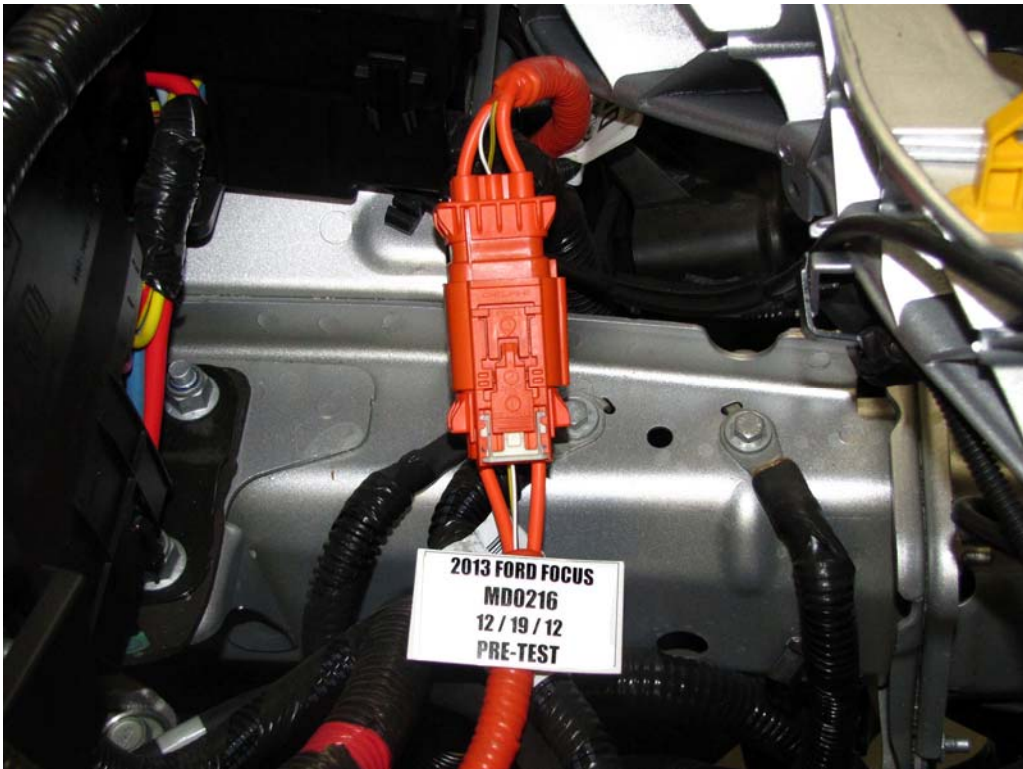
FIGURE 18. Pre-Impact View of High Voltage Interconnect(s)
