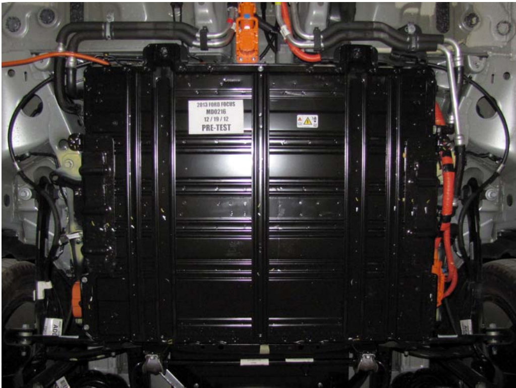
FIGURE 9b. Pre-Impact View of Propulsion Battery
