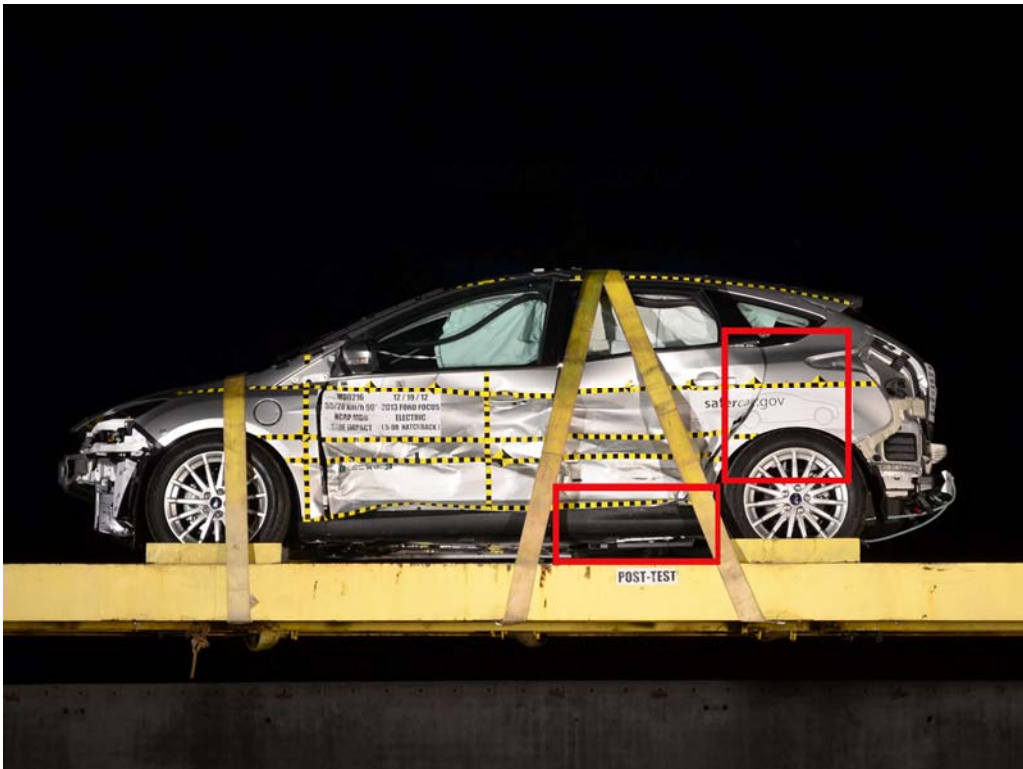
FIGURE 32. FMVSS No. 305 Static Rollover at 360°
