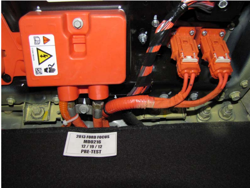
FIGURE 18a. Pre-Impact View of High Voltage Interconnect(s)
