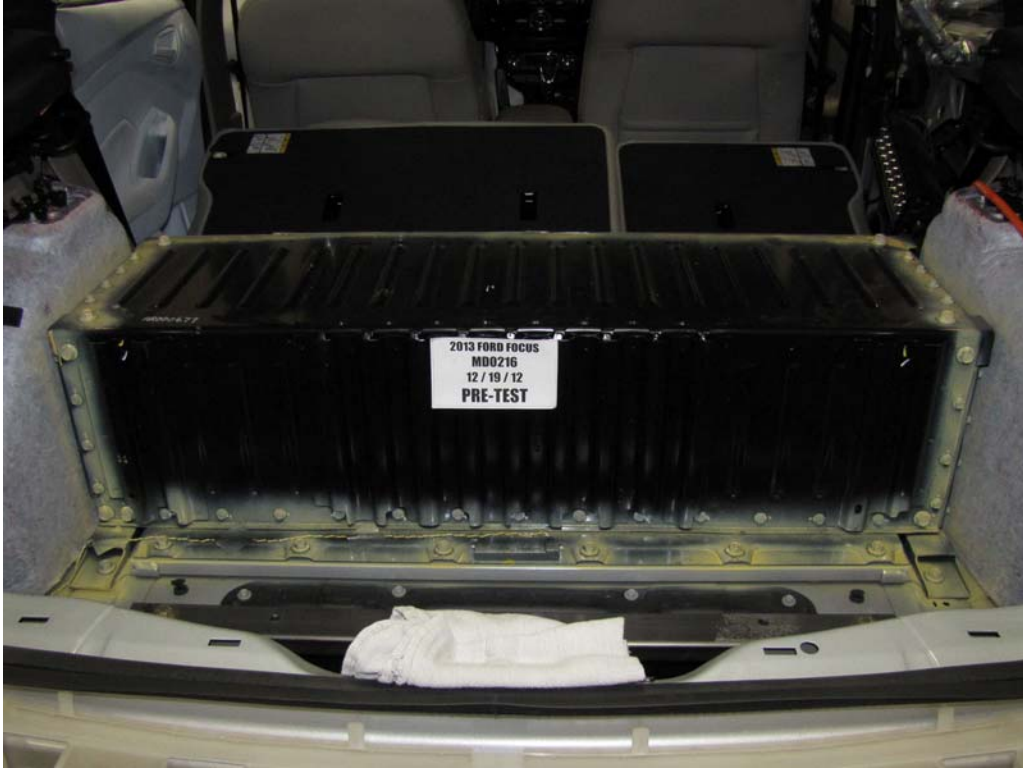
FIGURE 9a. Pre-Impact View of Propulsion Battery
