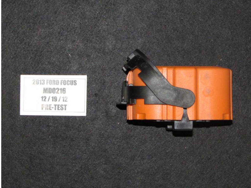
FIGURE 8a. Manual High Voltage Disconnect Removed
