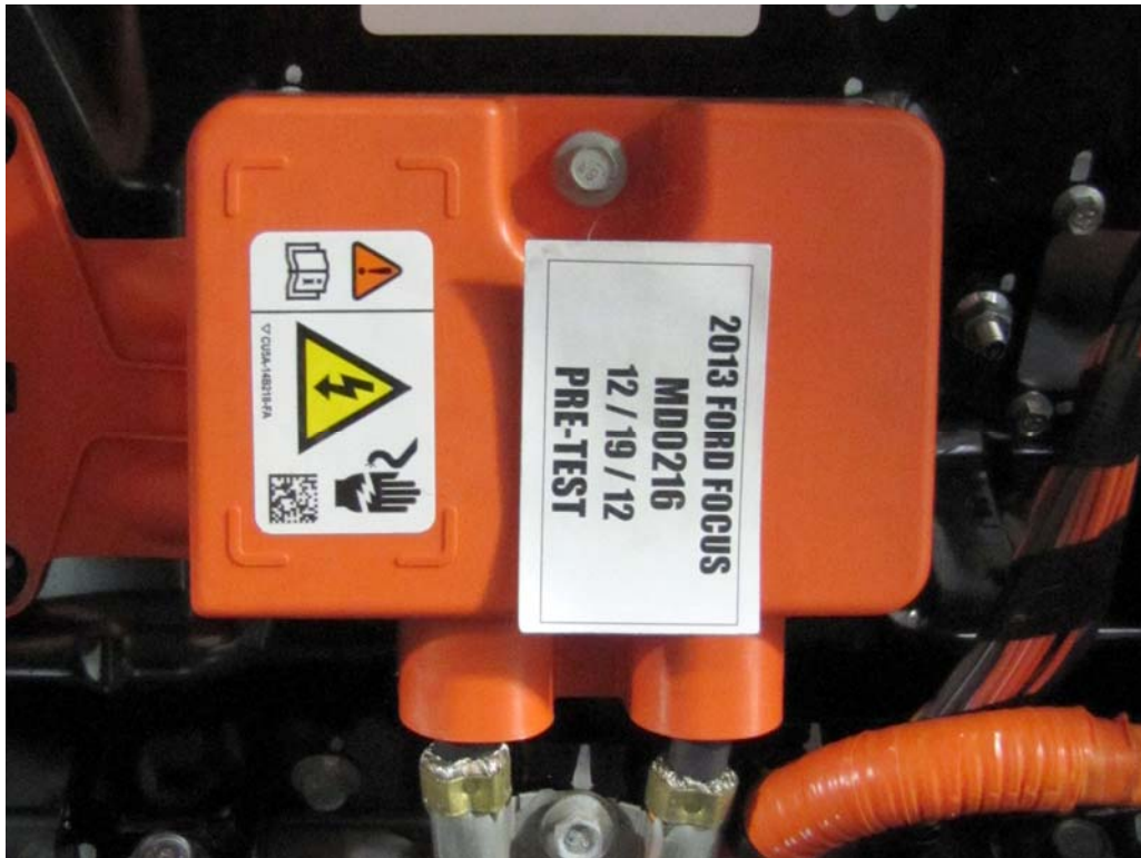
FIGURE 1c. Auxiliary Power Module Warning Label
