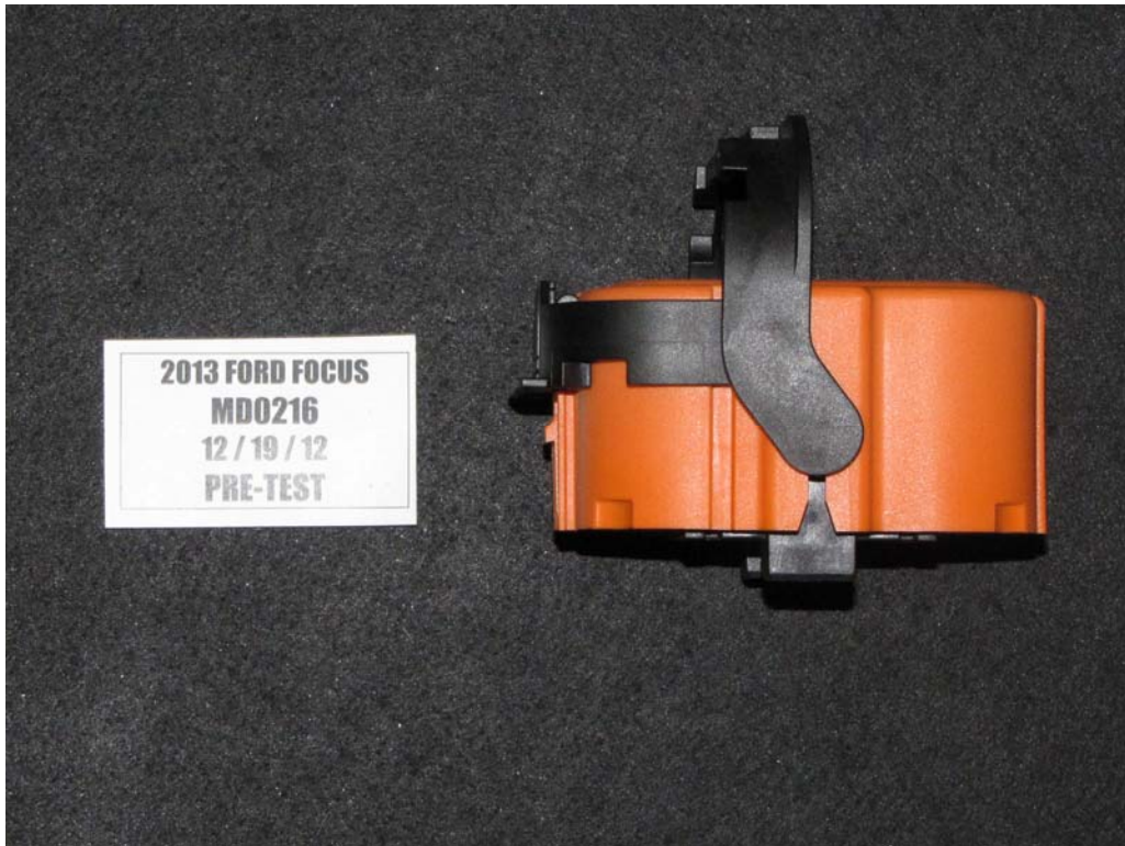
FIGURE 8. Manual High Voltage Disconnect Removed
