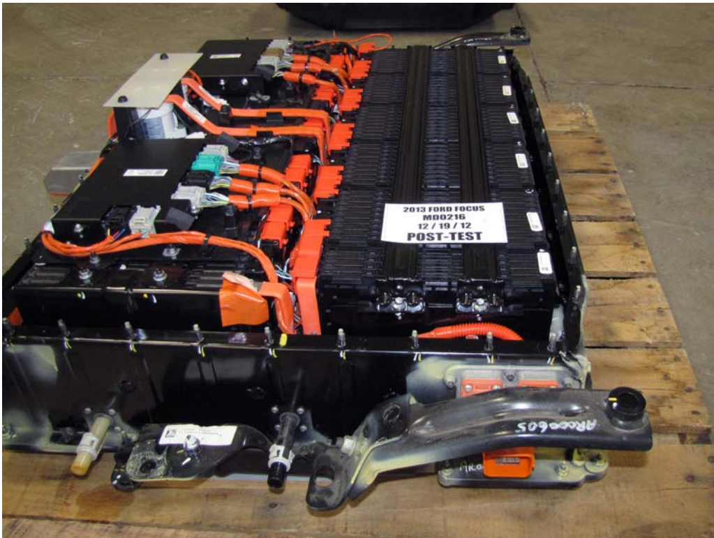
FIGURE 15b. Post-Impact View of Battery Modules
