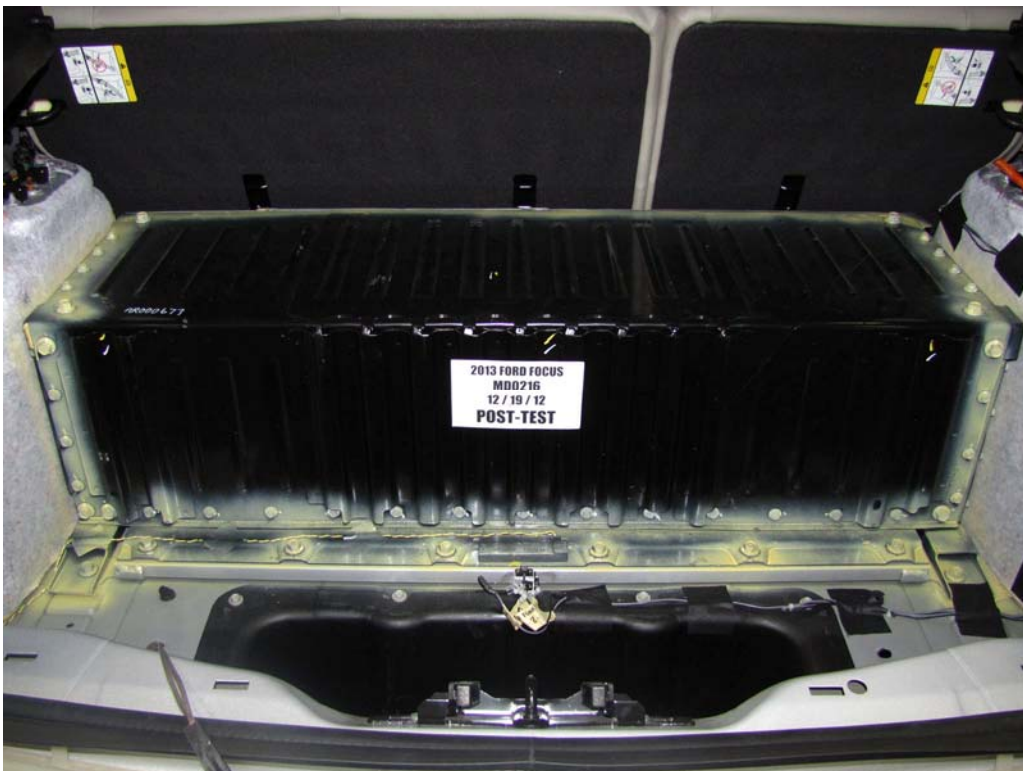
FIGURE 11. Post-Impact Rear View of Propulsion Battery
