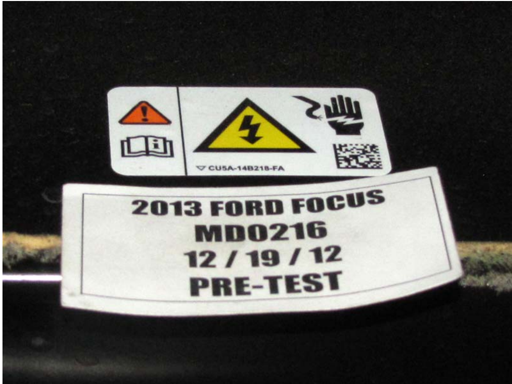
FIGURE 5c. Other Vehicle Label Related to Electrical Propulsion System
