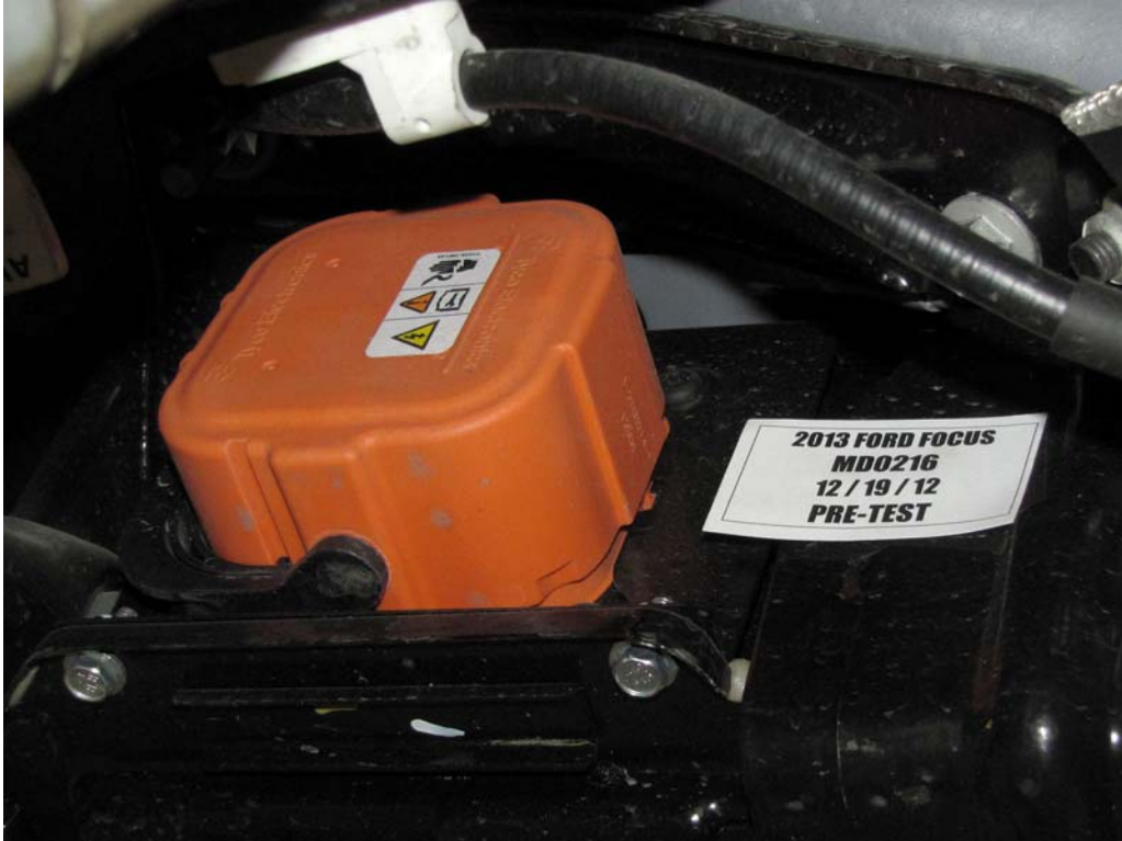
FIGURE 6a. Manual High Voltage Disconnect In Place
