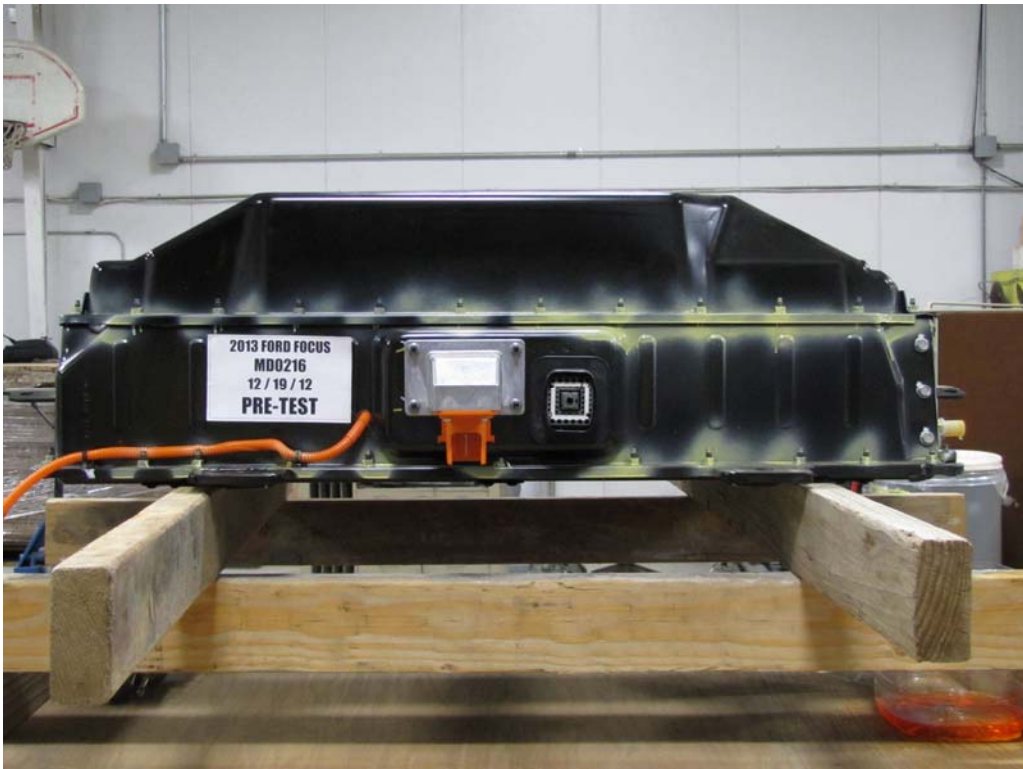
FIGURE 12d. Pre-Impact View of Battery Box or Container Which hold Individual Battery Modules
