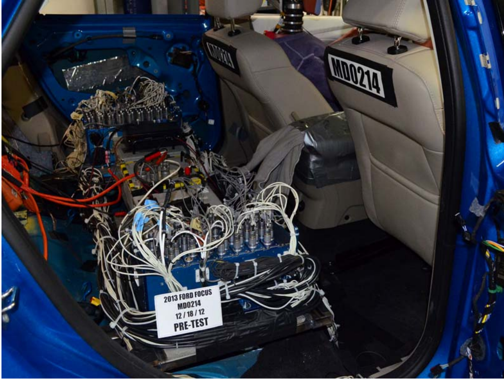
FIGURE 27. Pre-Test Dummy Cable Routing
