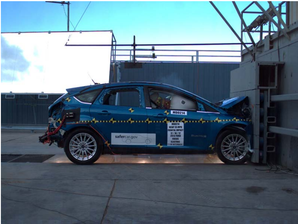
FIGURE 75. 2013 Ford Focus Electric Frontal Impact Event
