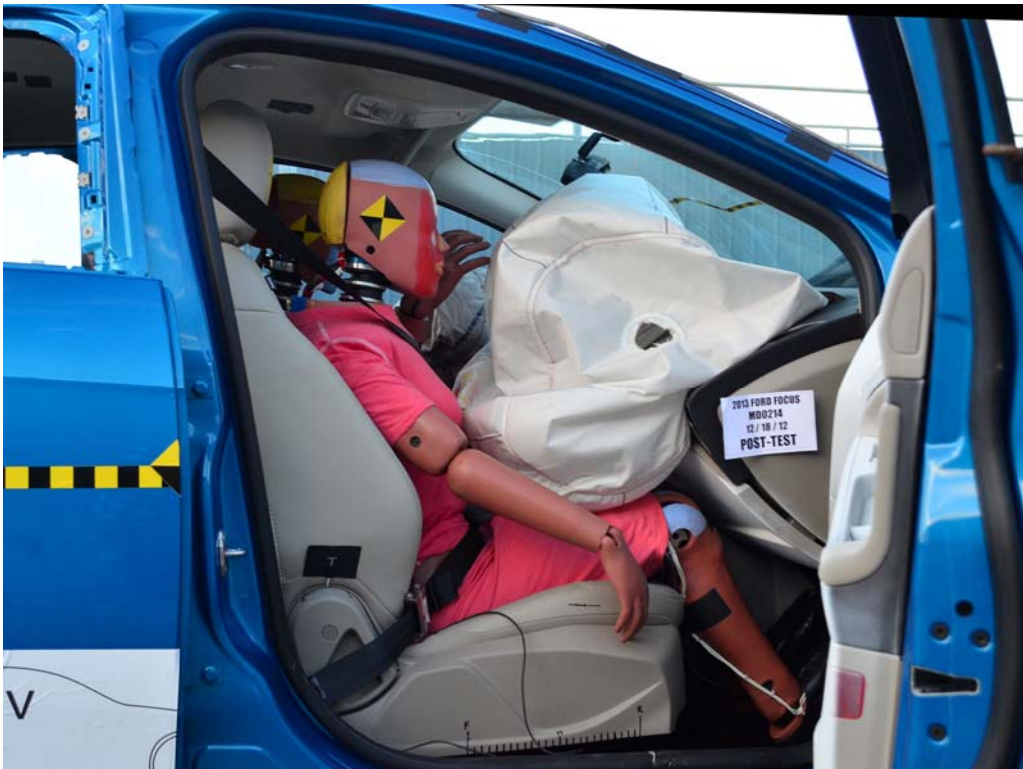
FIGURE 55. Post-Test Passenger Dummy and Vehicle Interior View
