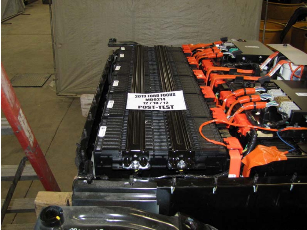
FIGURE 15c. Post-Impact View of Battery Modules
