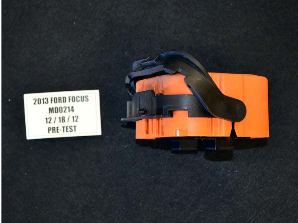
FIGURE 8a. Manual High Voltage Disconnect Removed
