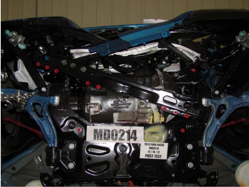
FIGURE 17a. Post-Impact View of Electric Propulsion Drive
