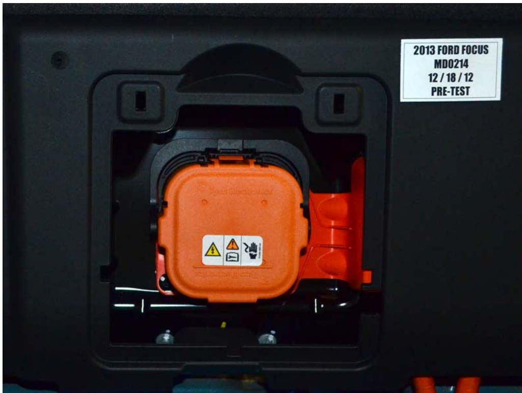
FIGURE 6. Manual High Voltage Disconnect In Place
