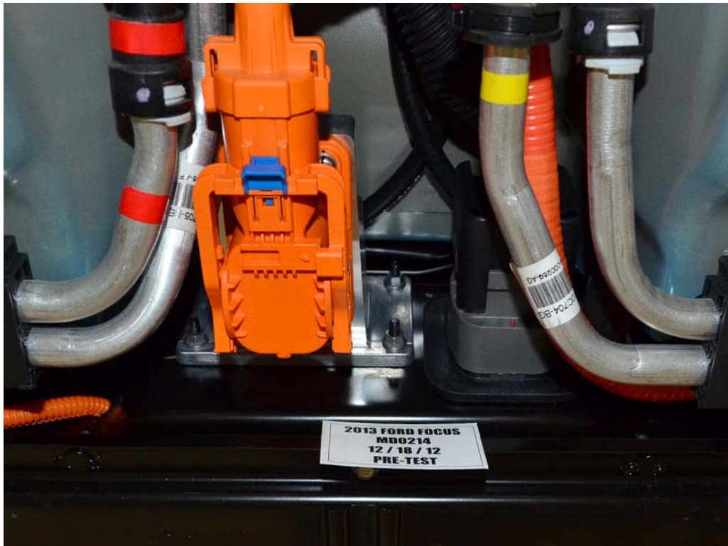
FIGURE 18b. Pre-Impact View of High Voltage Interconnect(s)
