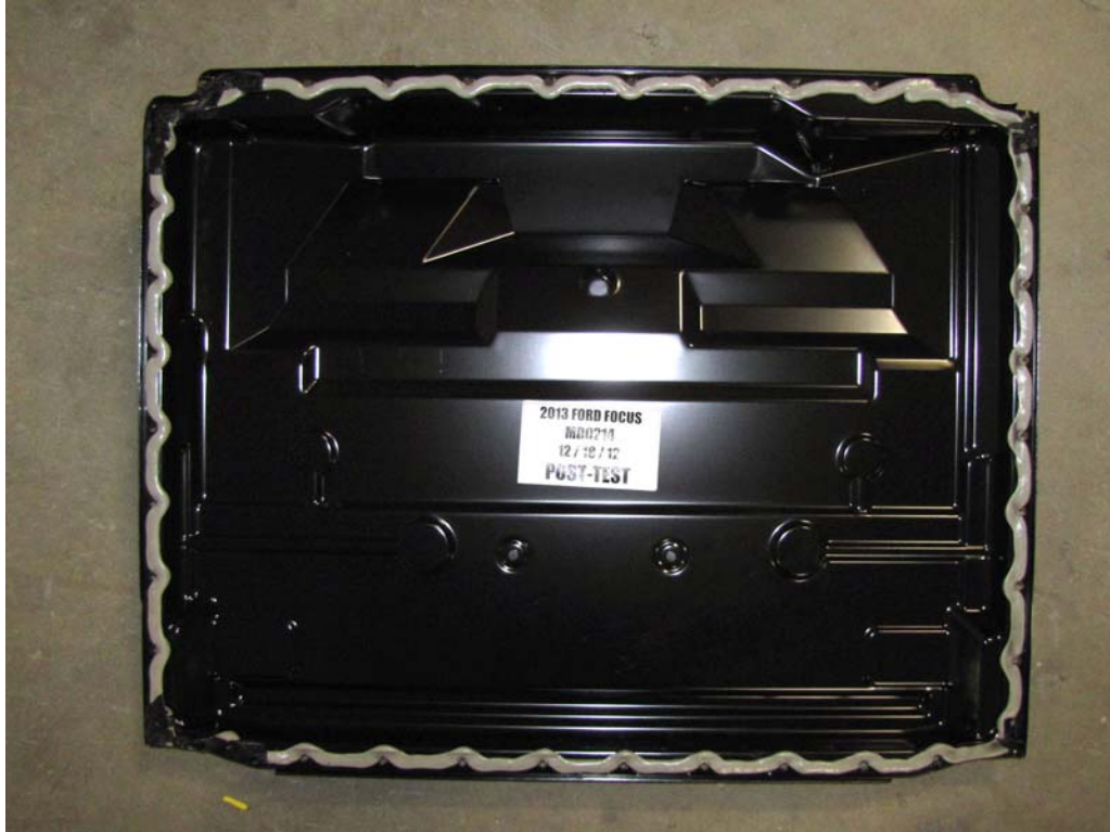
FIGURE 13b. Post-Impact View of Battery Box or Container Which hold Individual Battery Modules
