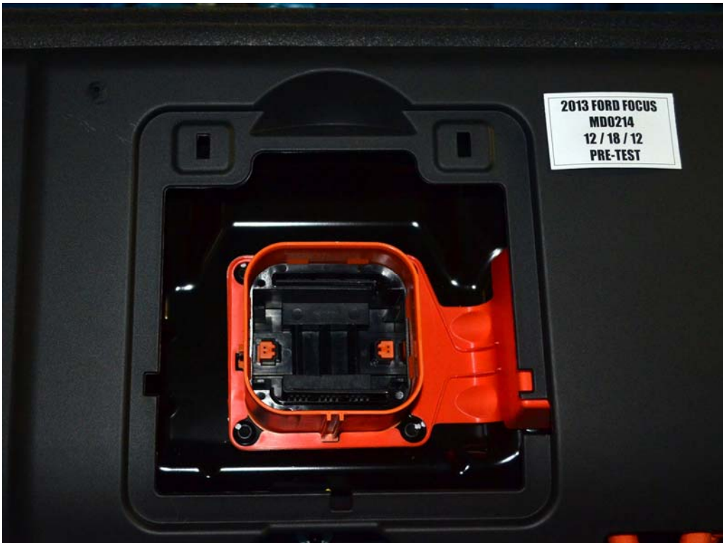
FIGURE 7. Manual High Voltage Disconnect Removed
