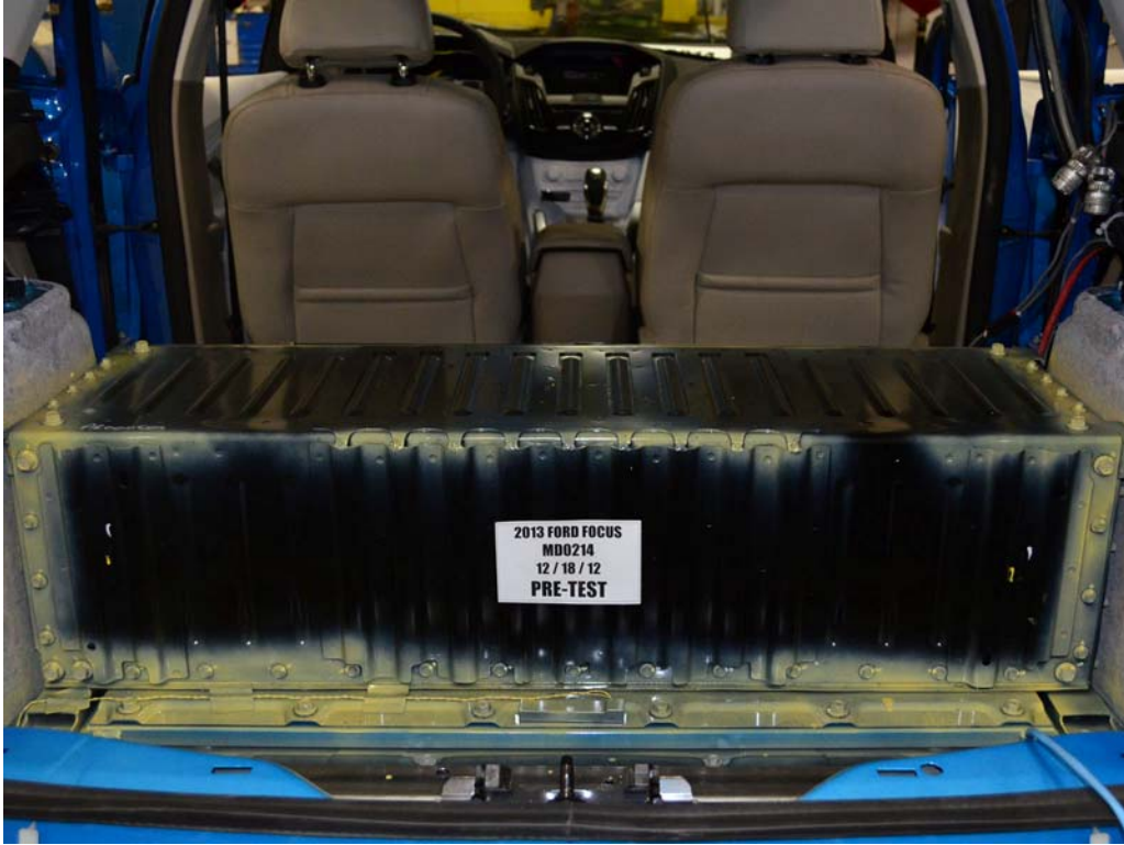
FIGURE 9a. Pre-Impact View of Propulsion Battery
