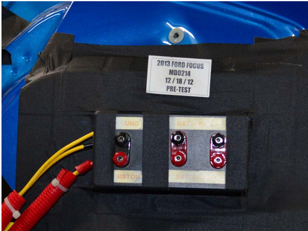
FIGURE 24. Pre-Impact View of Installed Test Interface Port
