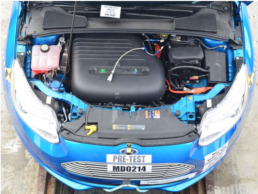
FIGURE 16. Pre-Impact View of Electric Propulsion Drive
