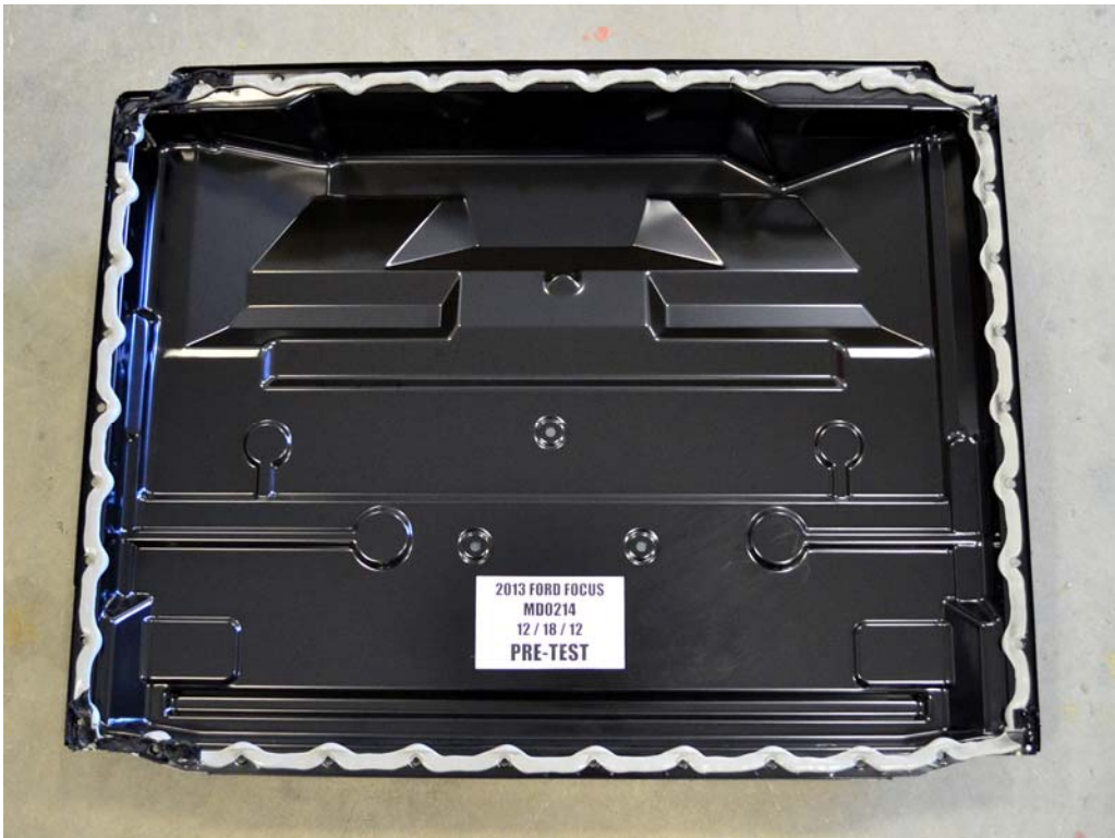
FIGURE 12b. Pre-Impact View of Battery Box or Container Which hold Individual Battery Modules
