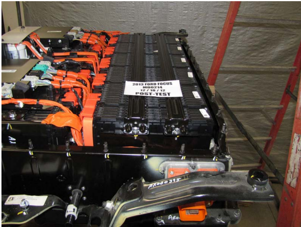
FIGURE 15b. Post-Impact View of Battery Modules
