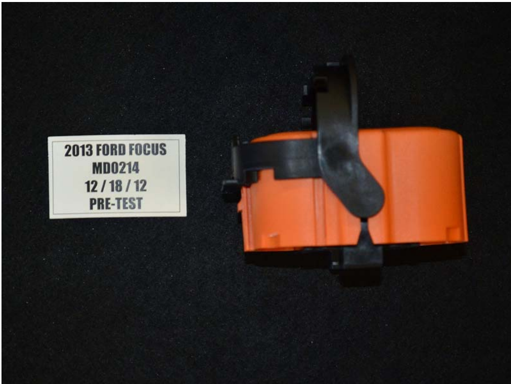
FIGURE 8. Manual High Voltage Disconnect Removed
