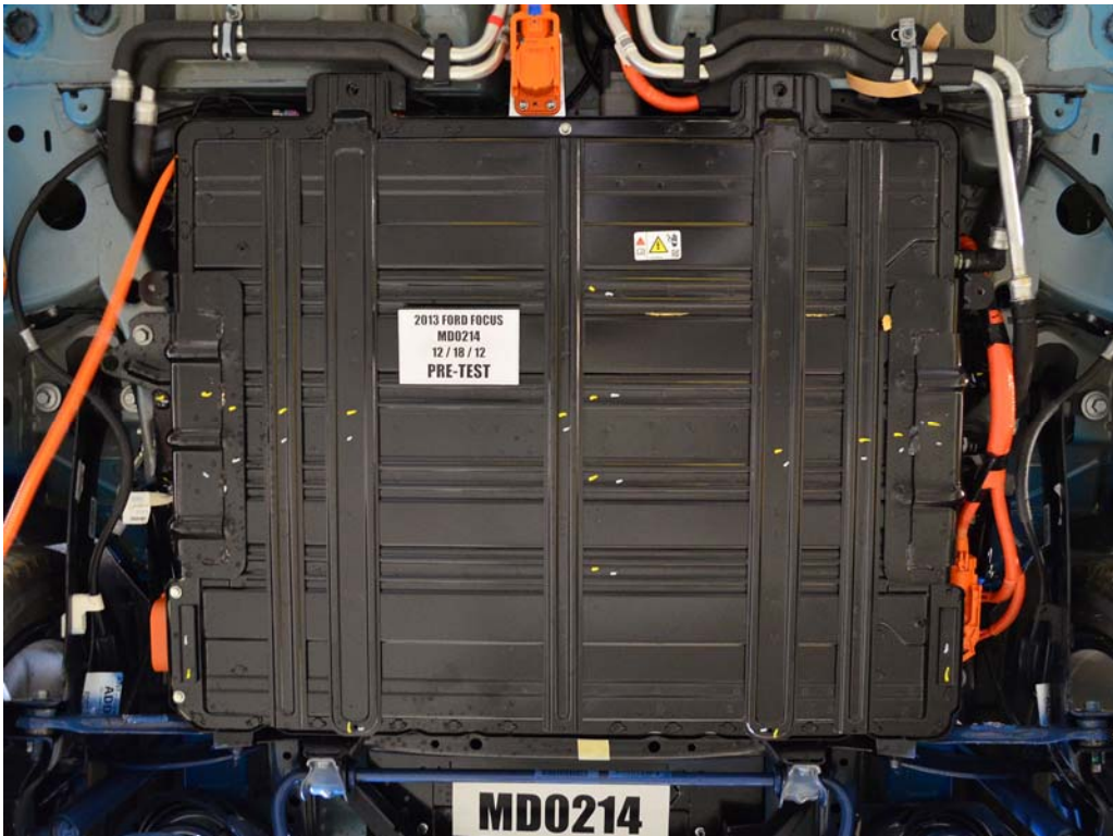
FIGURE 9b. Pre-Impact View of Propulsion Battery
