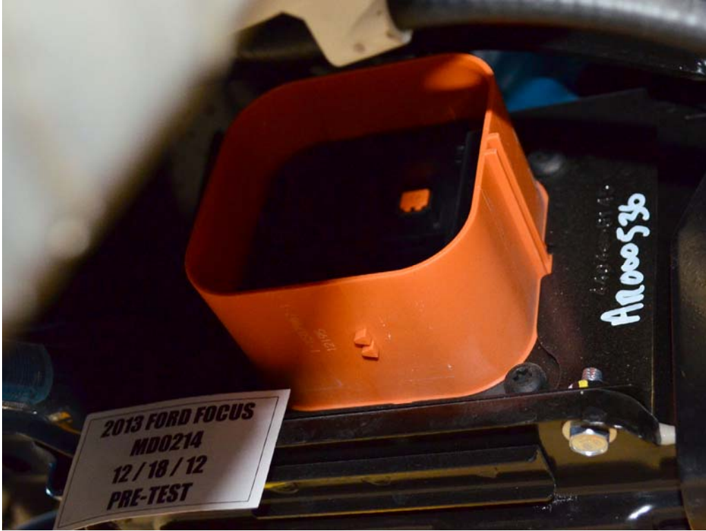
FIGURE 7a. Manual High Voltage Disconnect Removed
