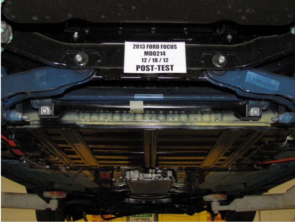
FIGURE 11a. Post-Impact Rear View of Propulsion Battery
