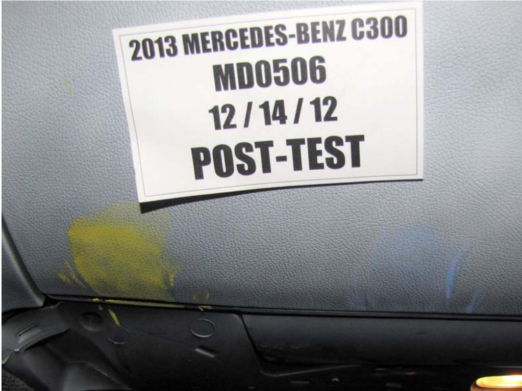
FIGURE 66b. Post-Test Passenger Dummy Contact With Glovebox
