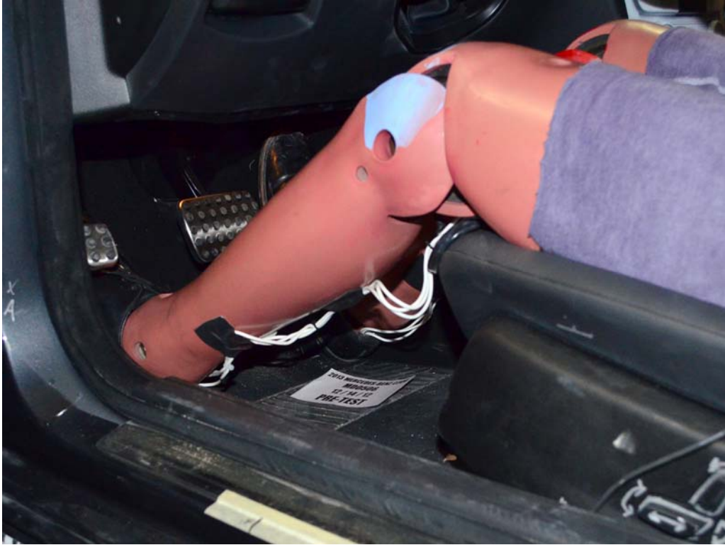
FIGURE 39. Pre-Test Driver Dummy Feet
