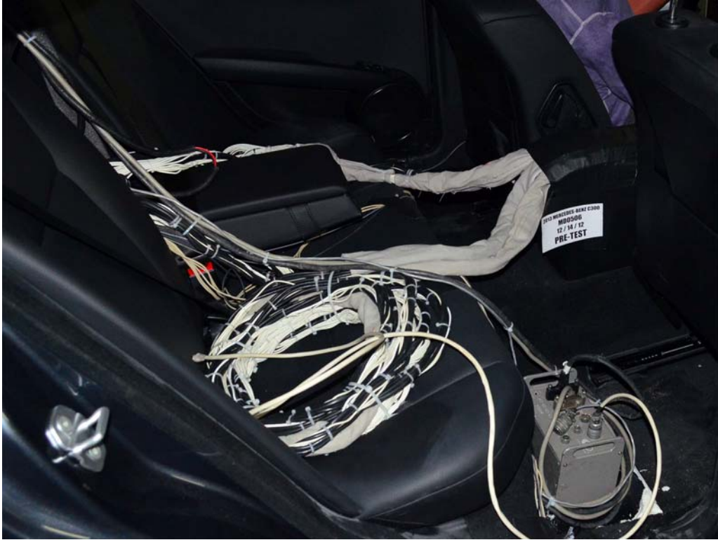
FIGURE 27. Pre-Test Dummy Cable Routing
