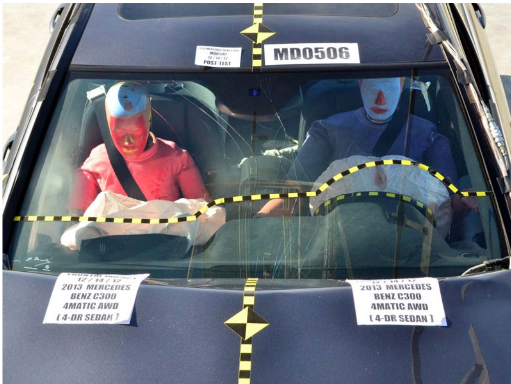
FIGURE 18. Post-Test Windshield View
