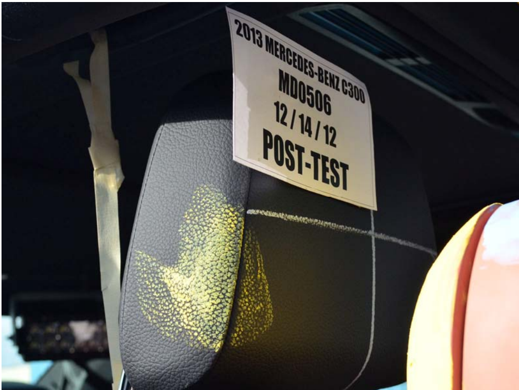
FIGURE 66a. Post-Test Passenger Dummy Contact With Headrest
