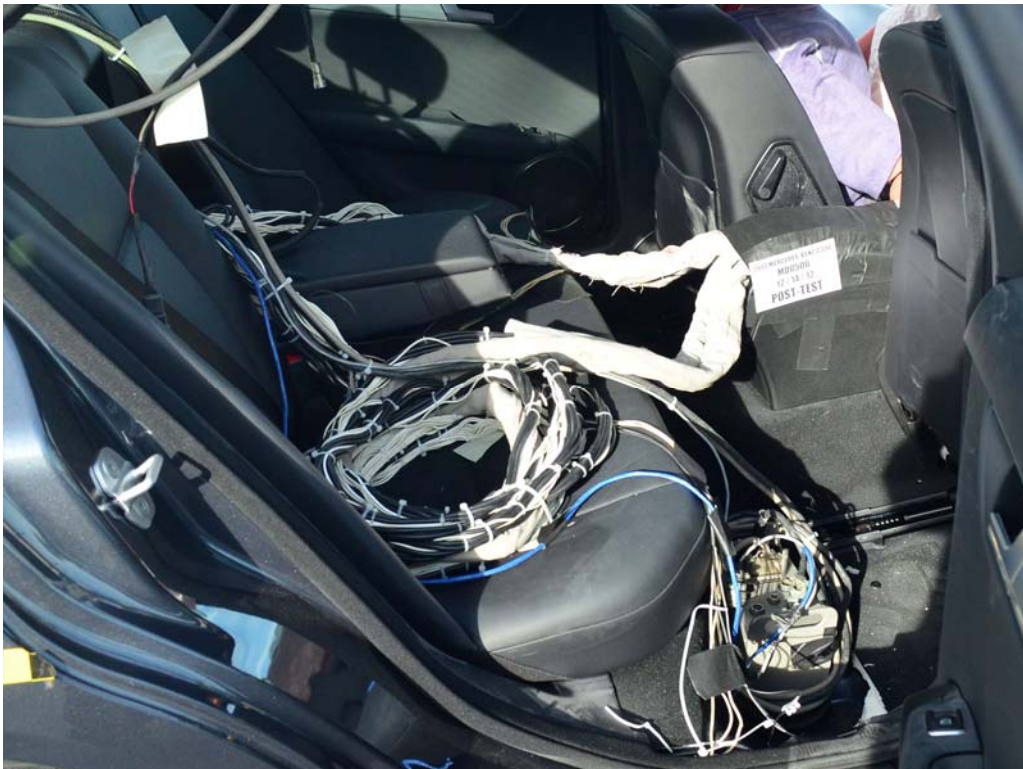
FIGURE 28. Post-Test Dummy Cable Routing
