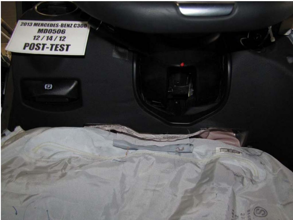
FIGURE 42. Post-Test Driver's Side Knee Bolster
