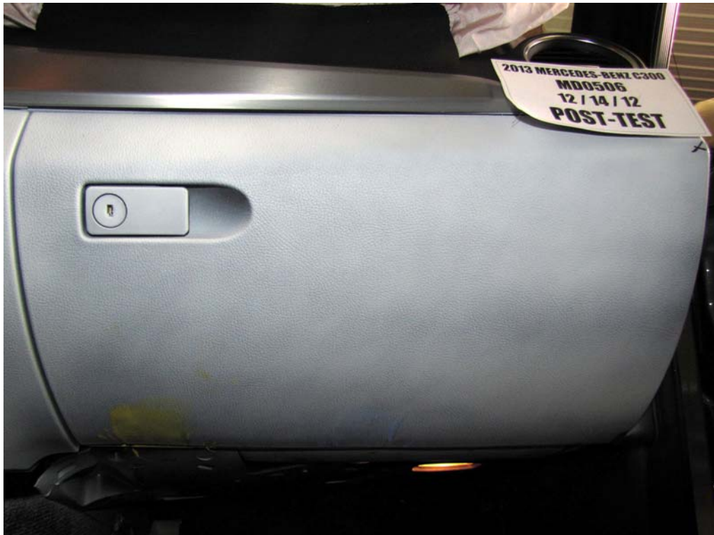
FIGURE 63. Post-Test Passenger's Side Knee Bolster
