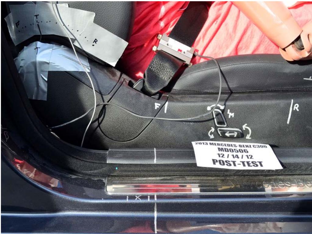
FIGURE 57. Post-Test Passenger's Seat Fore-Aft Markings
