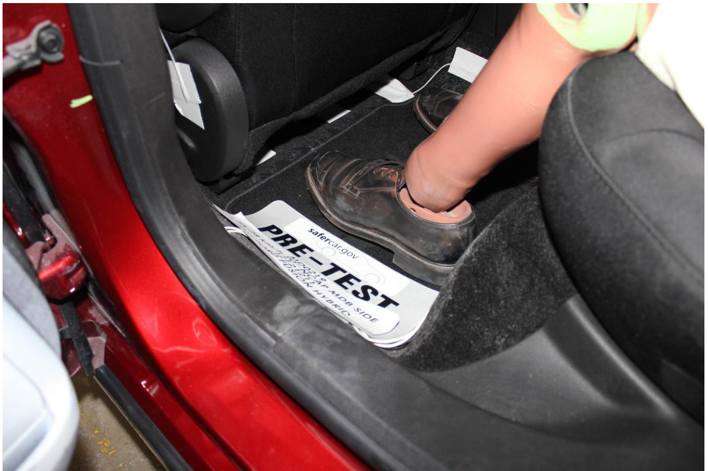
Pre-Test Placement of Rear Passenger Dummy's Feet
