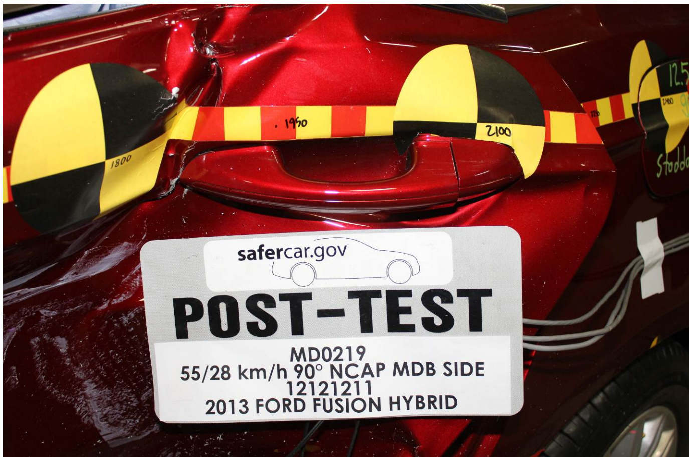
Post-Test Left Rear Door Latch Close-Up
