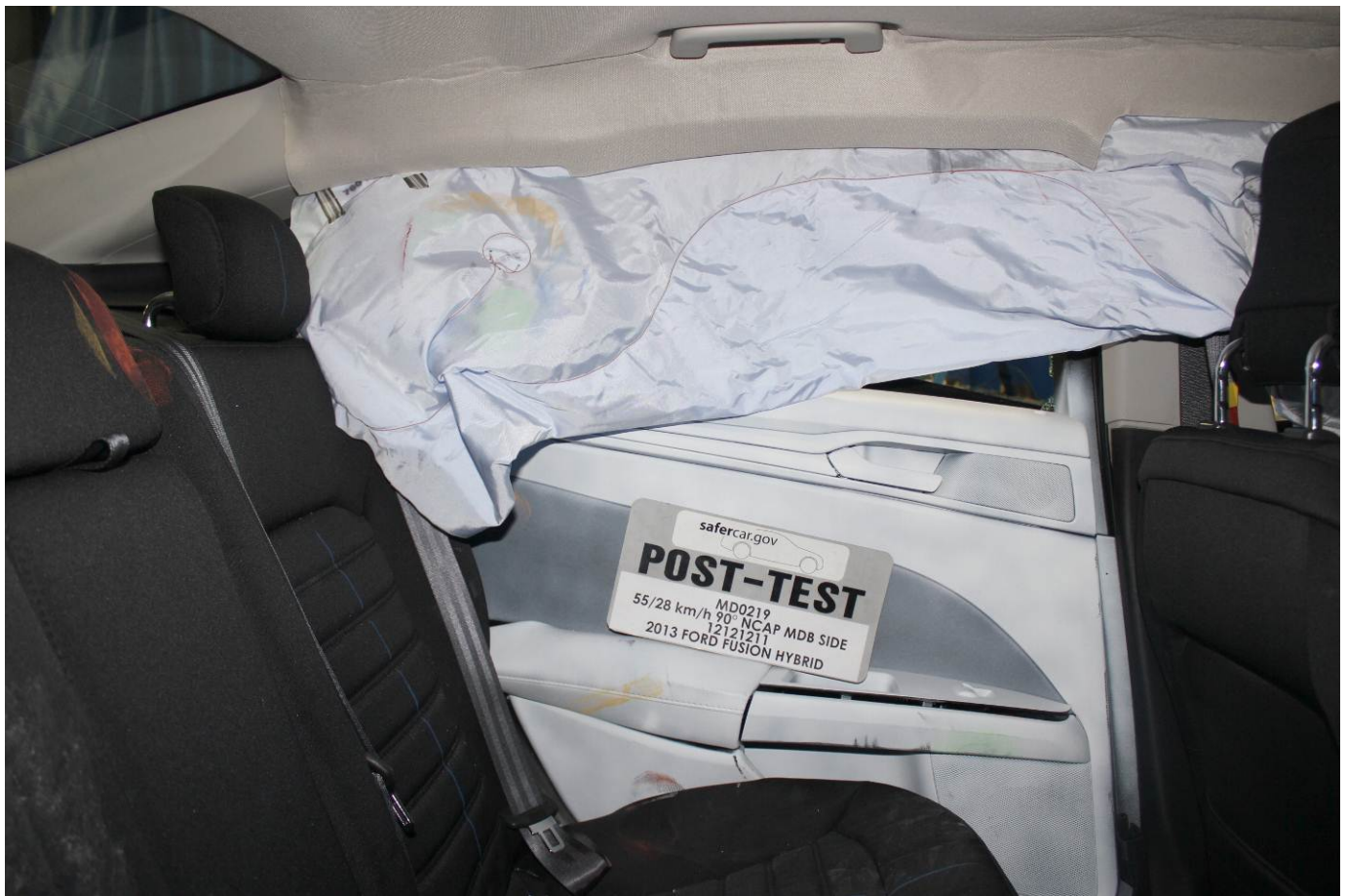
Post-Test Rear Passenger Inner Door Panel View
