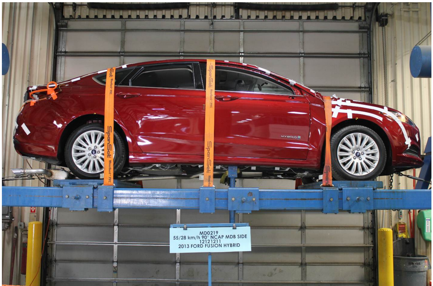
FMVSS No. 301 Static Rollover 0 Degrees
