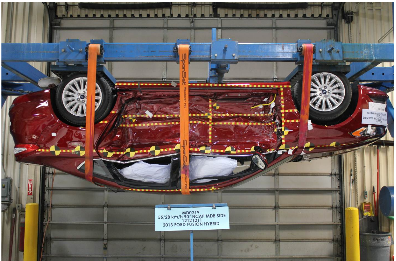
FMVSS No. 301 Static Rollover 180 Degrees
