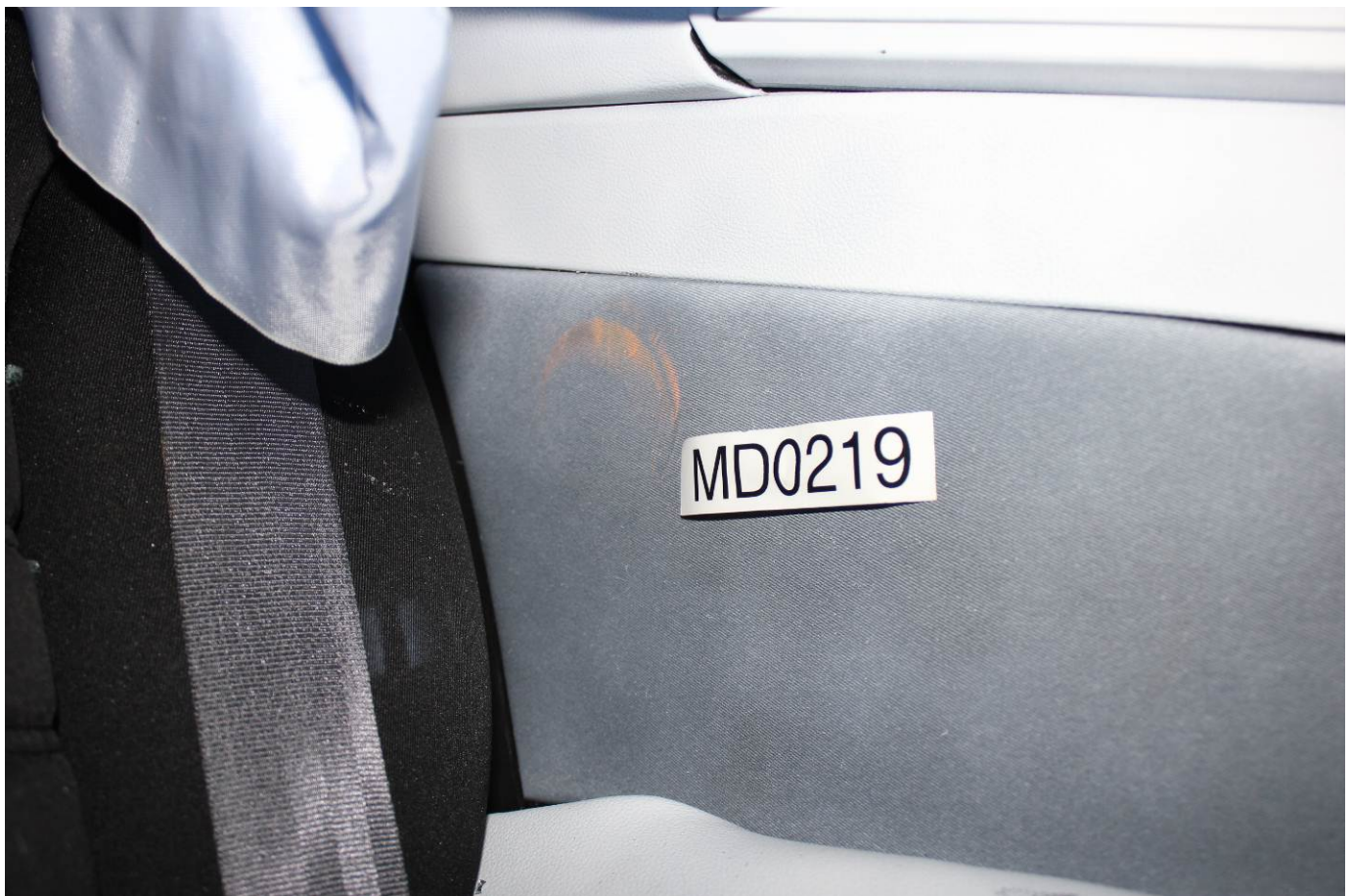
Post-Test Rear Passenger Dummy Close-up Torso Contact with Vehicle Interior View
