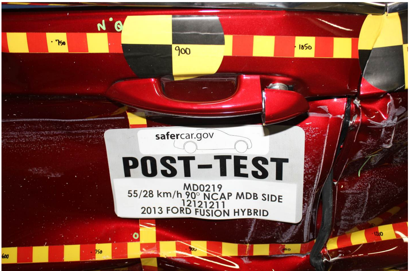
Post-Test Left Front Door Latch Close-Up
