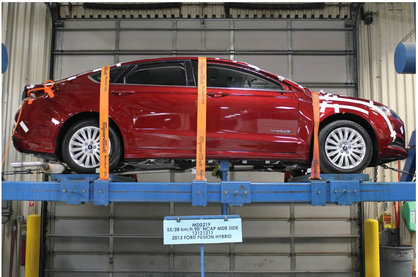
FMVSS No. 301 Static Rollover 360 Degrees
