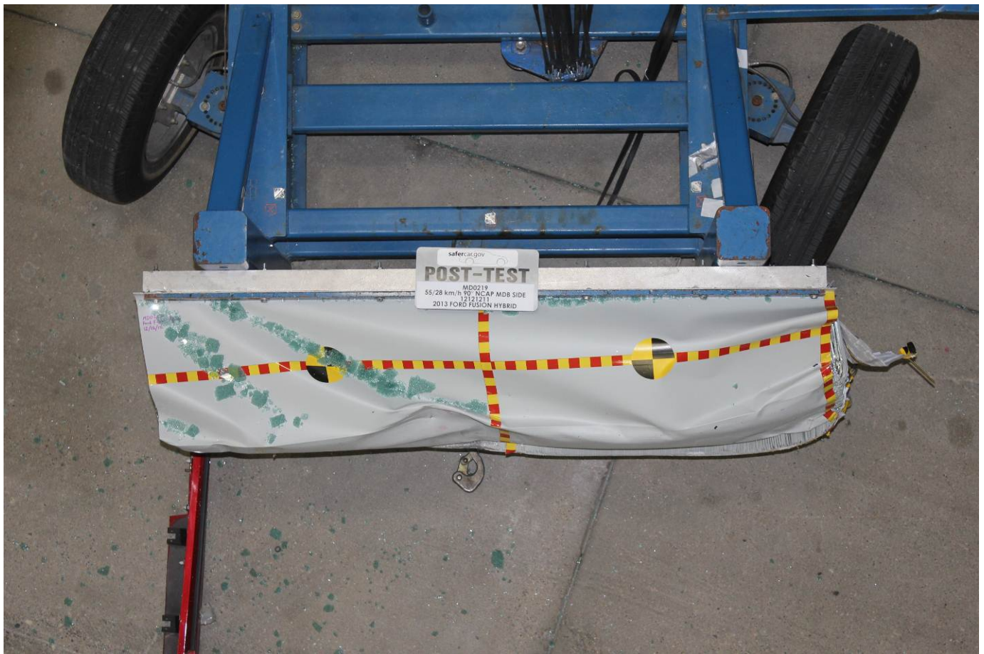
Post-Test Top View of MDB Impactor Face
