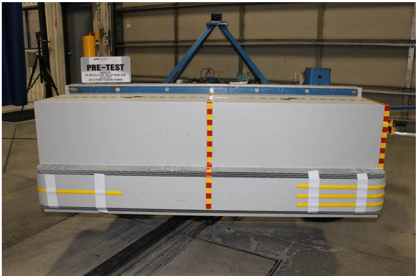
Pre-Test Front View of MDB Impactor Face
