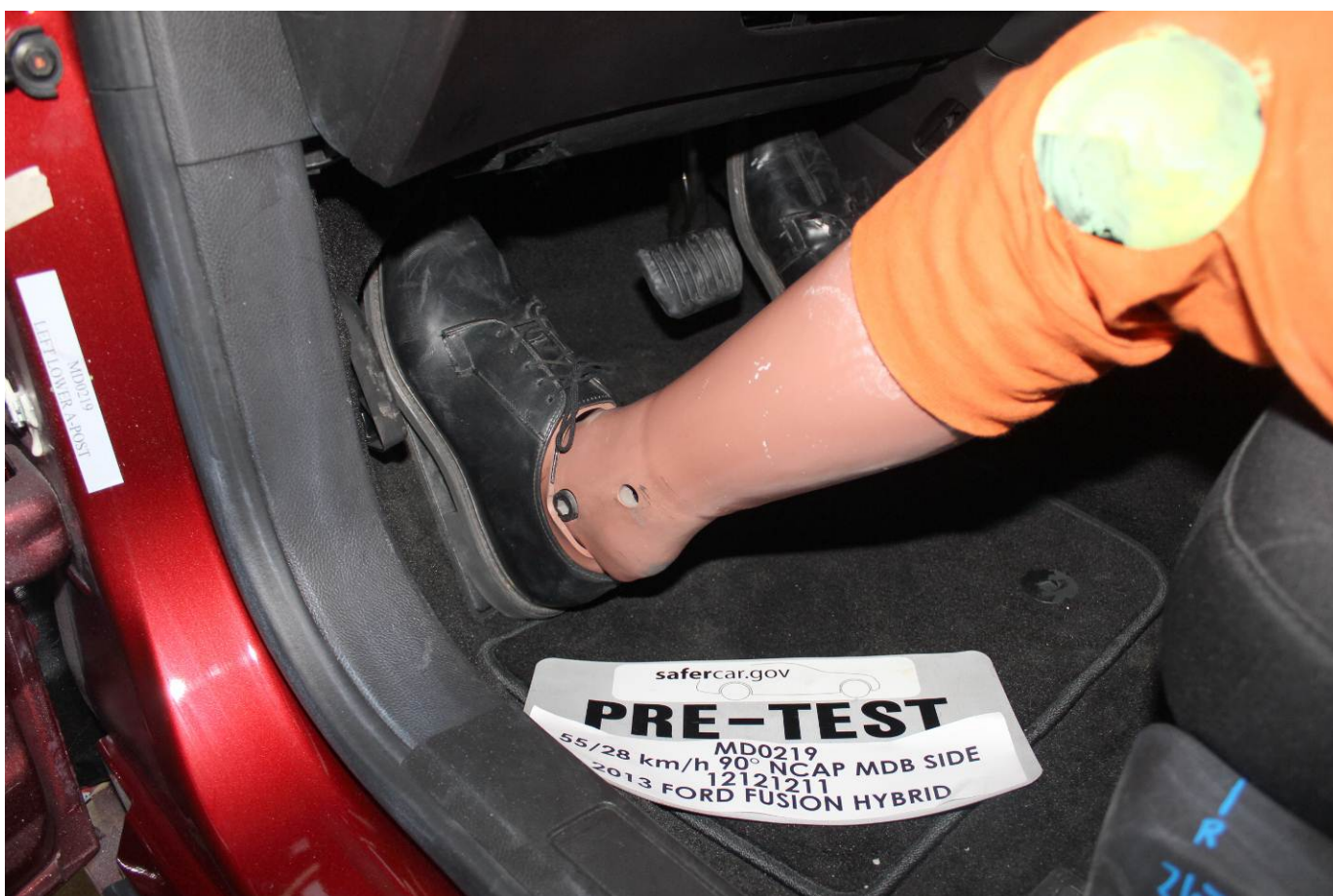
Pre-Test Placement of Driver Dummy's Feet
