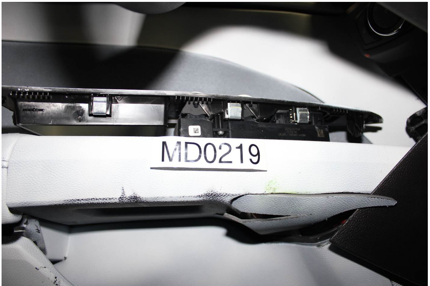
Post-Test Driver Dummy Close-up Knee Contact View
