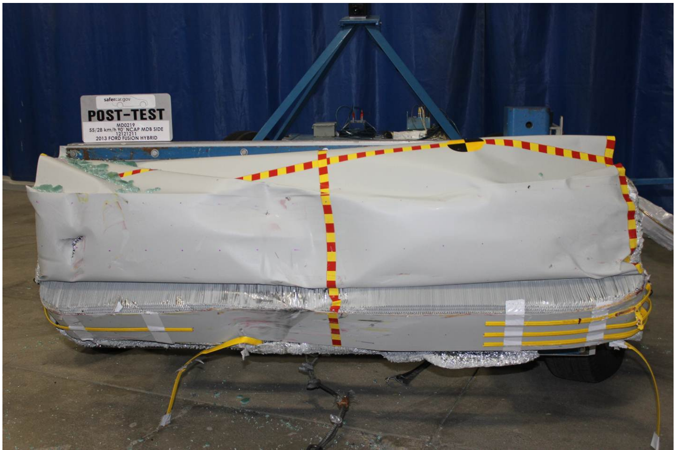
Post-Test Front View of MDB Impactor Face
