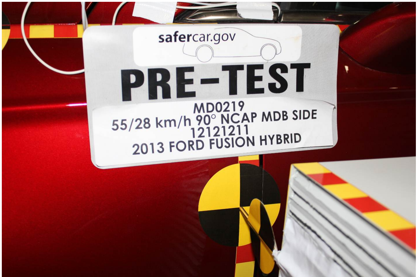
Pre-Test Close-Up View of Impact Point Target
