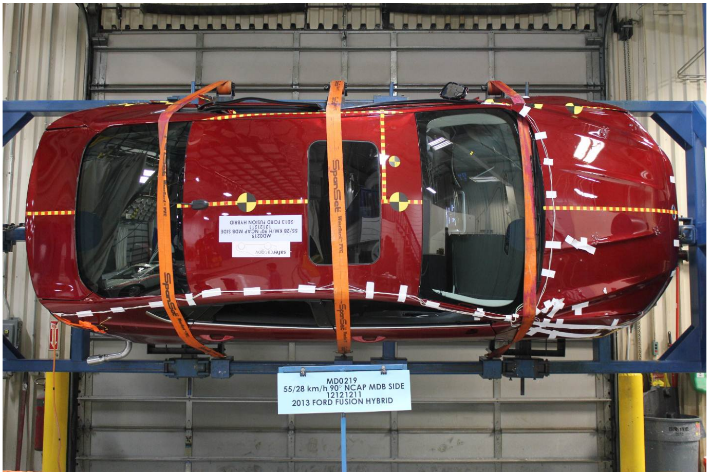
FMVSS No. 301 Static Rollover 270 Degrees
