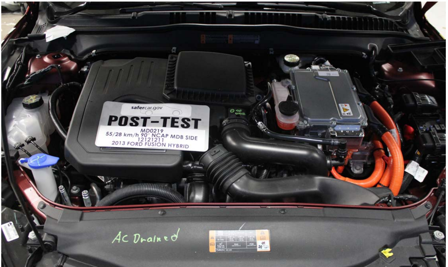
No. 017 Post-Impact View of Electric Propulsion Drive
