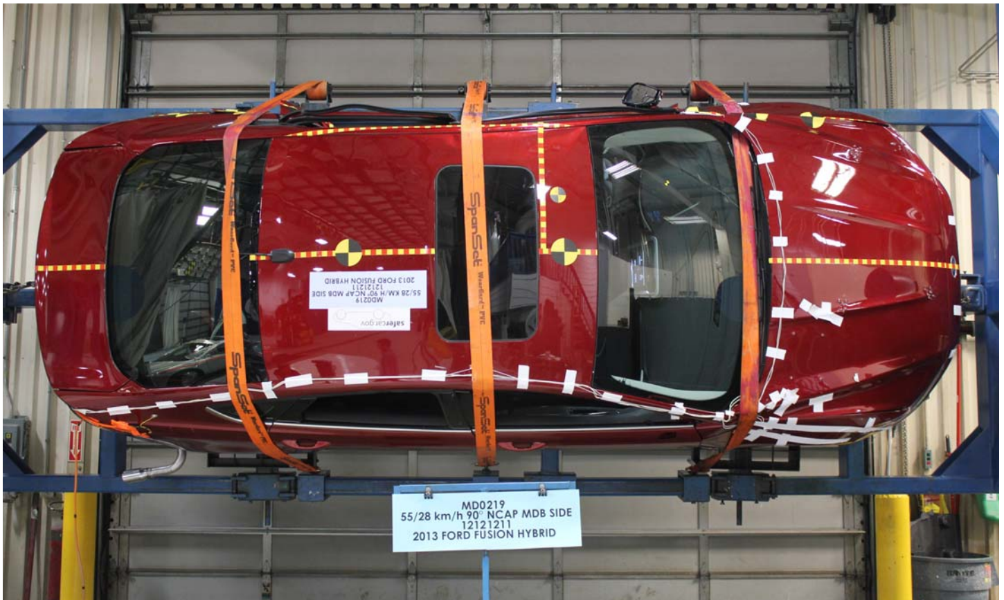
No. 030 FMVSS No. 305 Static Rollover at 270°
