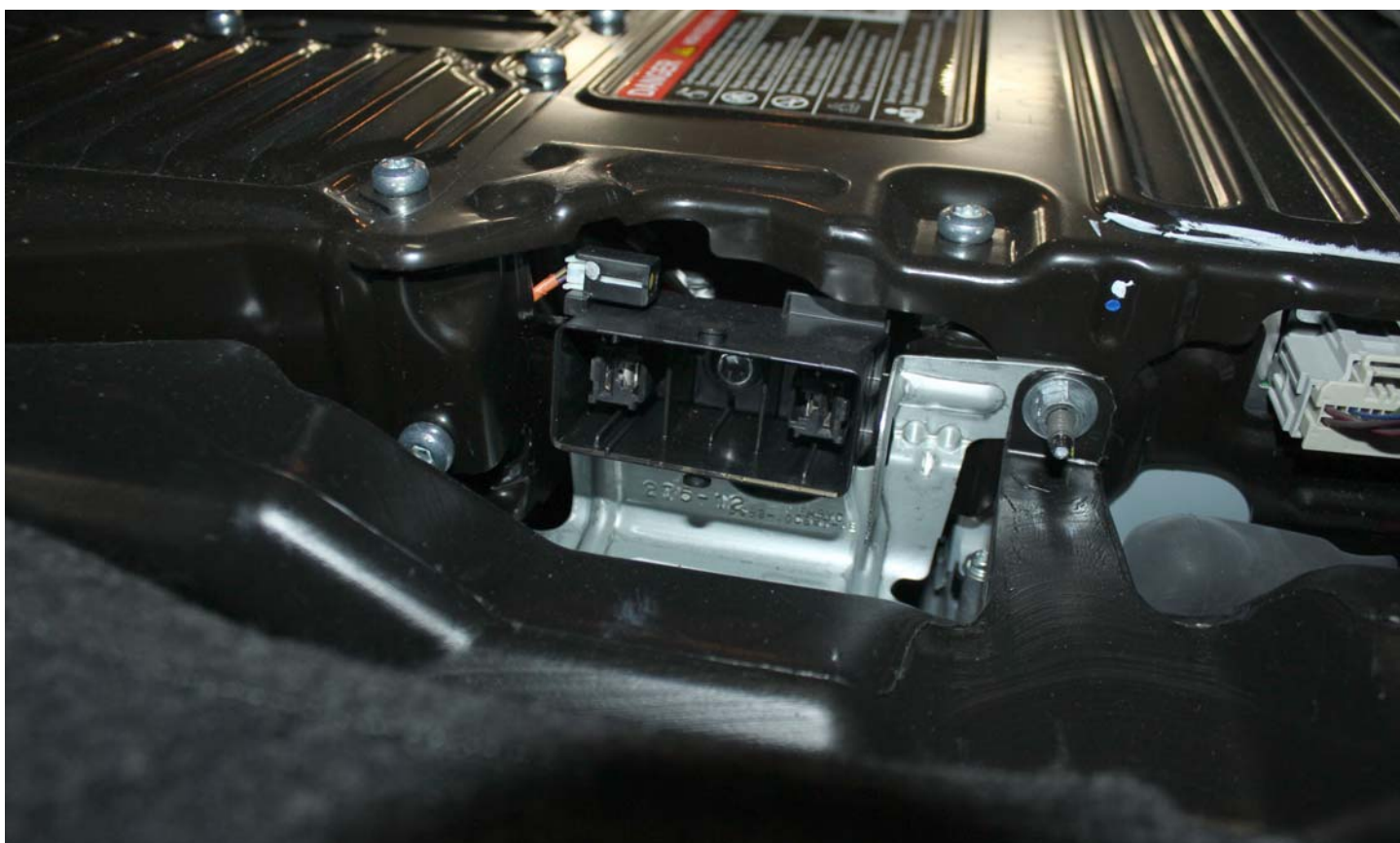
No. 007 Manual High Voltage Service Disconnect Removed
