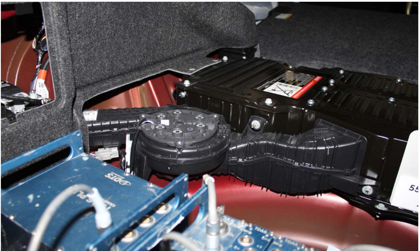
No. 019 Pre-Impact View Propulsion Battery Venting System(s)
