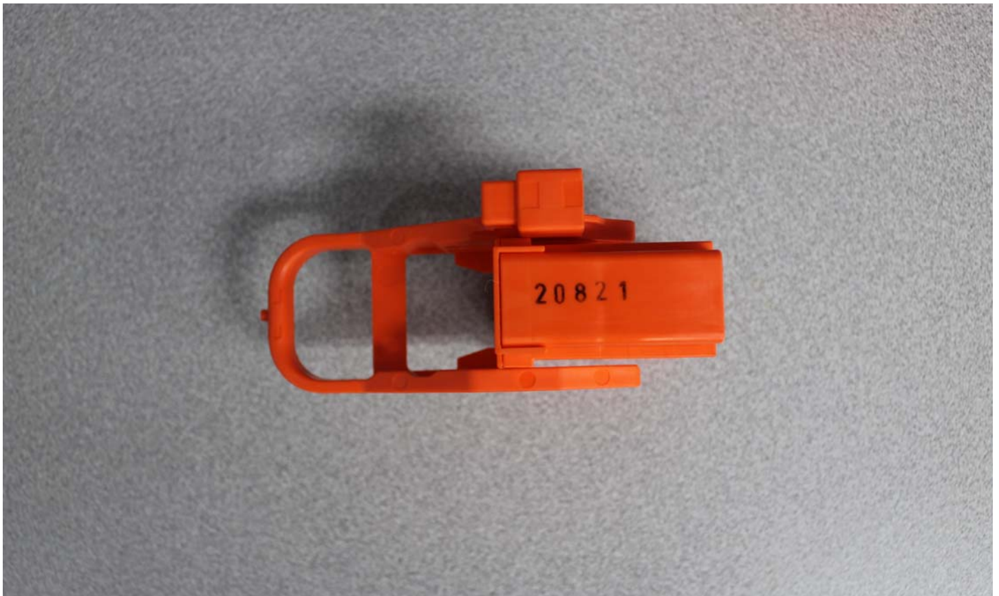
No. 008 Manual High Voltage Service Disconnect Removed
