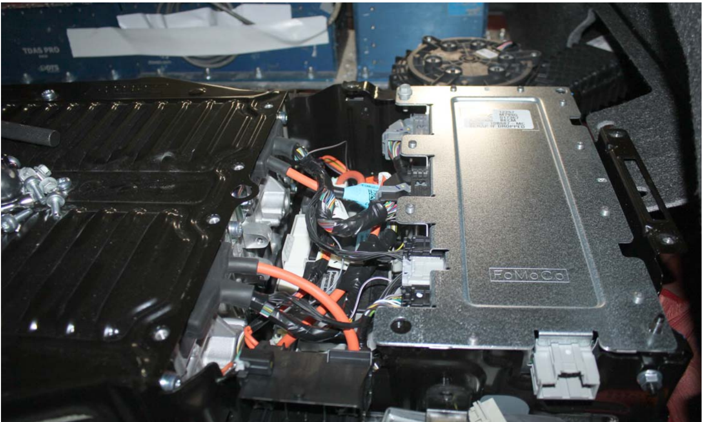
No. 018 Pre-Impact View of High Voltage Interconnect(s)
