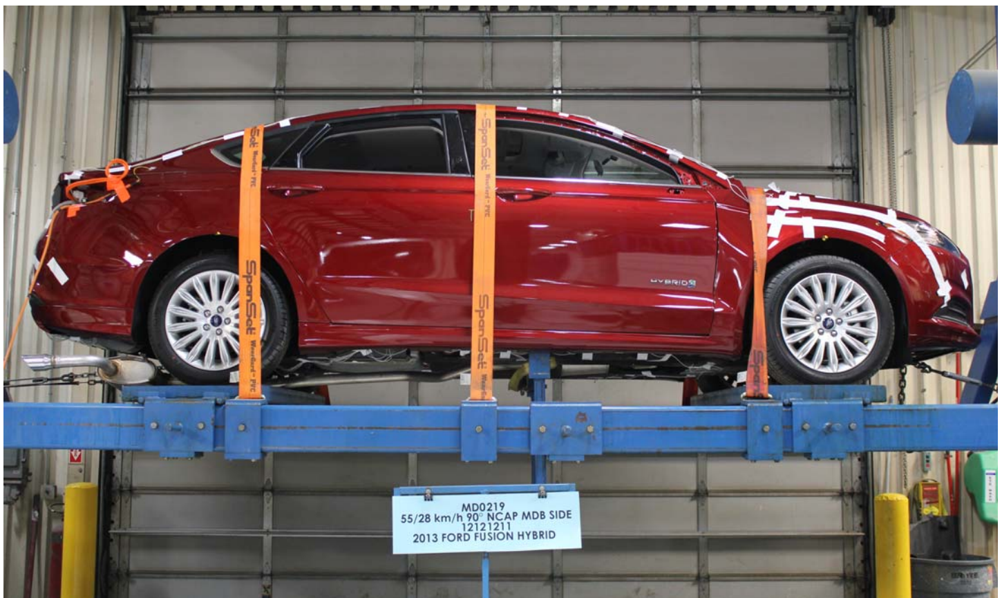
No. 031 FMVSS No. 305 Static Rollover at 360°
