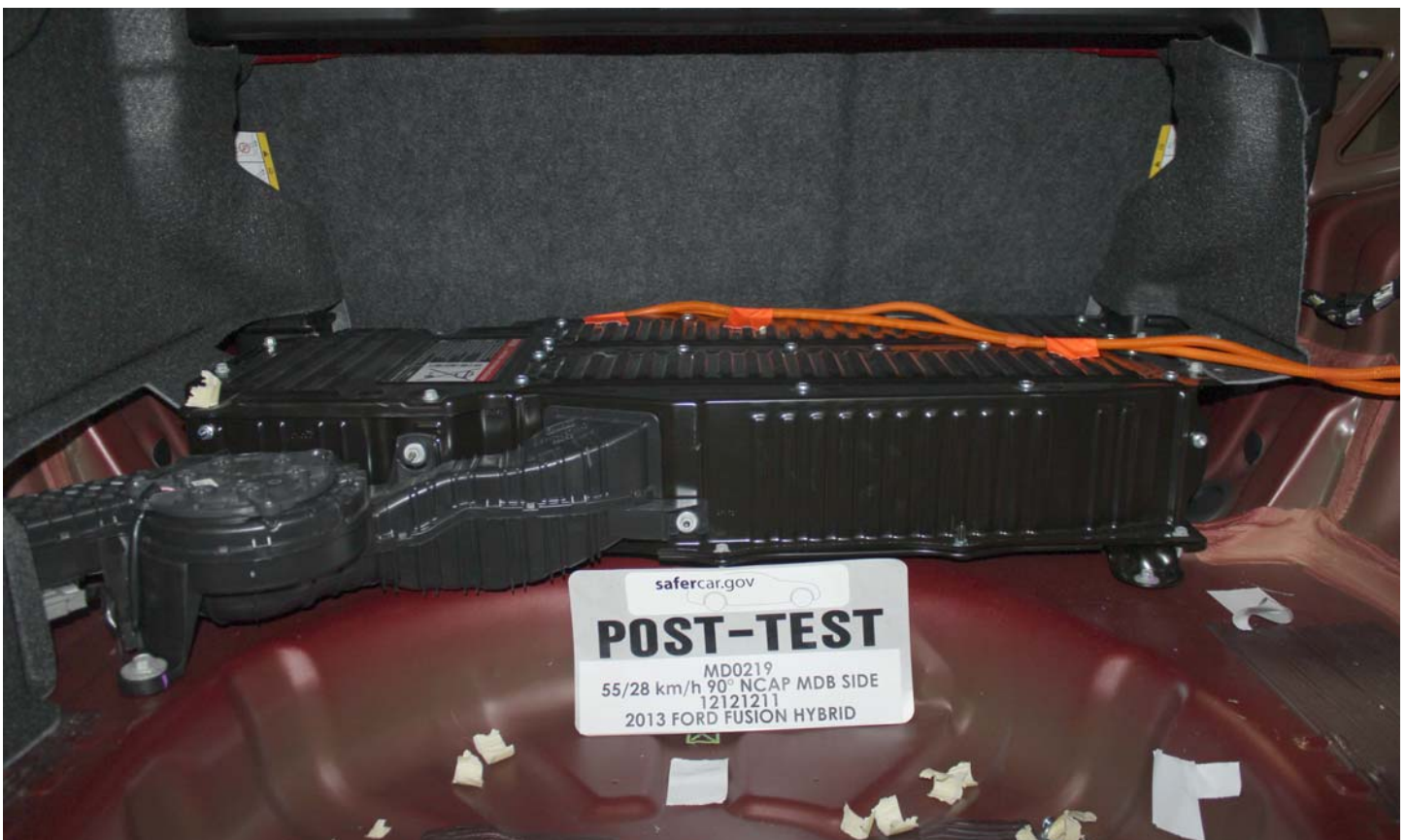
No. 011 Post-Impact Rear View of Propulsion Battery
