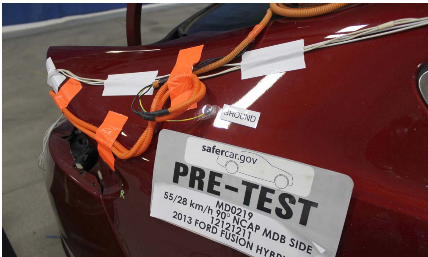
No. 021 Pre-Impact View of Ground Lead Attached
