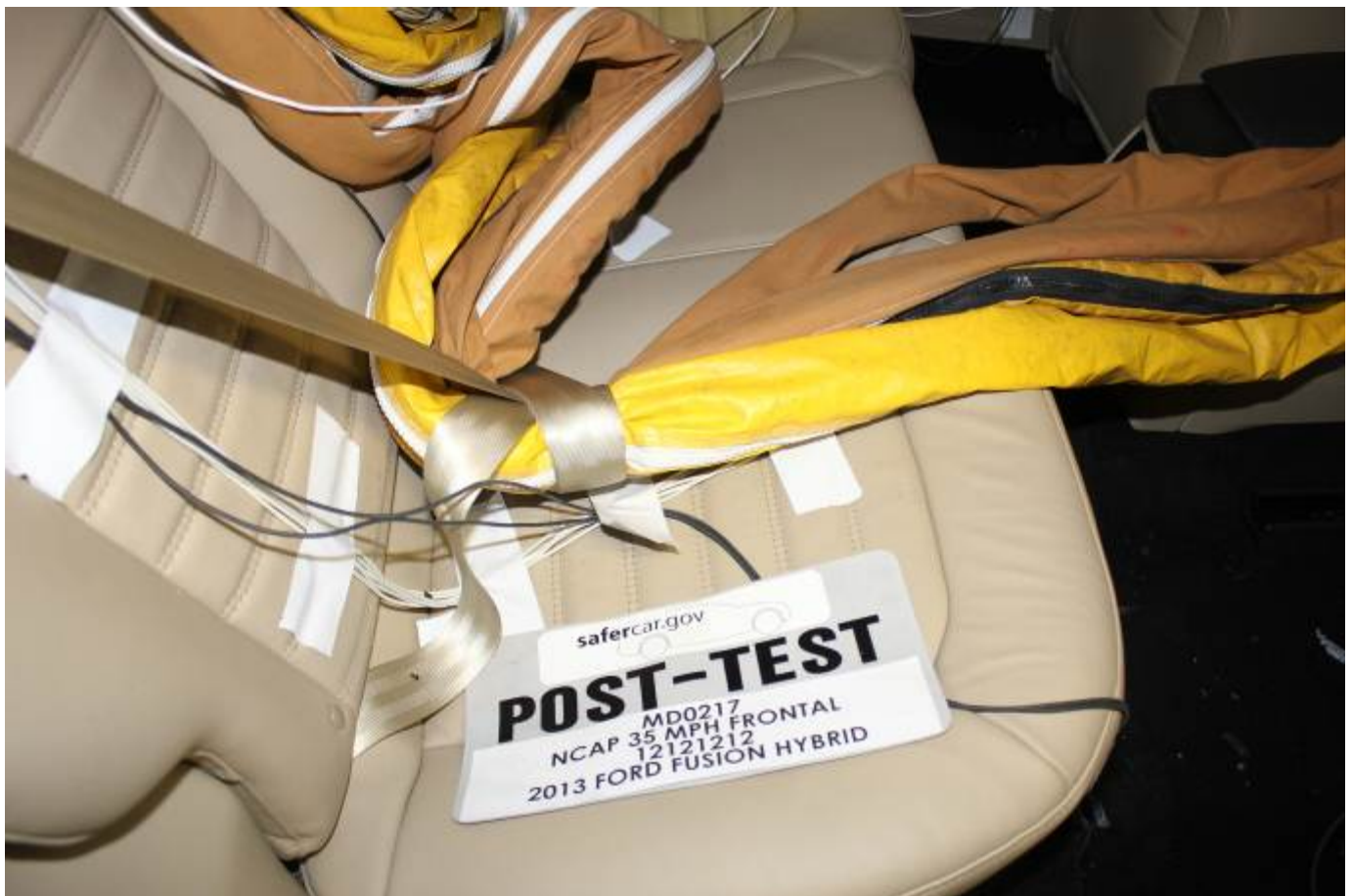
Post-Test Dummy Cable Routing
