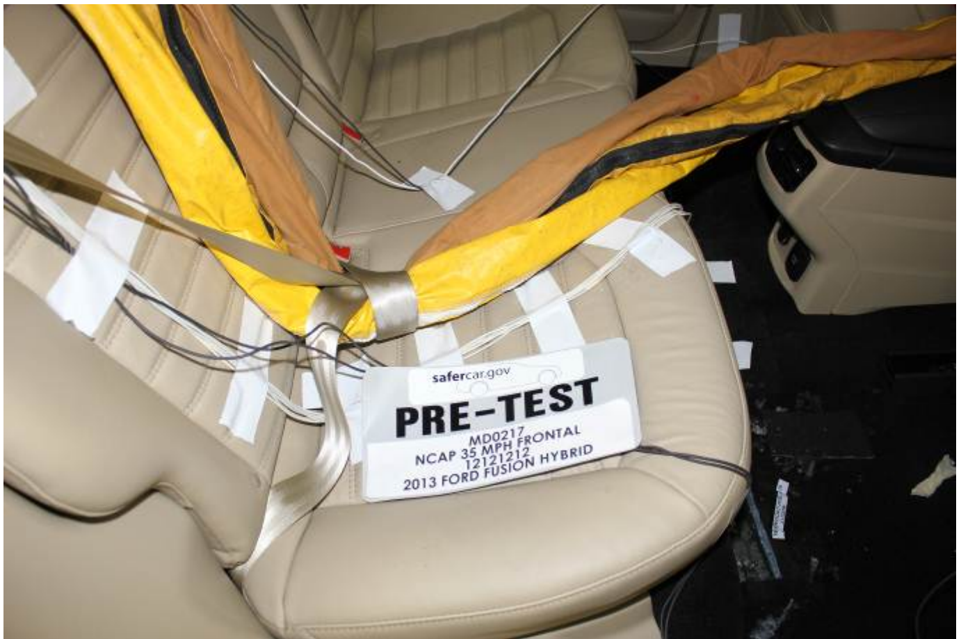
Pre-Test Dummy Cable Routing
