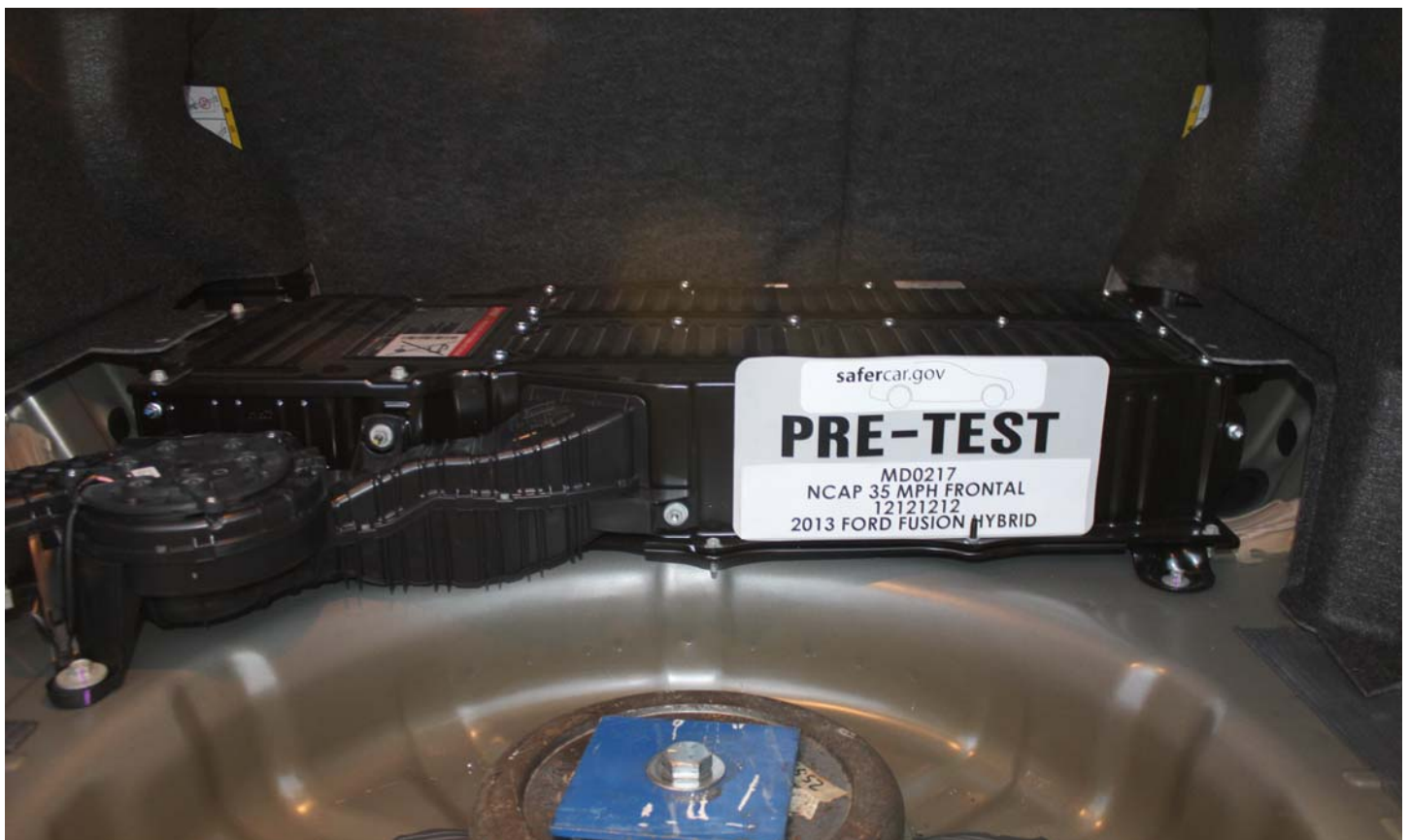
No. 009 Pre-Impact View of Propulsion Battery
