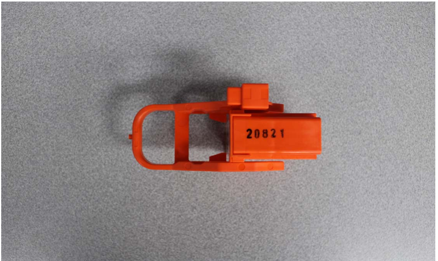
No. 008 Manual High Voltage Service Disconnect Removed
