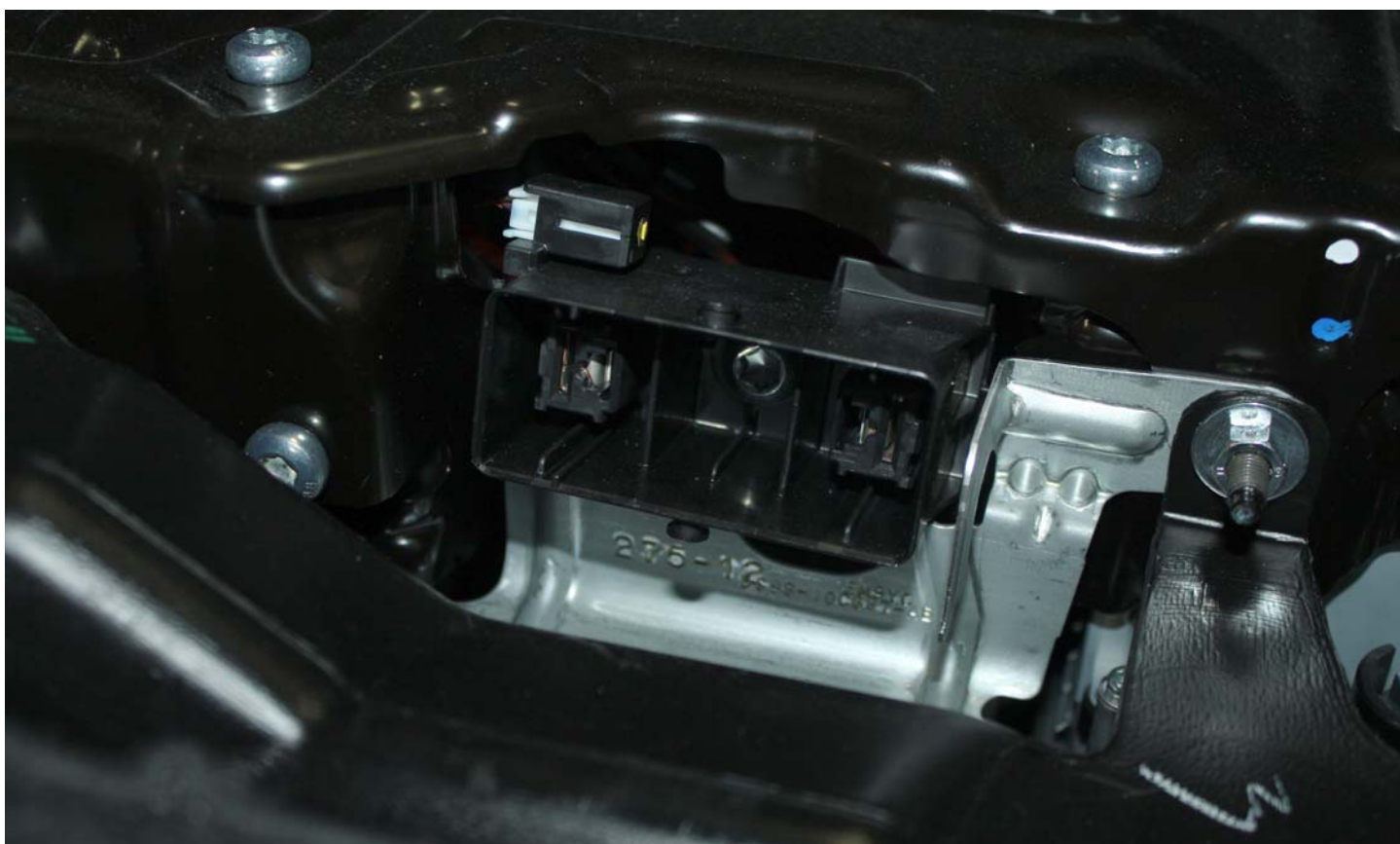
No. 007 Manual High Voltage Service Disconnect Removed
