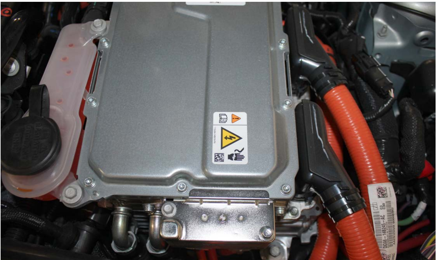
No. 002 Power Inverter Warning Label
