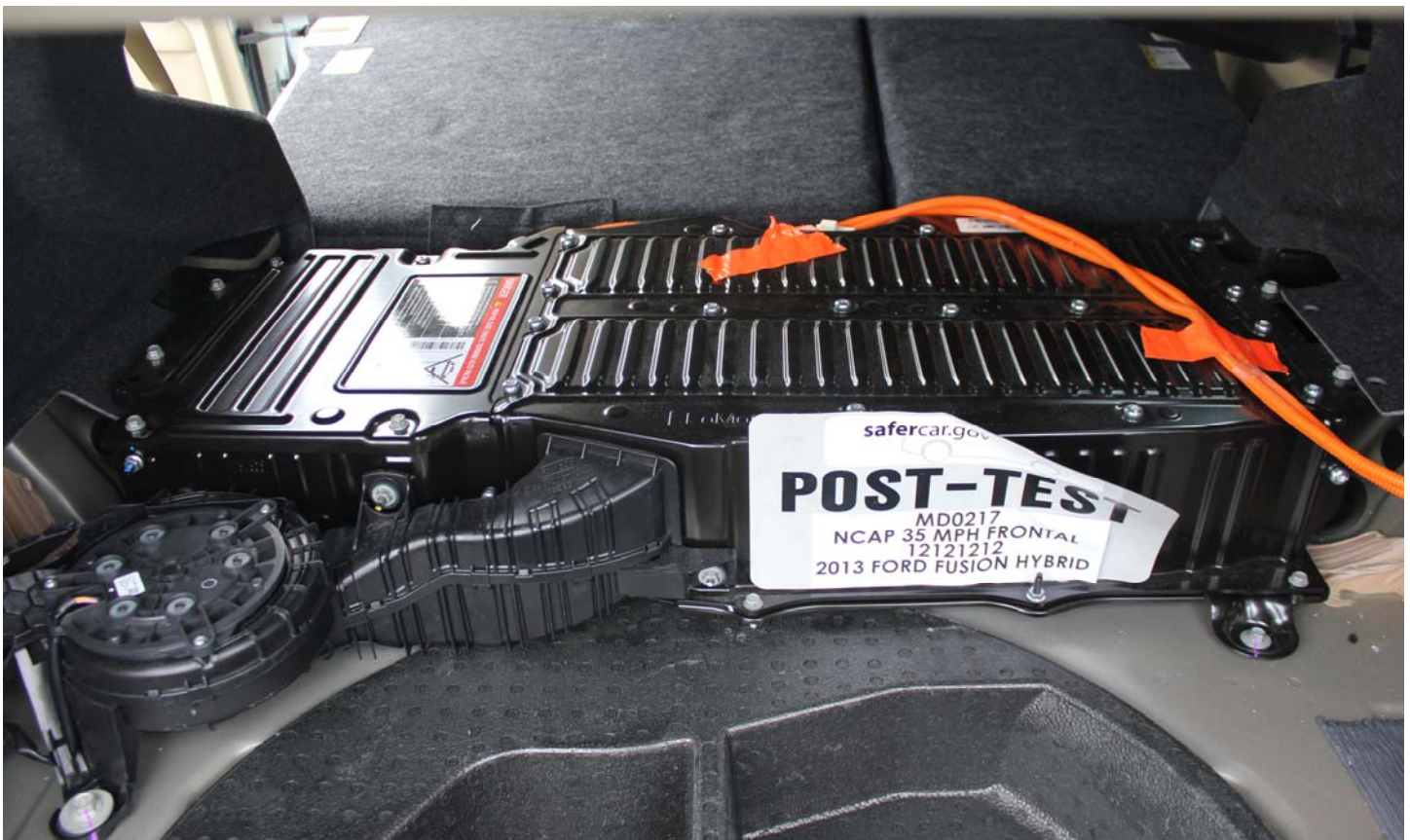
No. 011 Post-Impact Rear View of Propulsion Battery
