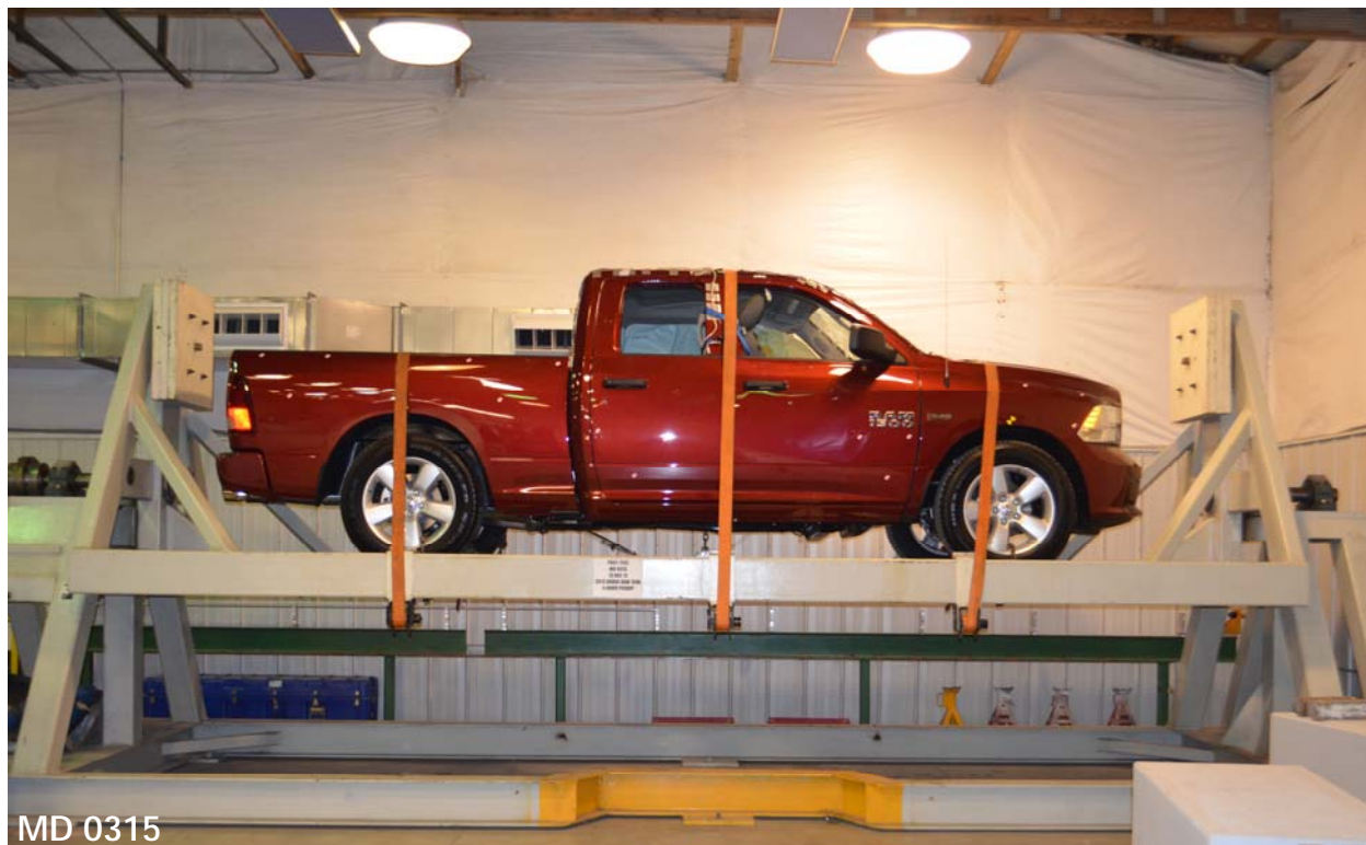
Figure 063: FMVSS No. 301 Static Rollover 0 Degrees
