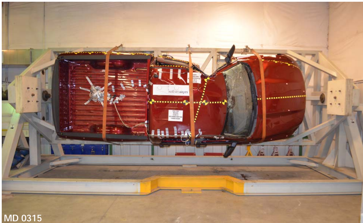
Figure 066: FMVSS No. 301 Static Rollover 270 Degrees
