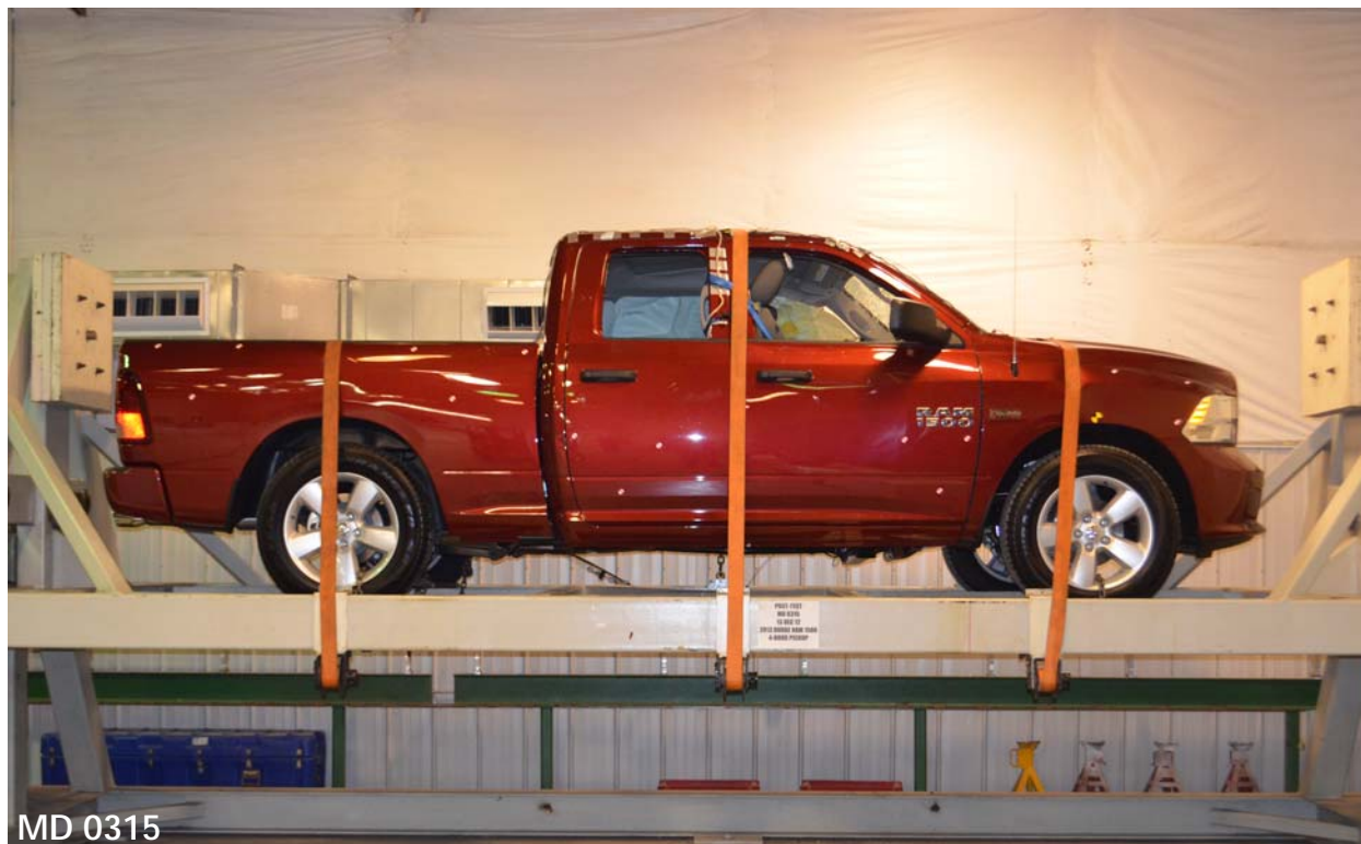
Figure 067: FMVSS No. 301 Static Rollover 360 Degrees
