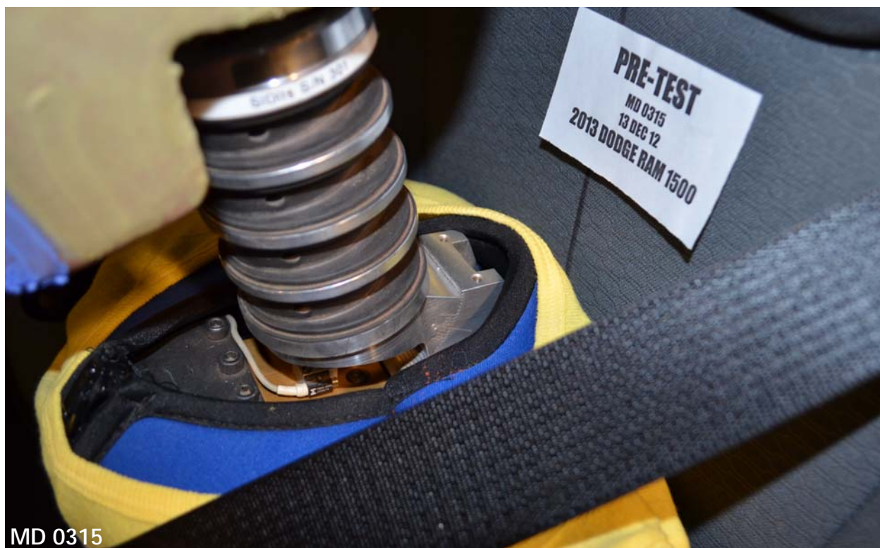
Figure 030: Pre-Test Left Side View of Dummy's Neck Showing Position of Adjustable Neck Bracket
