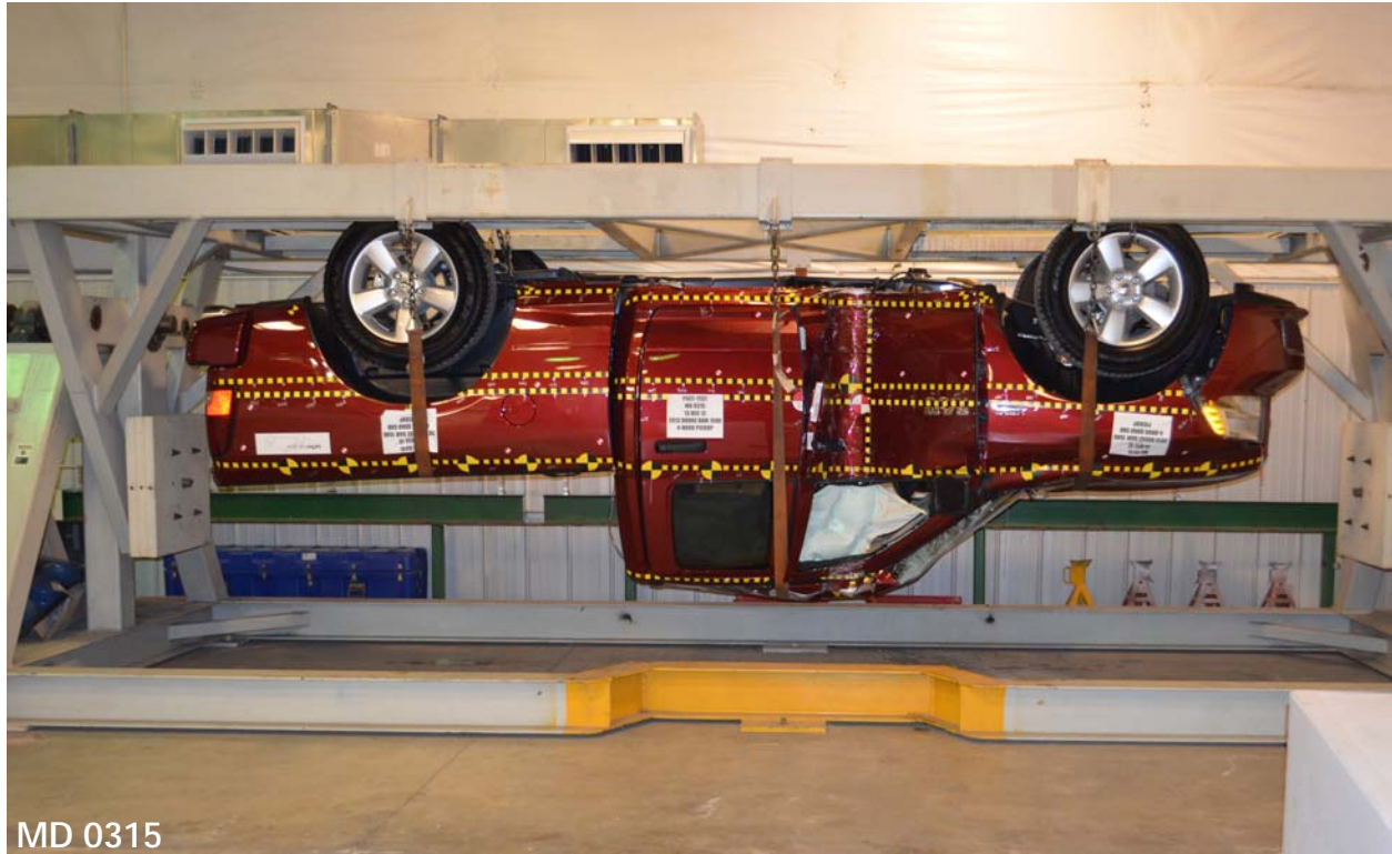
Figure 065: FMVSS No. 301 Static Rollover 180 Degrees
