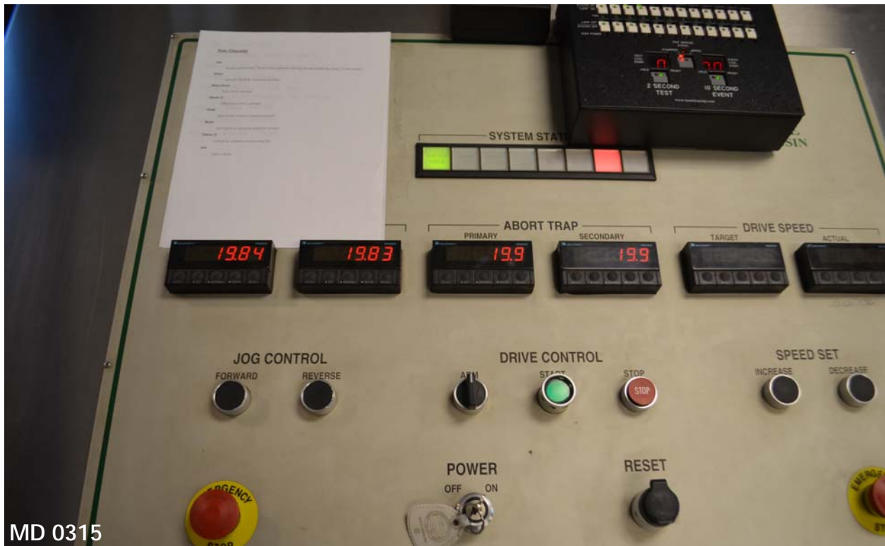
Figure 062: Post-Test Primary and Redundant Speed Trap Read-Out
