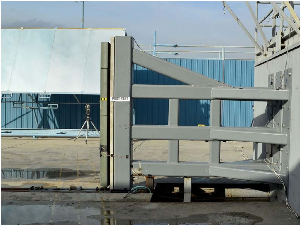
FIGURE 60. Post-Test Pole Barrier Side View
