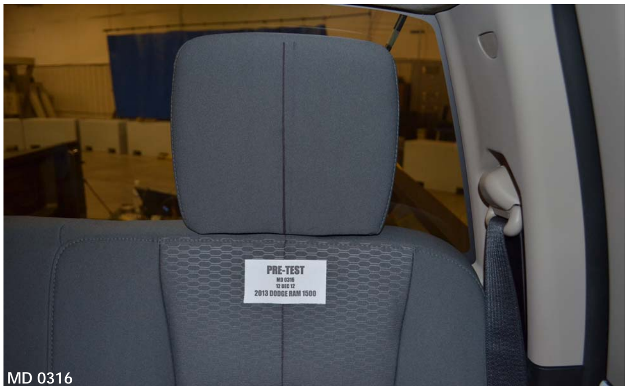
Figure A-58: Pre-Test Frontal View of Rear Passenger Seat Back Prior to Dummy Positioning
