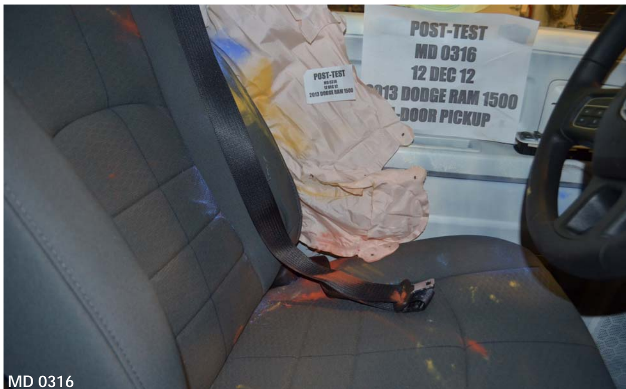
Figure A-53: Post-Test Driver Dummy Close-Up Pelvis Contact with Side Airbag View
