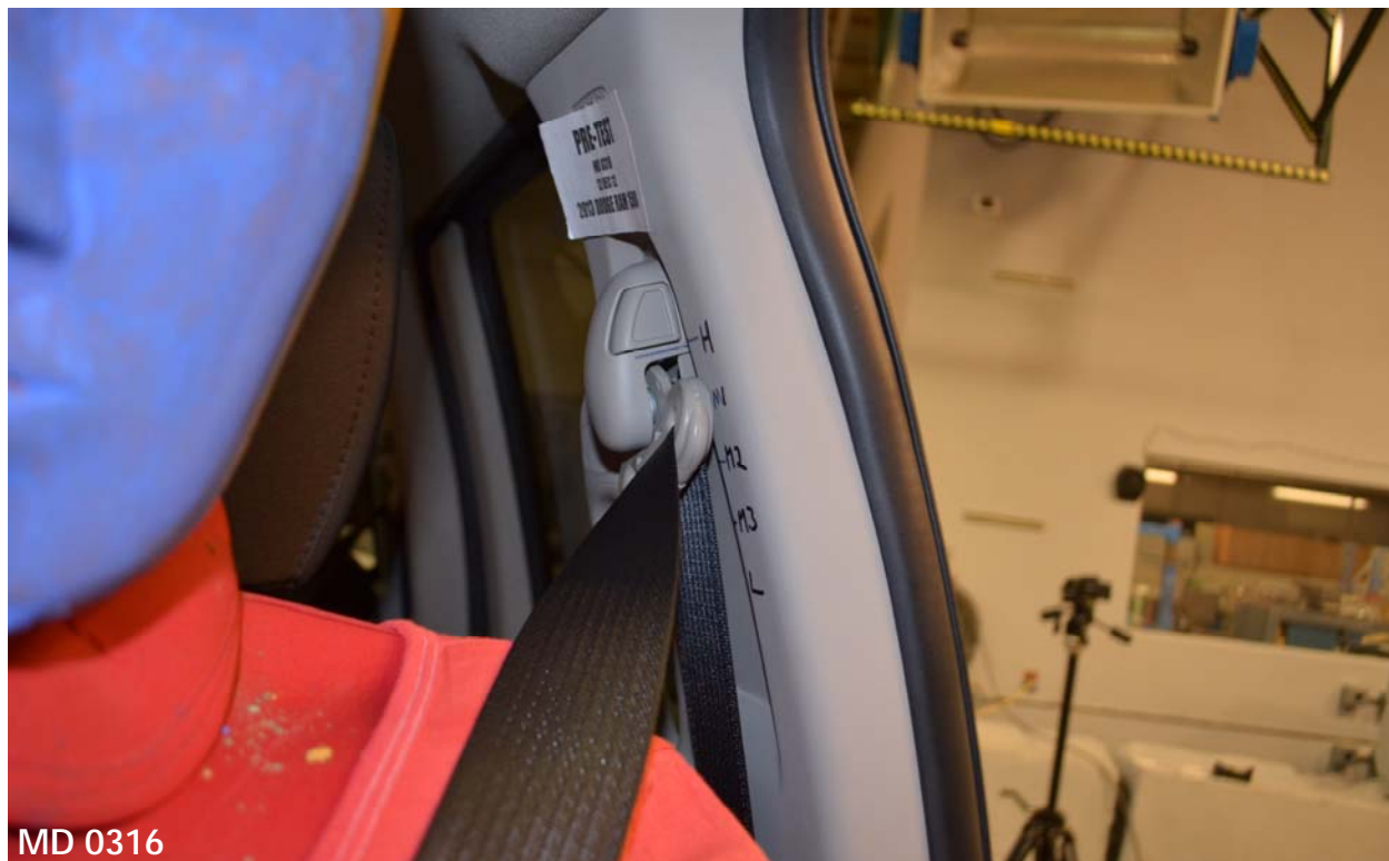
Figure A-35: Pre-Test View of Belt Anchorage for Driver Dummy
