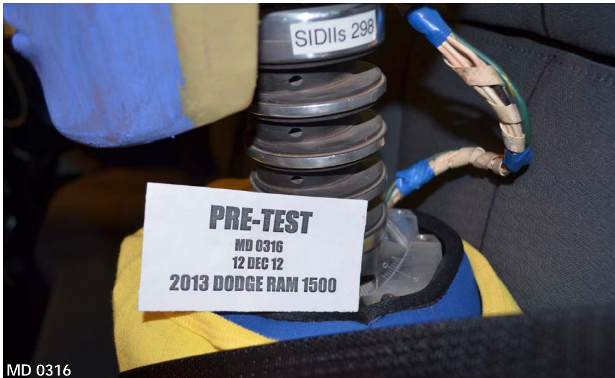
Figure A-62: Pre-Test View of Rear Passenger Dummy's Neck Showing Position of Adjustable Neck Bracket
