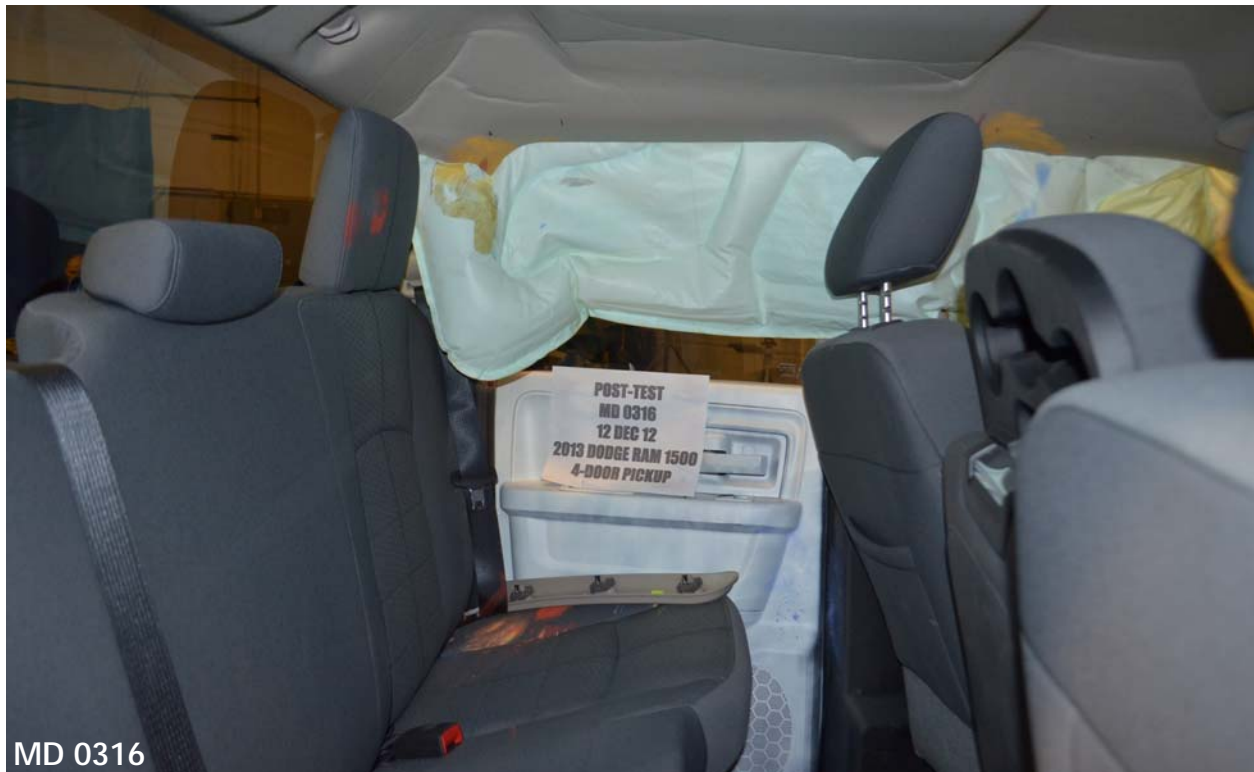
Figure A-74: Post-Test Rear Passenger Inner Door Panel View Showing Dummy Contact Locations
