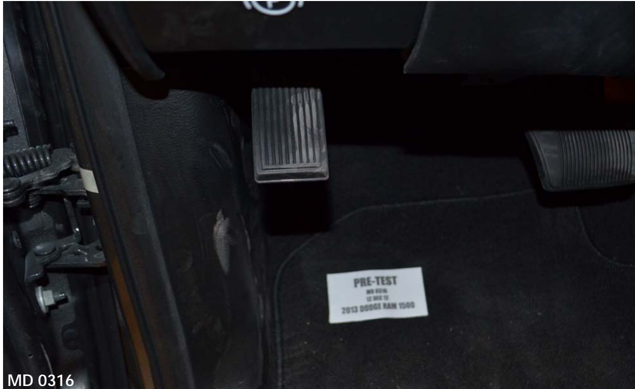
Figure A-37: View of Disengaged Parking Brake
