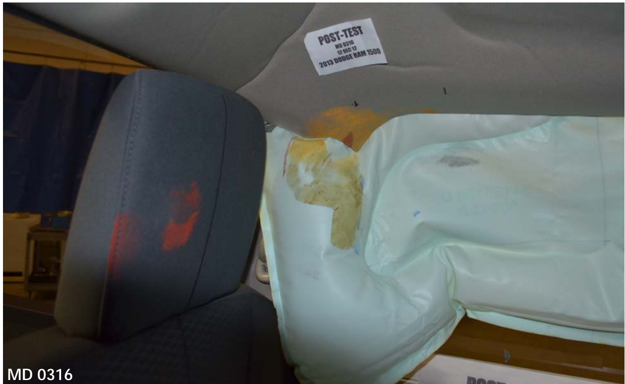
Figure A-75: Post-Test Rear Passenger Dummy Close-Up Head Contact with Vehicle Interior View
