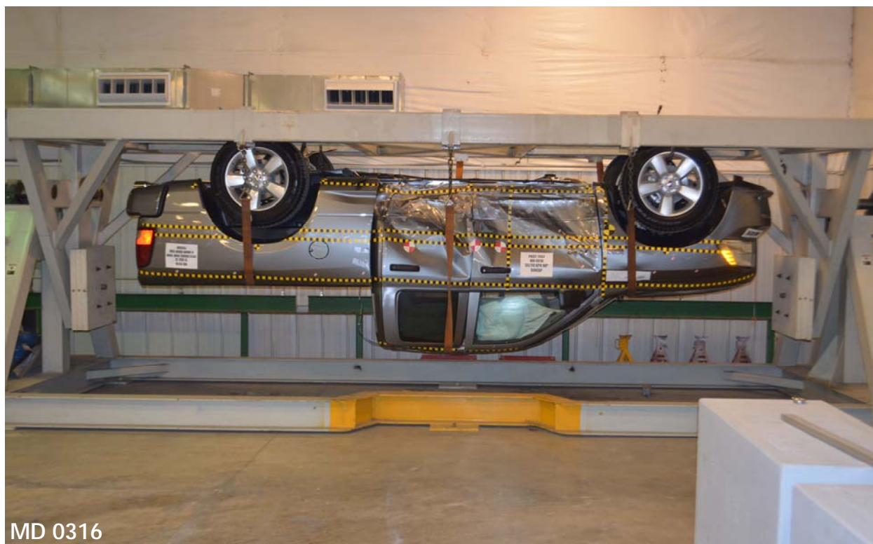
Figure A-98: FMVSS No. 301 Static Rollover 180 Degrees
