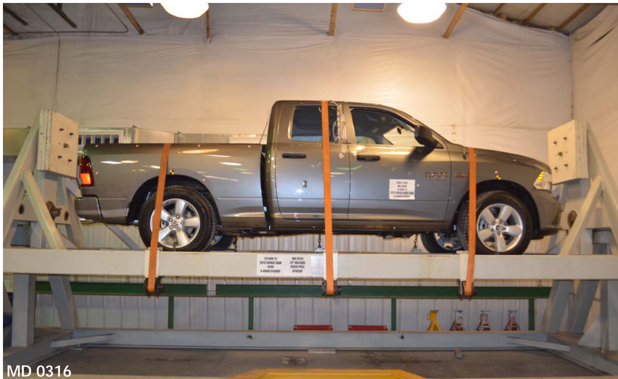
Figure A-96: FMVSS No. 301 Static Rollover 0 Degrees
