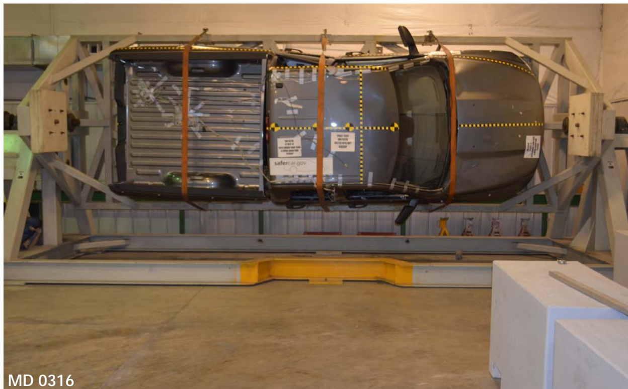
Figure A-99: FMVSS No. 301 Static Rollover 270 Degrees
