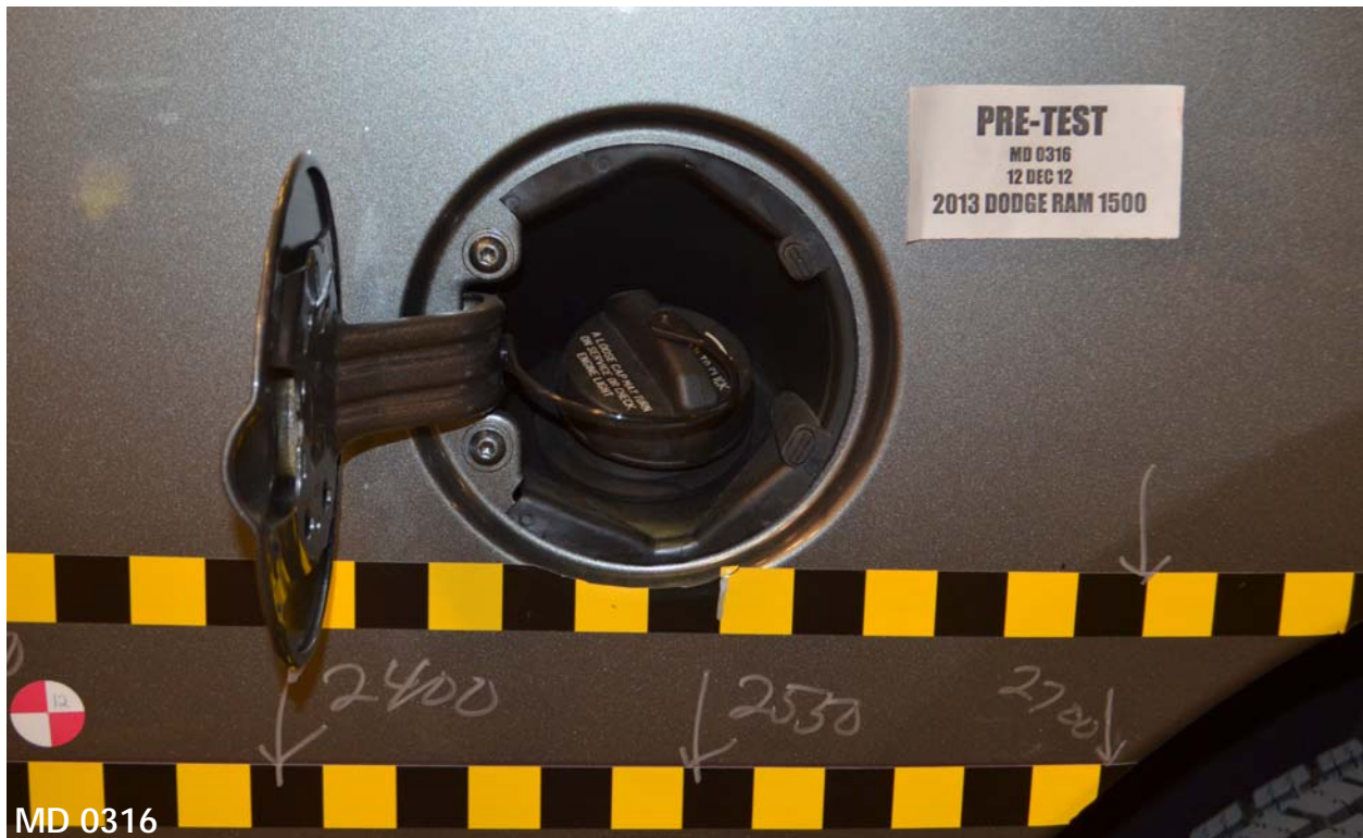
Figure A-82: Pre-Test View of Fuel Filler Cap or Fuel Filler Neck
