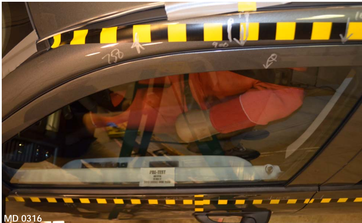
Figure A-42: Pre-Test Driver Dummy and Door Clearance View
