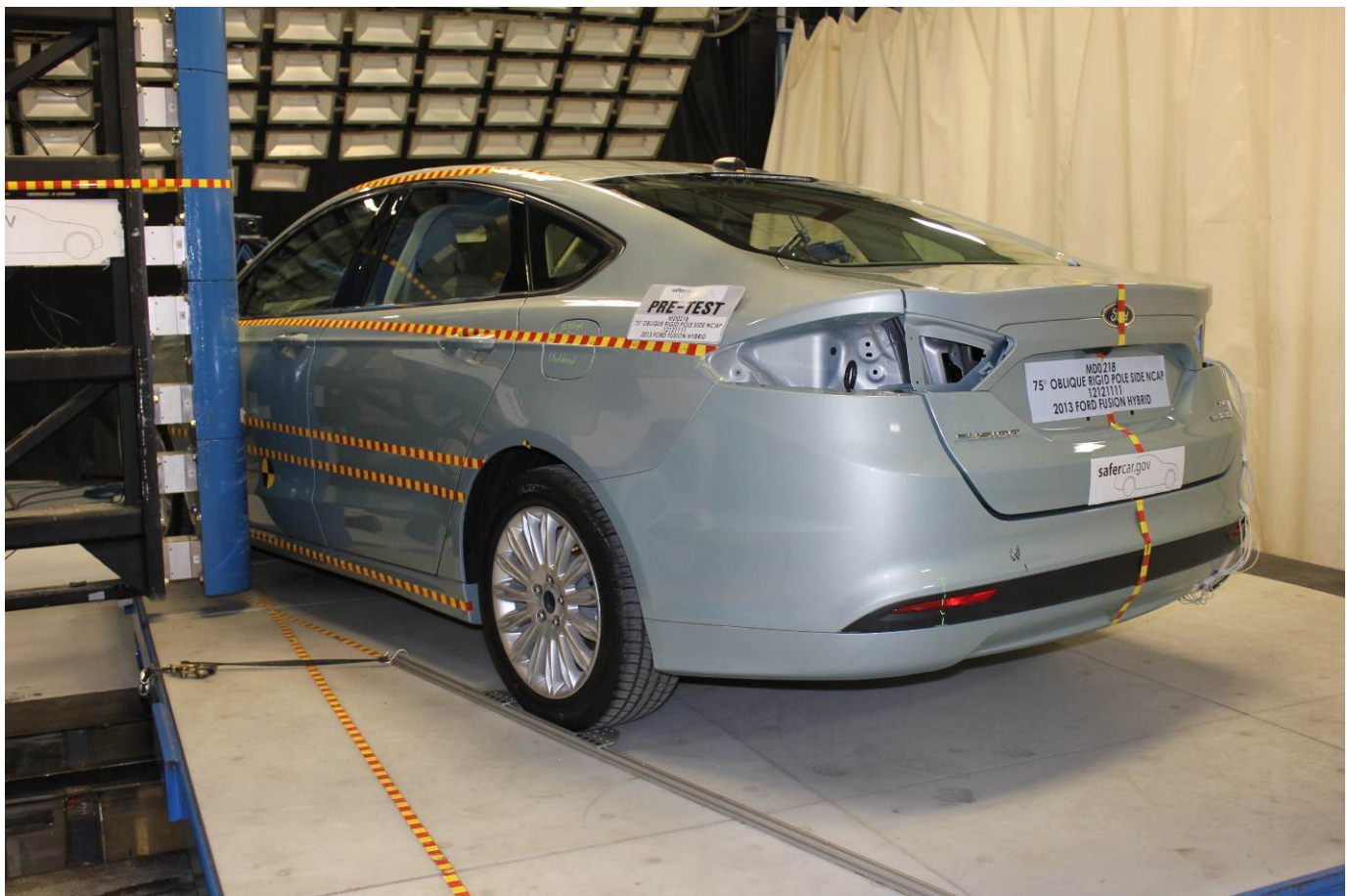
Pre-Test Right Side View of Pole Positioned Against Side of Vehicle
