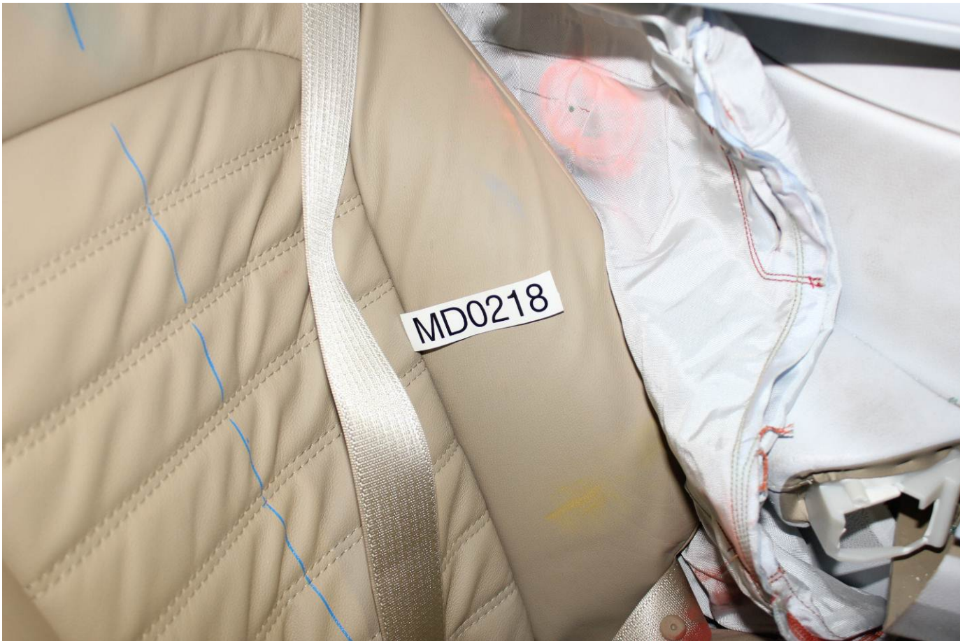
Post-Test Dummy Close-Up Torso Contact with Vehicle Interior View
