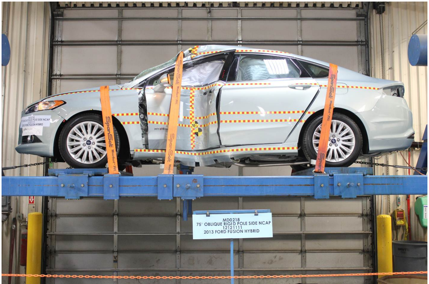
FMVSS No. 301 Static Rollover 0 Degrees
