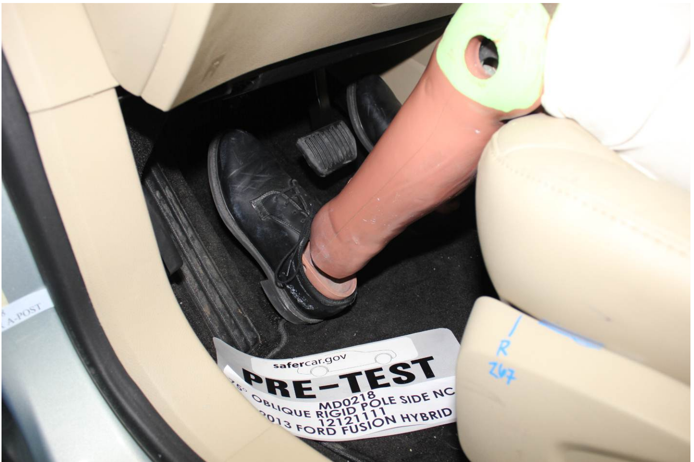
Pre-Test Placement of Dummy's Feet
