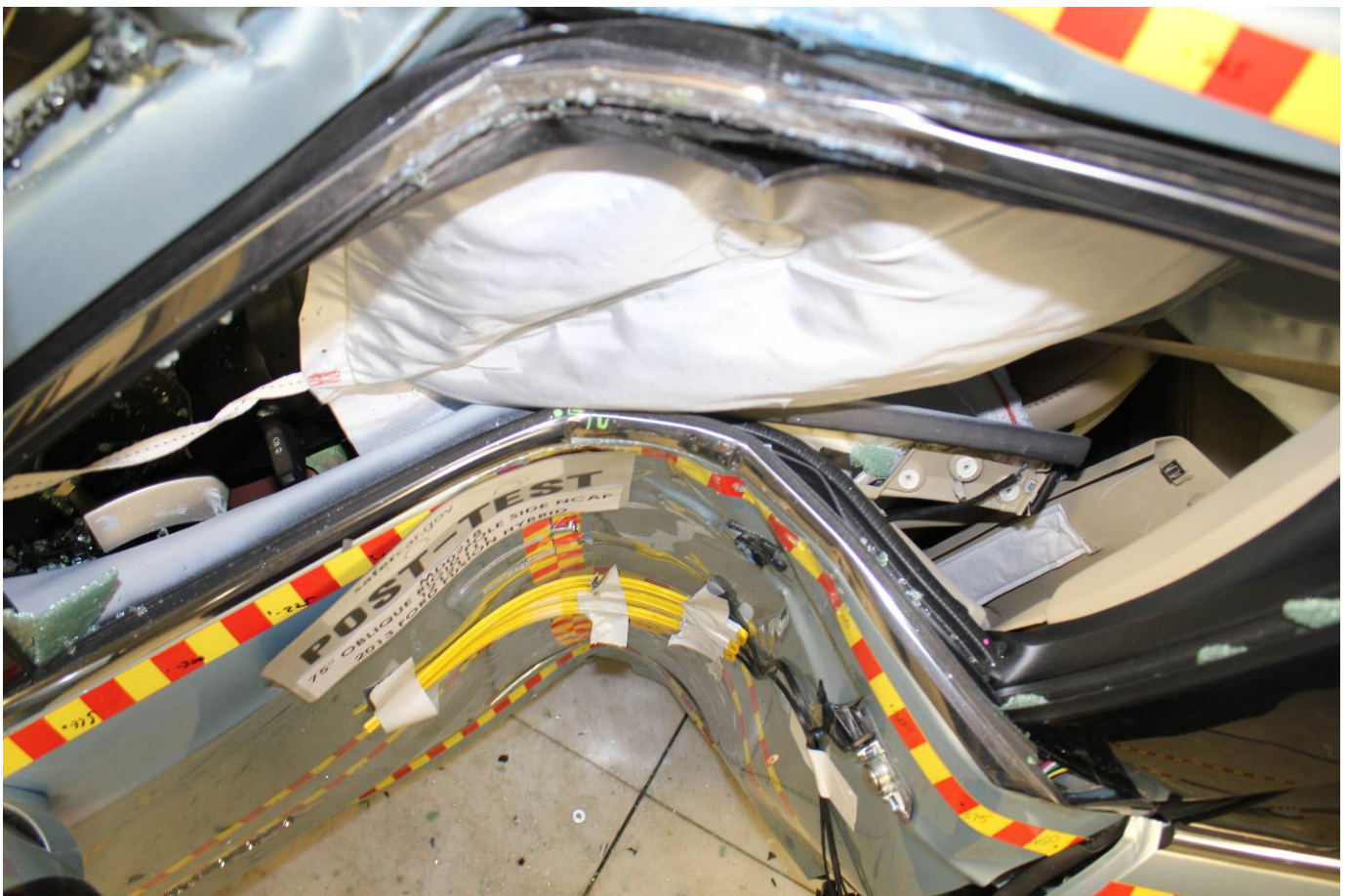
Post-Test Dummy and Door Clearance View
