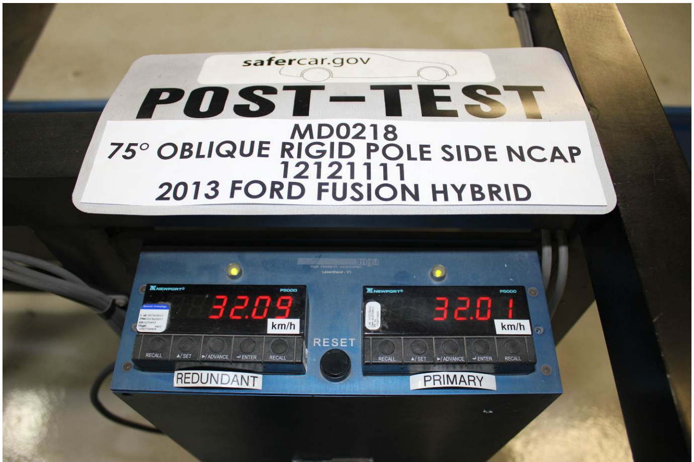
Post-Test Primary and Redundant Speed Trap Read-Out
