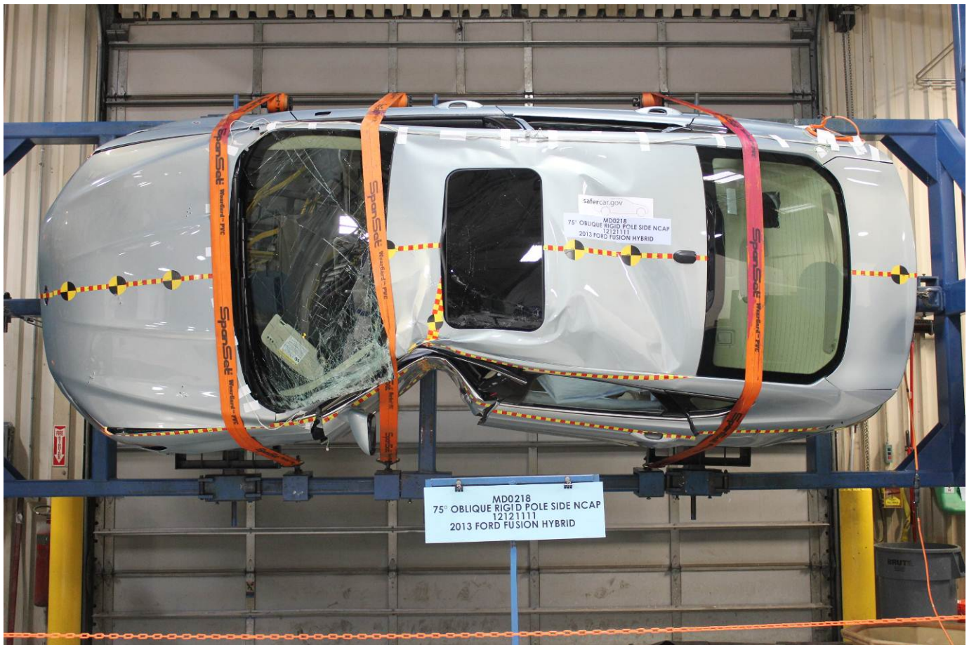
FMVSS No. 301 Static Rollover 90 Degrees
