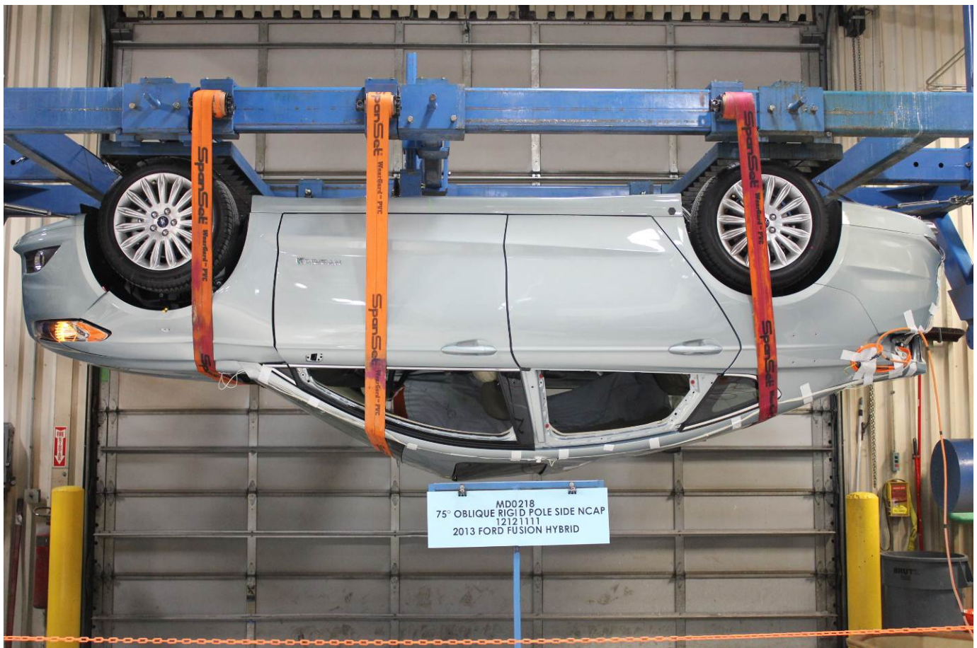
FMVSS No. 301 Static Rollover 180 Degrees
