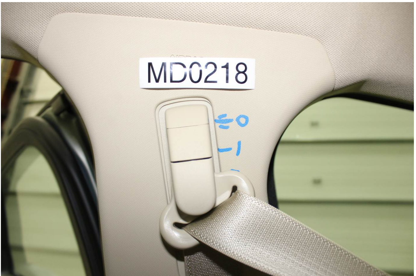
Pre-Test View of Belt Anchorage for Dummy
