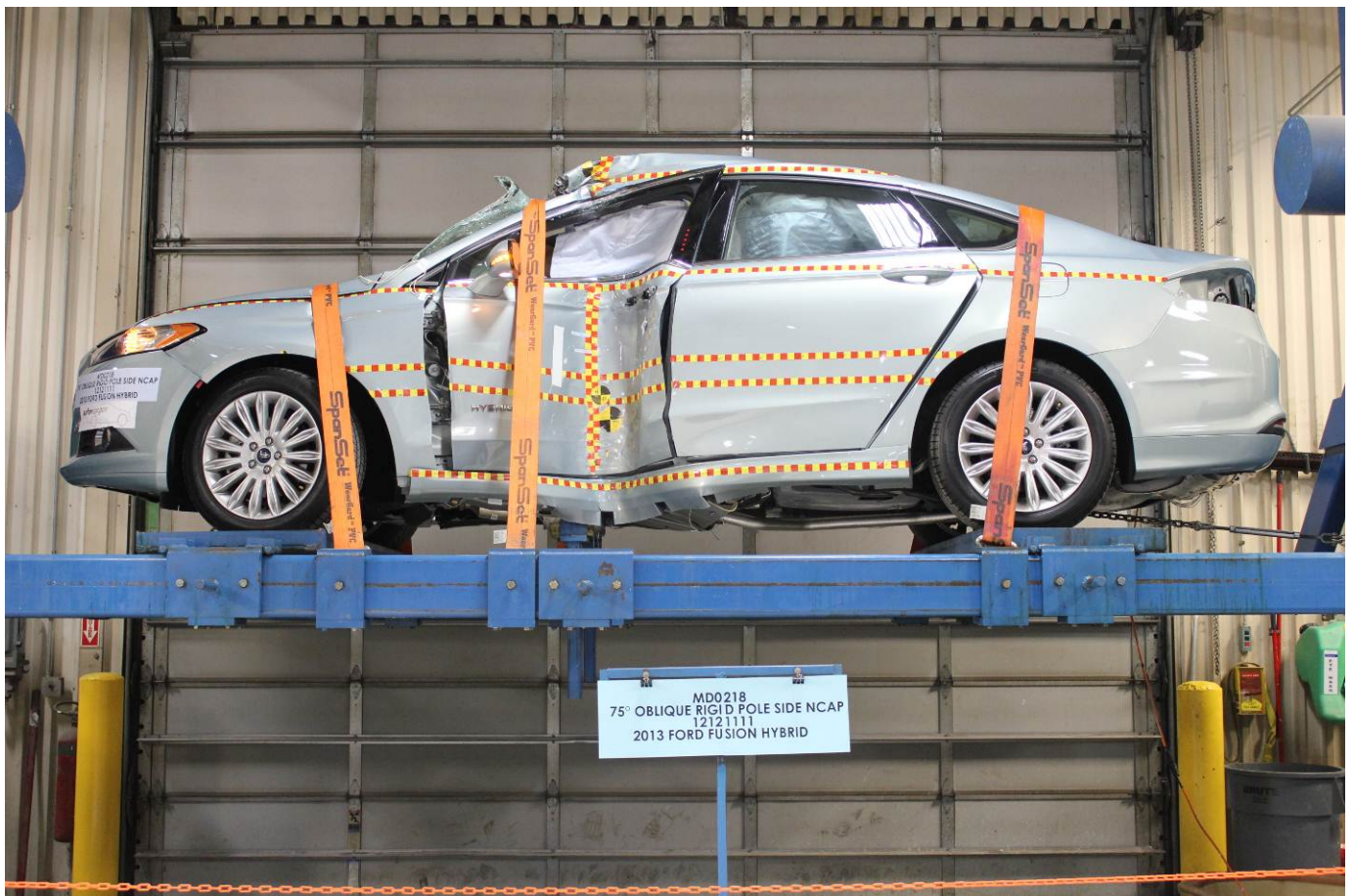
FMVSS No. 301 Static Rollover 360 Degrees
