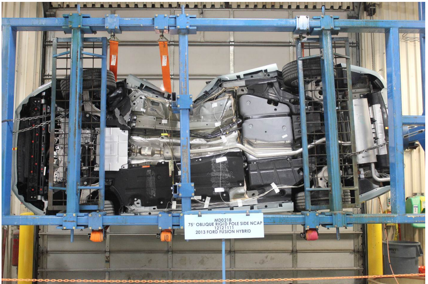
FMVSS No. 301 Static Rollover 270 Degrees
