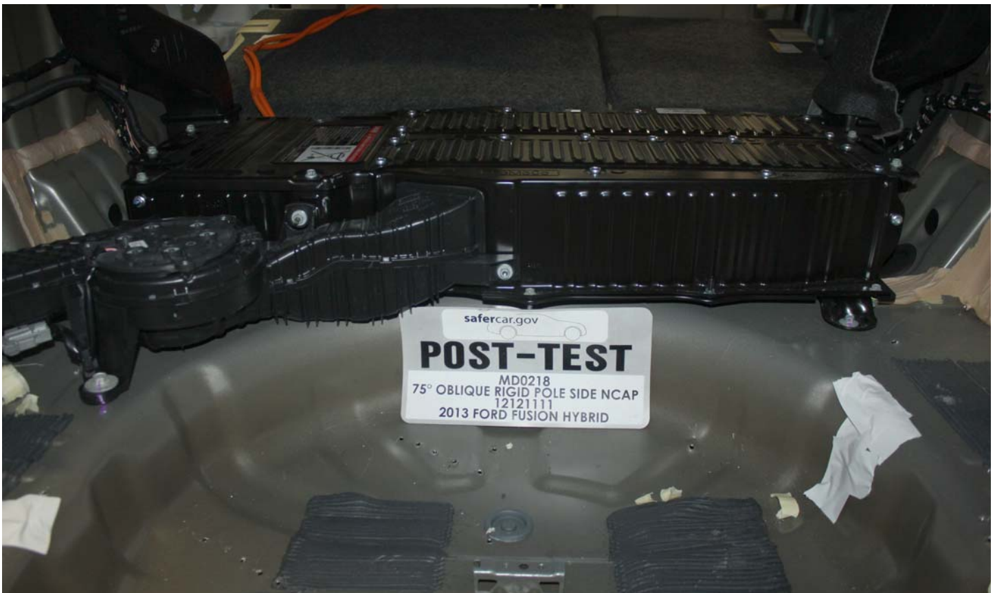
No. 011 Post-Impact Rear View of Propulsion Battery
