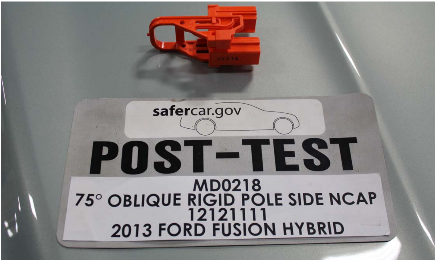
No. 008 Manual High Voltage Service Disconnect Removed
