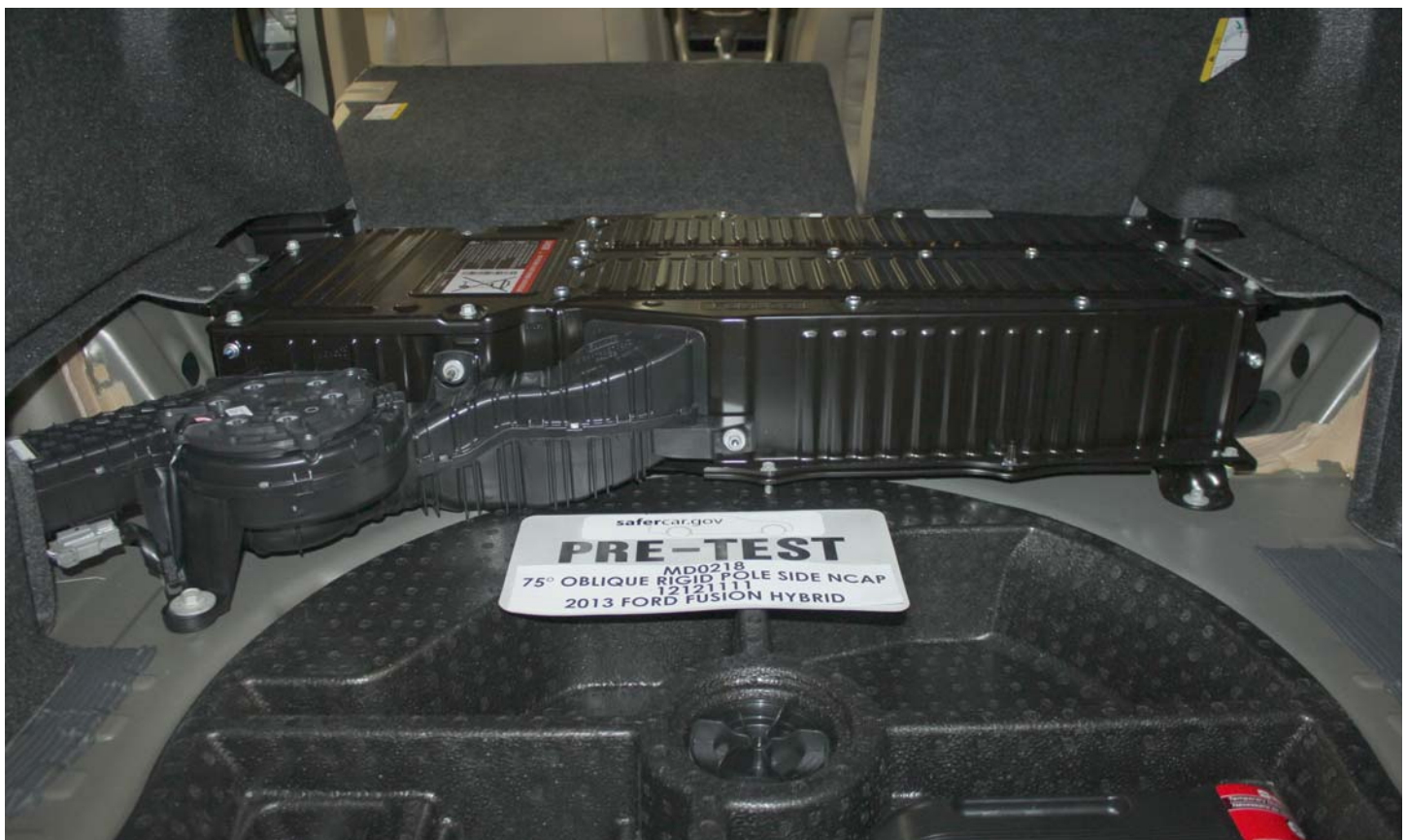
No. 009 Pre-Impact View of Propulsion Battery
