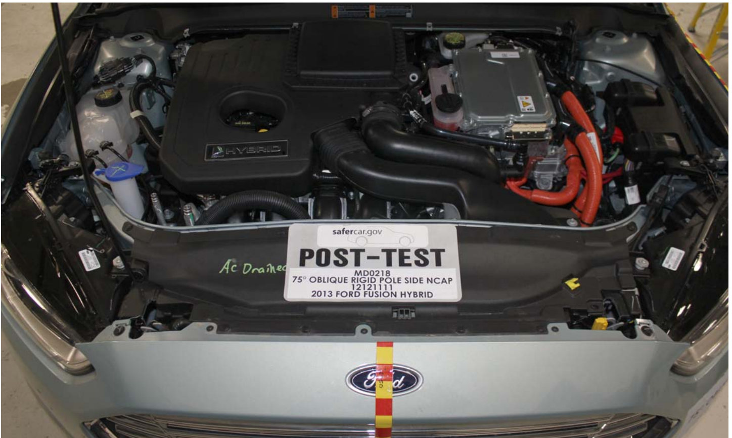
No. 017 Post-Impact View of Electric Propulsion Drive
