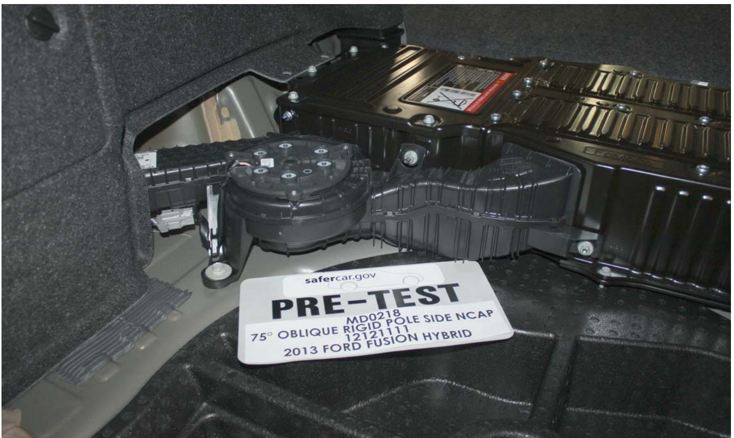
No. 019 Pre-Impact View Propulsion Battery Venting System(s)
