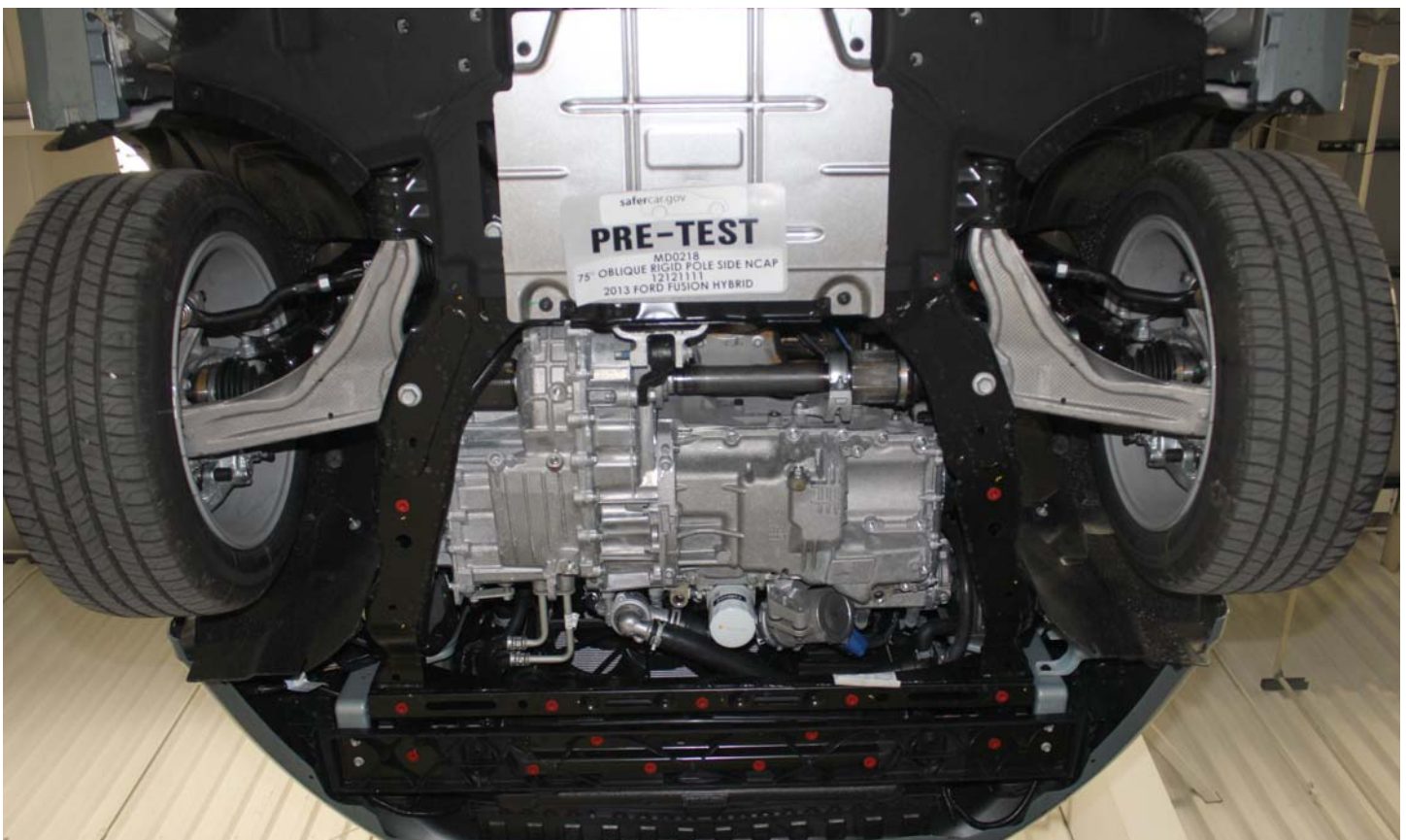
No. 016a Pre-Impact View of Electric Propulsion Drive
