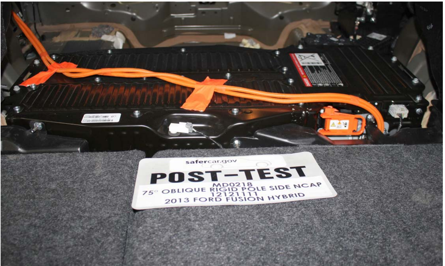
No. 010 Post-Impact Front View of Propulsion Battery
