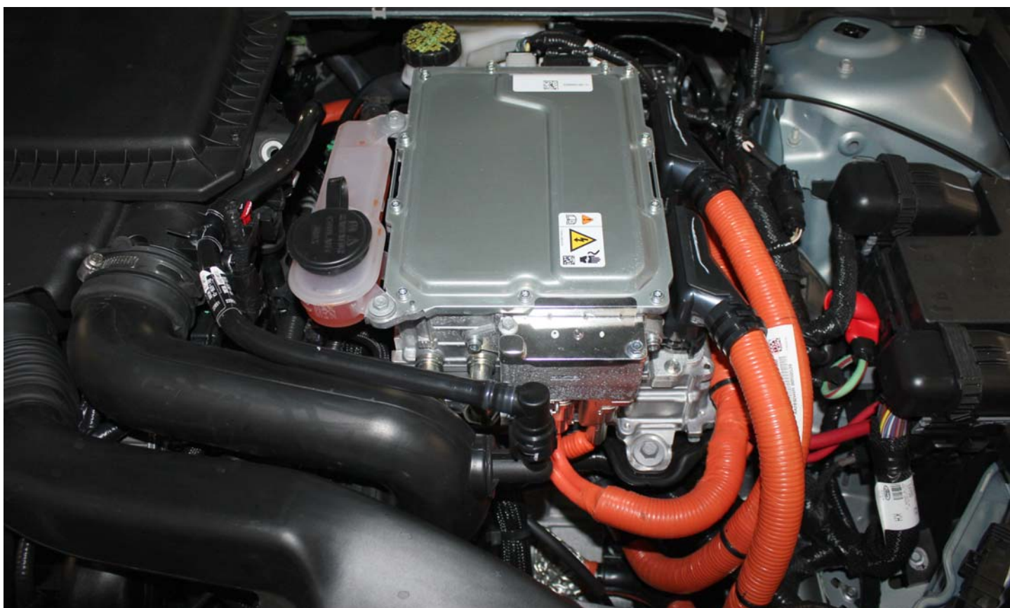
No. 002 Power Inverter Warning Label
