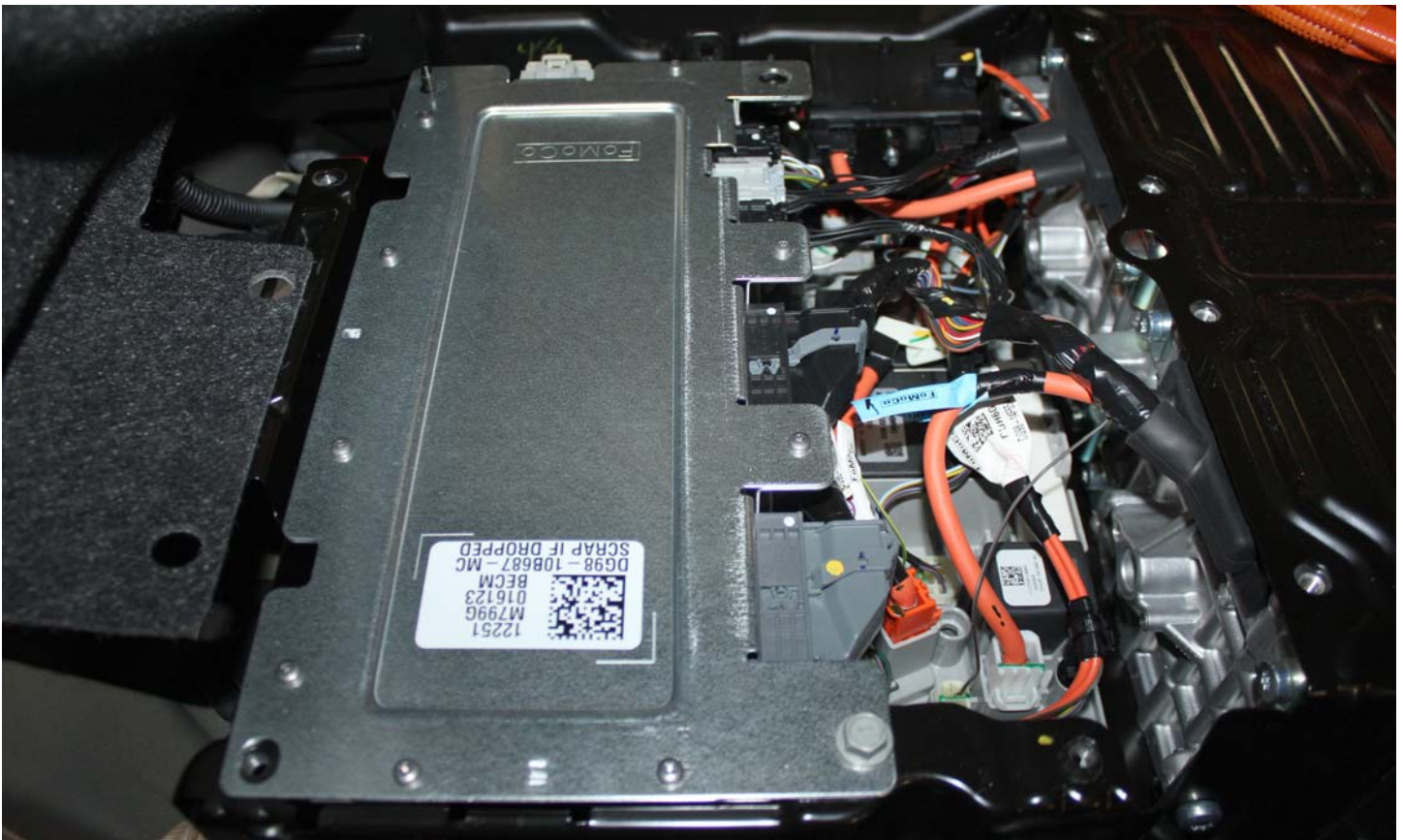
No. 018 Pre-Impact View of High Voltage Interconnect(s)
