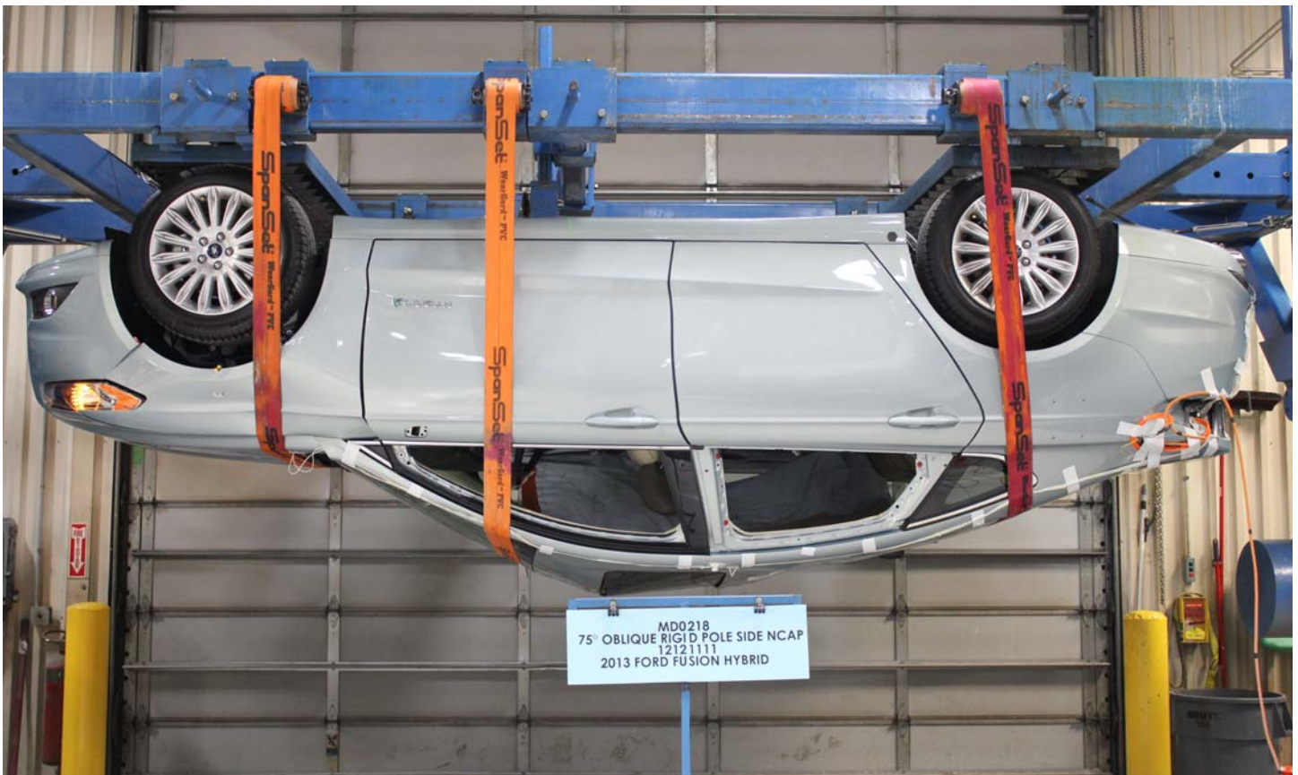
No. 029 FMVSS No. 305 Static Rollover at 180°
