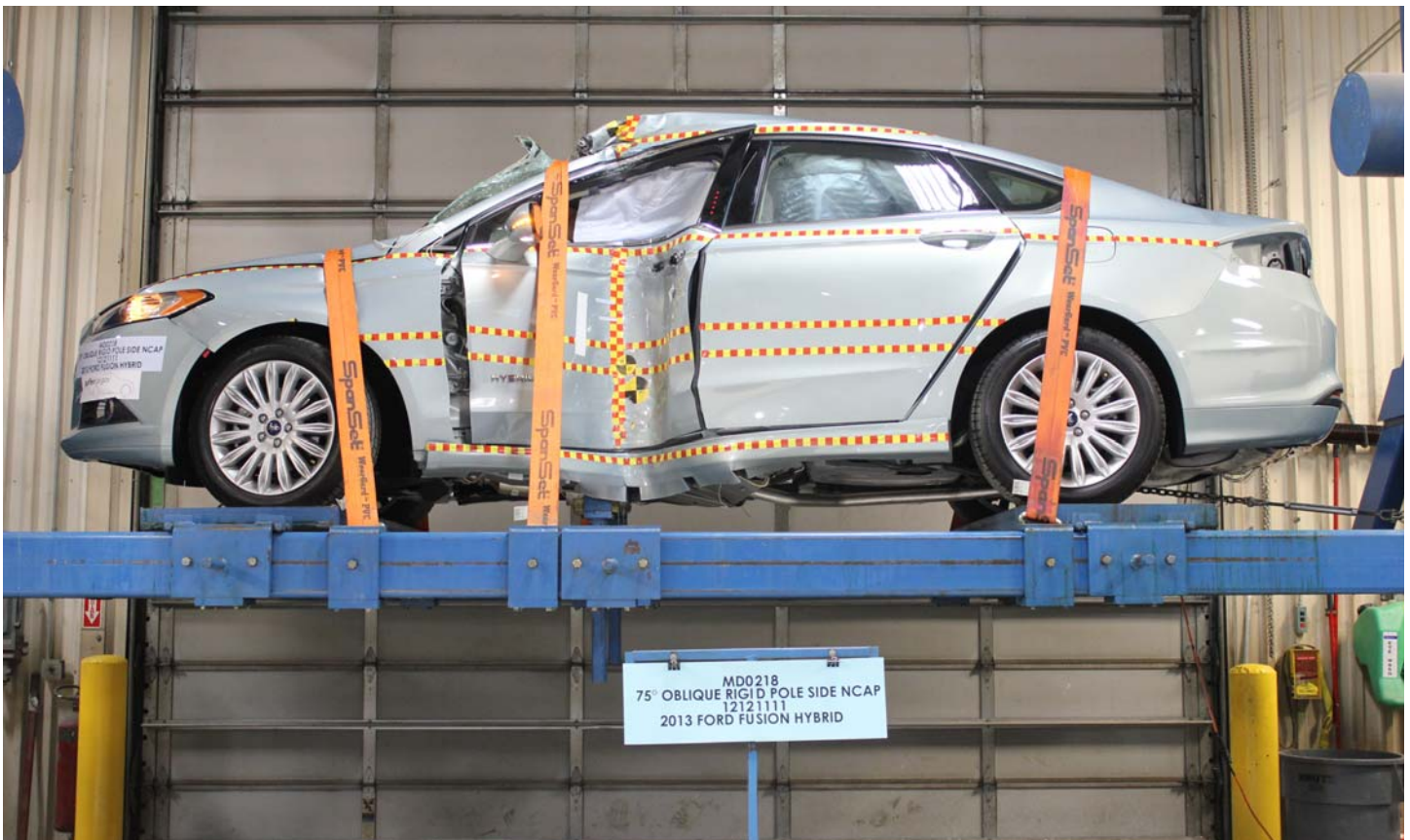
No. 031 FMVSS No. 305 Static Rollover at 360°
