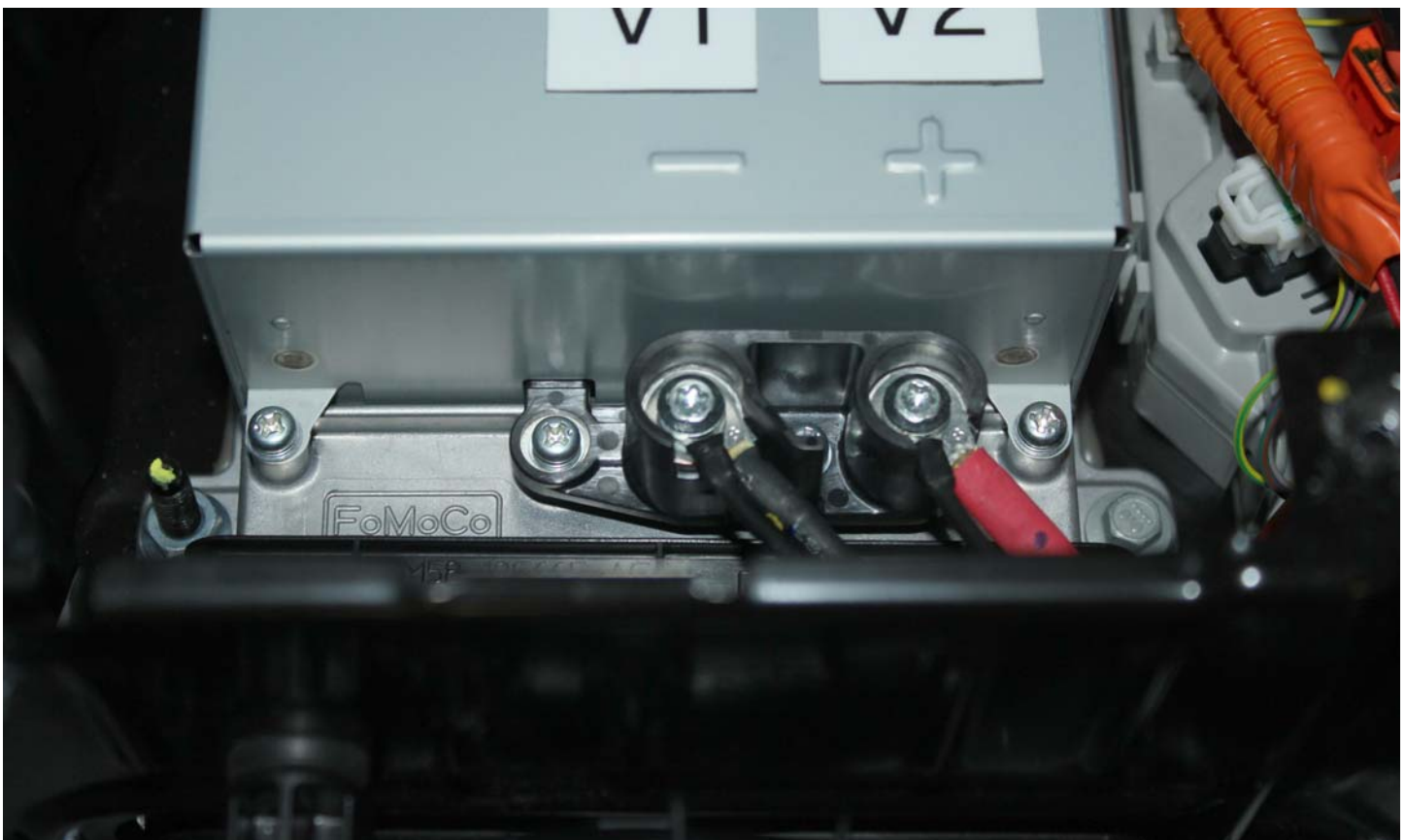
No. 023 Pre-Impact Close-Up View of High Voltage Leads Attached
