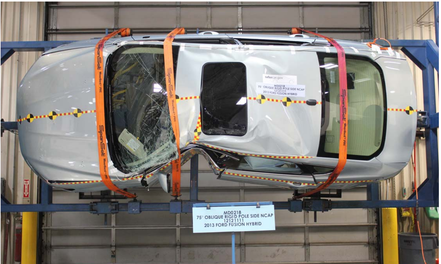
No. 028 FMVSS No. 305 Static Rollover at 90°
