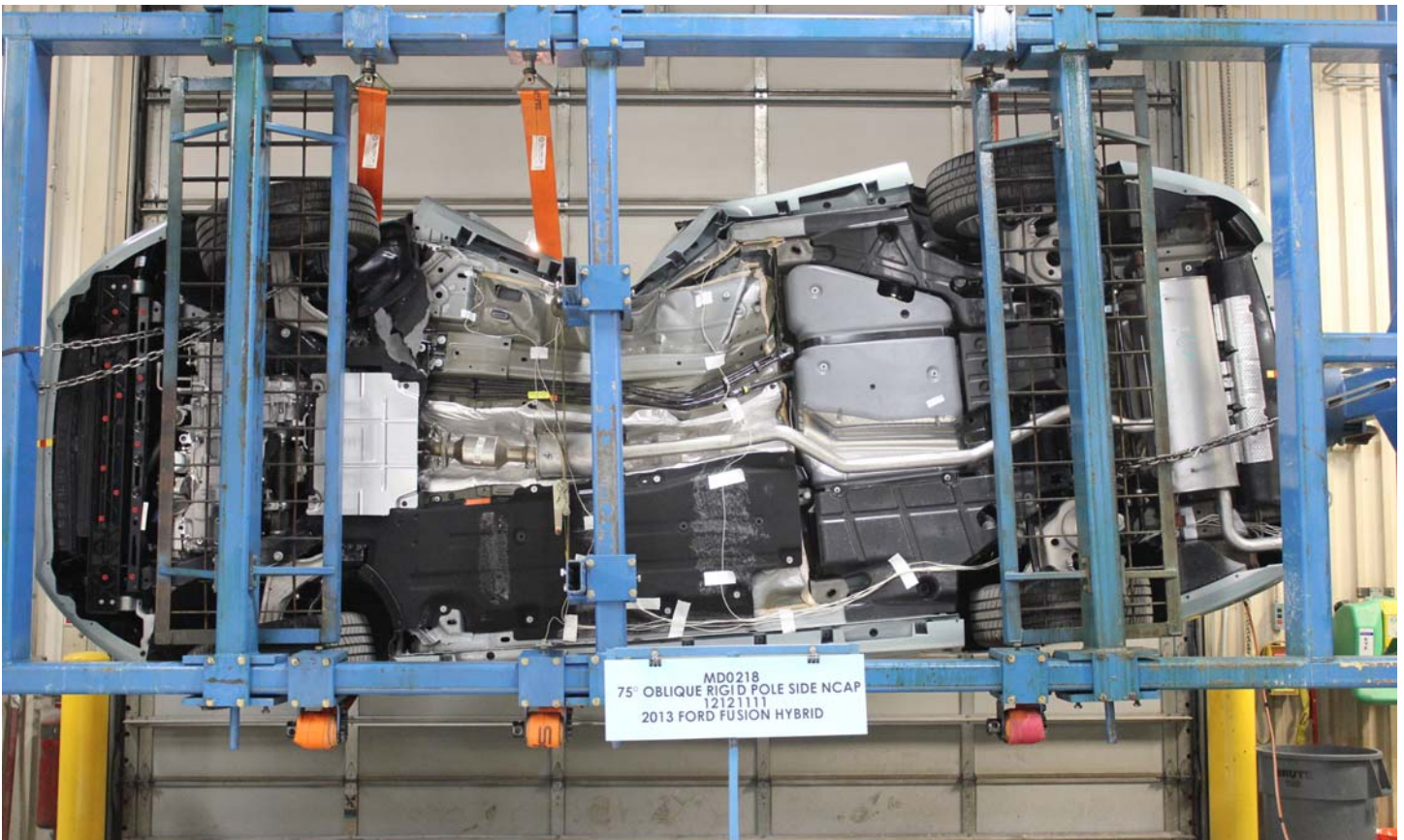
No. 030 FMVSS No. 305 Static Rollover at 270°
