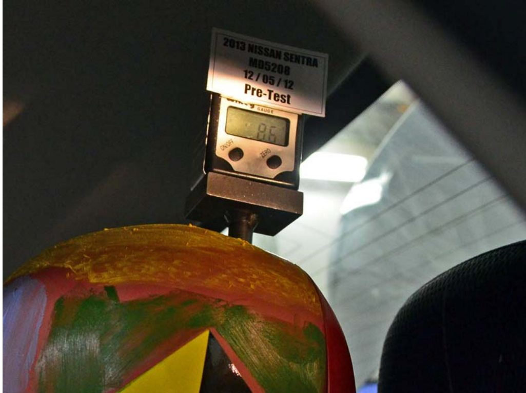
FIGURE 63. Pre-Test View of Rear Passenger Dummy's Head Showing Dummy's Head is Level
