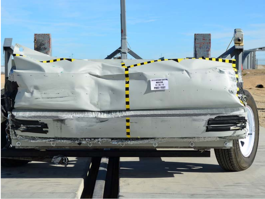
FIGURE 85. Post-Test Front View of MDB Impactor Face
