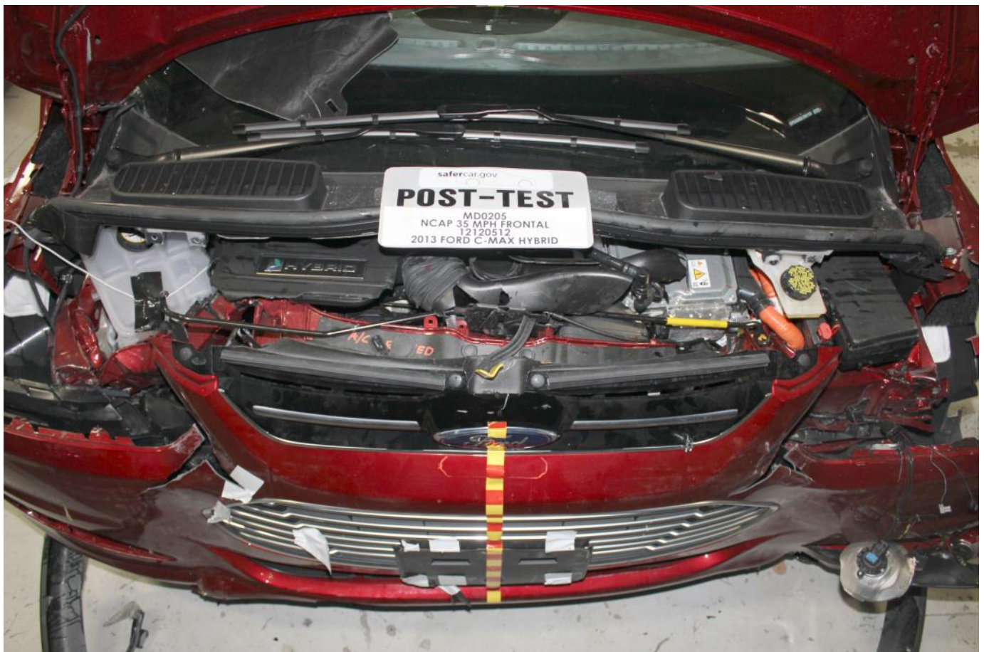
Post-Test Engine Compartment View
