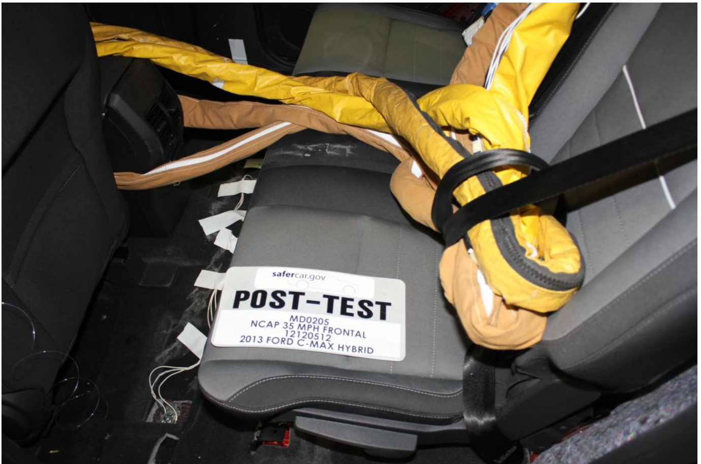
Post-Test Dummy Cable Routing
