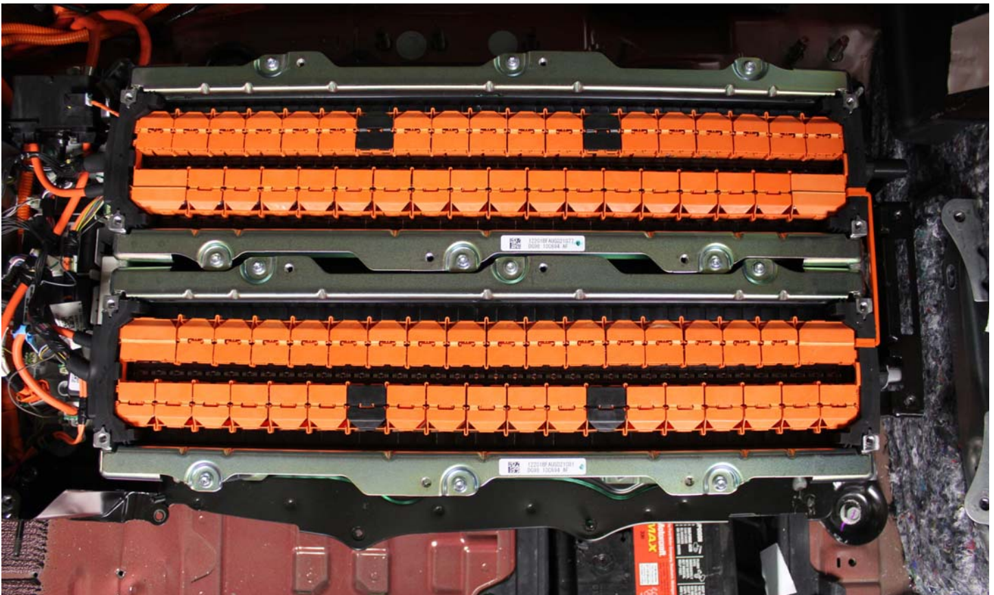
No. 015 Post-Impact View of Propulsion Battery Module(s)
