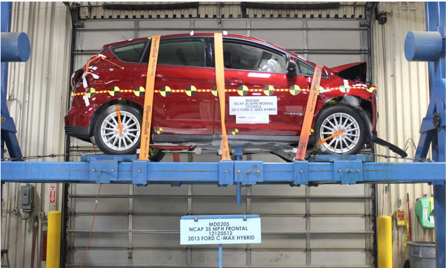
No. 031 FMVSS No. 305 Static Rollover at 360°
