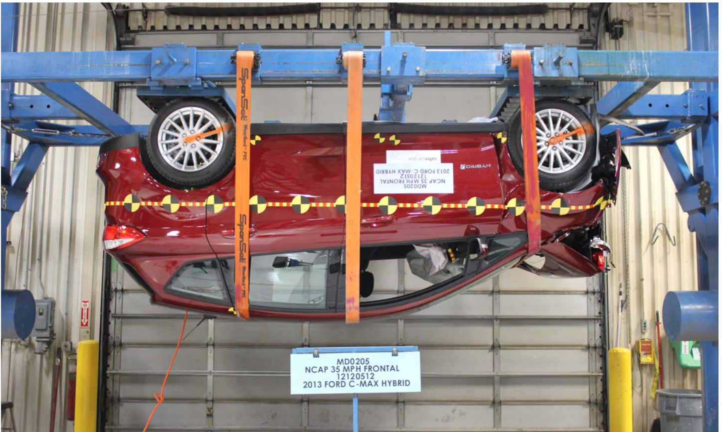
No. 029 FMVSS No. 305 Static Rollover at 180°
