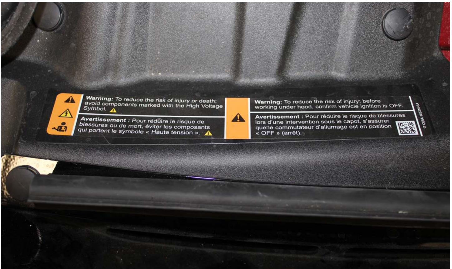
No. 005a Other Vehicle Label(s) Related to Electrical Propulsion System
