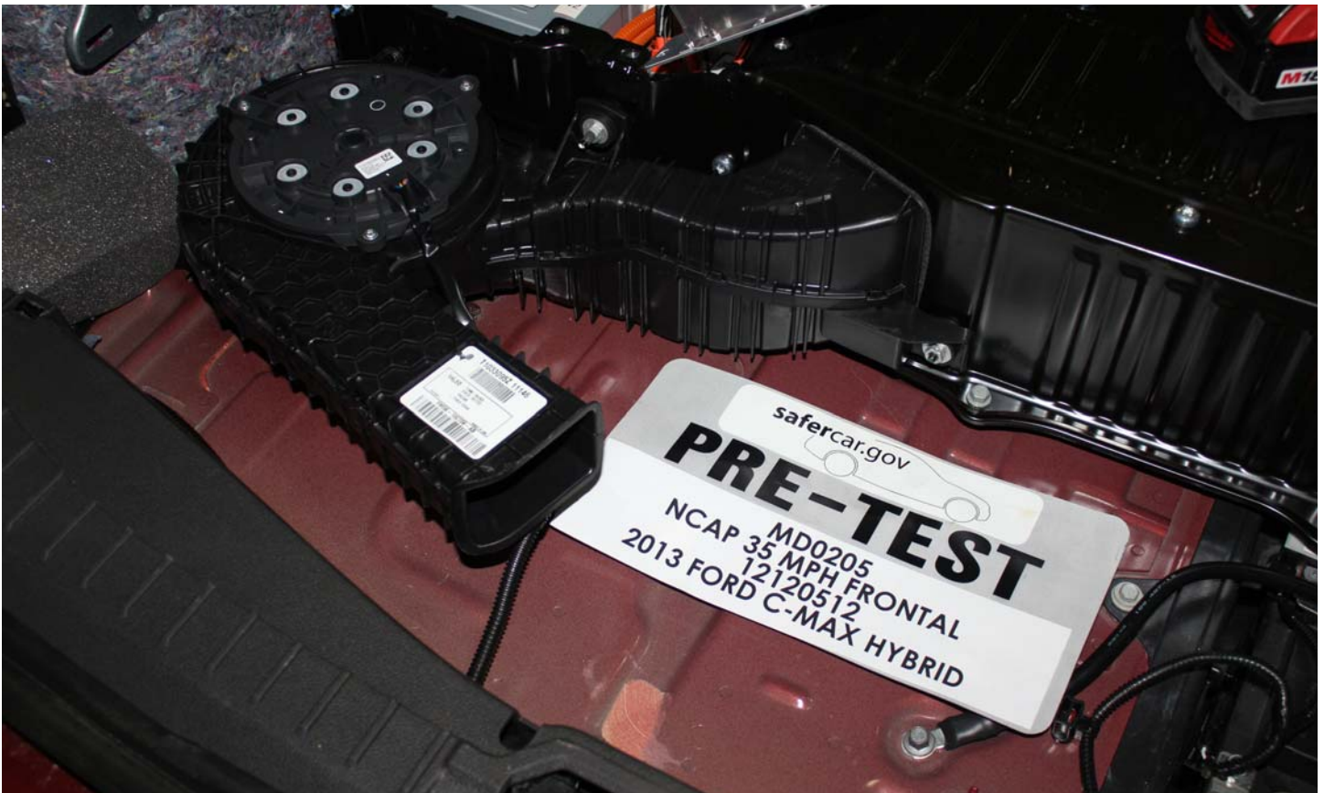
No. 019 Pre-Impact View Propulsion Battery Venting System(s)
