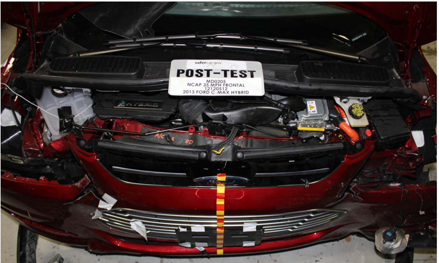
No. 017 Post-Impact View of Electric Propulsion Drive
