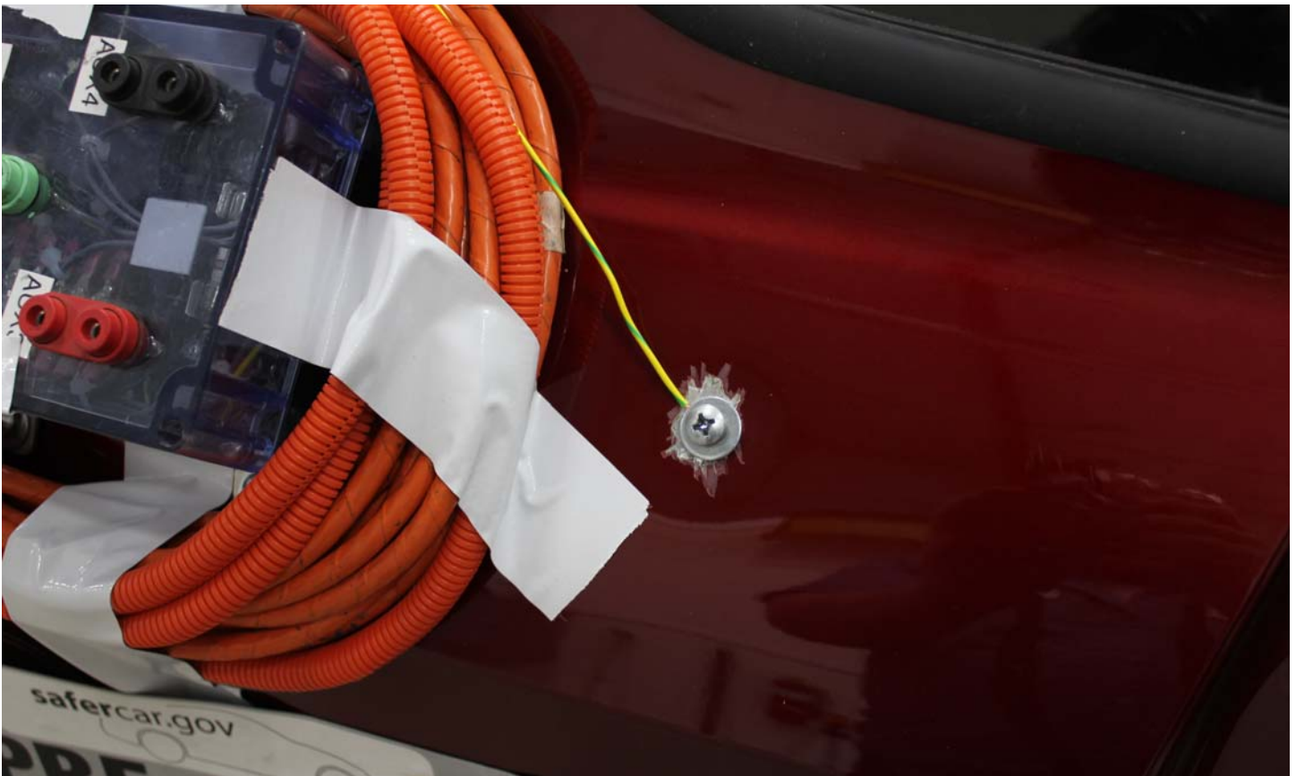
No. 021 Pre-Impact View of Ground Lead Attached
