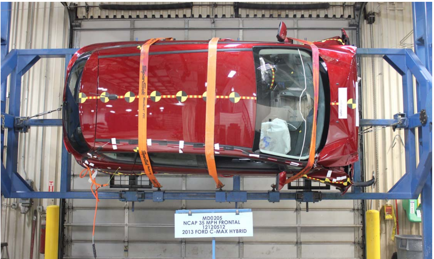
No. 028 FMVSS No. 305 Static Rollover at 90°
