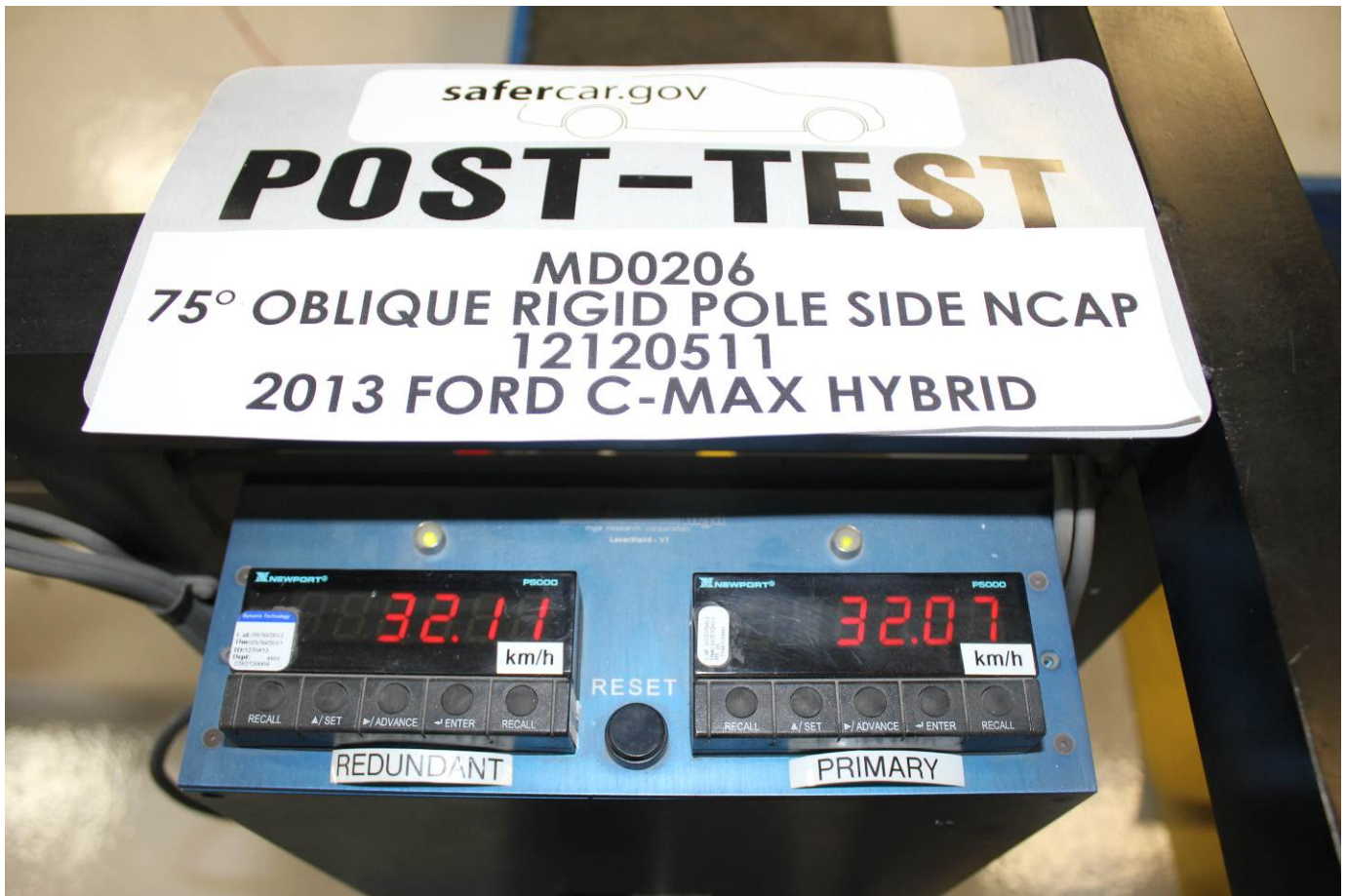
Post-Test Primary and Redundant Speed Trap Read-Out
