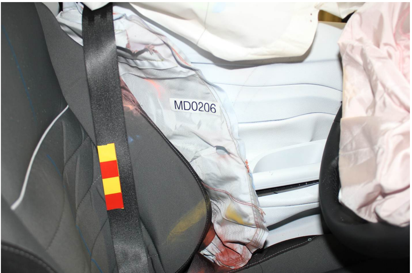
Post-Test Dummy Close-Up Torso Contact with Side Air Bag View
