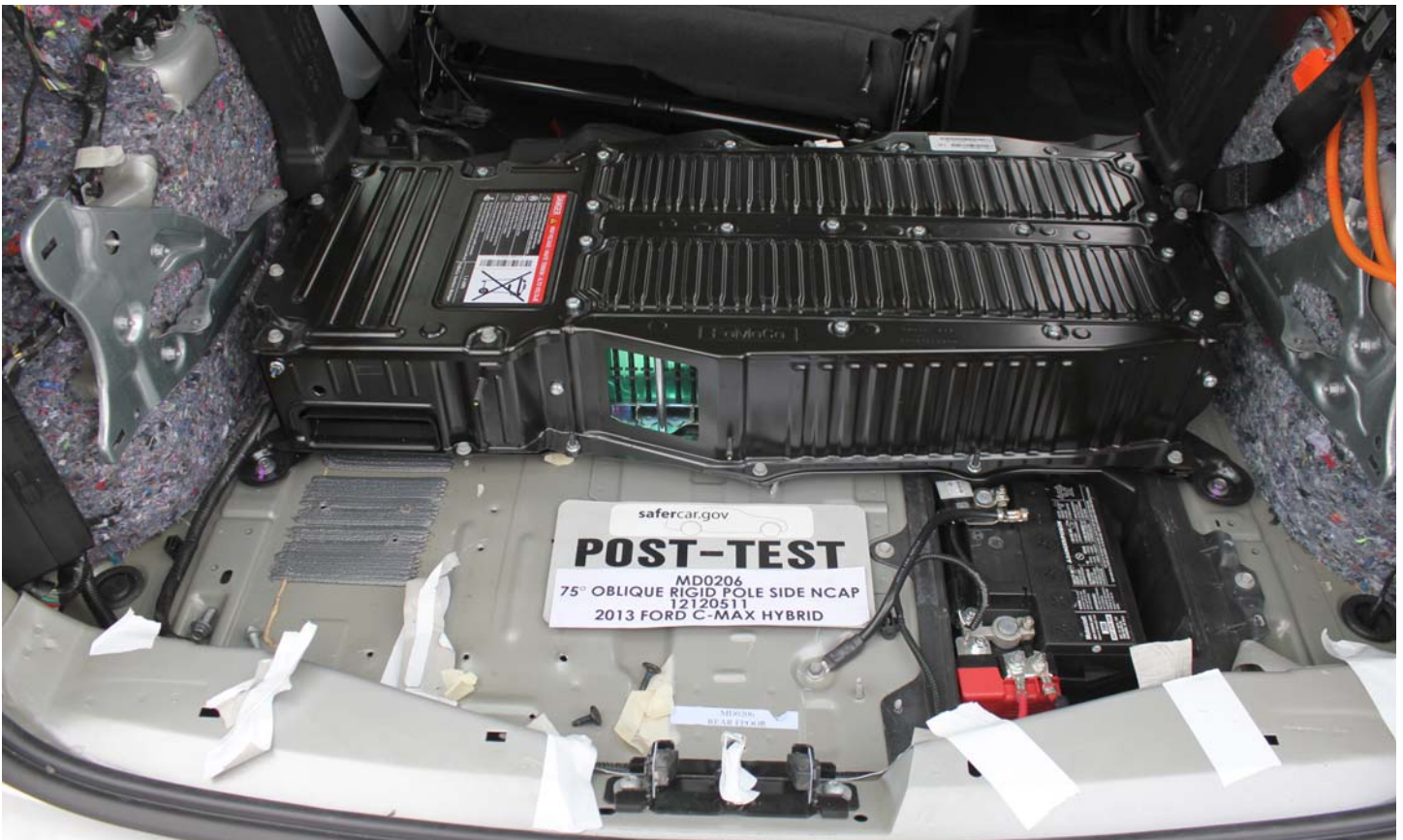
No. 011 Post-Impact Rear View of Propulsion Battery
