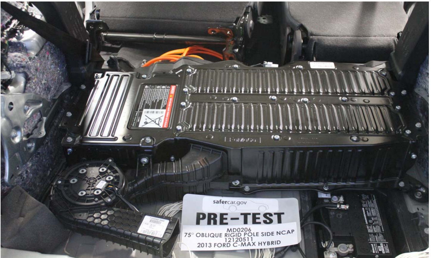
No. 019 Pre-Impact View Propulsion Battery Venting System(s)
