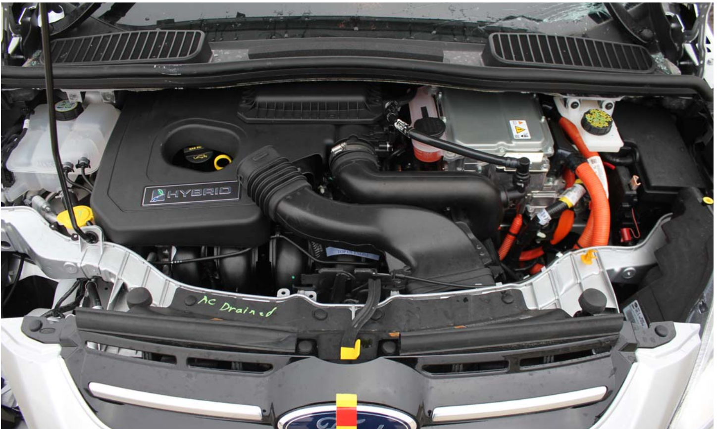
No. 017 Post-Impact View of Electric Propulsion Drive
