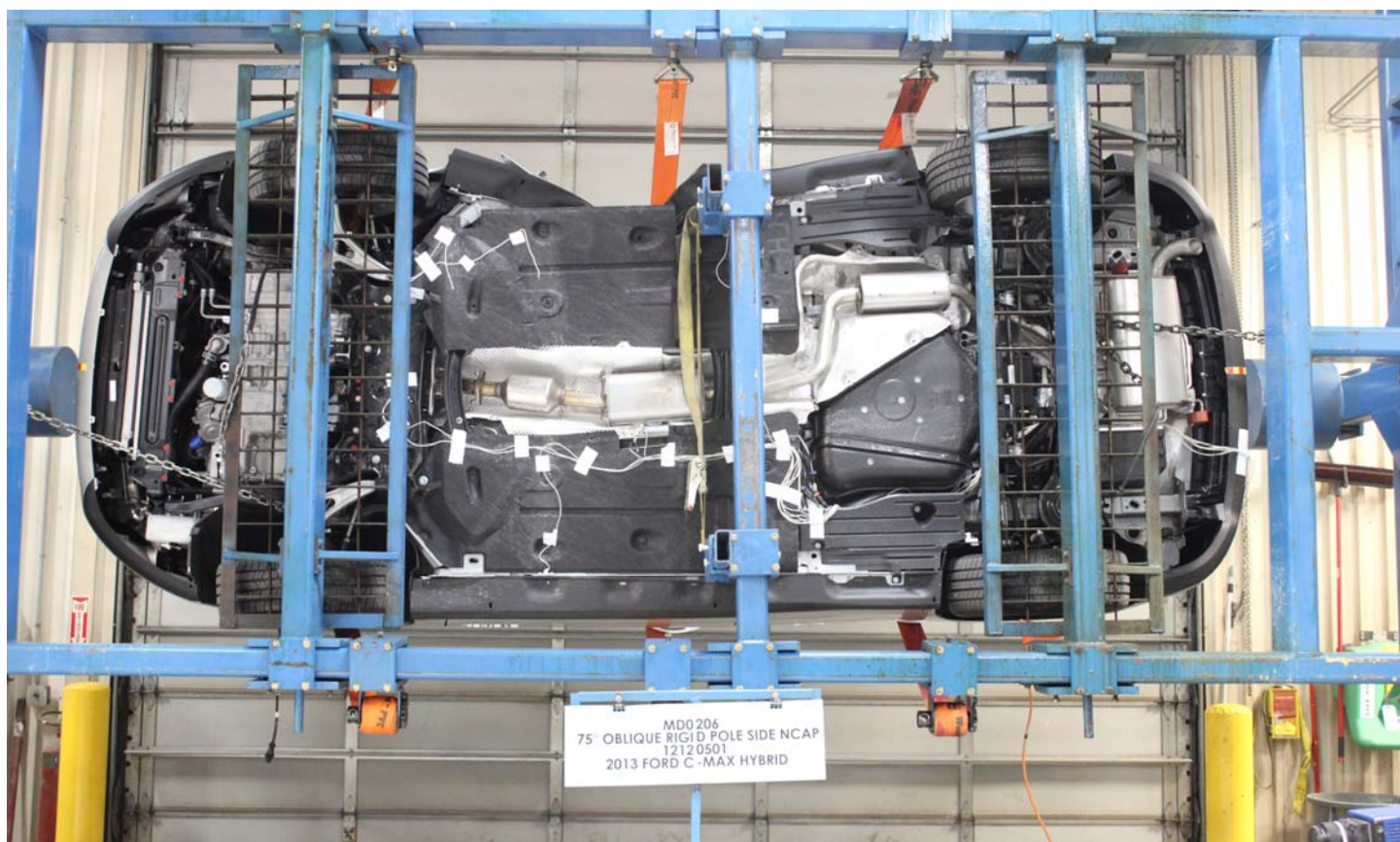
No. 028 FMVSS No. 305 Static Rollover at 90°
