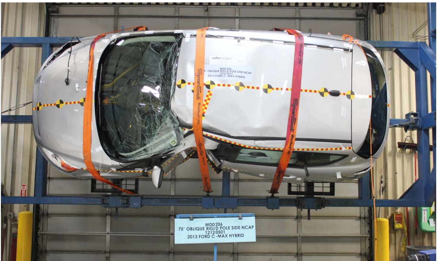
No. 030 FMVSS No. 305 Static Rollover at 270°
