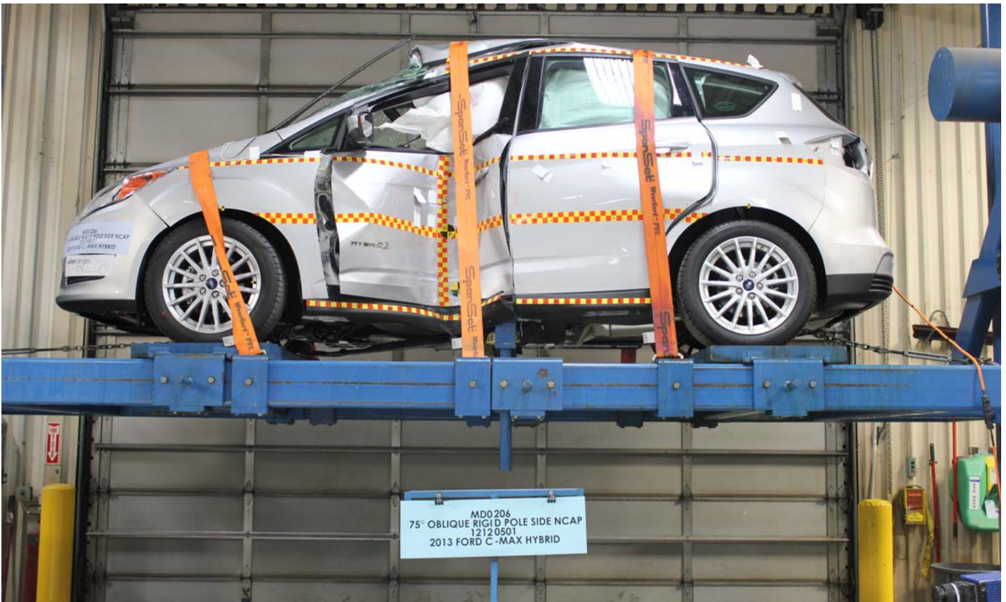
No. 031 FMVSS No. 305 Static Rollover at 360°
