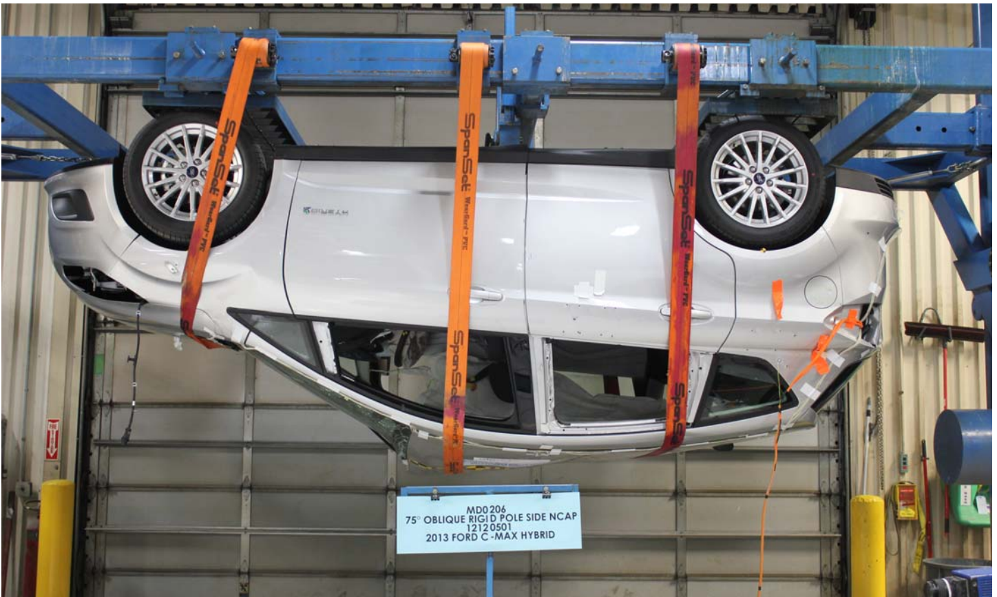
No. 029 FMVSS No. 305 Static Rollover at 180°
