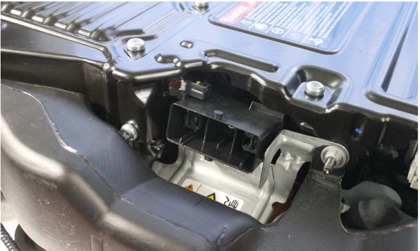
No. 007 Manual High Voltage Service Disconnect Removed
