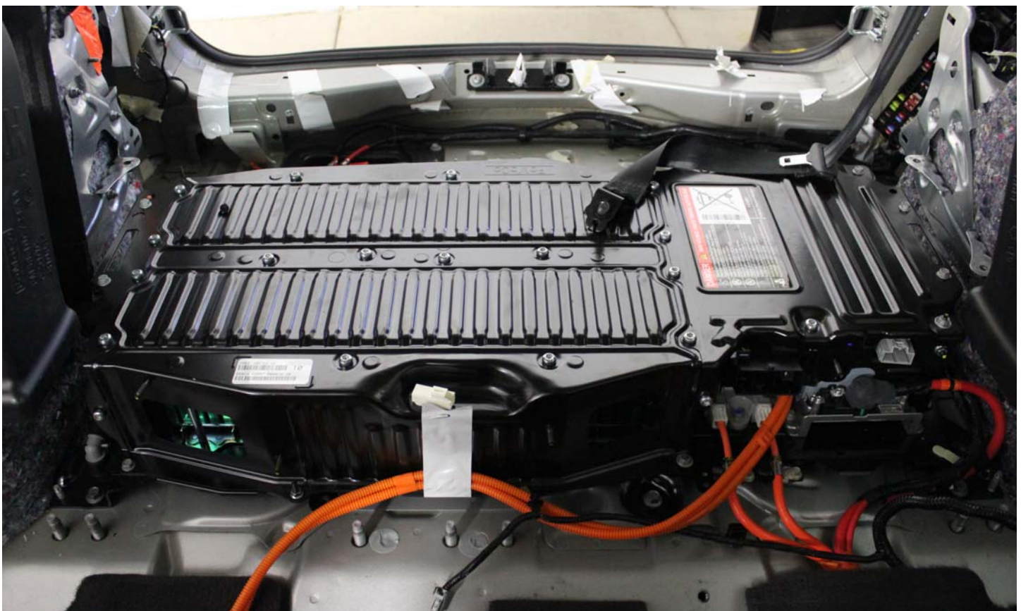
No. 010 Post-Impact Front View of Propulsion Battery
