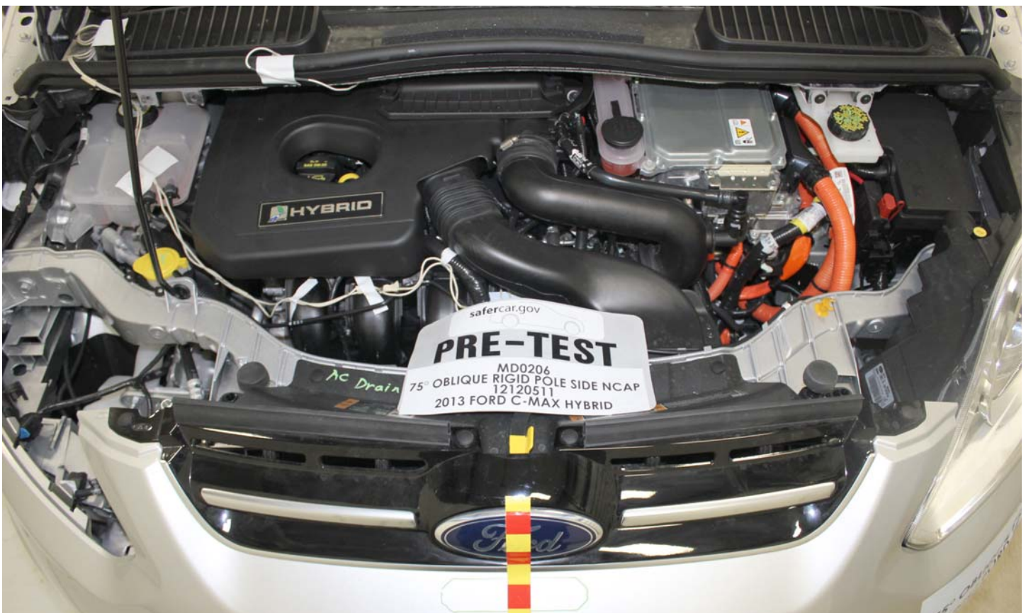
No. 016 Pre-Impact View of Electric Propulsion Drive
