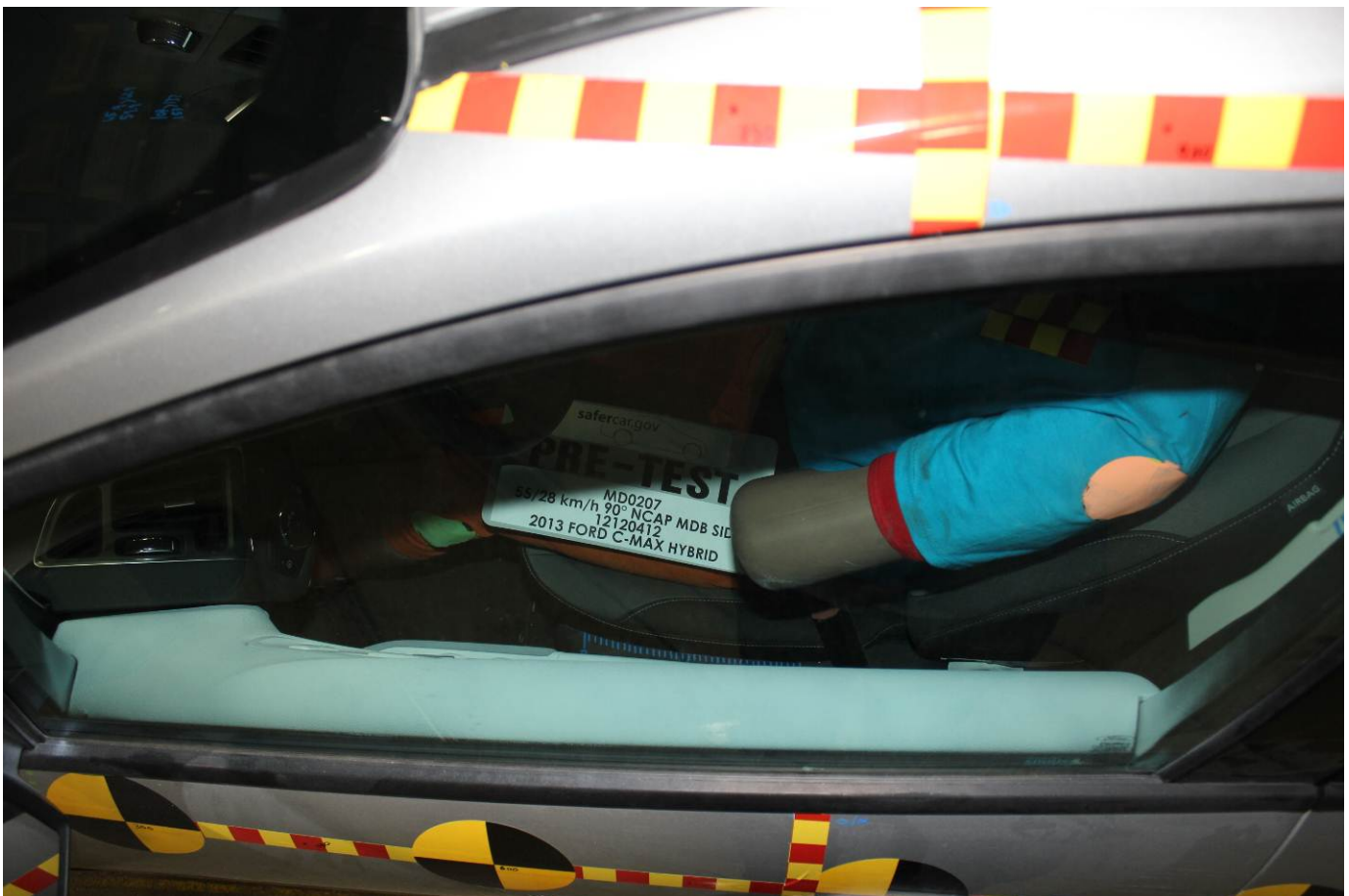
Pre-Test Driver Dummy and Door Clearance View
