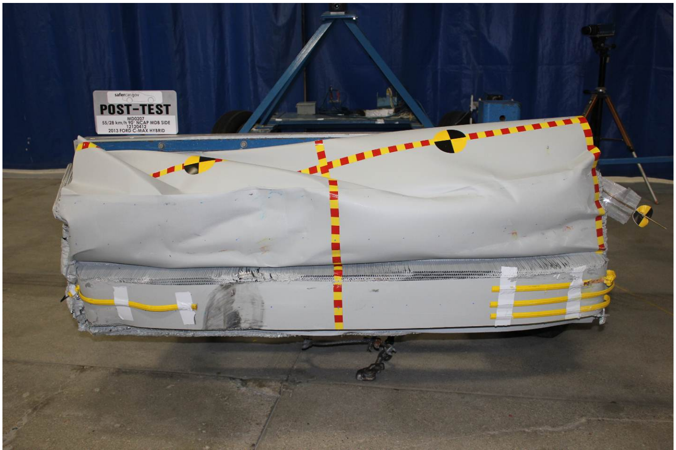
Post-Test Front View of MDB Impactor Face
