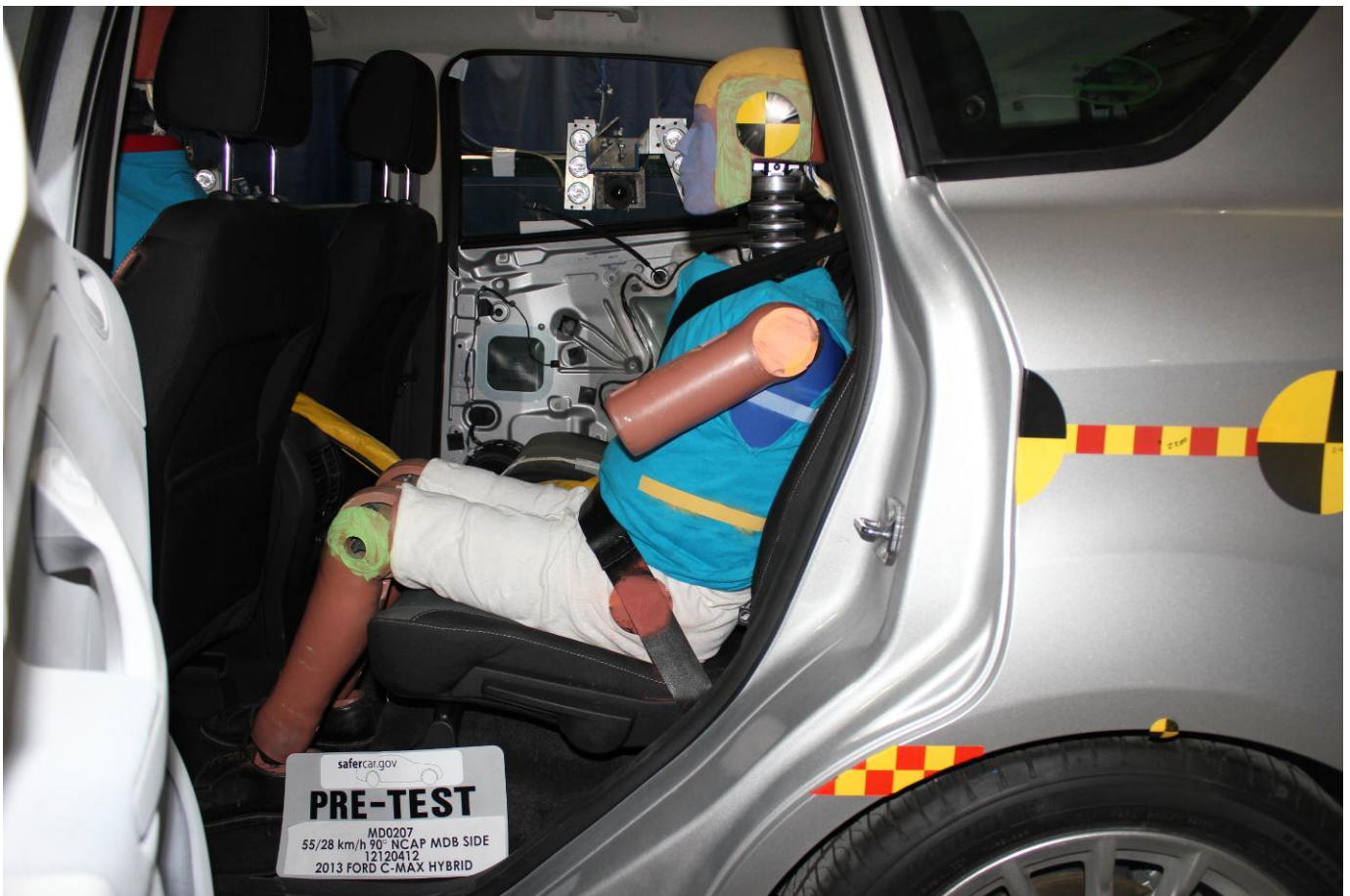
Pre-Test Left Side View of Rear Passenger Dummy Showing Belt and Chalking
