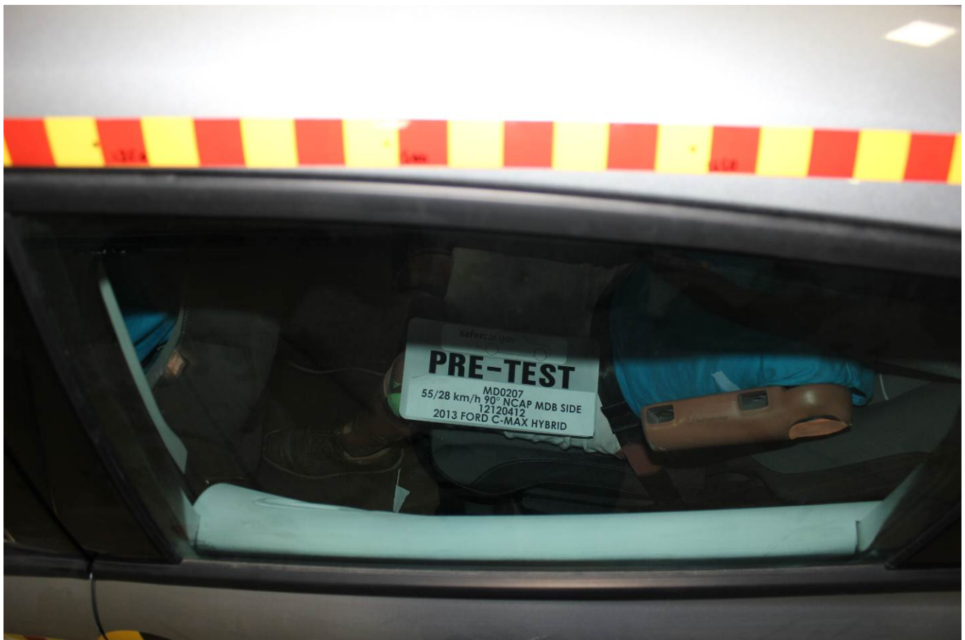
Pre-Test Rear Passenger Dummy and Door Clearance View
