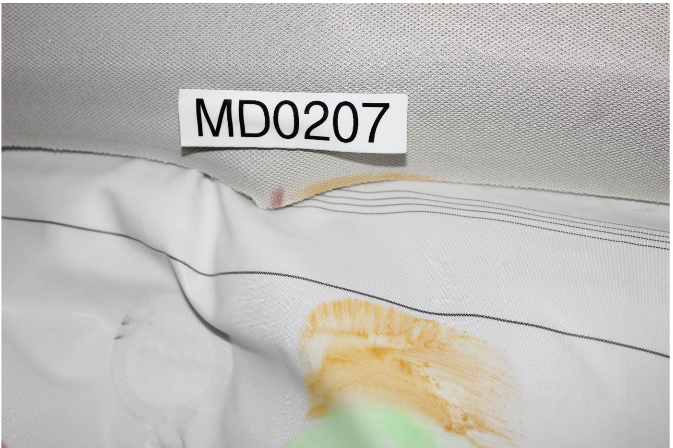
Post-Test Driver Dummy Close-up Head Contact with Vehicle Interior View
