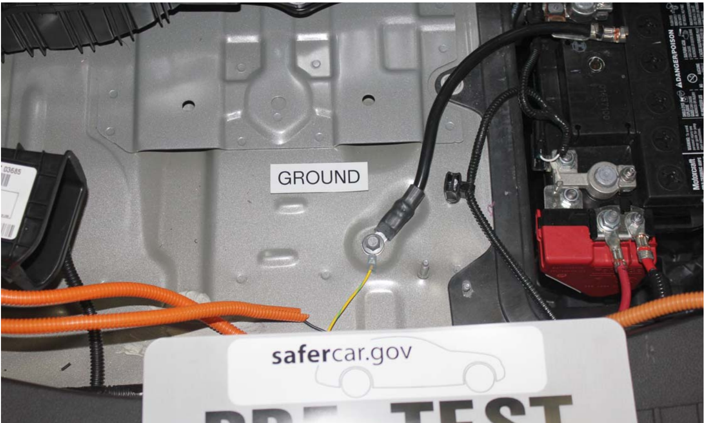
No. 021 Pre-Impact View of Ground Lead Attached
