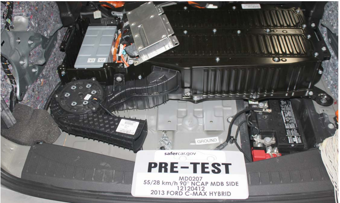
No. 019 Pre-Impact View Propulsion Battery Venting System(s)
