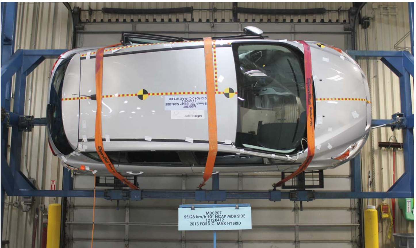
No. 028 FMVSS No. 305 Static Rollover at 90°
