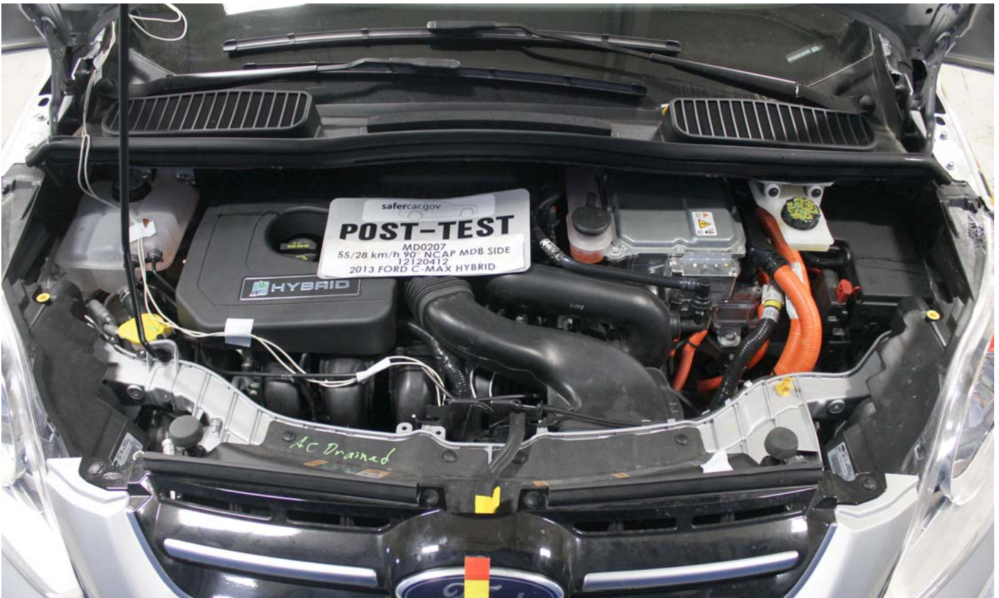
No. 017 Post-Impact View of Electric Propulsion Drive
