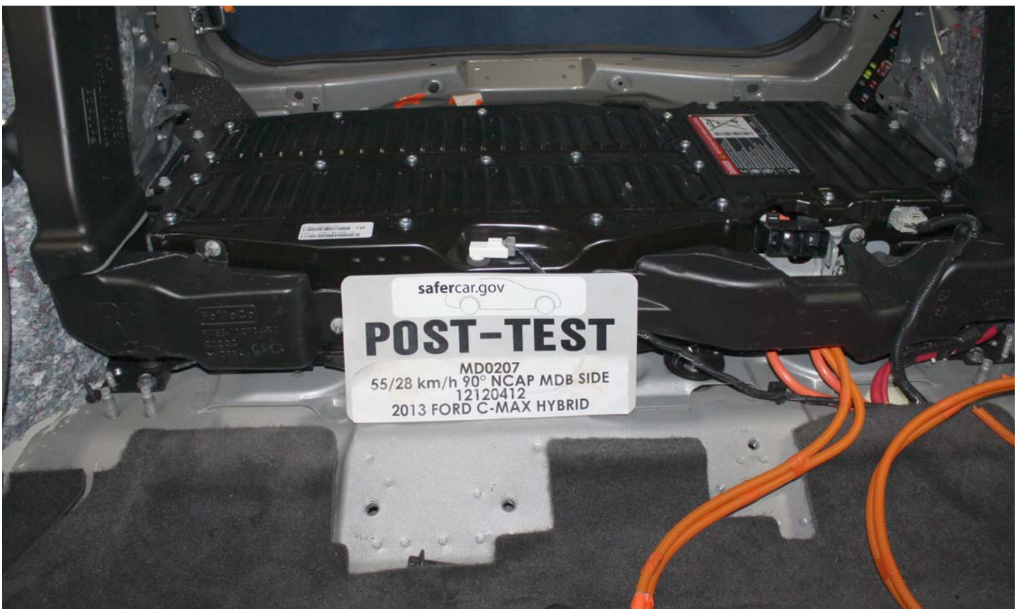
No. 010 Post-Impact Front View of Propulsion Battery
