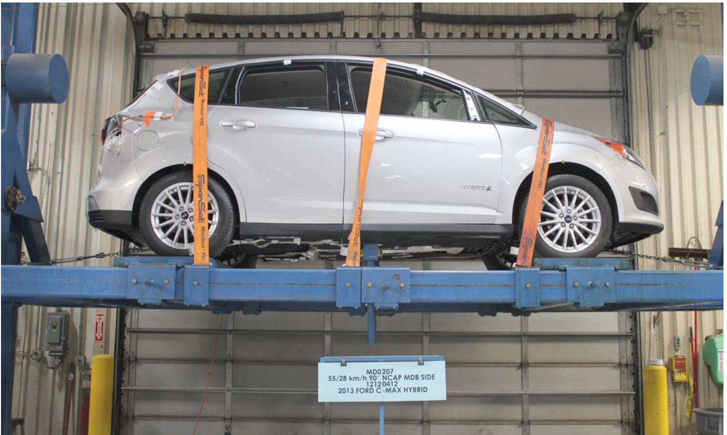
No. 031 FMVSS No. 305 Static Rollover at 360°
