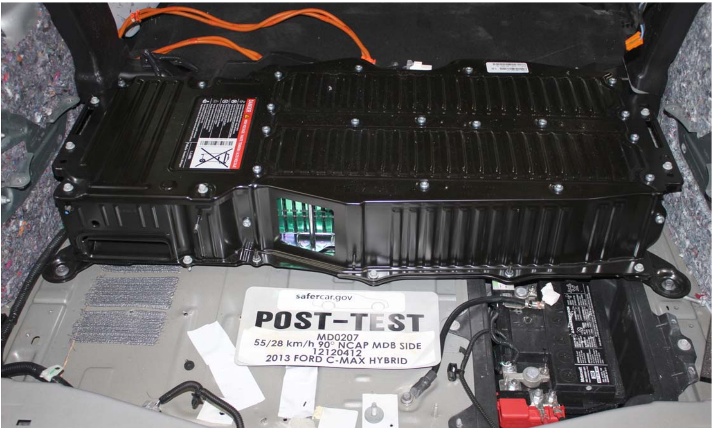
No. 011 Post-Impact Rear View of Propulsion Battery
