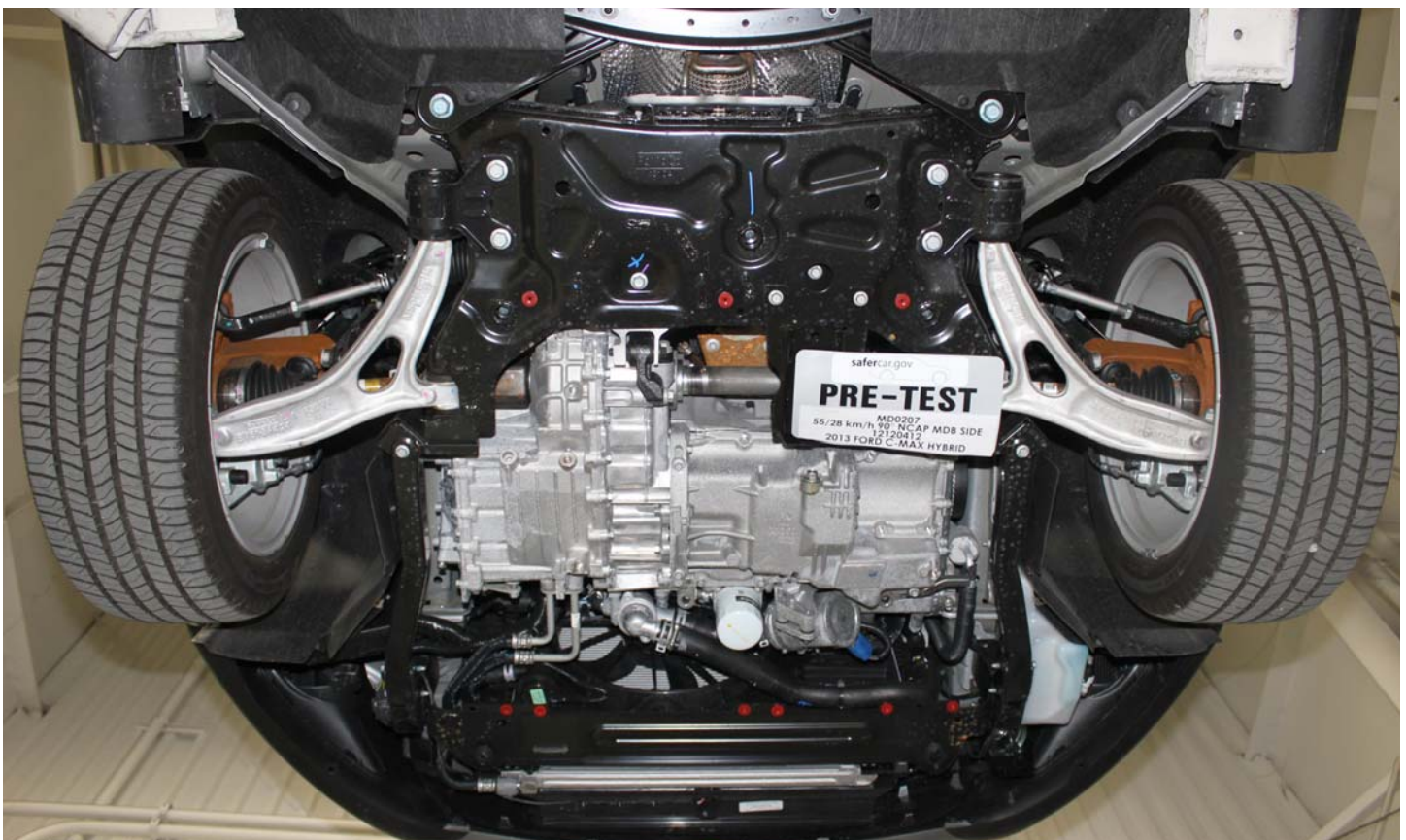
No. 020 Pre-Impact View of Other Visible Electric Propulsion Components
