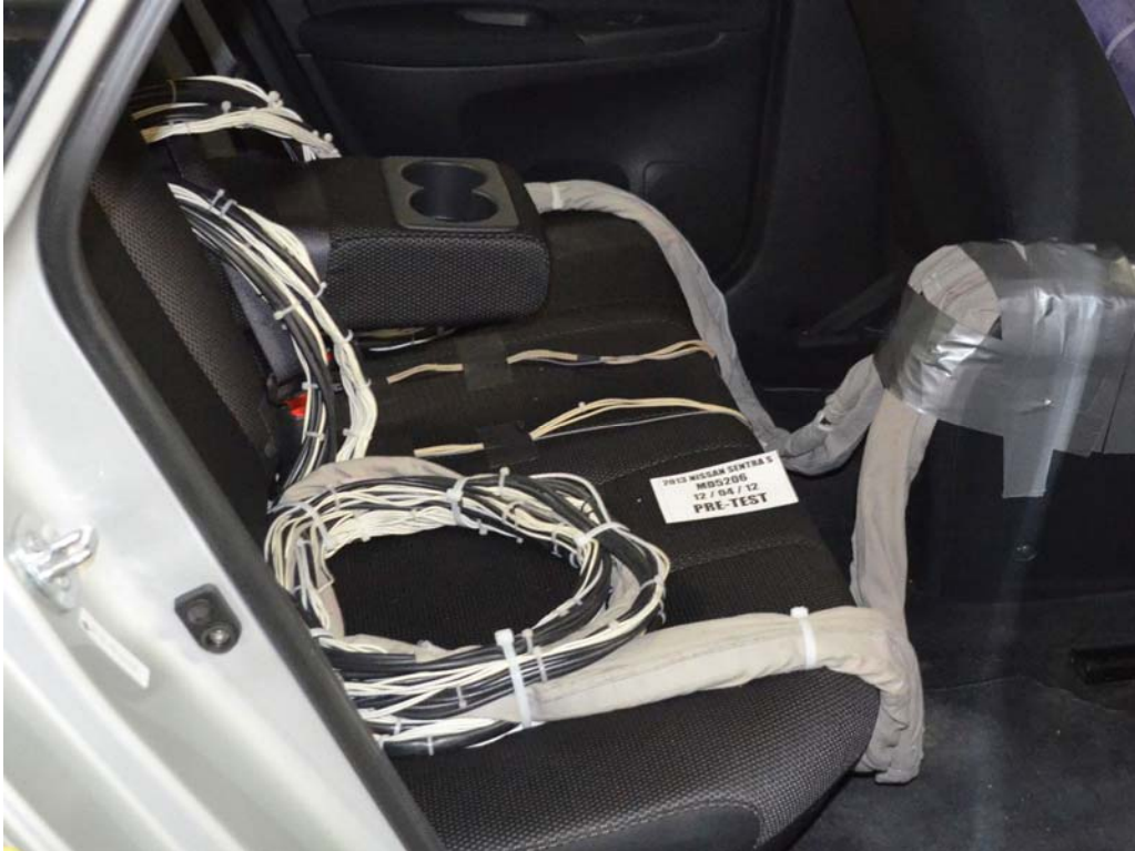
FIGURE 27. Pre-Test Dummy Cable Routing
