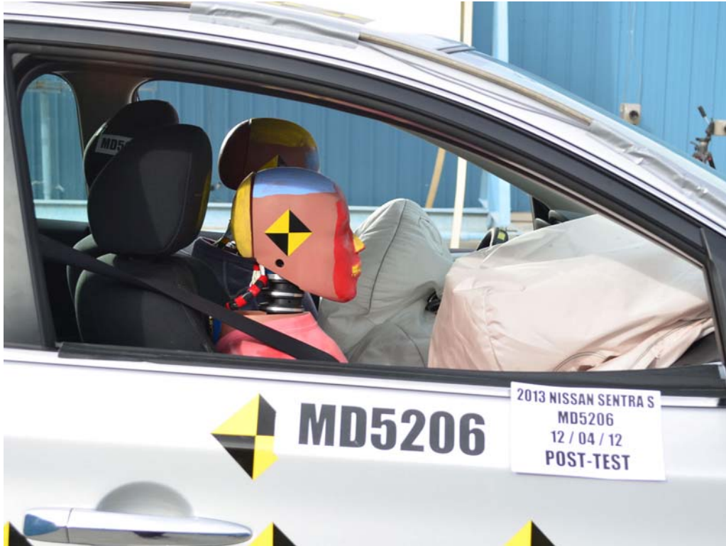
FIGURE 53. Post-Test Passenger Dummy Window View
