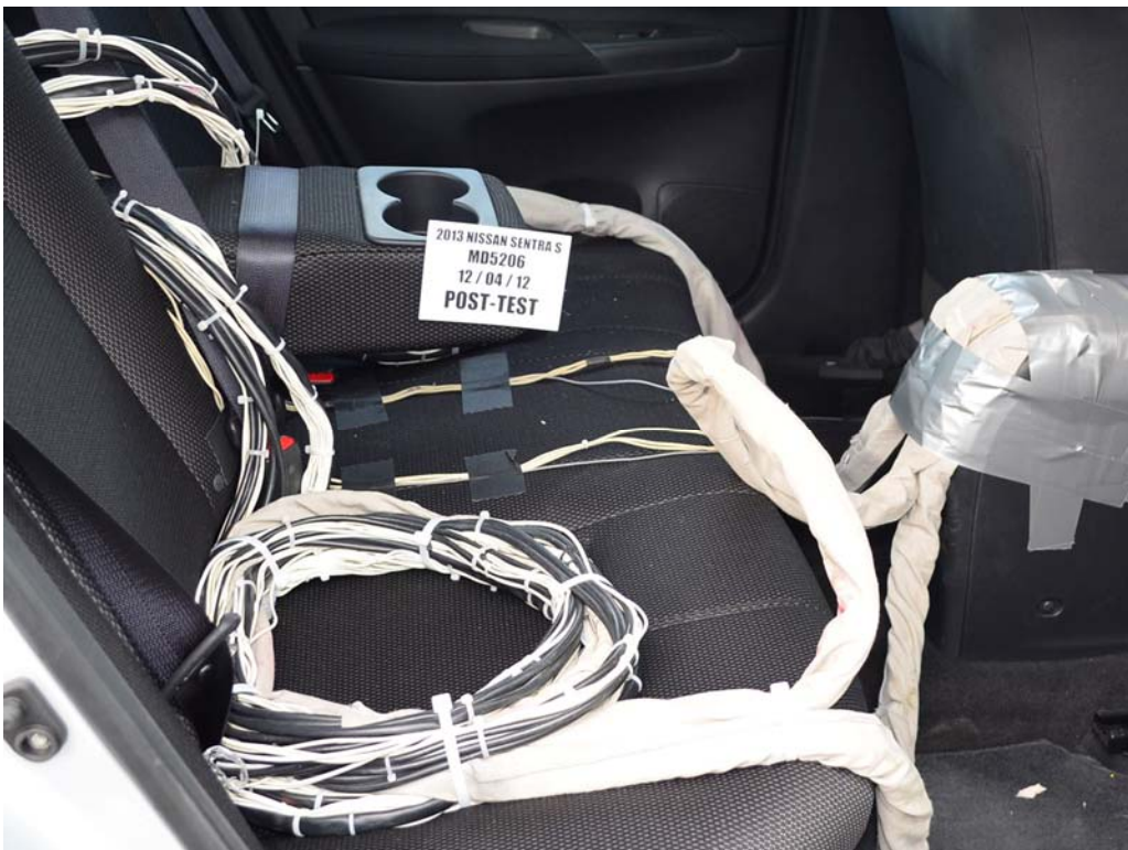
FIGURE 28. Post-Test Dummy Cable Routing
