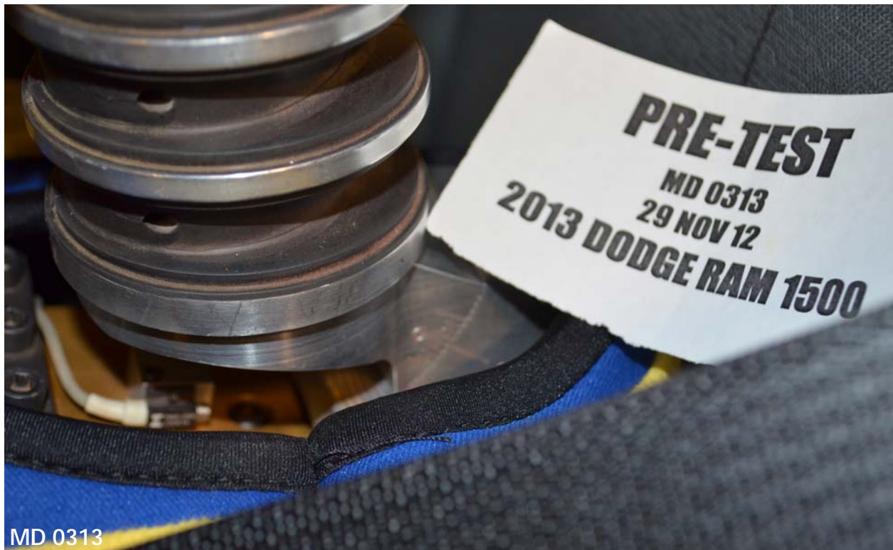
Figure 030: Pre-Test Left Side View of Dummy's Neck Showing Position of Adjustable Neck Bracket
