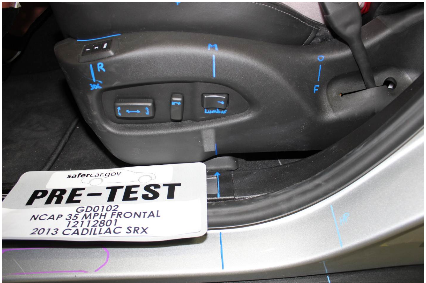
Pre-Test Driver's Seat Fore-Aft Markings
