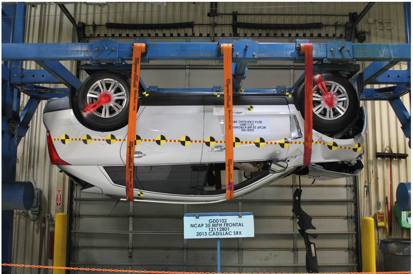
Vehicle at 180° on Static Rollover Device
