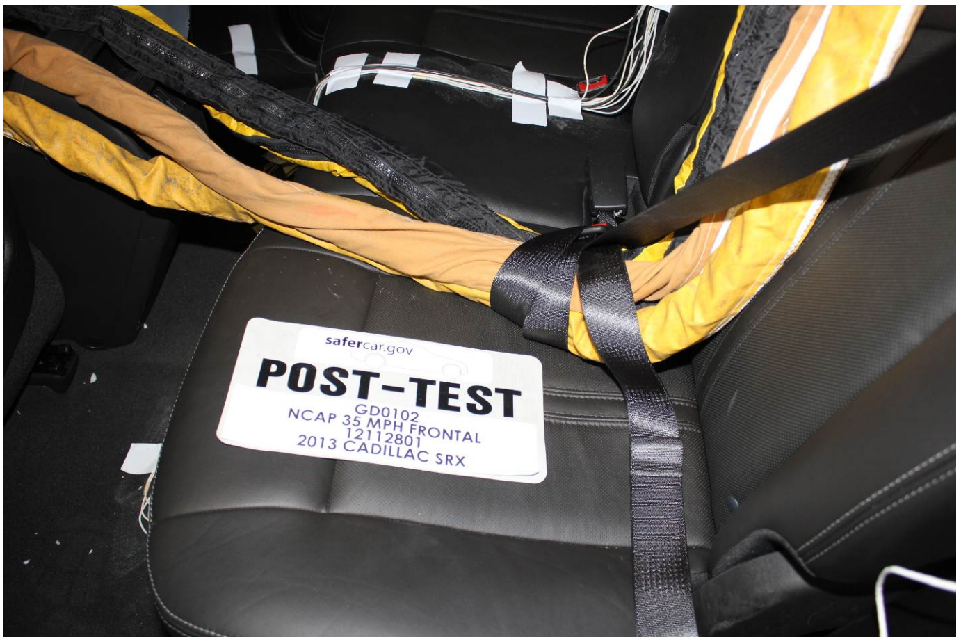
Post-Test Dummy Cable Routing
