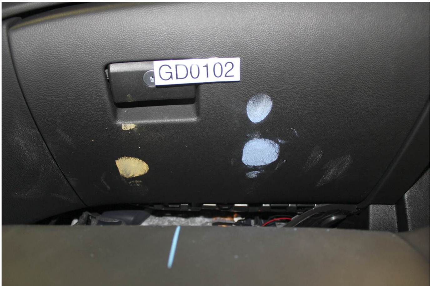
Post-Test Passenger Dummy Contact with Glovebox
