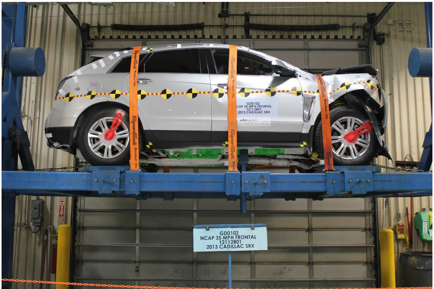
Vehicle at 360° on Static Rollover Device
