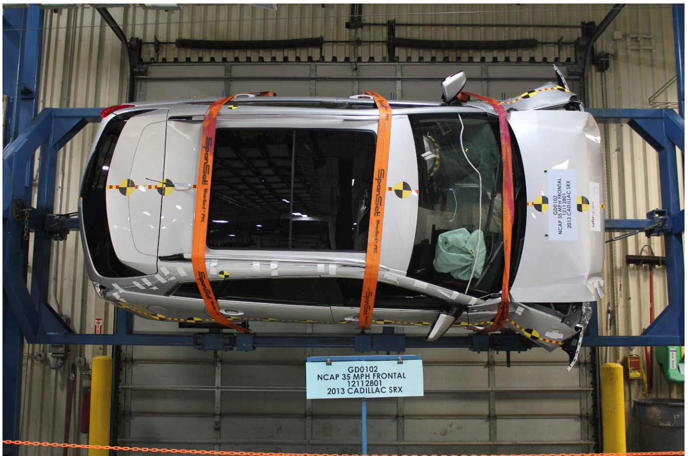
Vehicle at 90° on Static Rollover Device
