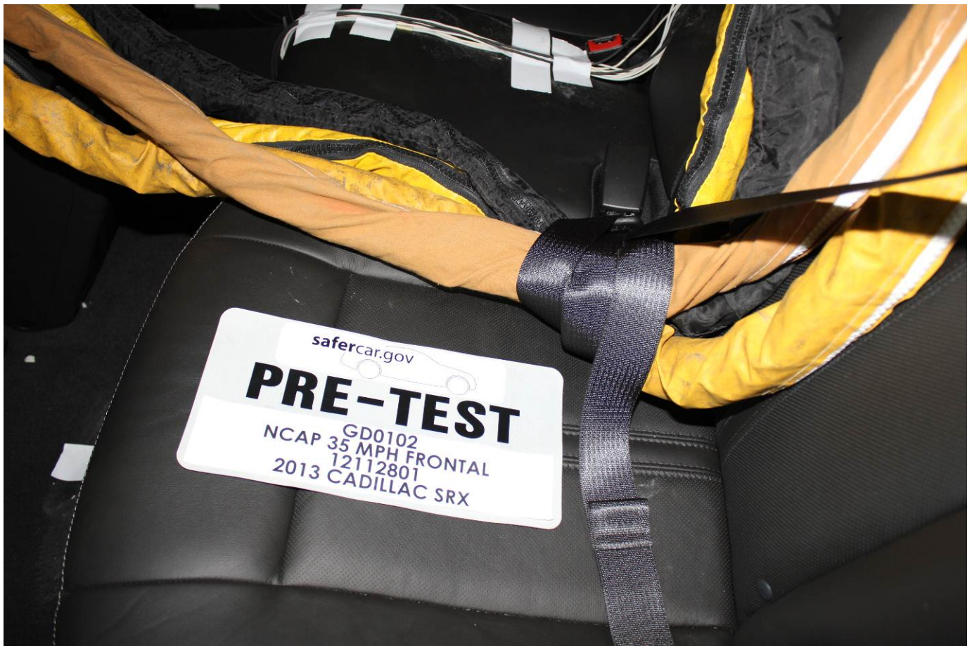
Pre-Test Dummy Cable Routing
