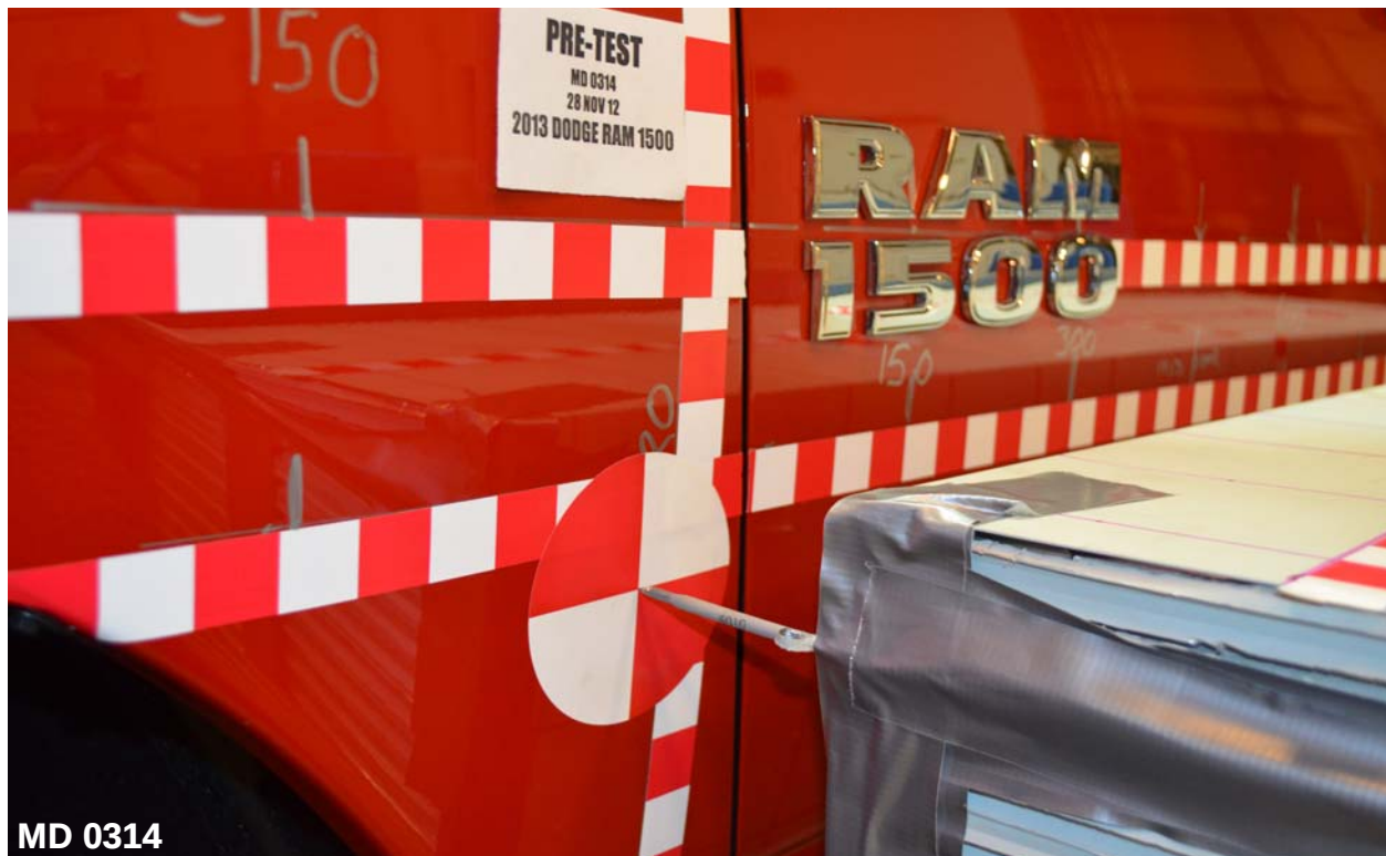
Figure A-19: Pre-Test Close-Up View of Impact Point Target
