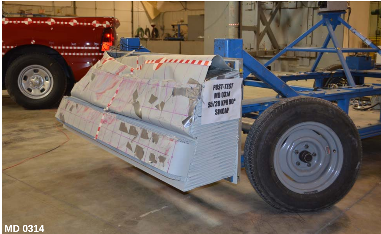
Figure A-89: Post-Test Left Side View of MDB Impactor Face
