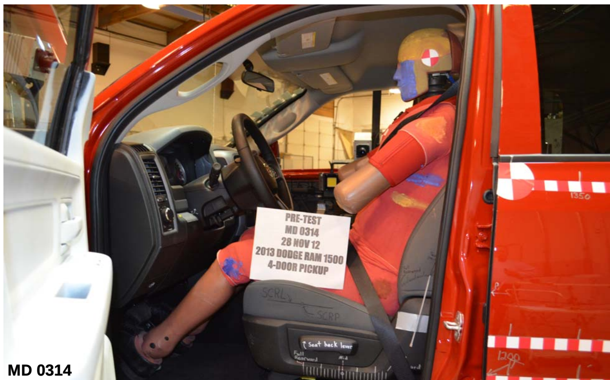
Figure A-27: Pre-Test Left Side View of Driver Dummy Showing Belt and Chalking
