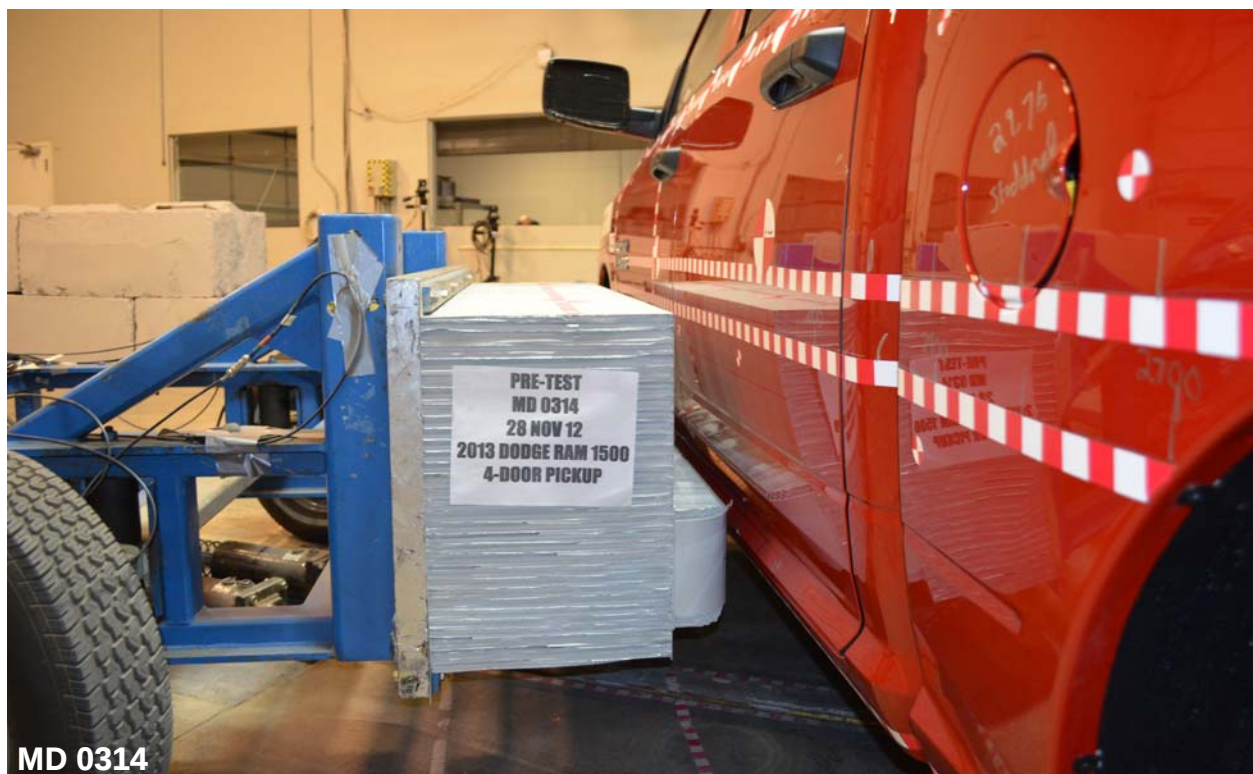
Figure A-18: Pre-Test Right Side View of MDB Positioned Against Side of Test Vehicle
