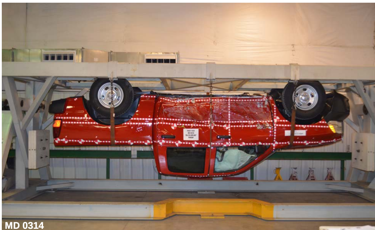
Figure A-98: FMVSS No. 301 Static Rollover 180 Degrees
