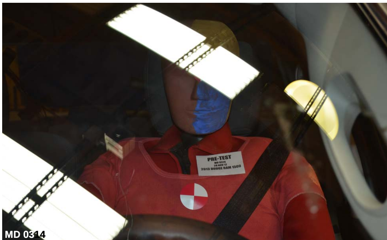
Figure A-31: Pre-Test Frontal View of Driver Dummy Head and Shoulders in Relation to Head Restraint
