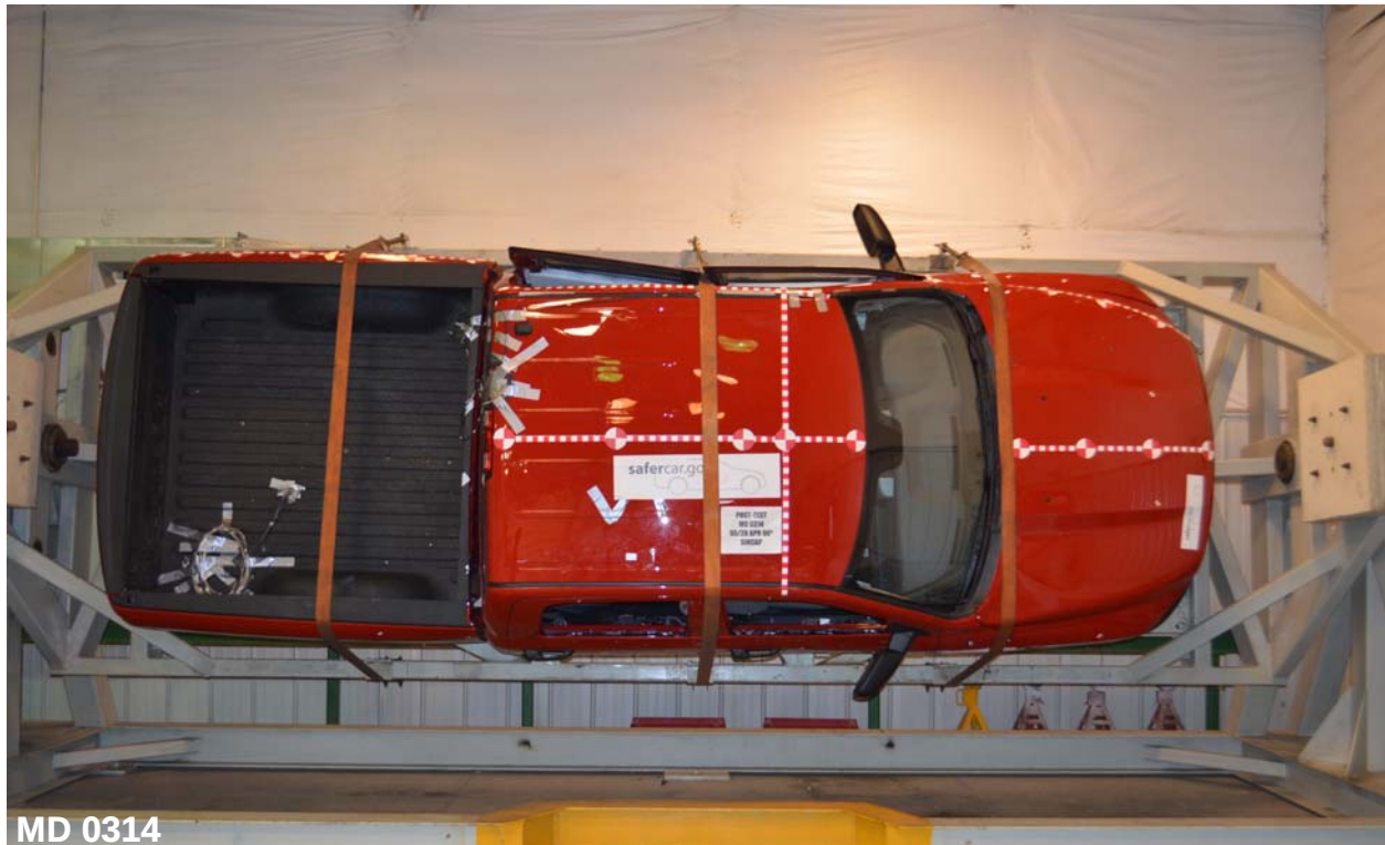
Figure A-99: FMVSS No. 301 Static Rollover 270 Degrees
