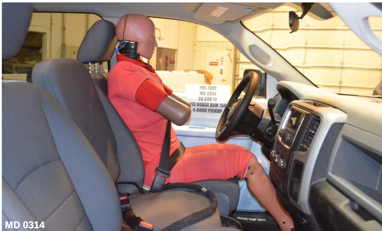
Figure A-44: Pre-Test Right Side View of Driver Dummy and Front Seat of Occupant Compartment
