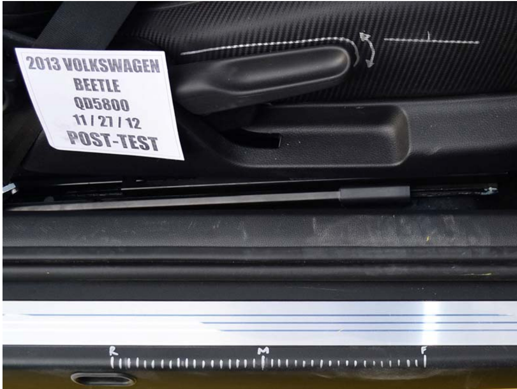
FIGURE 57. Post-Test Passenger's Seat Fore-Aft Markings
