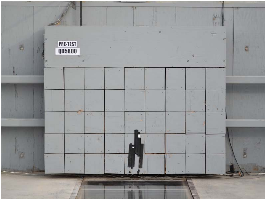
FIGURE 2. Load Cell Wall
