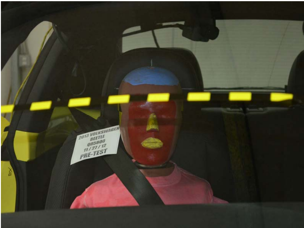
FIGURE 50. Pre-Test Passenger Dummy Front View
