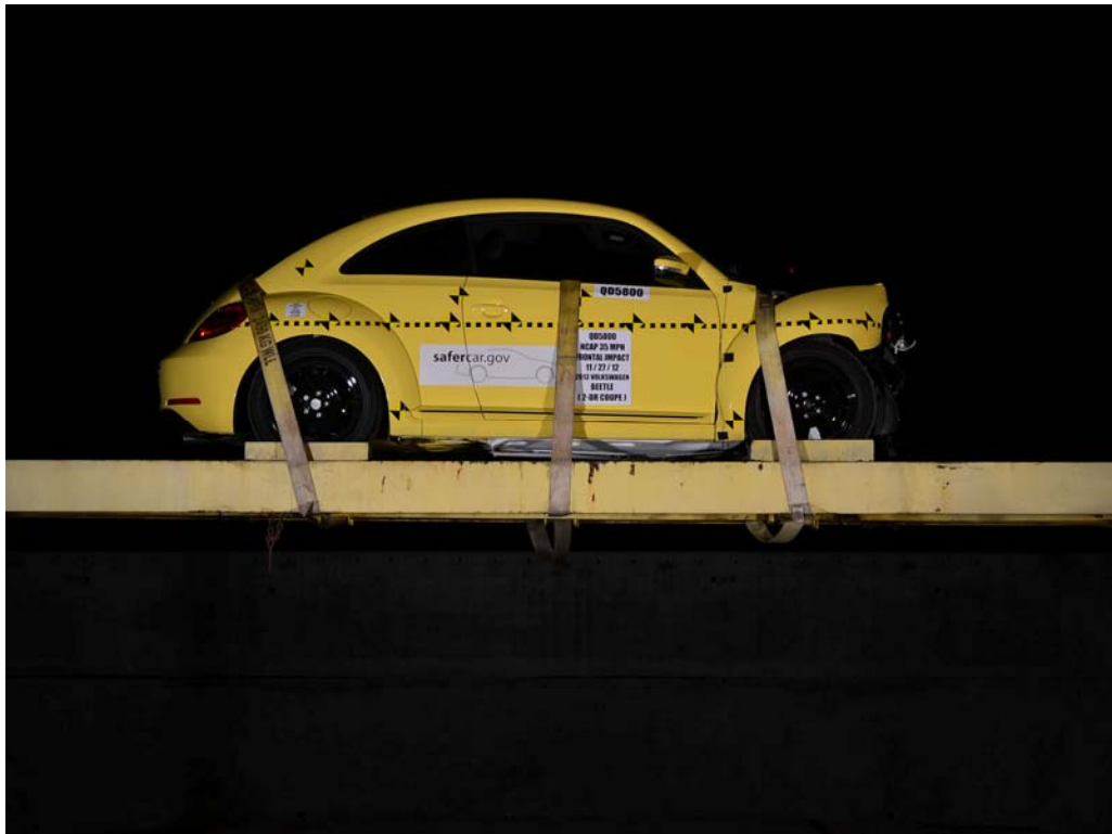
FIGURE 70. Vehicle at 0° on Static Rollover Device
