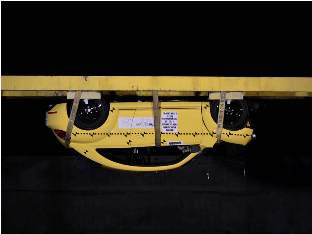
FIGURE 72. Vehicle at 180° on Static Rollover Device
