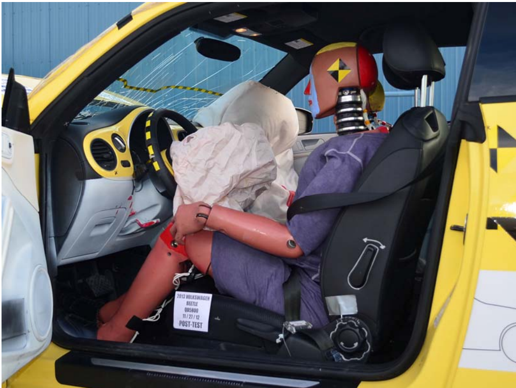
FIGURE 34. Post-Test Driver Dummy and Vehicle Interior View
