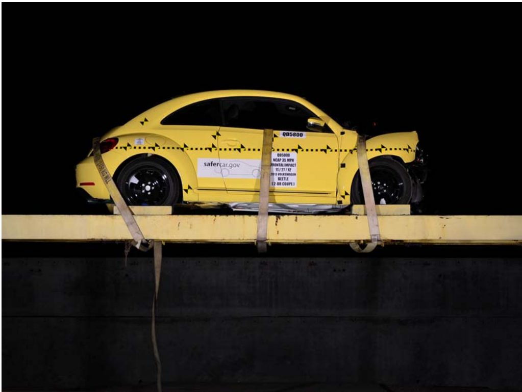
FIGURE 74. Vehicle at 360° on Static Rollover Device
