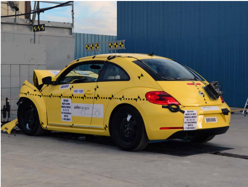
FIGURE 16. Post-Test Left Rear \frac{3}{4} View
