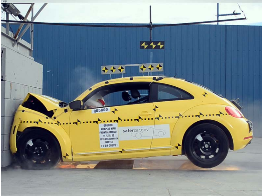
FIGURE 75. 2013 Volkswagen Beetle Frontal Impact Event
