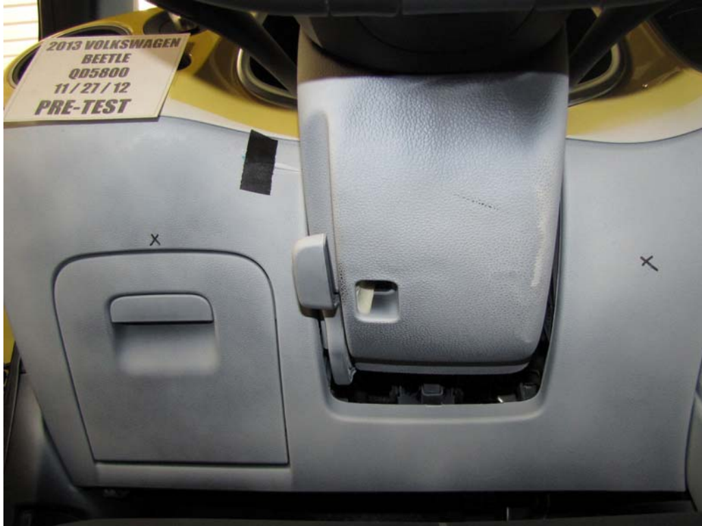
FIGURE 41. Pre-Test Driver's Side Knee Bolster
