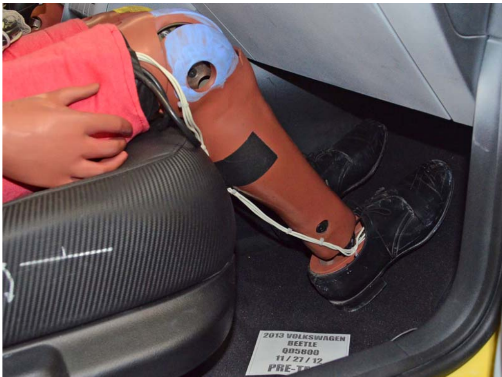
FIGURE 60. Pre-Test Passenger Dummy Feet
