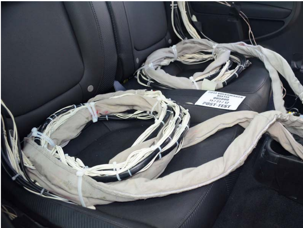
FIGURE 28. Post-Test Dummy Cable Routing
