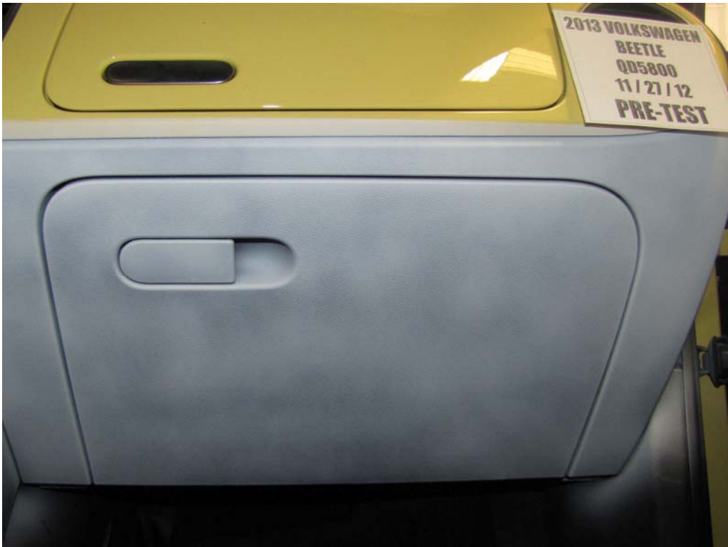
FIGURE 62. Pre-Test Passenger's Side Knee Bolster
