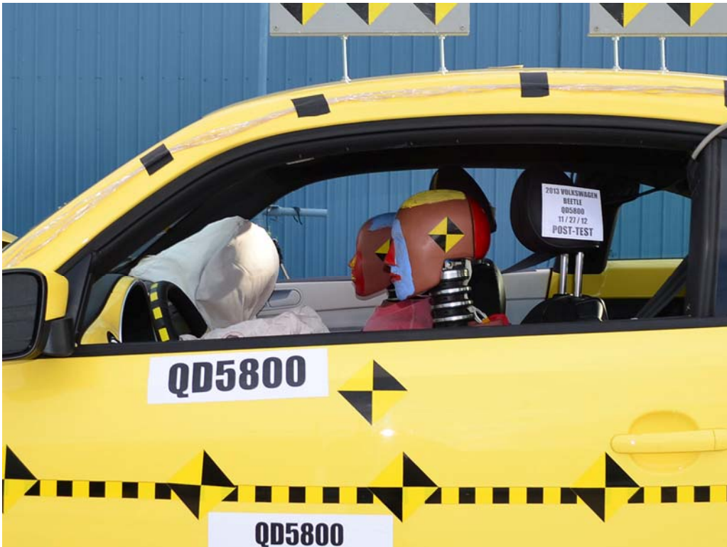
FIGURE 32. Post-Test Driver Dummy Window View
