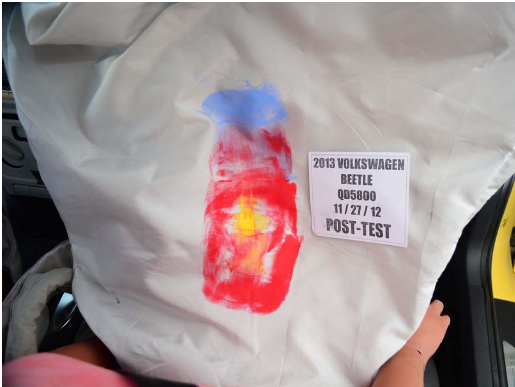
FIGURE 66. Post-Test Passenger Dummy Contact With Airbag
