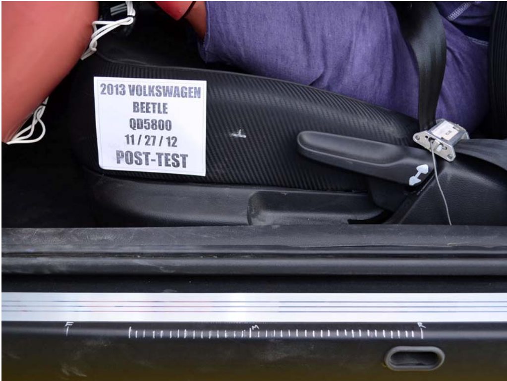
FIGURE 36. Post-Test Driver's Seat Fore-Aft Markings
