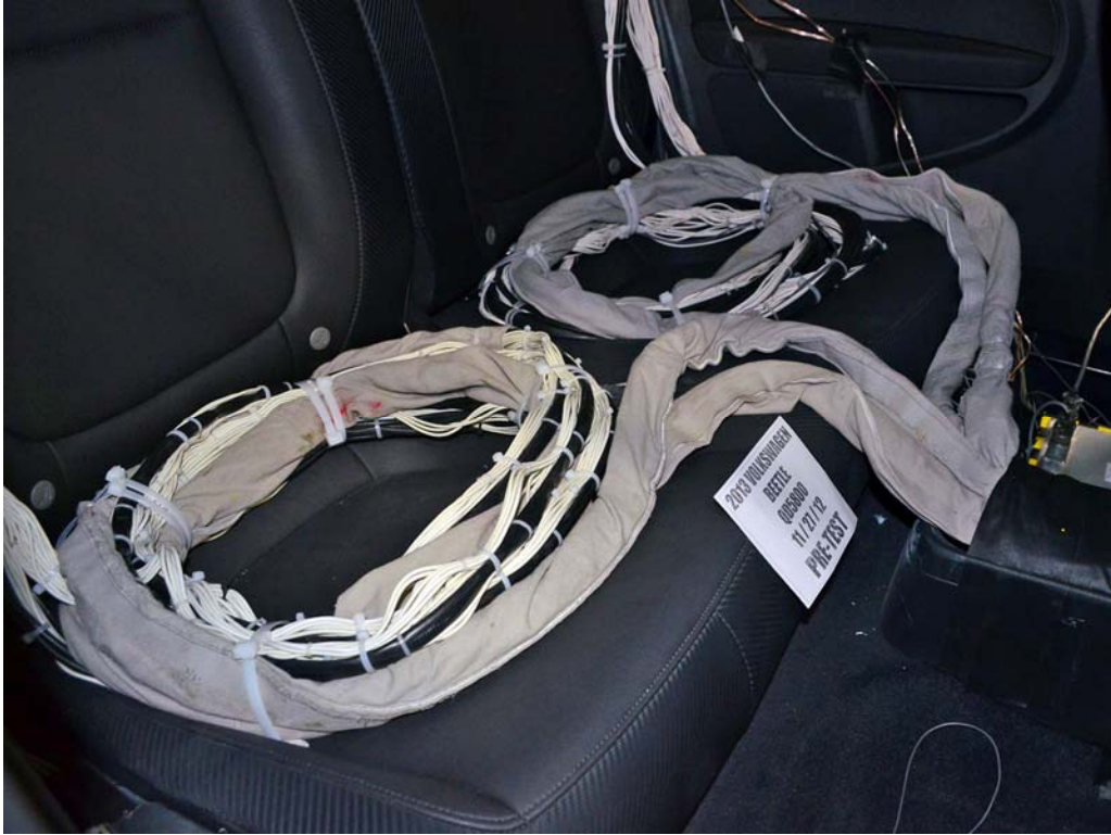
FIGURE 27. Pre-Test Dummy Cable Routing
