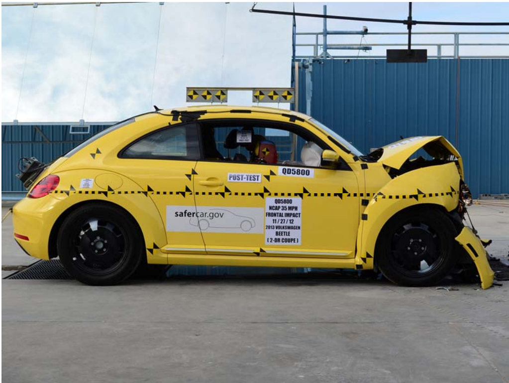
FIGURE 12. Post-Test Right View of Test Vehicle
