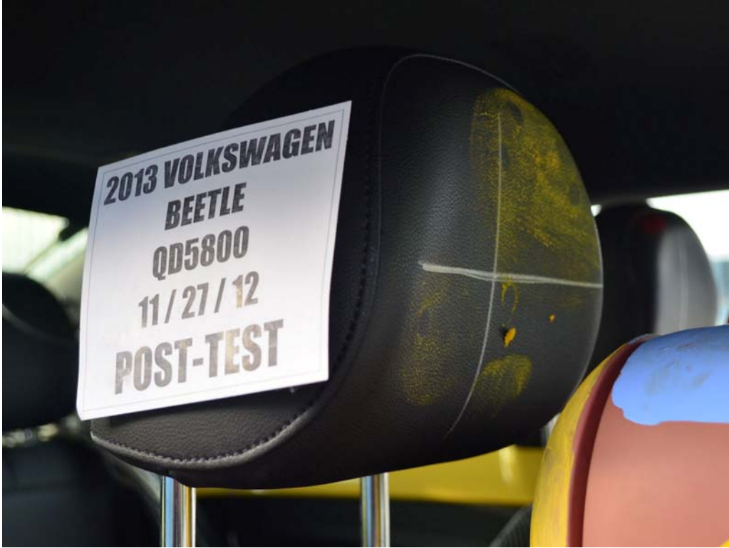
FIGURE 66a. Post-Test Passenger Dummy Contact With Headrest
