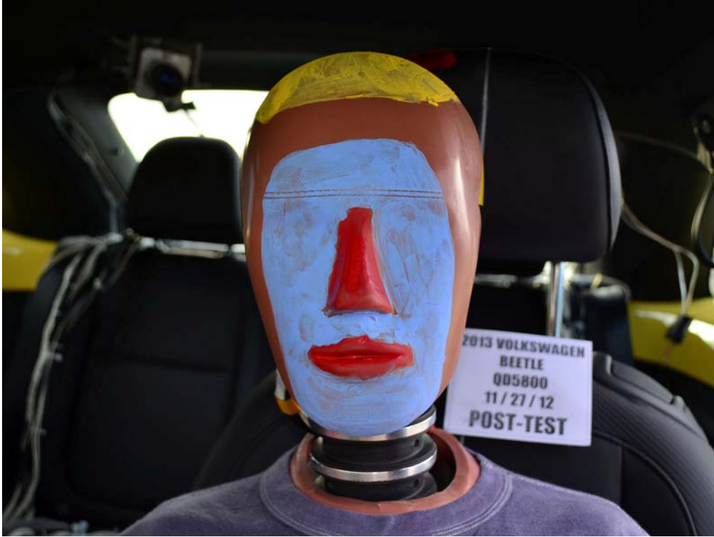
FIGURE 45. Post-Test Driver Dummy Face
