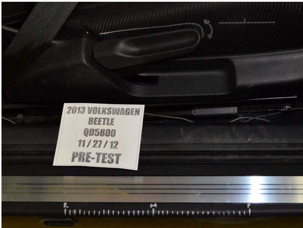
FIGURE 56. Pre-Test Passenger's Seat Fore-Aft Markings
