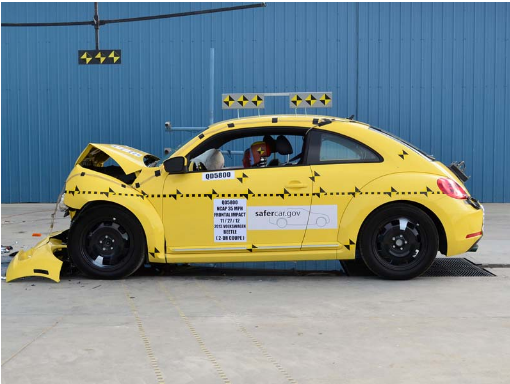
FIGURE 10. Post-Test Left View of Test Vehicle
