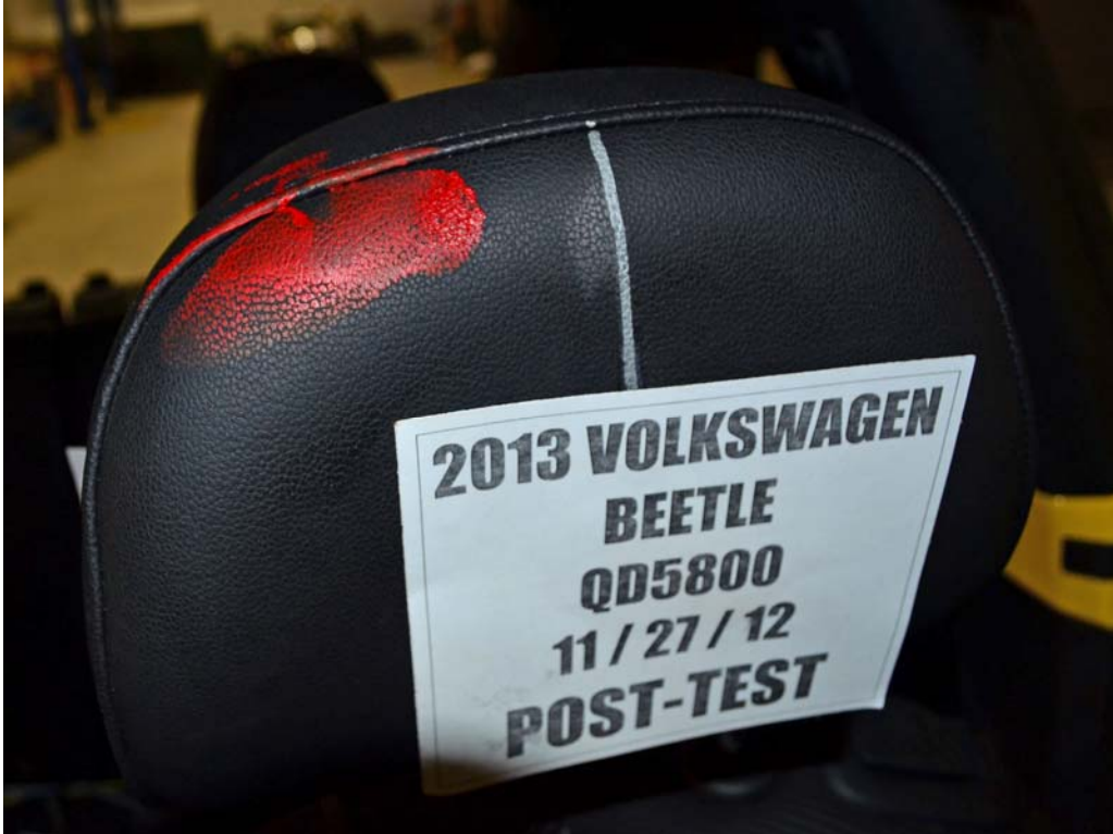
FIGURE 47. Post-Test Driver Dummy Contact With Headrest
