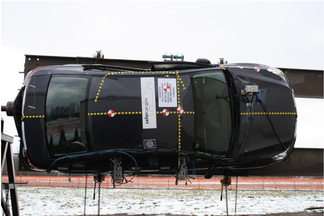
Figure A-97: FMVSS No. 301 Static Rollover 90 Degrees
