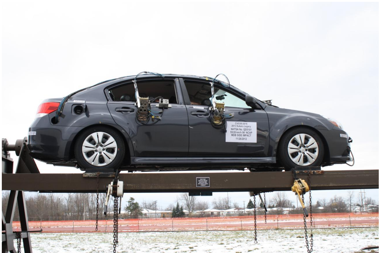
Figure A-96: FMVSS No. 301 Static Rollover 0 Degrees
