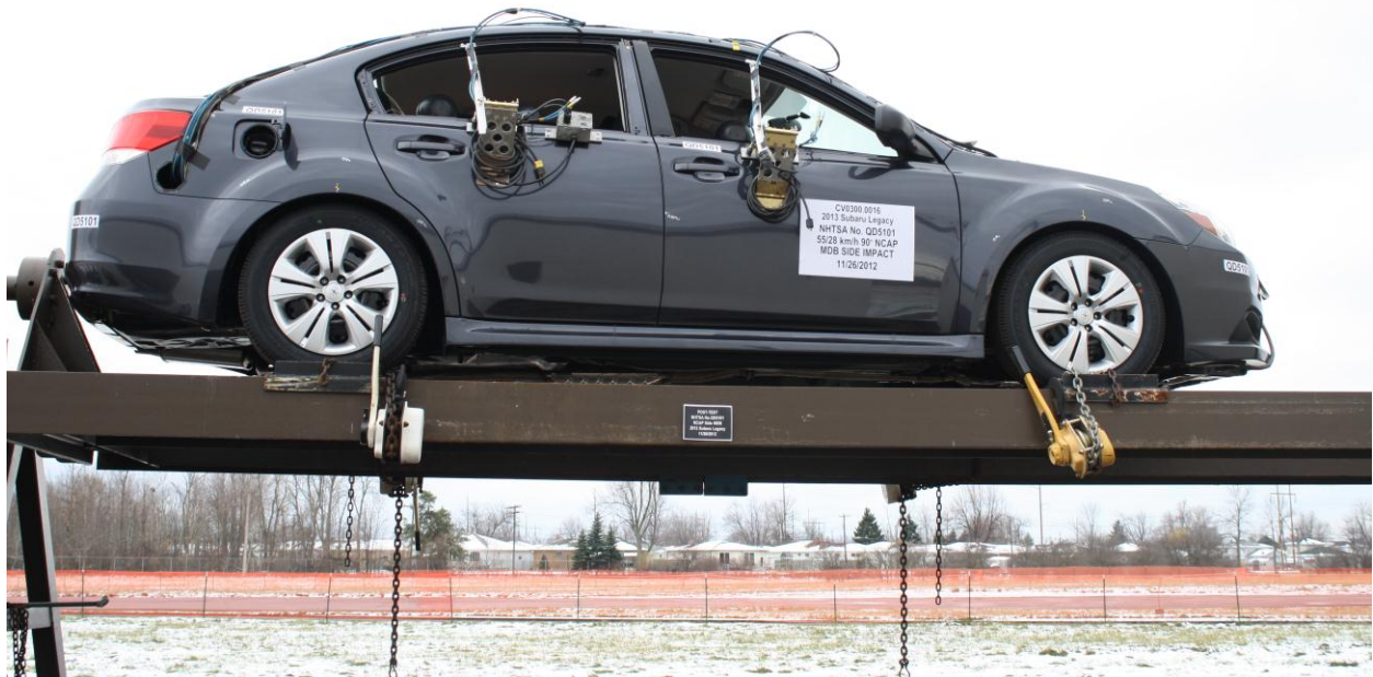
Figure A-100: FMVSS No. 301 Static Rollover 360 Degrees
