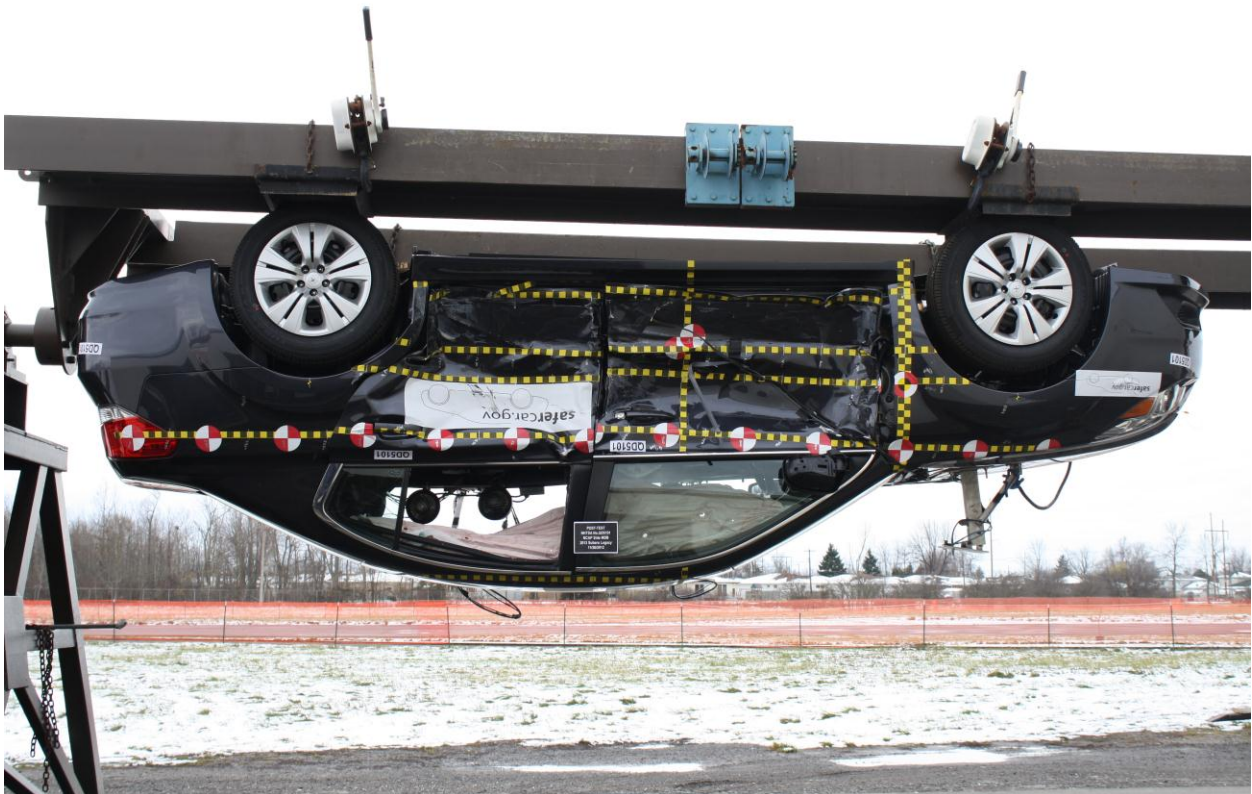
Figure A-98: FMVSS No. 301 Static Rollover 180 Degrees
