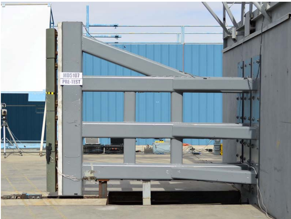
FIGURE 59. Pre-Test Pole Barrier Side View
