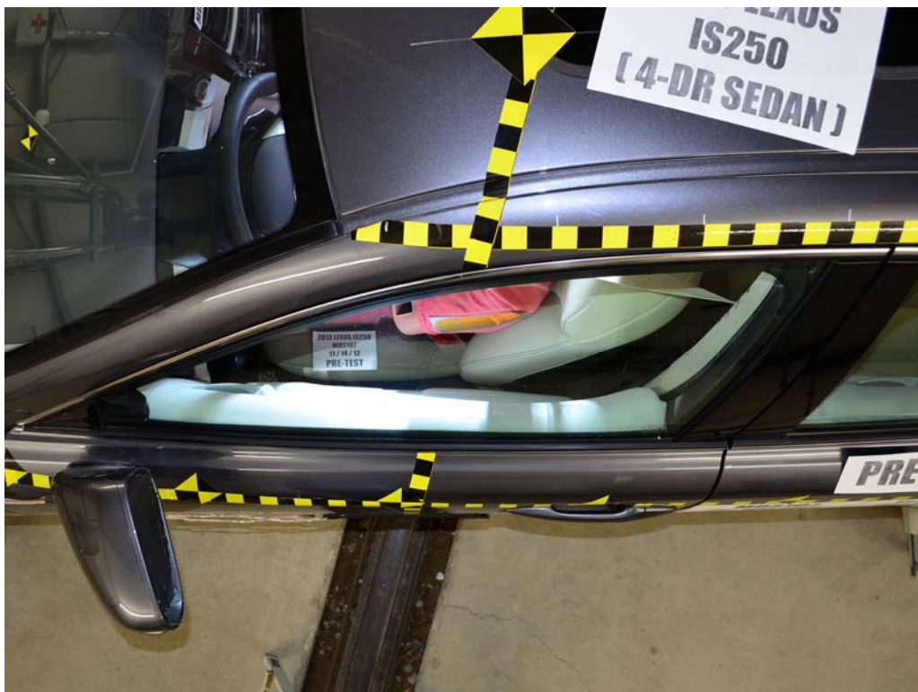
FIGURE 40. Pre-Test Dummy and Door Clearance
