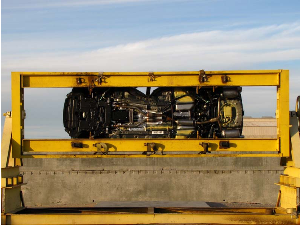
FIGURE 66. FMVSS No. 301 Rollover 270 Degrees
