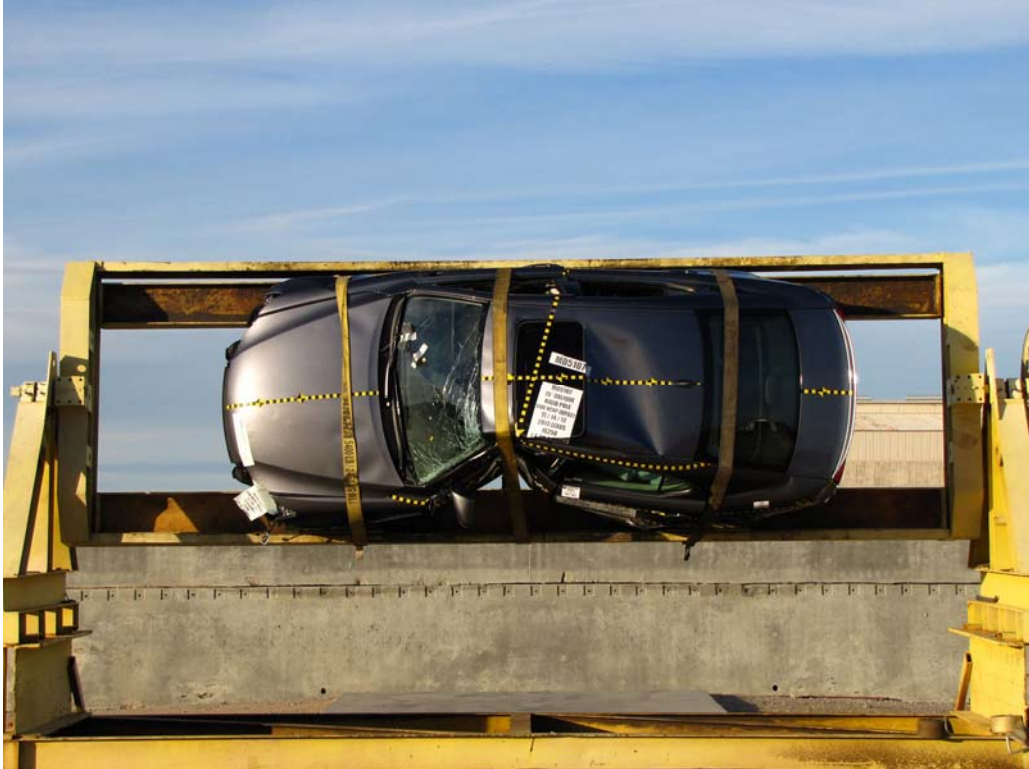
FIGURE 64. FMVSS No. 301 Rollover 90 Degrees
