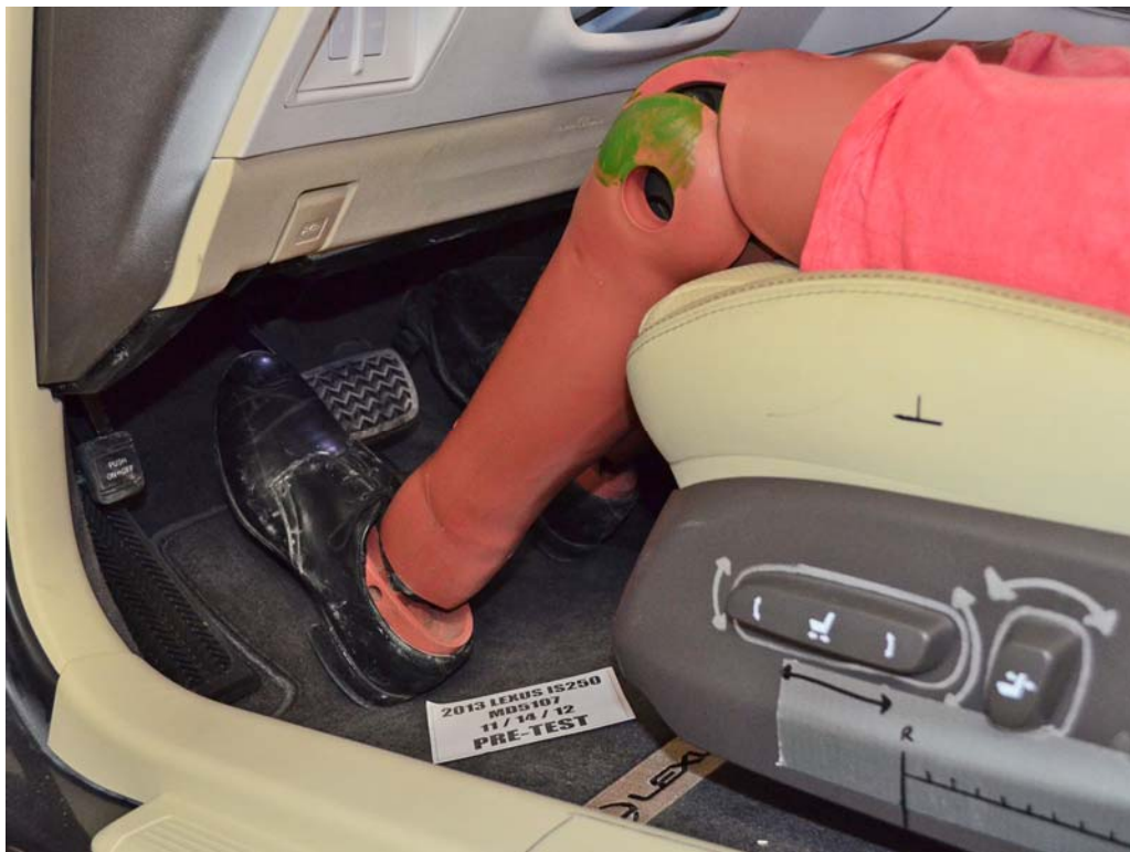
FIGURE 32. Pre-Test Placement of Dummy's Feet
