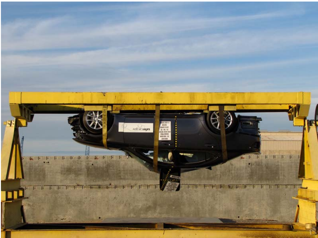
FIGURE 65. FMVSS No. 301 Rollover 180 Degrees
