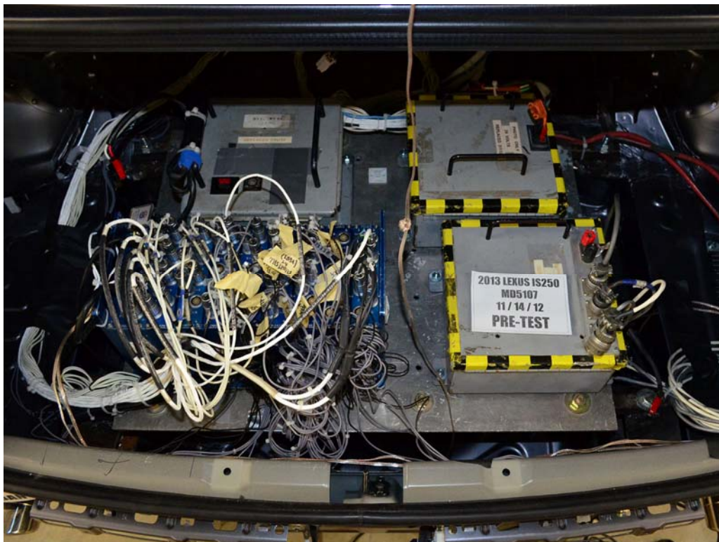
FIGURE 61. Pre-Test Ballast View
