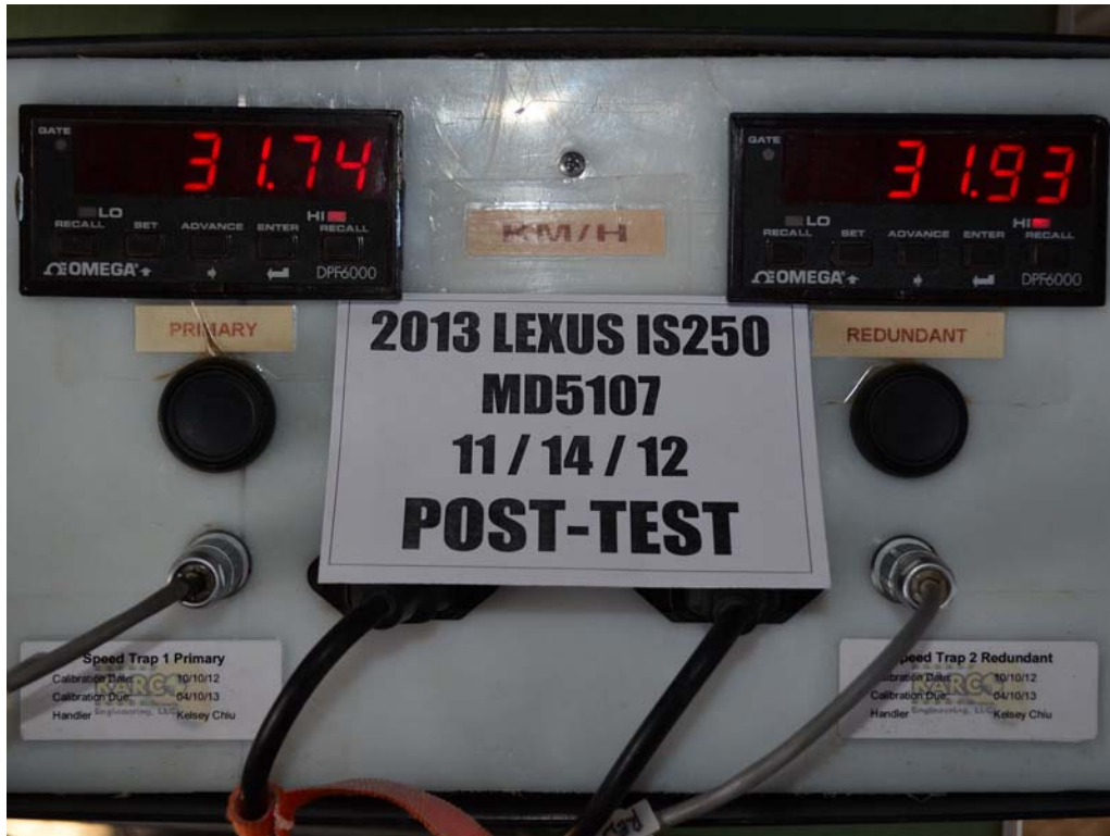
FIGURE 62. Post-Test Primary and Redundant Speed Trap Read-Out
