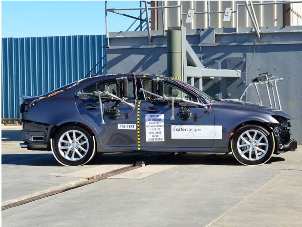
FIGURE 13. Pre-Test Right Side View of Test Vehicle
