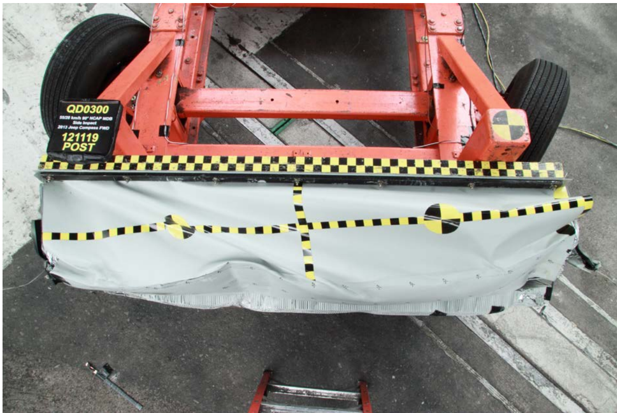
087 Post-Test Top View of MDB Impactor Face
