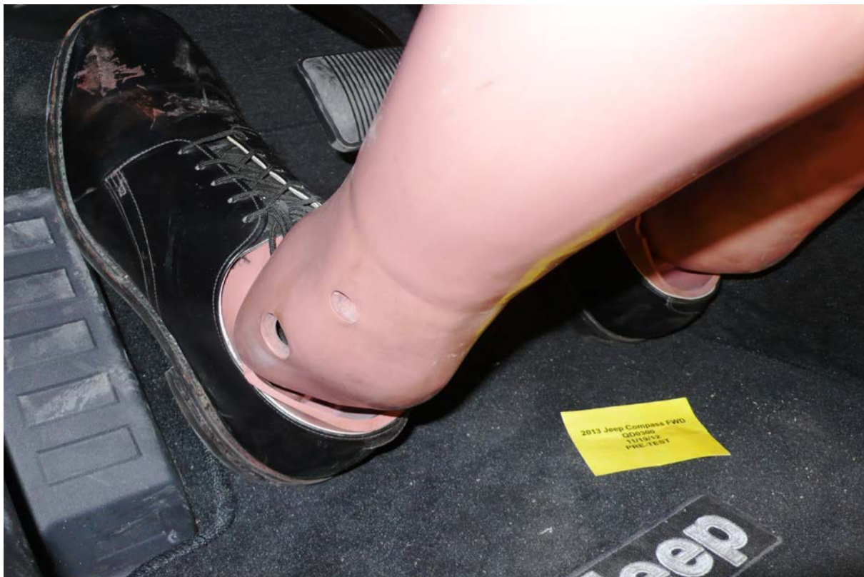
034 Pre-Test Placement of Driver Dummy Feet
