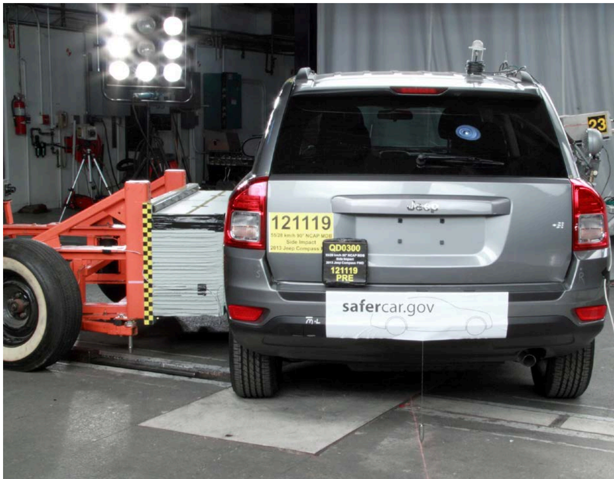
018 Pre-Test Right Side View of MDB Positioned Against Side of Test Vehicle
