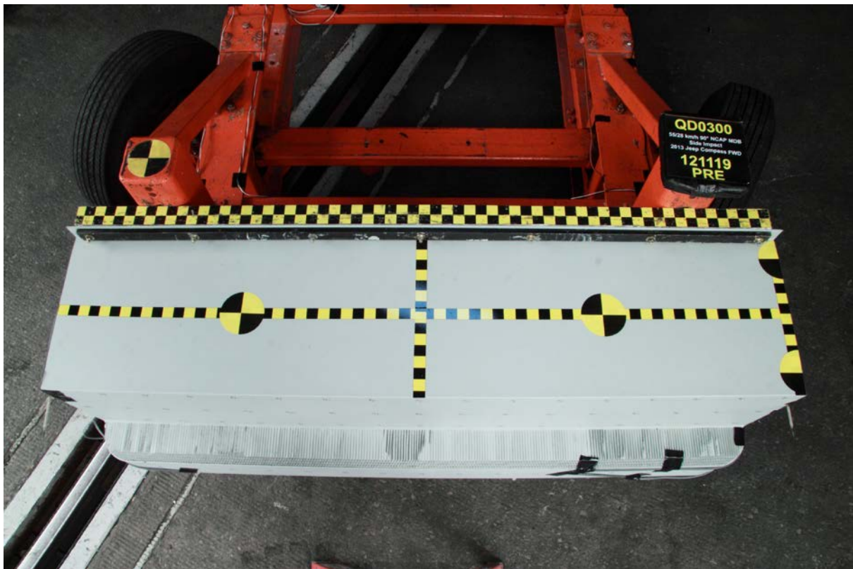
086 Pre-Test Top View of MDB Impactor Face
