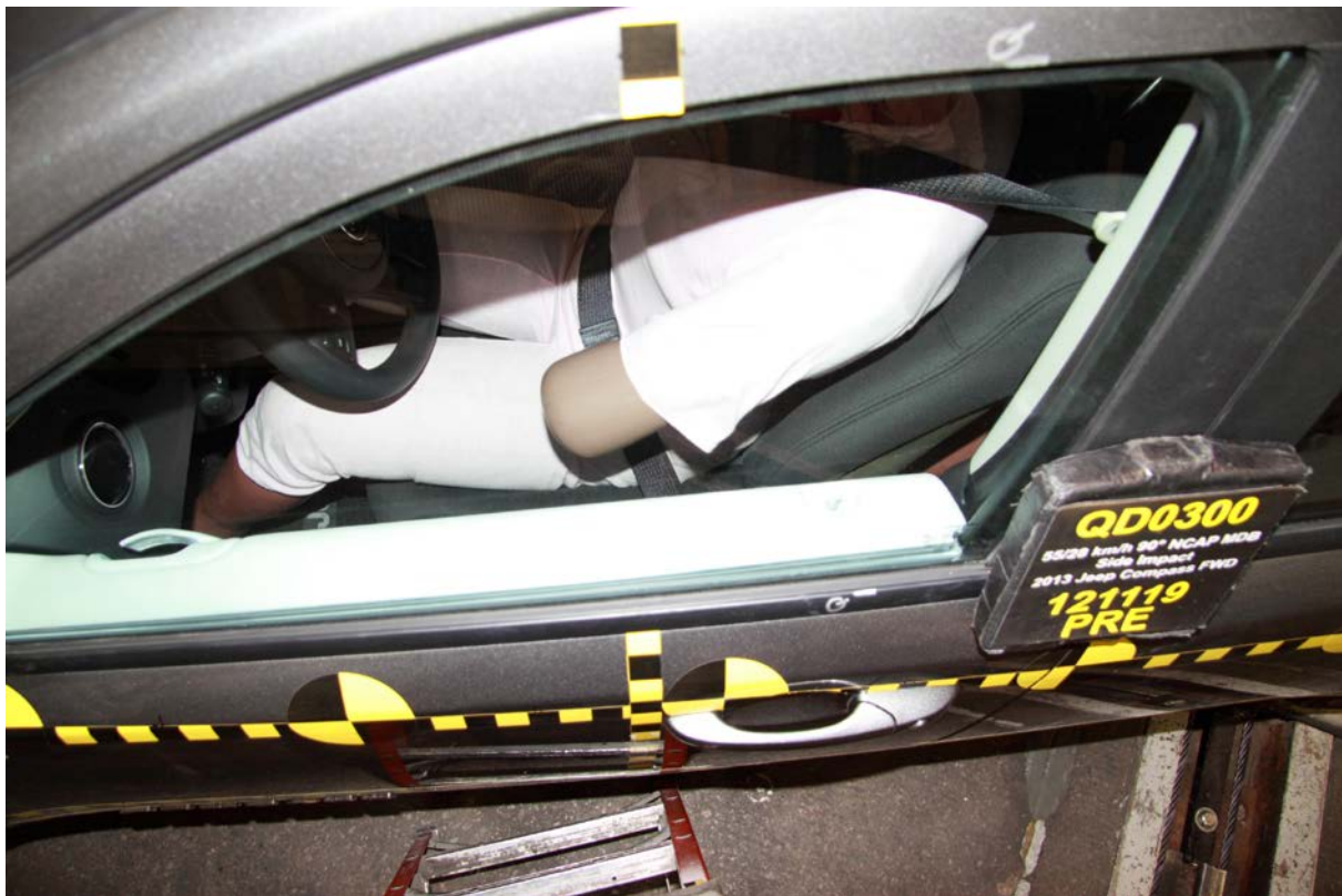
042 Pre-Test Driver Dummy and Door Clearance View
