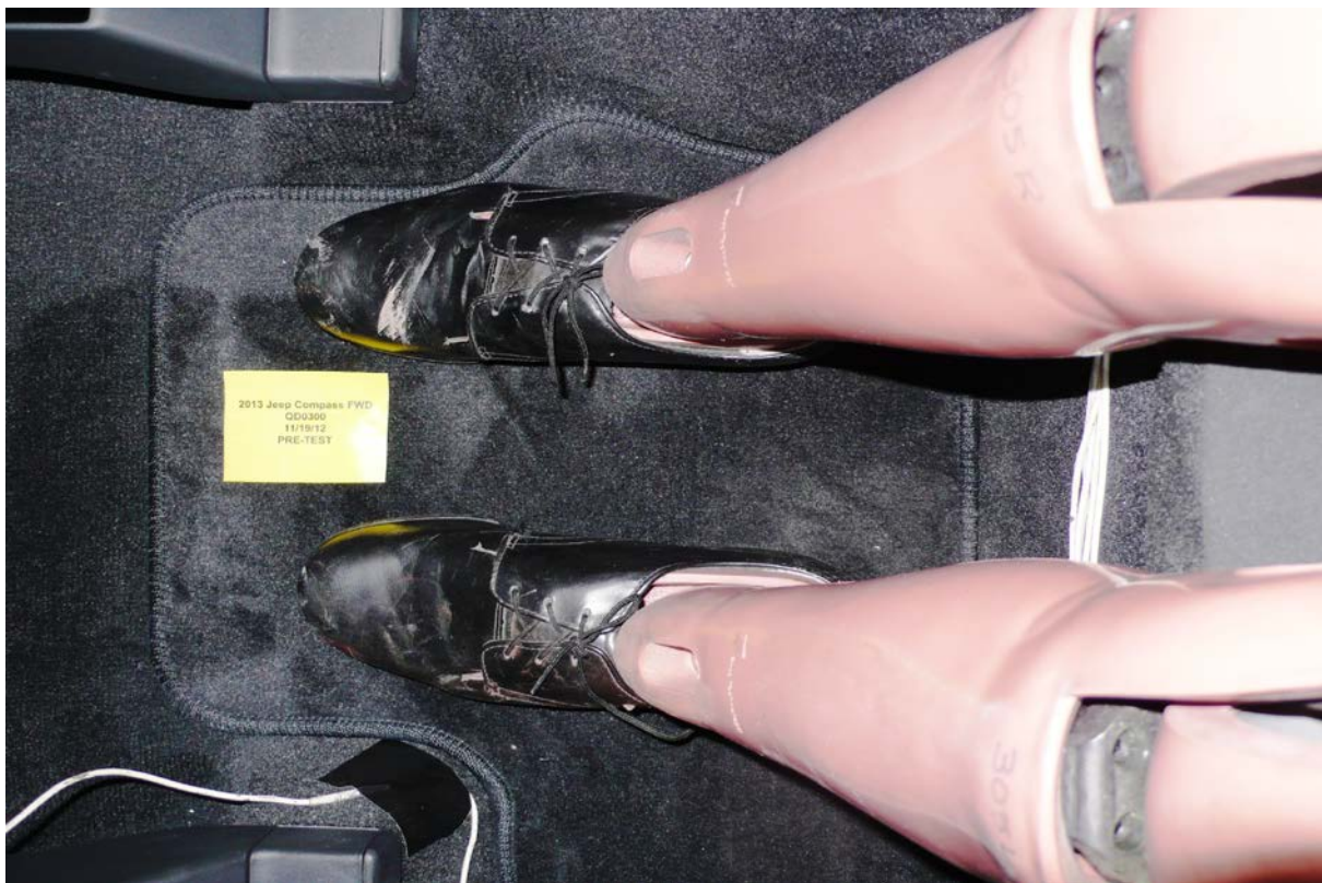
064 Pre-Test Placement of Rear Passenger Dummy Feet
